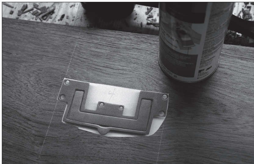
Fig. 4.38 Scans. Scan each pull and print out its image. Cut it free from the paper and spray it with adhesive. Stick each in place on the drawer front.
