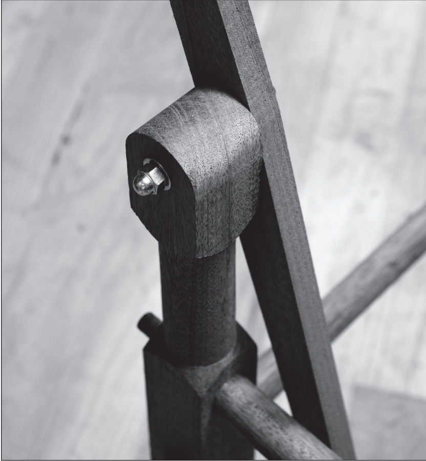
Fig. 7.18 Woodwork done. The back pieces have shallow tapers that face the sitter. Attach the back to the frame of the chair using bolts, washers and nuts. The acorn nut shown in the photo is temporary.
