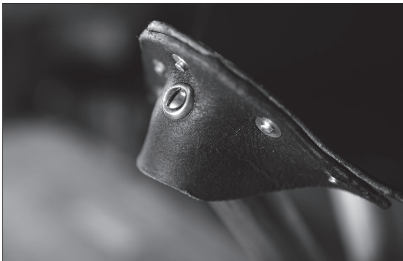
Fig. 6.16 Finishing washers. The brass washer gives the screw head some extra bite into the leather – and it looks nice, too.
