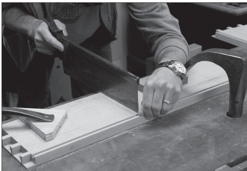
Fig. 11.3 Saw the walls. Place your thumb in the groove to stop your saw as you saw each wall of the dado.
