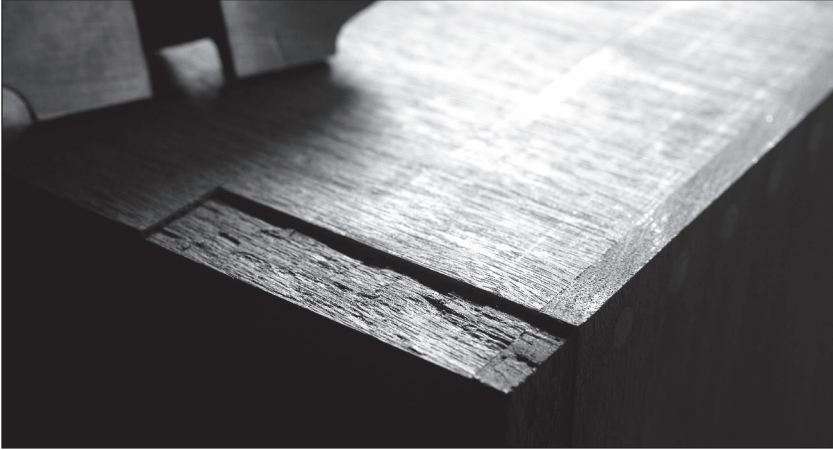
Fig. 3.15 Clean your bottom. A small router plane is – hands down – the best tool for this job. You can make one from an Allen key and a piece of Lexan if you are a cheapskate.
