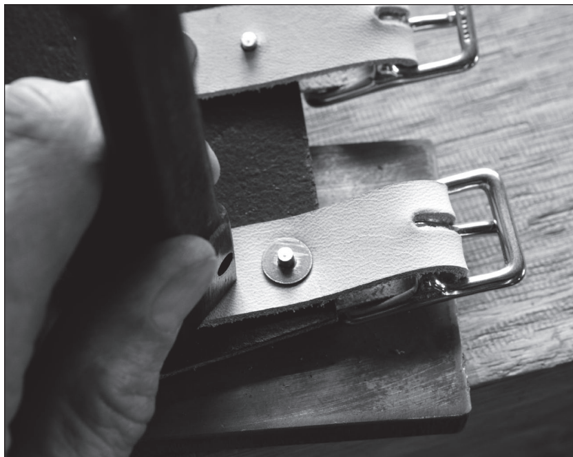
Fig. 7.28 Set the burr. After you place the burr on the post of the rivet, you need to push it down to pinch the leather bits. Do this with a rivet setter. Most rivet setters have a hole designed for this operation.
