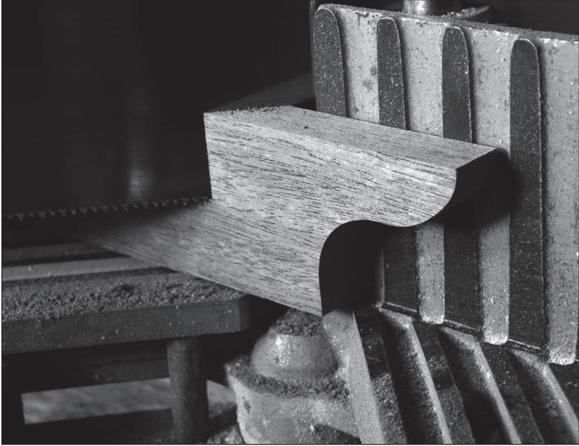
Fig. 8.26 Shape, then cut. First cut the ogee shape into the foot when it is part of a longer piece. This makes it easier to clamp and work. Then miter the corner.
