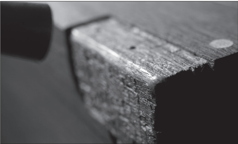
Fig. 3.22 Whack to fit. After installing hundreds of these bits of brass, I typically beat the corners into submission. But then, I love hammers.
