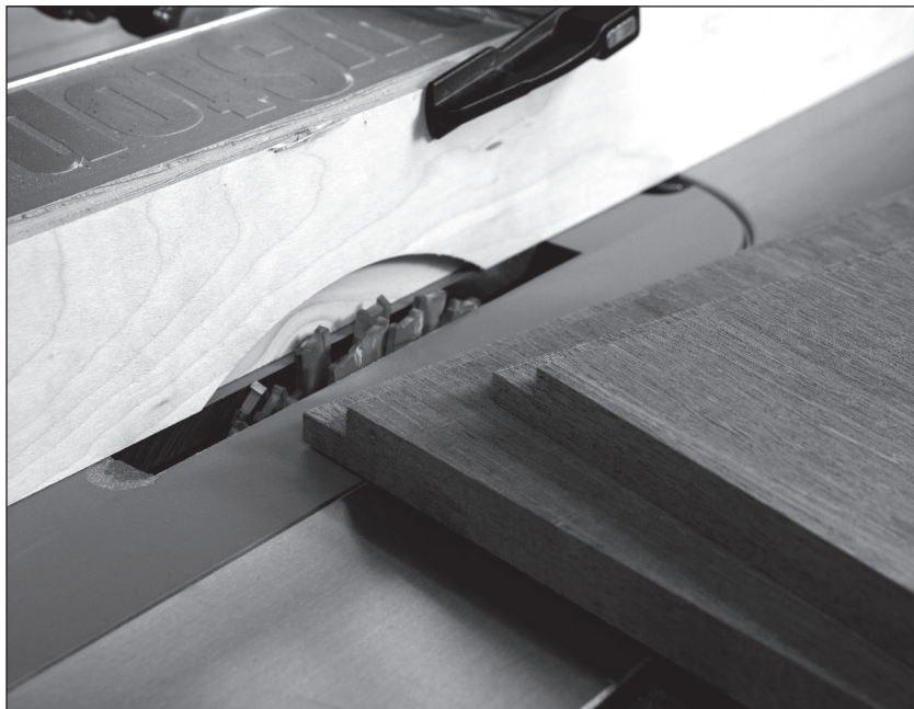
Fig. 8.4 Rabbeted ends. The cross-grain rabbets wrap around the ends. I cut these joints using a dado stack in my table saw.
