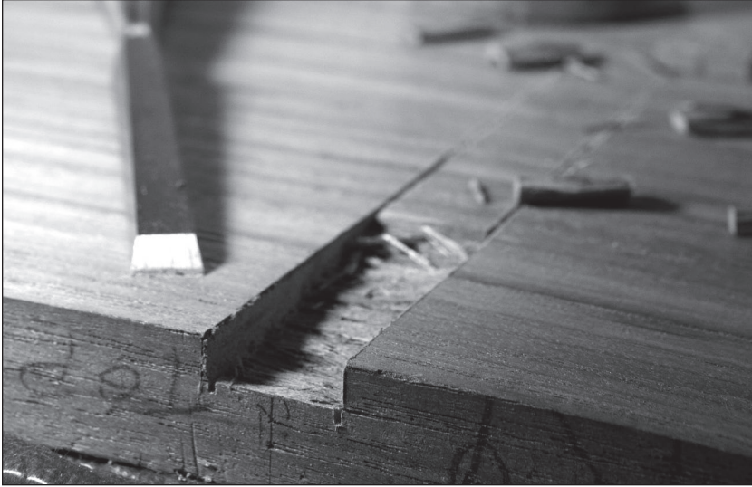
Fig. 4.17 For the vertical divider. This is a quick joint to cut by hand. Saw the walls of the dado, rip out the waste with a chisel and flatten the bottom of the dado with a router plane if necessary.
