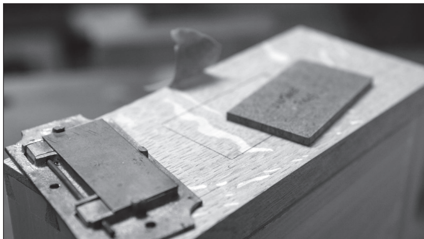
Fig. 3.26 A hardboard guide. A simple template from hardboard can guide the first stage in installing pulls.
