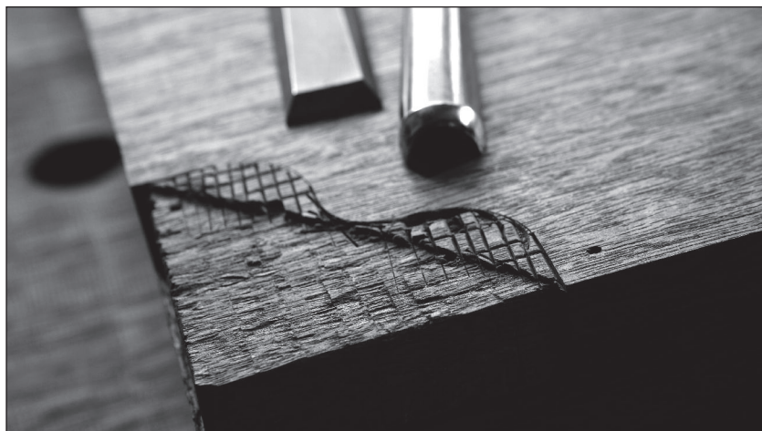
Fig. 3.24 Gouges for ogees. When the shape becomes more complex, I usually just clean up the recesses by hand. With some care, a straight chisel and a carving gouge can do the job.
