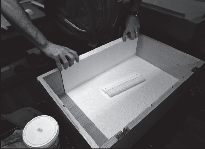
Fig. 11.21 Paste then trim. Use one piece of paper on the sides of the carcase. After the paste has dried 24 hours, use a knife to slice away the paper covering the dados.
