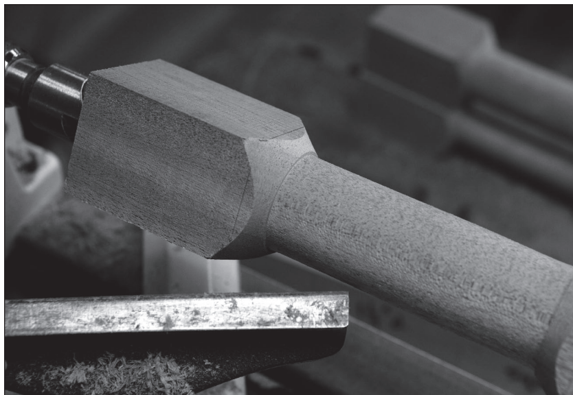
Fig. 7.5 Tough cut. This transition from square to round is tricky if you are aggressive. It's easy to splinter the exterior surface of the leg. Light cuts, and a tool with a radiused cutting tip, can make it easier for a beginning turner.
