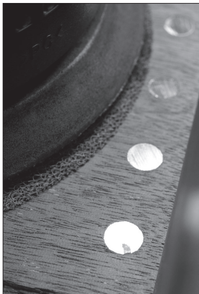
Fig. 8.20 A little abrasive action. When you reach the screw slot, you can move things along a little faster with a random-orbit sander and some #120-grit sandpaper.
