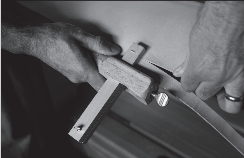
Fig. 7.20 A slitter. This leather-slitting tool works a bit like a table saw. You move the fence of the tool away from the cutter ( 3/4 " in this case) and feed the leather between the fence and cutter and it will make leather straps all day long. You can usually cut up an entire side of a cow into ribbons before resharpening or replacing the cutter.
