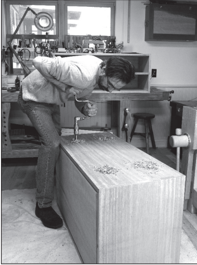
Fig. 4.23 Bigger bits. Drill stopped holes that are the same diameter as your dowels.
