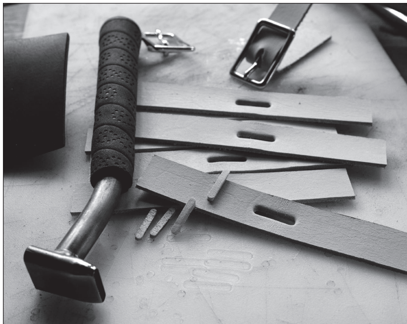
Fig. 7.25 Shortcut. If you plan to make a lot of these chairs, purchase a special punch that will make the oval orifice needed for the buckle. The leather piece is 5-1/2", folded over in the middle of its length and moistened in the mouth. Yum.
