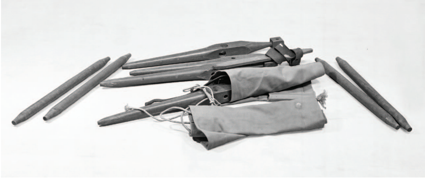
Fig. 1.56 Tapers. Here you can see the tapered tenons on the stretchers that go into tapered mortises. (Courtesy of the Council of the National Army Museum, London)
