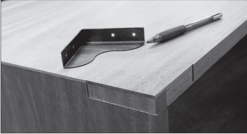
Fig. 3.21 Two legs relieved. When installing the top corners, first cut away the two legs of the hardware. That allows you to get the hardware in place to trace the profile on the carcass.
