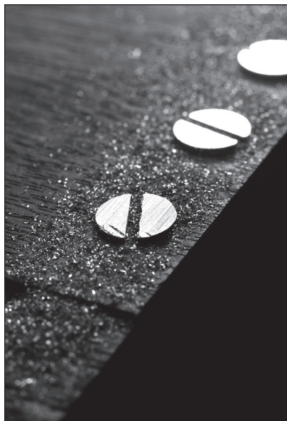
Fig. 8.19 Slow & steady. After 10 minutes of filing, you will reach the bottom of the slot. Then you have to clean up your work deliberately in order to avoid gouging the surrounding wood.
