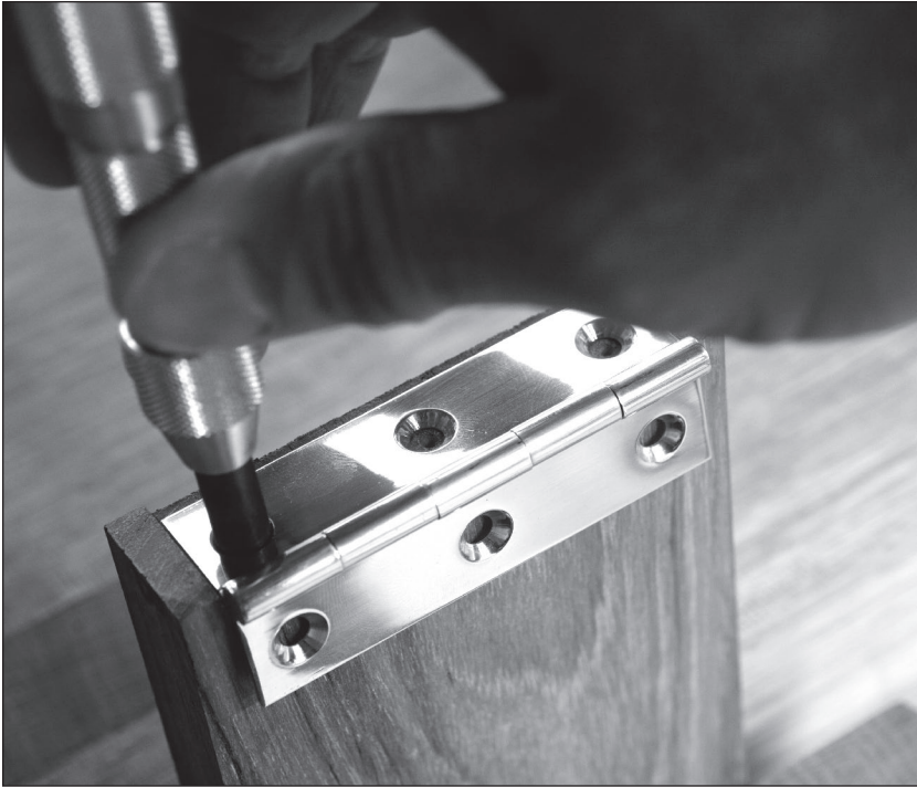
Fig. 9.10 Punch it. When you have lots of hinges to install, a center punch is quite handy. I think this tool is superior to a hinge-installation bit because the point never breaks.
