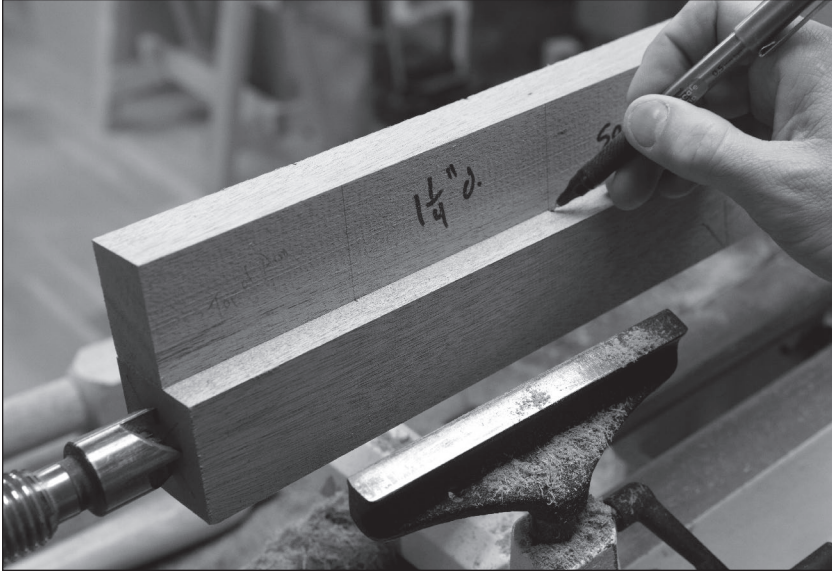
Fig. 7.3 A simple template. Here my story stick is sitting on a leg blank chucked into the lathe. Mark out the sections of your turning on the leg blanks.
