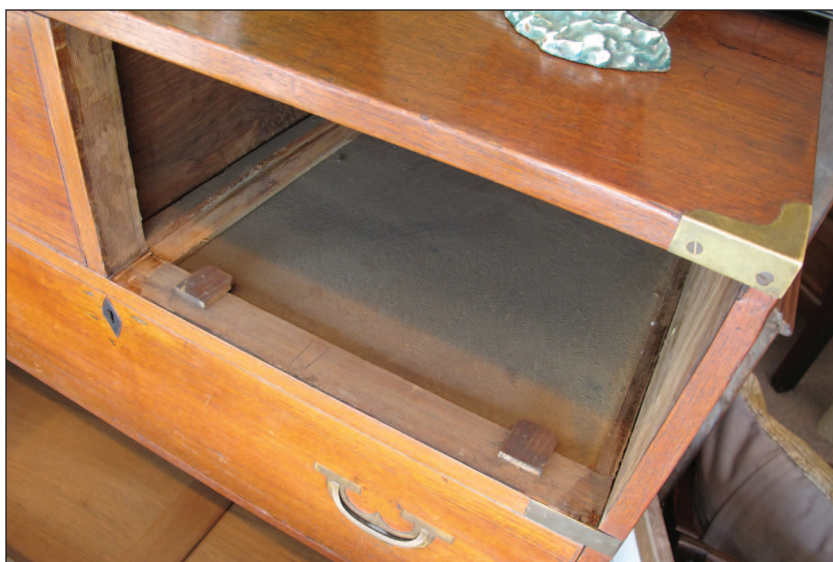
Fig. 1.26 Inside a chest. You can see the web frame and dust panel inside this vintage campaign chest. Also, note the locations of the drawer stops, which keep the drawer front flush to the frame of the carcass.
