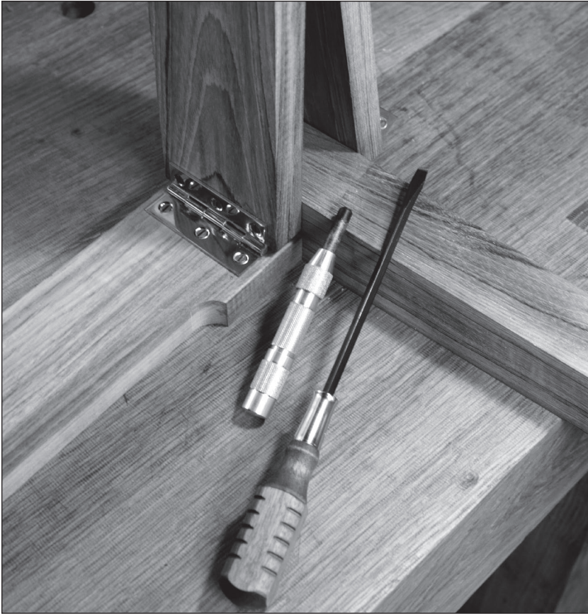
Fig. 9.13 Easy installation. Push the folding apron into this position. Punch in your screw centers. Drill your pilots. Screw. Done.
