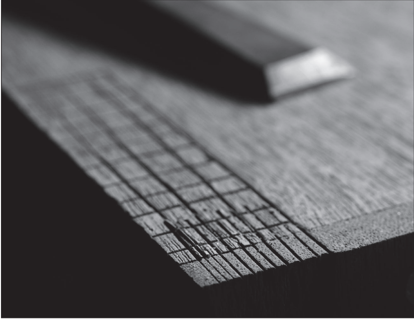
Fig. 8.24 Chop with care. At times you will chop a combination of face grain and end grain. If you get too aggressive, you can split both. Always begin with light chops until you have a feel for the grain.
