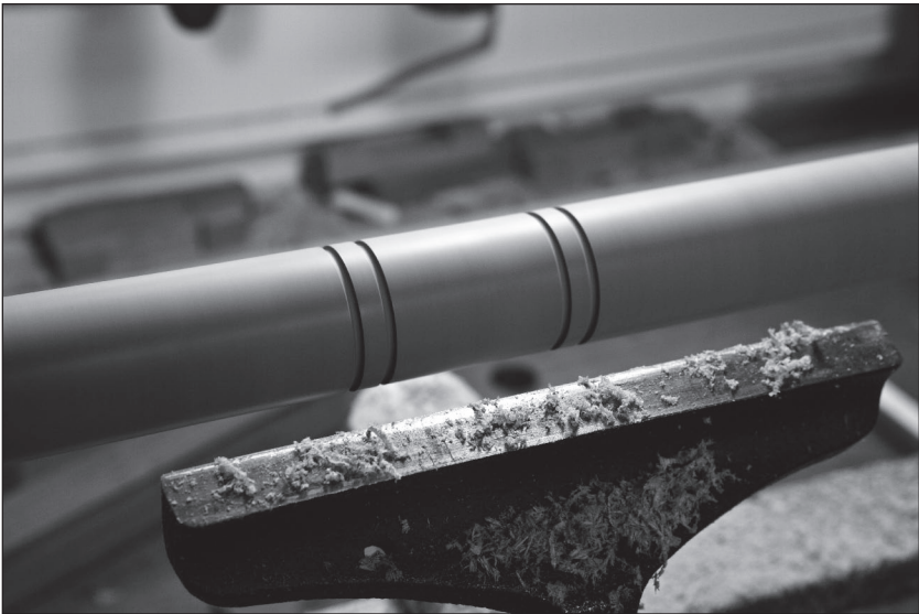
Fig. 6.4 Not original. These little grooves add some visual interest to the joint. However, they're not a detail I found on any original stool. So skip them if you are going for authenticity.
