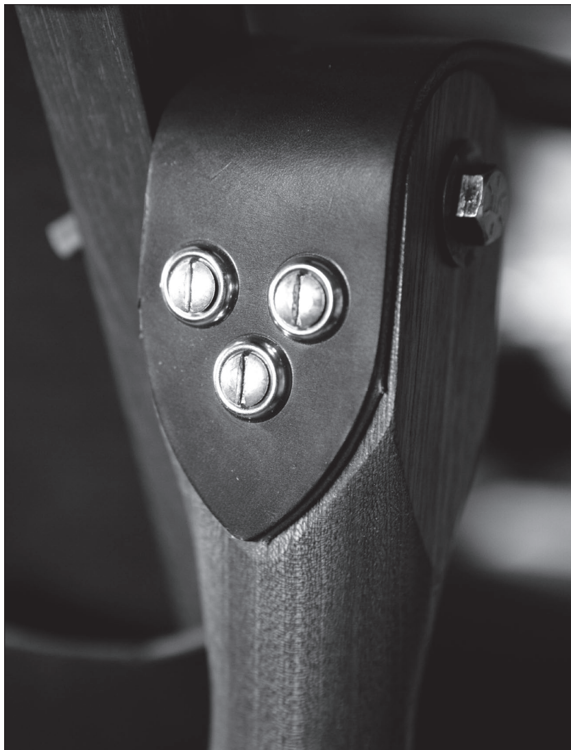
Fig. 7.31 Screws instead of studs. These No. 8 x 1-1/2" brass screws with finishing washers are a simple and strong way to secure the armrest to the rear legs.
