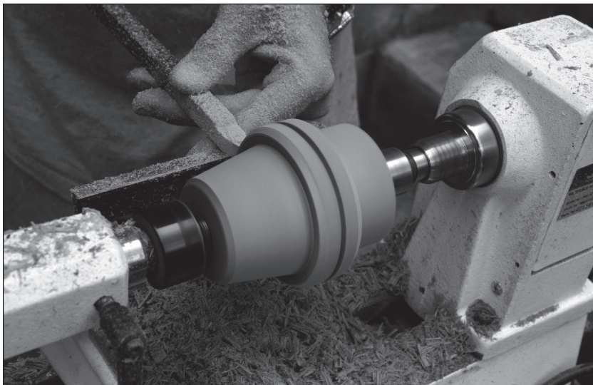
Fig. 4.30 Simple feet. This foot is easy to turn on a lathe with just a couple tools. The hardest part is finding a piece of teak that is 3\frac{1}{8} " thick to begin with.
