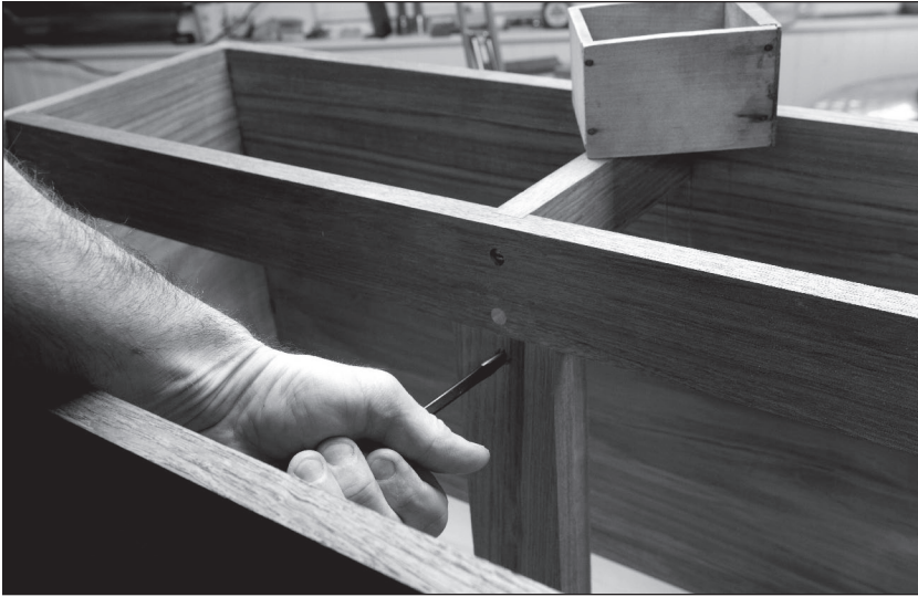
Fig. 4.20 Screws from below. The No. 8 x 1-1/4" brass screws help support the vertical divider and web frame. They also hold the drawer guide in place.
