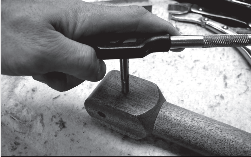
Fig. 7.30 Tapping. It's best to tap the hole for the 13mm ball studs. If you don't have a tap you can make do with an undersized hole – and perhaps a dab of epoxy.
