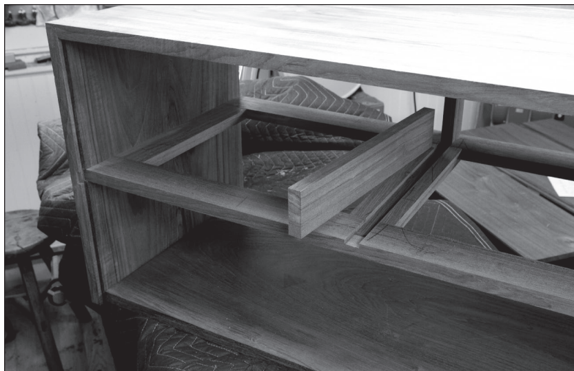
Fig. 4.18 Dado for the runner. Here you can see how the dado in the web frame holds the drawer runner and the vertical divider.
