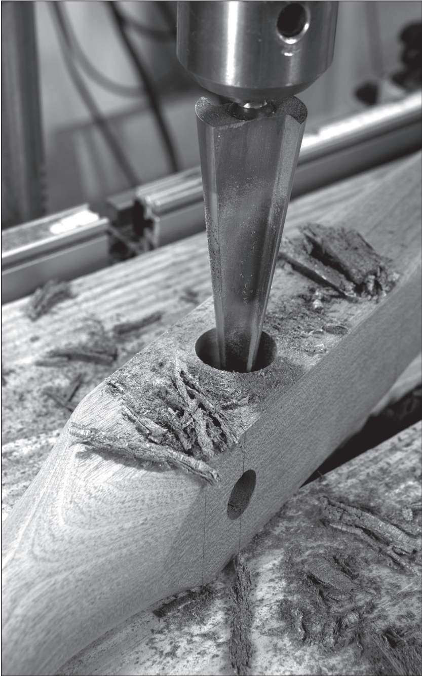
Fig. 7.14 With a drill press. Some reamers can be used in a drill press at a slow speed. This is a quick and easy way to guarantee your hole is straight and true.
