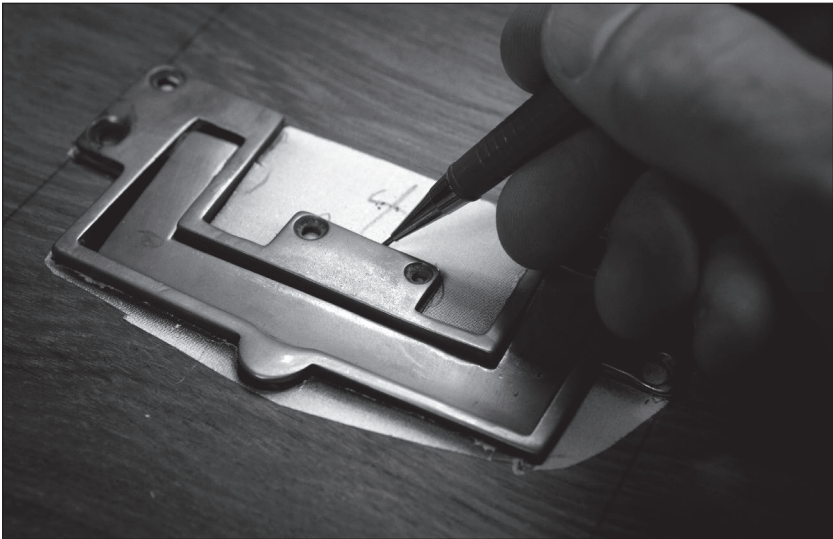
Fig. 4.41 Trace & chisel. Trace around the pull intended for that spot. Then remove the pull and excavate the area so the outer plate can be seated flush with the drawer front. The pulls might be warped a tad. Be prepared to slice and screw.
