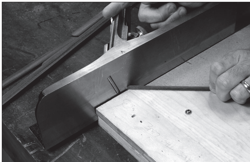
Fig. 8.12 Shoot the miters. If you set the plane to take a light cut, you won't have any trouble with the outside edge of the seal's miter splintering.
