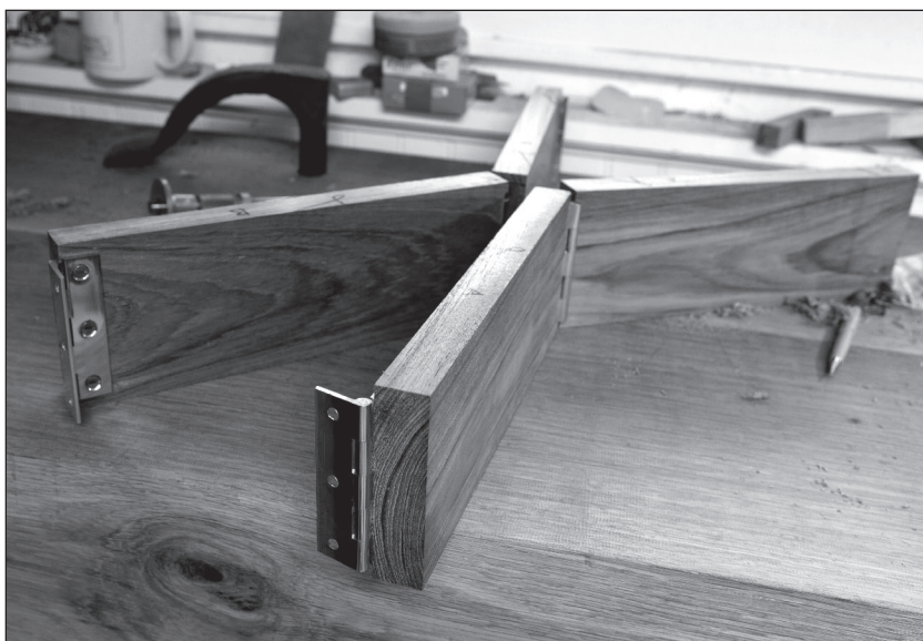
Fig. 9.12 Three-way fold. With three hinges installed on each end apron, you are ready to attach these flexible aprons to the fixed front and rear aprons.
