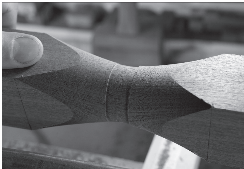
Fig. 7.6 Or a curve. Some Roorkee chairs had a curved grip instead of a straight-walled cylinder.
