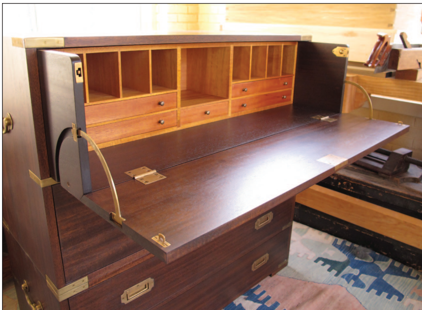
Fig. 5.5 Open gallery. The gallery is merely a drawer with a front that folds down to reveal cubbyholes and drawers inside.
