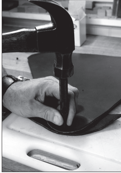
Fig. 6.10 First punch. Using a leather punch, make a hole through the seat and pocket piece. I'm using a kitchen cutting board as a backer.
