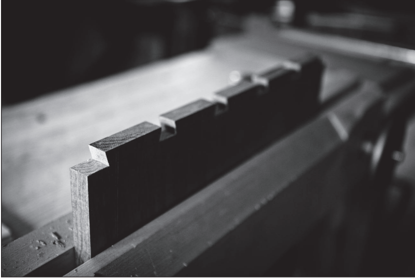
Fig. 4.8 Six tails. When cutting dovetails that are for structural purposes and won't be seen much, use tails and pins that are fairly large. For a campaign chest, lay out five tails or so on the tops and bottoms that join the sides. These tails are 1/2" long.
