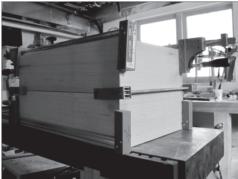
Fig. 11.9 Glue the two. You want these carcasses to mate. So glue them up in tandem. Clamp the tops, bottoms and sides. But also clamp the carcasses together so their edges align.
