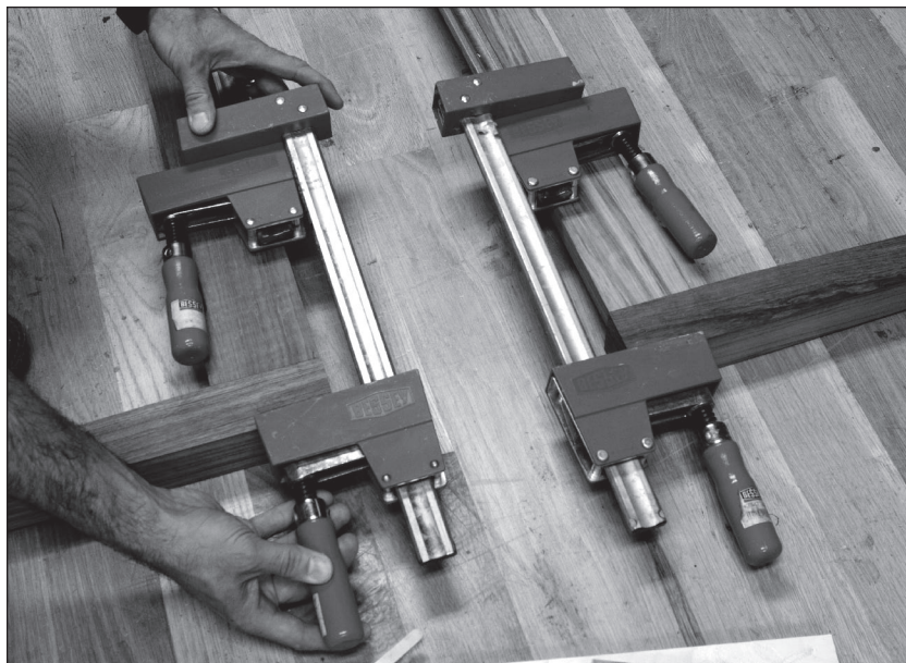
Fig. 9.9 Epoxy time. I used epoxy for this joint because I have found it to be unsailable. It fills gaps. It bonds almost anything. Yeah, it stinks and you have to mix it up, but it is hard to argue with its results.
