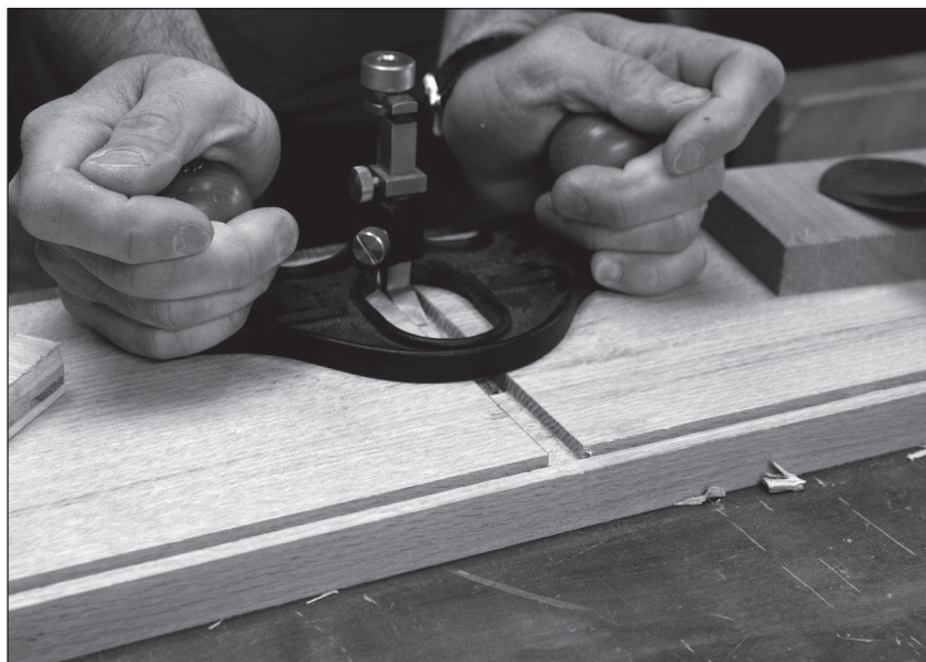
Fig. 11.6 Plunge forward. The router plane isn't suited to take a big bite. The waste jams up against the post of the iron too easily. Use the router to remove the smallest amount of waste from the bottom of the dado.
