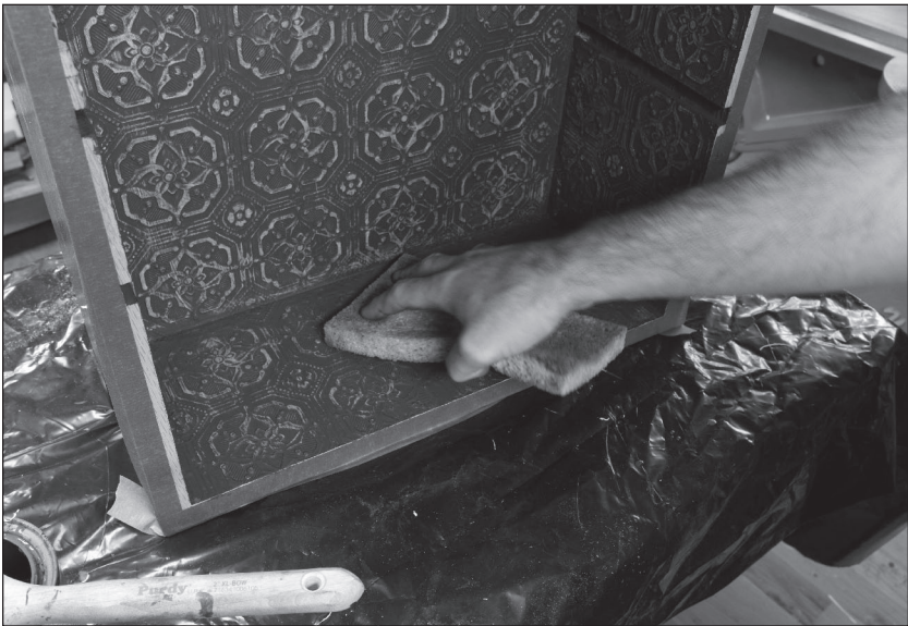
Fig. 11.22 A little dab. After the paint flashes, gently wipe the high spots with a sponge to brush away part of the paint.
