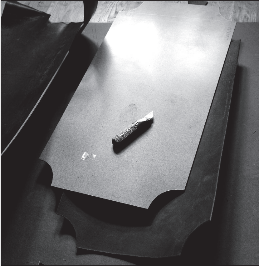
Fig. 7.24 Do it on the floor. Hardboard templates are an inexpensive way to more easily make several chairs. When I cut out a set of leather pieces, I kneel on the template parts to hold them in place.
