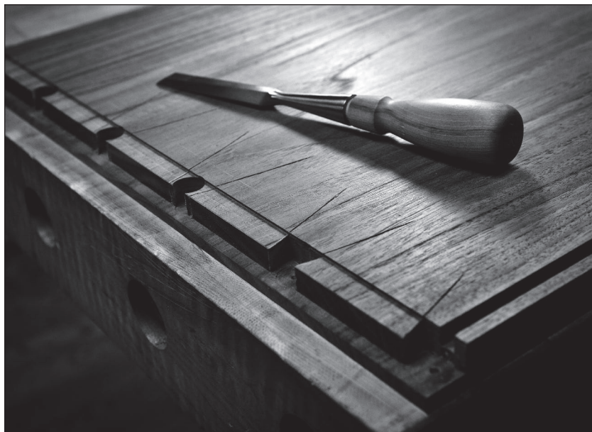
Fig. 4.11 Double rabbets. Here you can see the shallow rabbet cut on the tails of the joint and the deeper rabbet cut on the ends of the top. I am in the middle of chopping out the waste between the tails.
