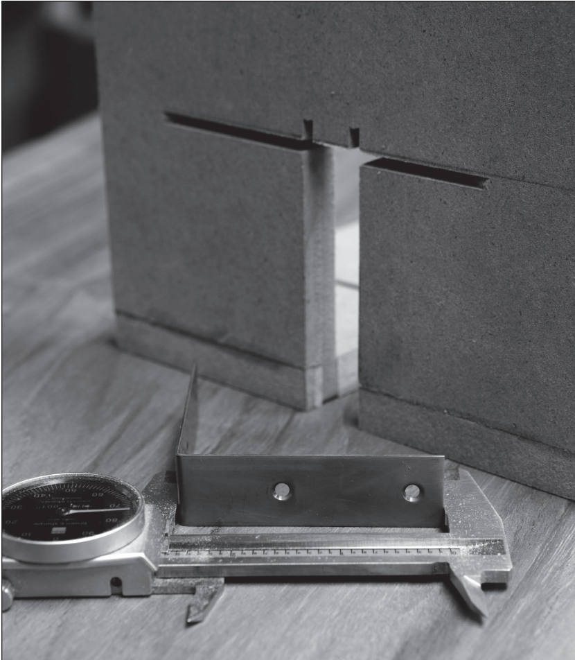
Fig. 4.33 The real length. Don't measure the bracket from its inside. Measure it only from the outside, as shown here. This measurement represents the size of the notch in the template.
