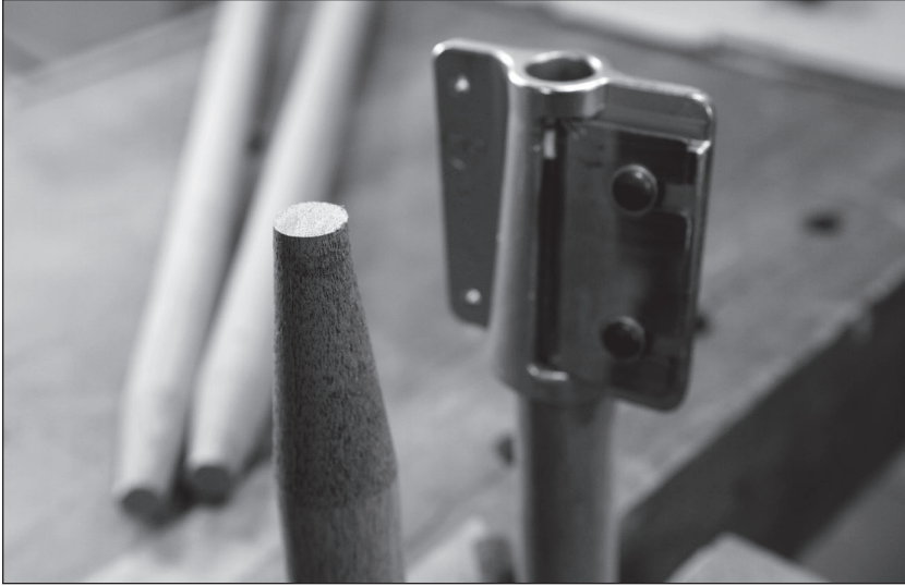
Fig. 7.16 Quick work. Using a tapered tenon cutter is like using a giant pencil sharpener. Focus on keeping the tool centered on the work. If you don't own a tapered tenon cutter, turn the taper on the lathe and adjust it with a spokeshave.
