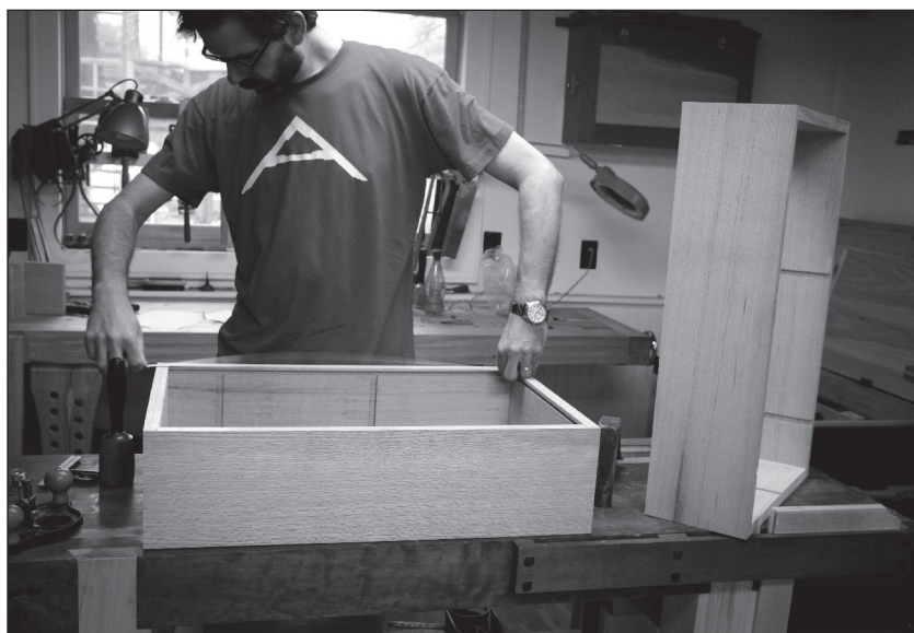
Fig. 11.7 About that much. I don't cut my panels to size until I have the carcasses dry-fit. This (usually) prevents me from making a stupid error.
