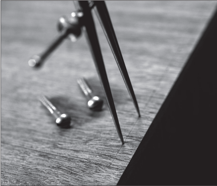
Fig. 8.14 Walk it off. On the chests I examined, the spacing between each screw was greater than the diameter of one screw. So don't space them too tightly.
