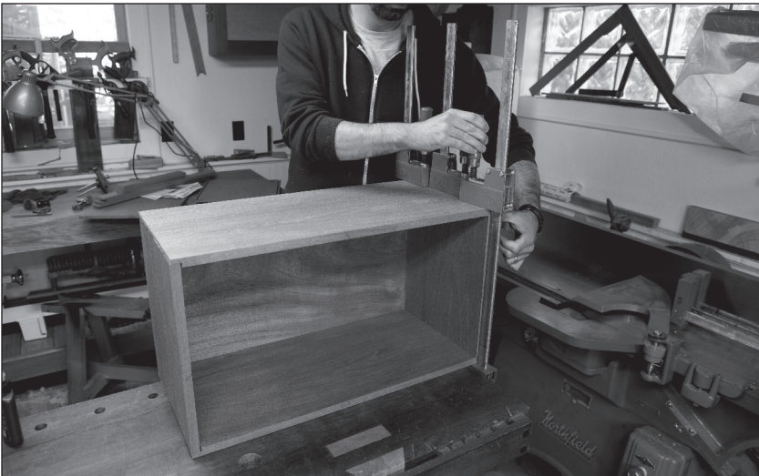
Fig. 8.8 Clamp off the edge. Push the end of the carcass off your workbench to clamp across the joint. Try to keep the jaws of the clamps positioned over the joint line only.
