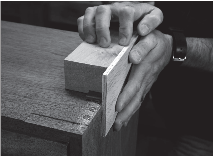
Fig. 8.18 Push or pull. By orienting the file one way or the other, you can use the jig in a pushing or pulling position. Both work.
