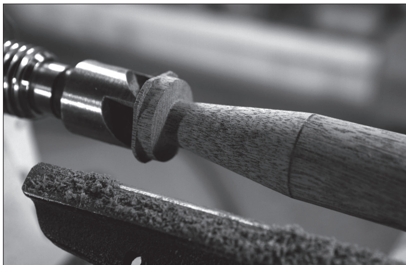
Fig. 7.15 Pre-tapered. If you rough in the taper on the lathe, it will greatly reduce the work needed to shape the final taper.
