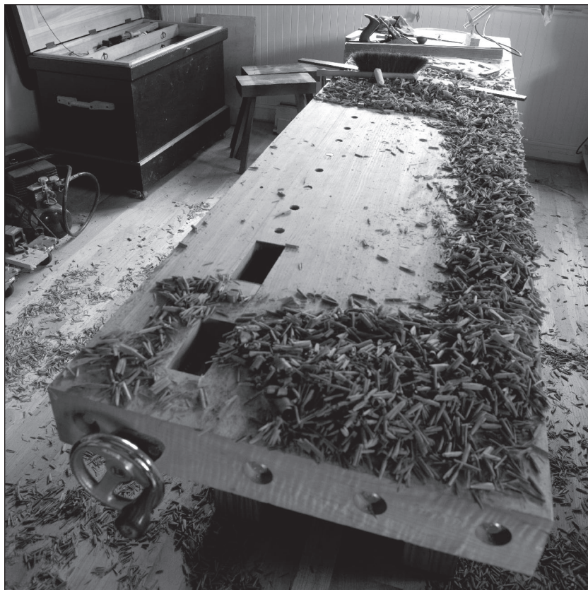
Fig. 4.7 Traversing teak. If you use a jack plane or fore plane with a heavily cambered iron, you can flatten panels with ease. The trick: Work across the grain.
