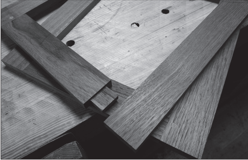
Fig. 4.15 Loose in the rear. Don't glue the rear stile to its tenons. You want that stile to be able to move slightly as the case moves.
