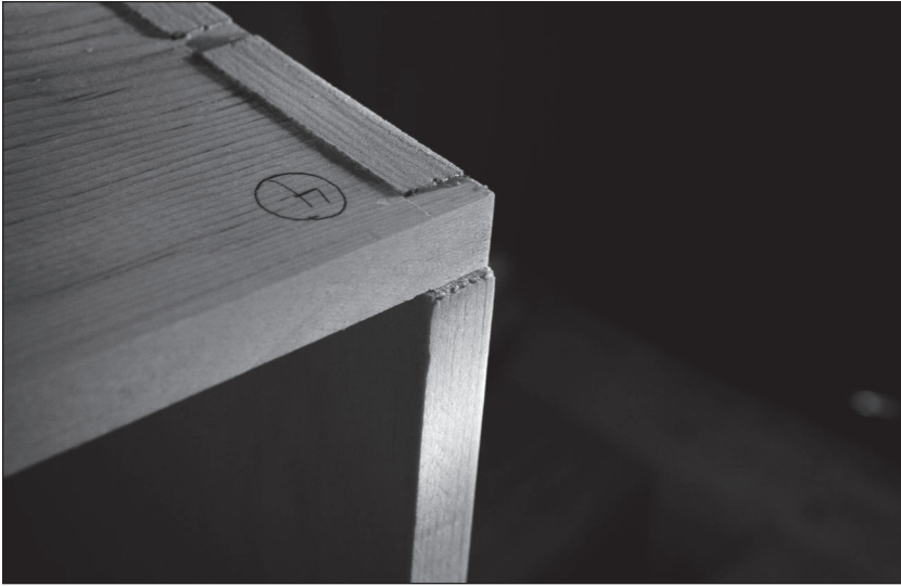
Fig. 4.27 Also narrow at the top. I also rip the drawer back down a bit on its top edge. This prevents the drawer from dragging against the carcass, and it lets air move around.
