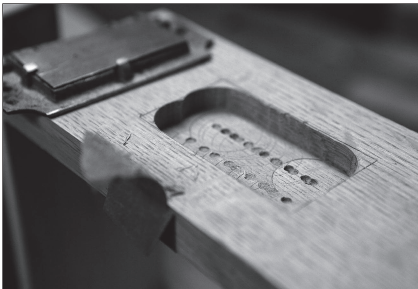
Fig. 11.18 Drilled out. I usually remove most of the waste with a drill – in this case a Forstner bit. All this ugliness will be hidden behind the pull's backplate.
