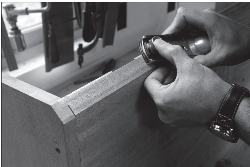
Fig. 5.8 Matching bevels. The front edge of the drawer bottom should have a 45° bevel, as should the front corner of each drawer side. After assembling the secretary drawer, you might need to plane these three bevels to match.
