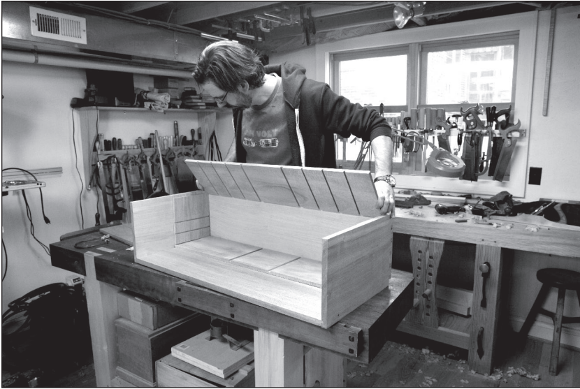
Fig. 5.12 Fit before nailing. The sides, top and bottom of the gallery all fit into the top drawer. Confirm their fit before putting the gallery together with glue and nails.
