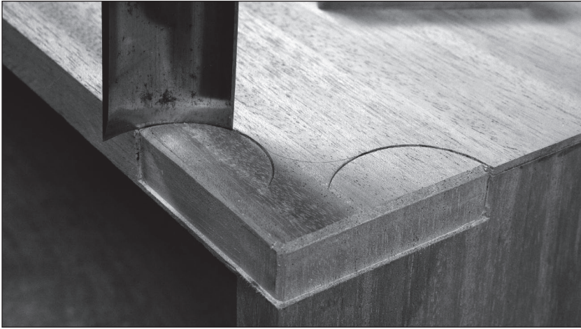
Fig. 3.25 A firm choice. If you have firmer gouges, you'll find this part of the job a lot easier.
