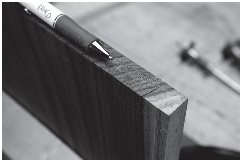
Fig. 4.9 How to see better. Knife lines in dark and porous woods can be murder to see. One solution is to use a fabric-marking pencil, such as the one shown here. The pencil's "lead" is actually a soft ceramic material that comes in bright colors: pink, green and white are typical. All help you to better see your knife lines.
