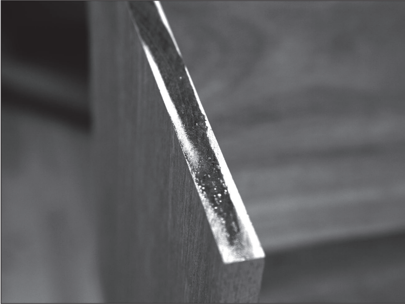
Fig. 8.7 I feel dry. You can see how the end grain of the end pieces has soaked up this hide glue after less than 60 seconds. A second coat of glue will make the joint stronger.
