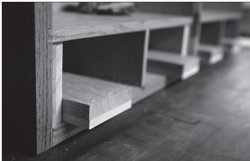
Fig. 11.17 Parts in place. Fit your drawer parts so they match the dimensions of the drawer opening. If the individual parts fit too tight, the drawer will surely stick.
