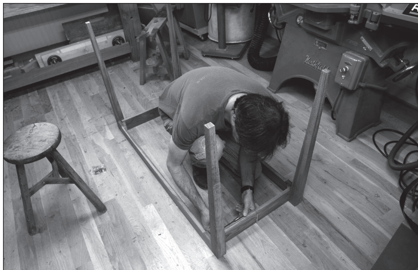
Fig. 9.14 On the floor. Install the second fixed apron with the parts on the floor, upside-down.
