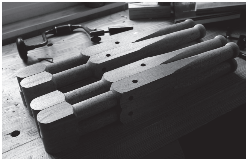
Fig. 7.12 Clustered & complete. I've bored the through-holes and can now ream them out. When making these chairs, I keep the legs organized like this throughout construction.
