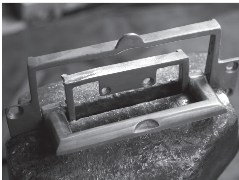
Fig. 3.37 Final fitting. Don't be afraid to file away bits of brass here and there so that the pull swings sweetly.
