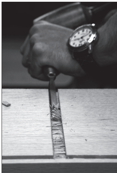
Fig. 11.5 Plow the waste. Remove most of the waste with a chisel. Work bevel-up to remove material quickly; work bevel-down to add some control.
