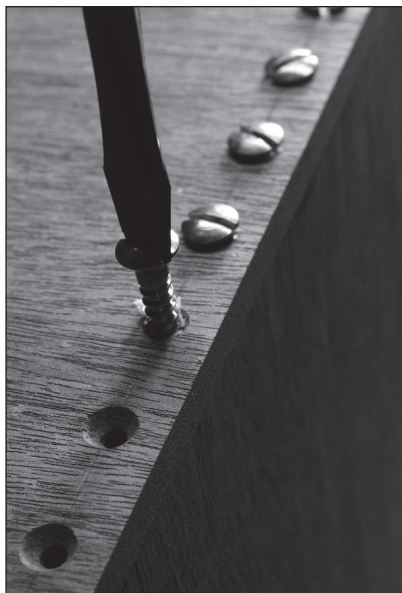
Fig. 8.16 And screw. Drive the No. 10 screws in so the bottom of the slot is coplanar to the carcass. That will result in the least amount of brass to remove.
