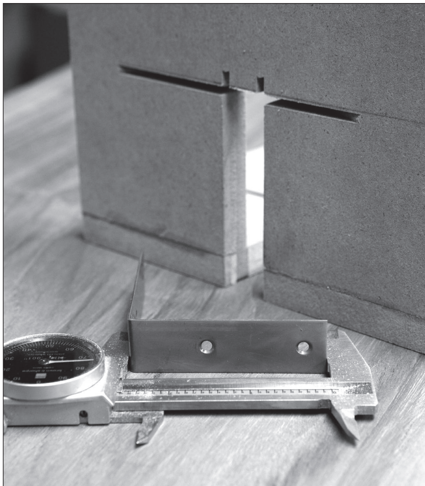
Fig. 3.17 First gauge. The outside length of one leg of the bracket is the place to start when making a router jig.
