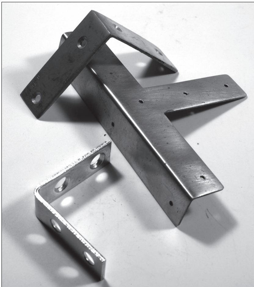
Fig. 3.8 Or bend it. Bending your corner guards can be easier than casting them. So it's a common practice with this piece of hardware. The big difference is that the corner is radiused instead of sharp.
