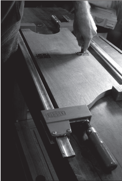
Fig. 10.10 Punch it. Clamp the top and bottom together to ensure the parts are aligned and stay that way as you install the hinges. I use a center punch to mark where the screw holes should go.
