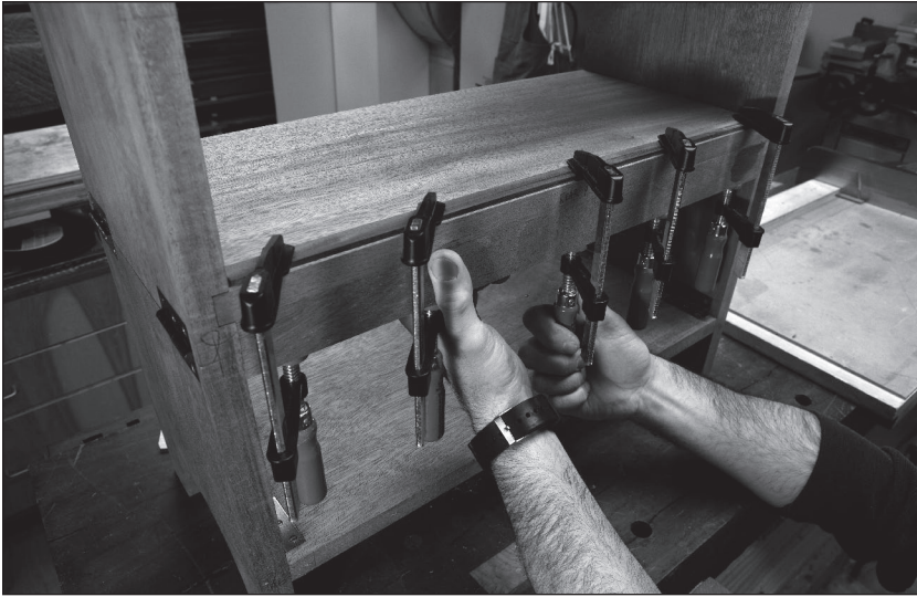
Fig. 10.16 Glued in place. Adding the dropped edge while the case is assembled removes the risk of it sliding around as you apply clamp pressure.
