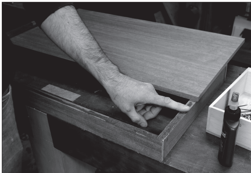
Fig. 8.10 Tricky. Glue only the front part of the lid to the top, but nail it all around. That's the best strategy in this situation.
