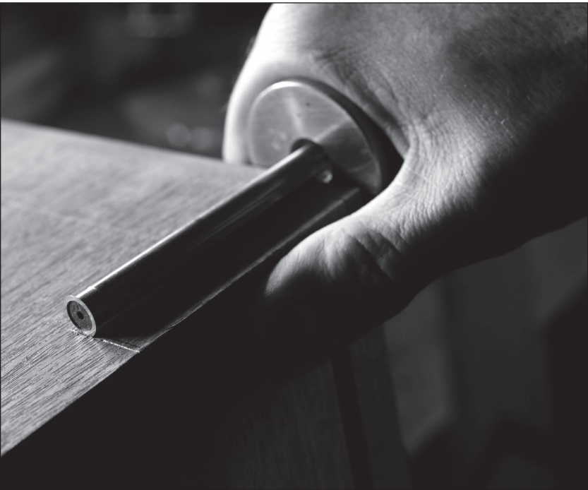
Fig. 3.13 Length of the leg. Set the cutting gauge to the outside length of one leg of the bracket. Gauge this on your work.
