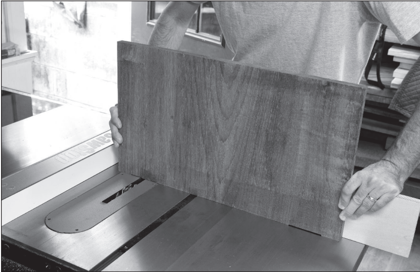
Fig. 9.16 Notches for hinges. Here a leaf is up on end on the top of the table saw. I have a 5/8" dado blade installed in the saw and its height matches the thickness of the hinge leaf. Mark where your hinge starts and stops. Nibble out the wood between the two lines.
