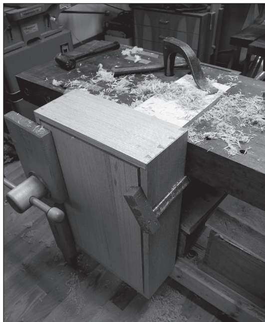
Fig. 11.9 Glue the two. You want these carcasses to mate. So glue them up in tandem. Clamp the tops, bottoms and sides. But also clamp the carcasses together so their edges align.
