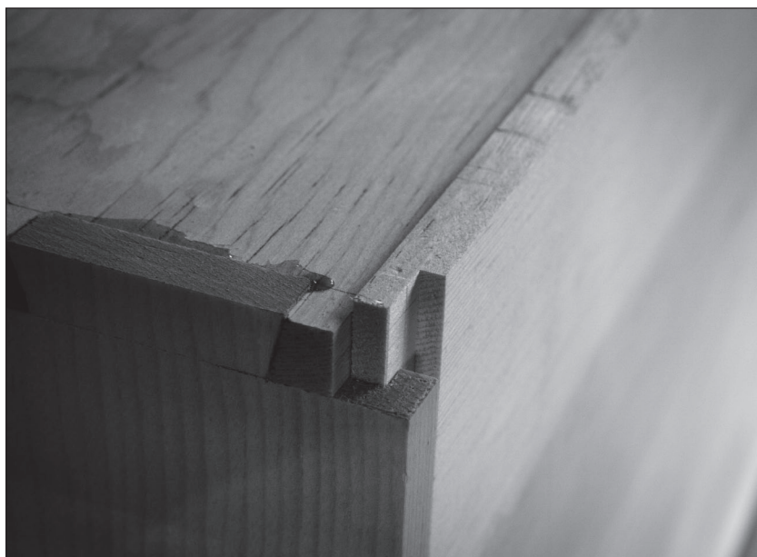
Fig. 4.26 Drawer bottom in place. Here you can see how I've ripped the back narrower so the bottom can slide in.
