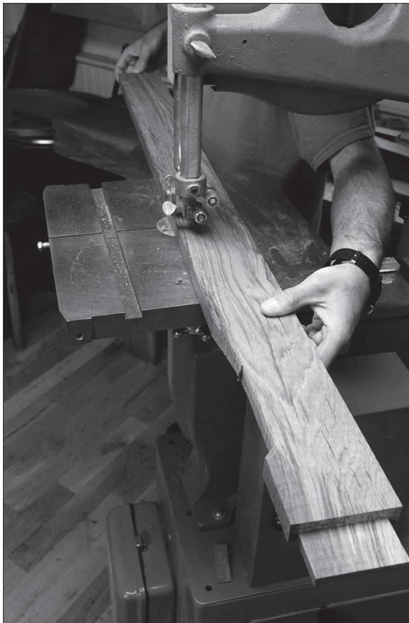
Fig. 9.7 Quick relief. The 1/2"-wide relief on each apron is easy to cut on the band saw. Be sure to make a couple relief cuts so you don't cut yourself into a corner.
