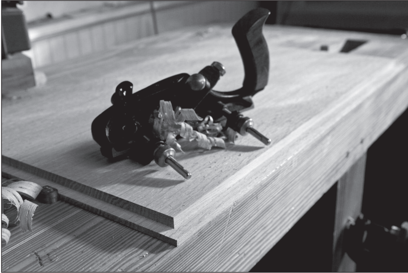
Fig. 11.8 Rabbet that. Cut the rabbets on the back panels. Cut the rabbets across the grain first. Then follow that with the rabbets that run parallel to the grain.
