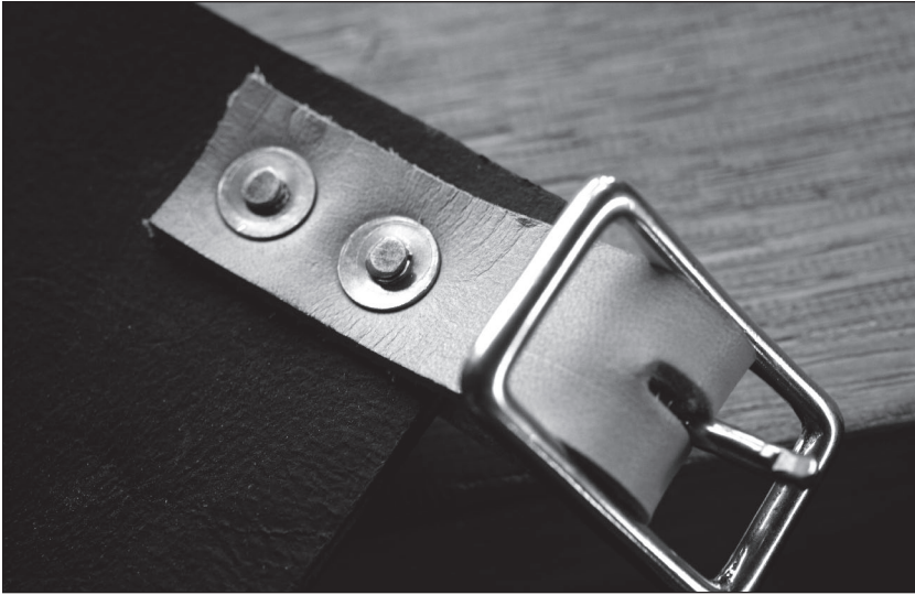
Fig. 7.22 A bit slower. Riveting with copper rivets takes a couple extra steps. Punch the hole. Push the post through the holes. Set the washer. Snip the post and peen the post. Installed correctly, rivets are remarkably strong.
