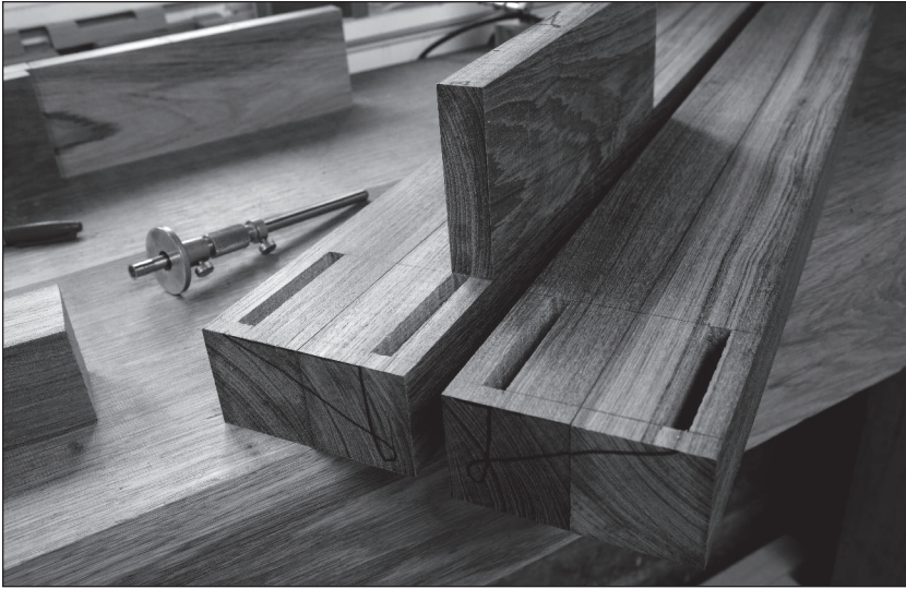
Fig. 9.4 The right mortise. Here are the four mortises in the legs. As you can see from the apron sitting on top of the leg, the tenon will need only three shoulders instead of four. Shifting the tenon to the back of the apron gives you a thicker mortise wall.
