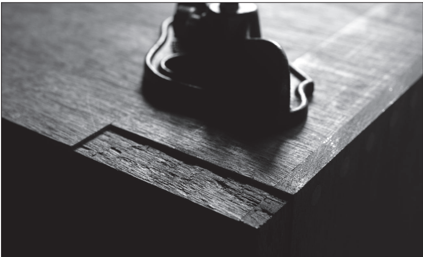
Fig. 8.25 Rout it. A small router plane can remove the waste in one pass if your chisel chops have been strategic. Plan your cuts so the waste supports the tool's sole for as long as possible.
