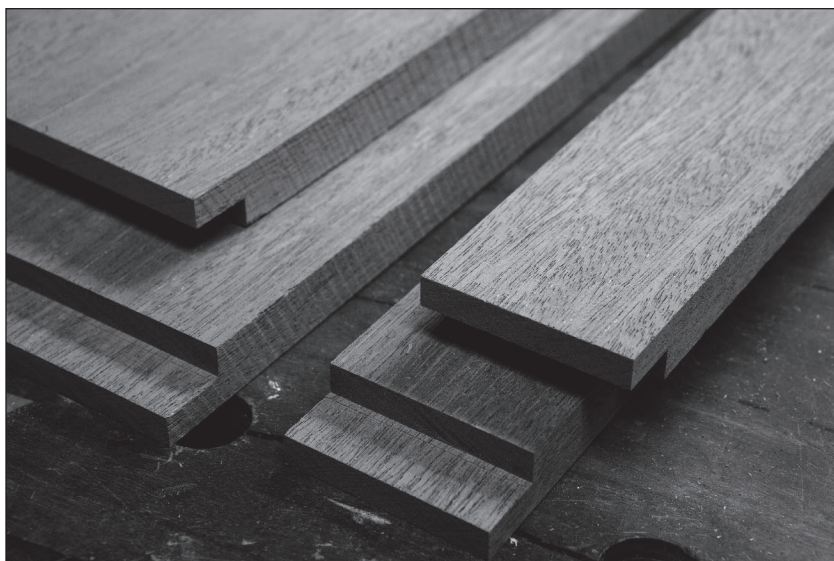
Fig. 8.5 Free lid. I cut the rabbets first then ripped the lid pieces free from the carcase pieces. Cutting rabbets on narrow parts can be difficult.
