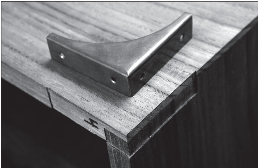
Fig. 4.36 First recess. Using the template for the corner brackets, I roughed in a too-small recess for the corner guards. This allowed me to press the guard into the corner and sketch its final shape on the work.
