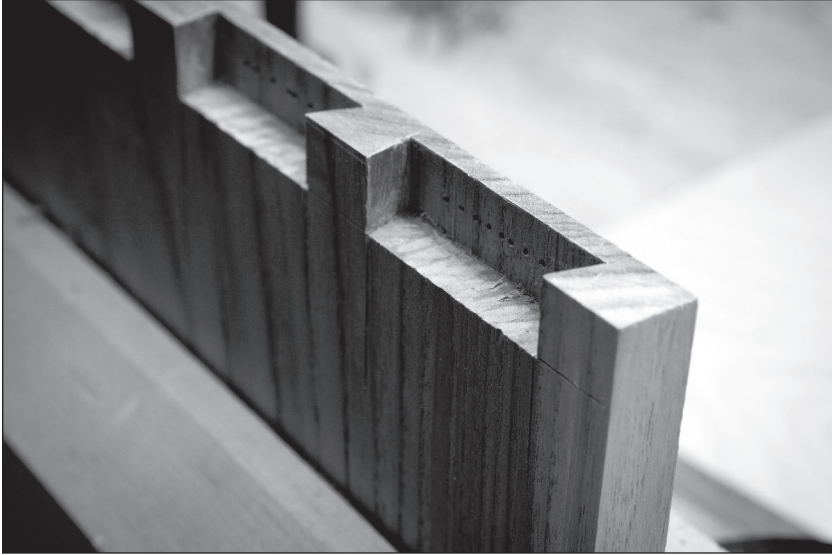
Fig. 4.10 Tidy sockets. Here you can see the points left by a Forstner bit, which I used to bore out most of the waste on the pin board. Don't get too sloppy here. Even though the joint won't show, it does hold the case together.
