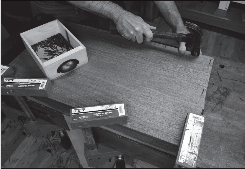
Fig. 8.11 Nail & set. I clamped the front edge of the top and lid together while I nailed the top down all around. The clamps keep everything in place while you do your nailing.
