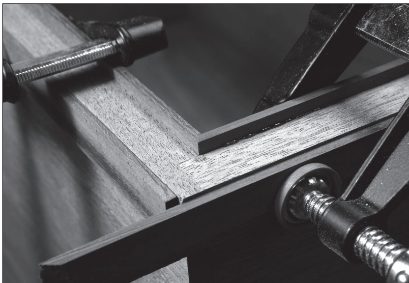
Fig. 8.13 Glue & clamps. Here you can see the seal poking up above the rim of the carcase. That's all it takes to keep out the bugs.
