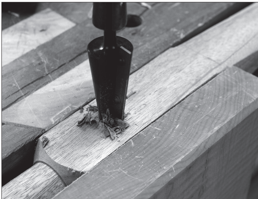
Fig. 7.13 Reaming with a brace. Mark your stopping point on the tooling. You want to stop reaming as soon as the tip of the reamer is cutting a 5/8"-diameter hole.
