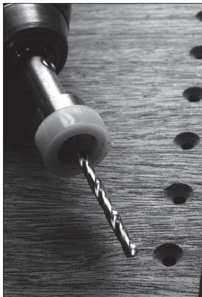
Fig. 8.15 Tiny countersinks. Set the stop on your bit so it makes just a shade of a countersink – less than 1/16" deep. This will allow the screw to compress the wood a bit and leave a seamless joint.
