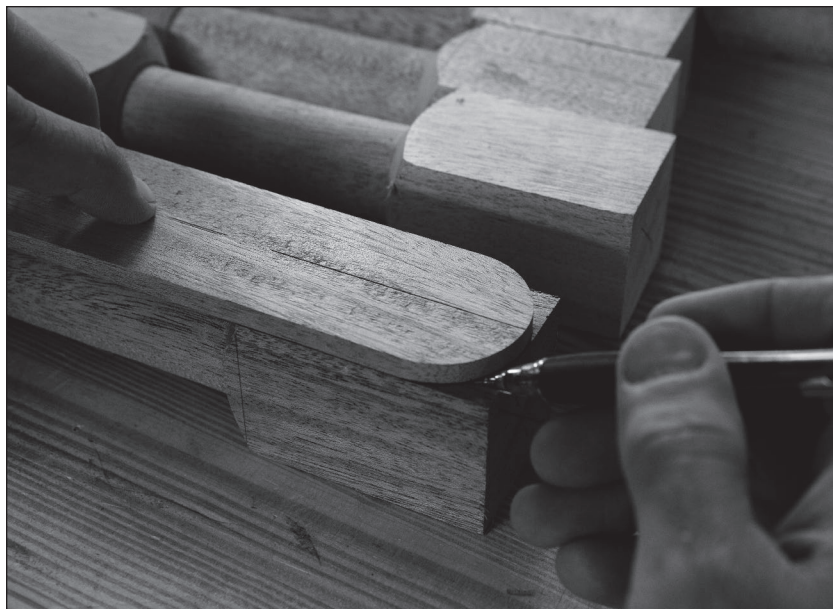
Fig. 7.10 Around the bend. A thin wooden pattern ensures that all four legs will receive the same shape at top.
