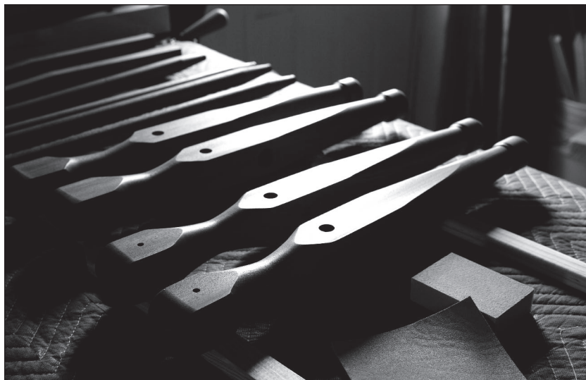
Fig. 7.19 Before the wax. After two coats of garnet shellac, the mahogany has warmed up considerably. The wax will complete the classic mahogany look.
