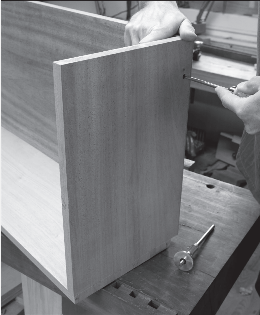
Fig. 5.7 Screw that bottom. This brass screw holds the bottom in place so the bottom will slide in and out with the rest of the secretary drawer.
