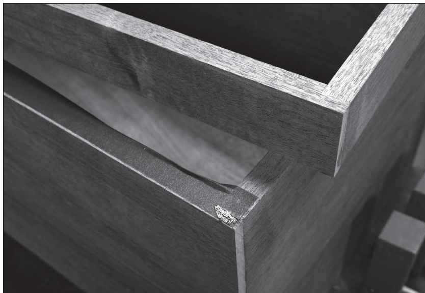
Fig. 8.9 Two clamps & done. The lid parts sit on top of some masking tape. Clamps (not shown) hold the lid pieces together and to the carcase below.
