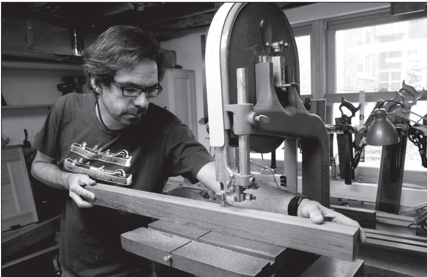
Fig. 9.5 Safer taper. Most table saw tapering jigs put your hands in harm's way. Tapering legs on the jointer can push small machines to their limits. So I like to cut the taper with a band saw and clean the cut with a handplane.
