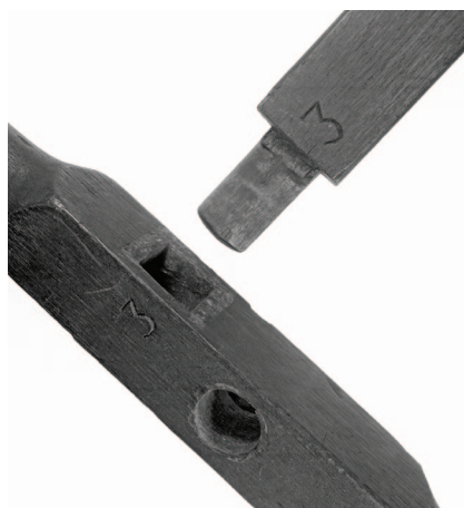
Figs. 1.57 & 1.58 Squared. This Roorkee has cylindrical tenons that have a square shoulder. This prevents the stretcher from rotating in service. (Courtesy of the Council of the National Army Museum, London)
