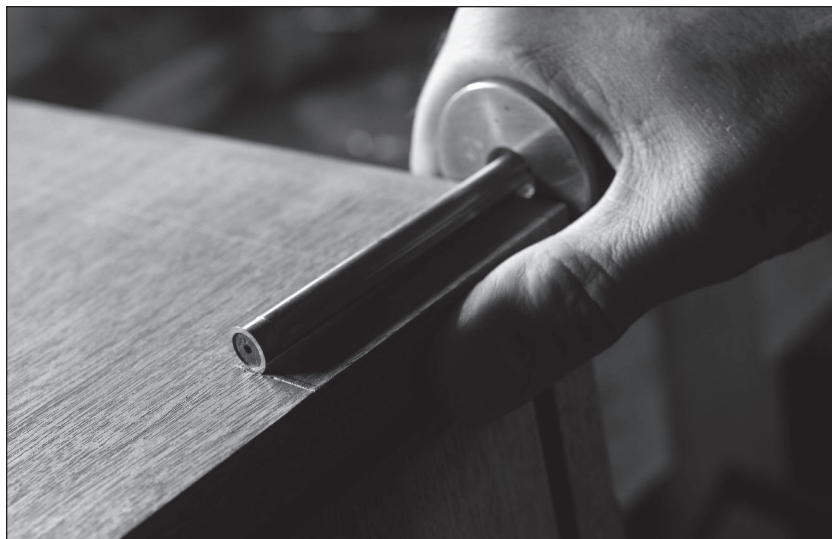
Fig. 8.23 Gauge the length. With a second gauge, cut in the exact length of the corner hardware.
