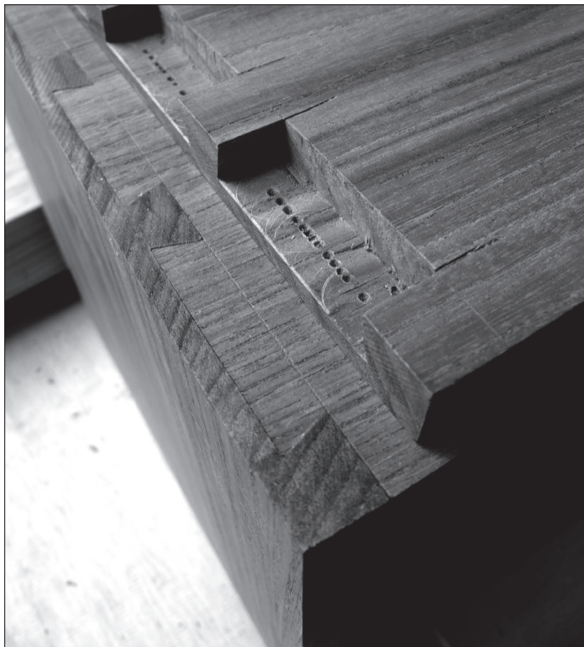
Fig. 1.23 Half-blinds. The top board of the lower case that is joined to one of the ends. When the two components of the chest are stacked on top of one another, the tails are concealed.
