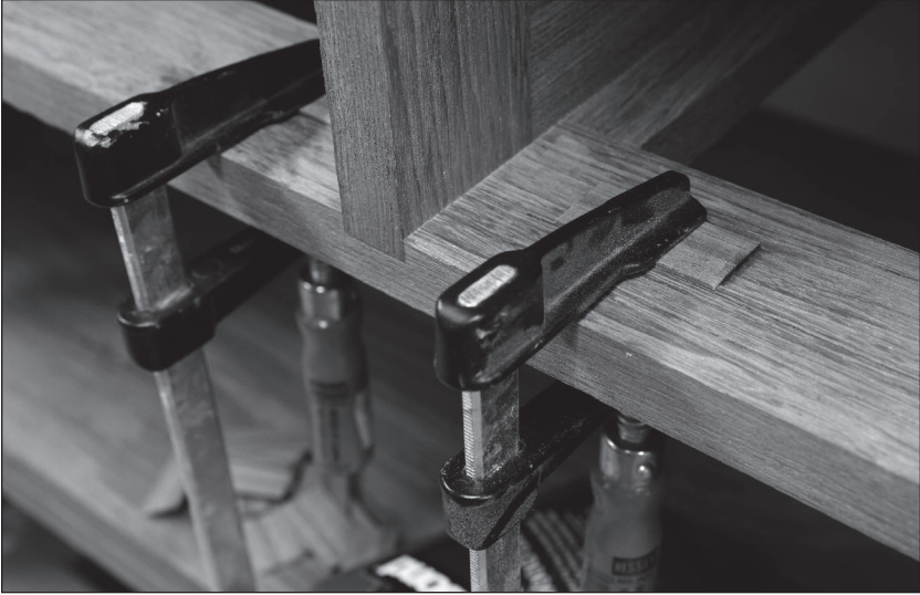
Fig. 4.43 Stop here. These small drawer stops are affixed with hide glue. They keep the drawer front positioned in the correct place year-round.
