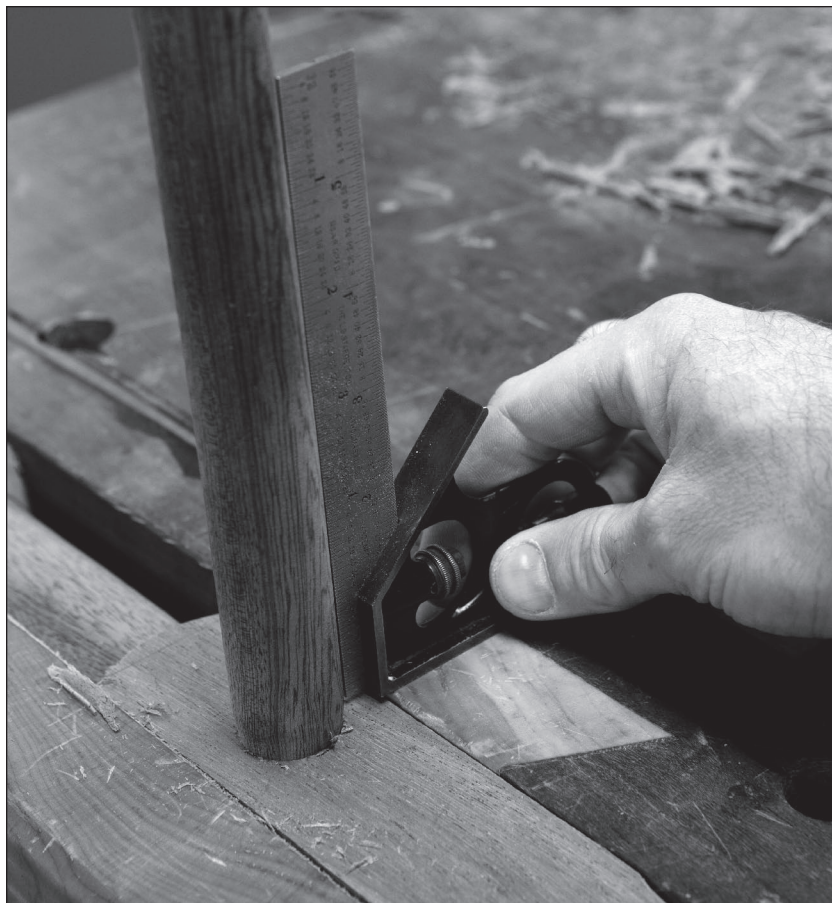
Fig. 7.17 Check & check. If you clamp the leg so its exterior surface is flush to the benchtop, it is easy to check the Z-axis of this joint from multiple directions. Get it as close to plumb as possible without shaving the stretcher to a nub or reaming the mortise into a sinkhole.
