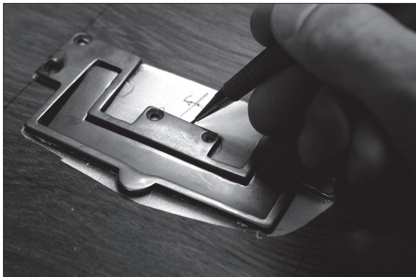
Fig. 3.36 And trace. Once the pull can drop into the recess, you can trace around the thin parts. And you should trace around the hardware. Even though you scanned that piece of hardware, your deep recess might be tilted or shifted.
