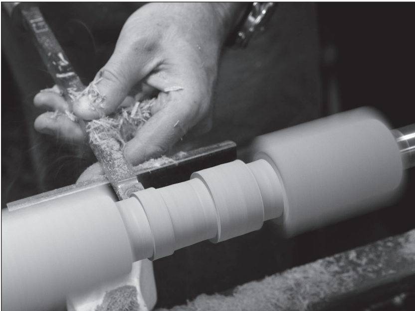
Fig. 7.4 Begin with the cylinder. If you are going to have a round cylinder at the top of the leg, turn it down with a roughing gouge or a roughing tool, such as this carbide-tipped turning tool.
