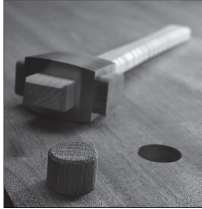
Fig. 4.24 The dowel. This protruding dowel will slide into a matching hole in the other case, preventing the top case from sliding laterally.
