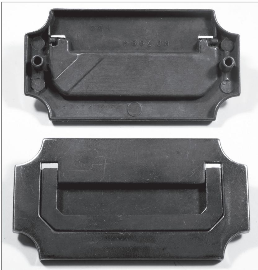
Fig. 3.6 Die-cast. These die-cast pulls are perfectly consistent and inexpensive, but lightweight. One of the advantages of die-casting is that it is easy to cast in threads and other details that might otherwise have to be machined in a sand casting or investment casting.
