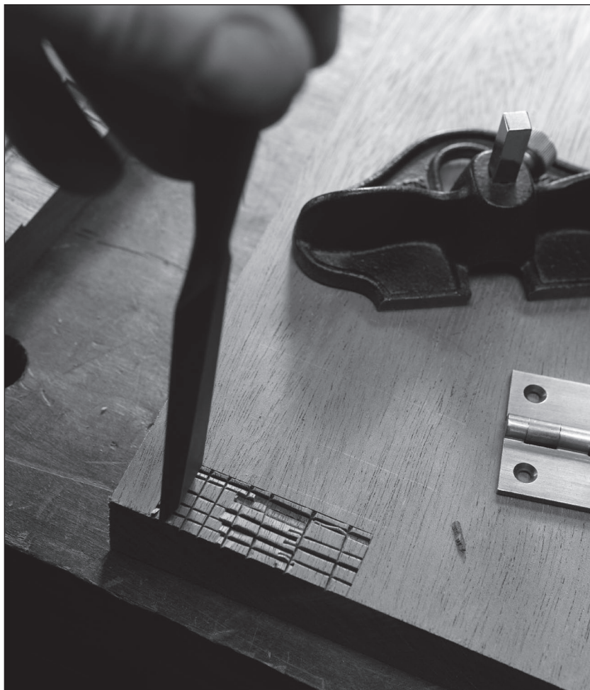
Fig. 10.9 Chop & rout. To cut a hinge mortise, first chop across the grain deeply. Then chop parallel to the grain more shallowly to avoid splitting the work. Pop out the waste with a router plane.
