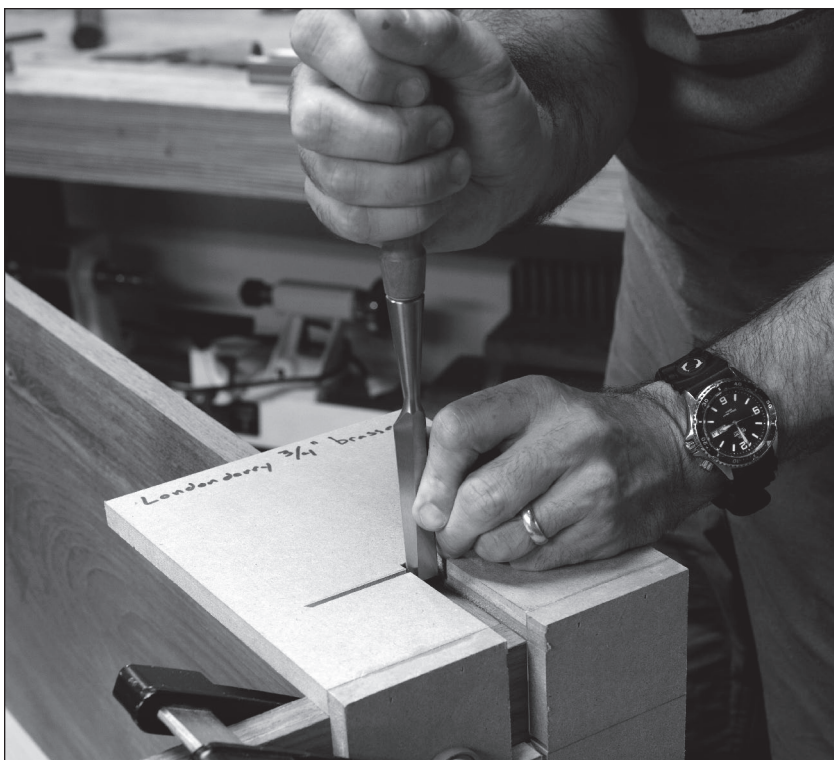
Fig. 3.20 Down, then in. Chop the corners using the template as a guide. Then remove that waste with the chisel flat-on. Keep the template in place during this operation. The downward pressure from the template helps prevent you from plunging too far.
