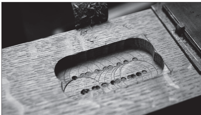
Fig. 3.27 Trace & drill. Remove as much waste as you can with a Forstner bit, if that's the route you choose to go.
