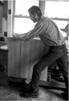
Saw & square. Squaring up a tabletop with hand tools is far easier than trying to set up a small machine to do the job. Try handsawing and planing the ends square. You'll be surprised by how easy it is.
