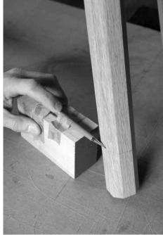
Mark around. This block-and-pencil method simultaneously levels the saw-bench and marks the final length of each leg.
