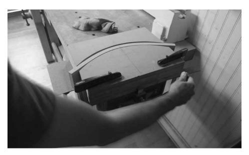
Screwed  $\ensuremath{\mathfrak{C}}$  bent. You can easily bend the crest in a form (the same form for the backstool) by pressing the two halves of the form together on a workbench's vise.
