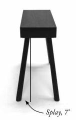
Side, rake; front, splay. Chair geometry is like saw geometry. From the side of a saw or chair (left), the teeth or legs are raked, either forward or back. Looking at the front of the saw or the chair (right), the teeth or legs are splayed out; we call this "set" in a saw and "splay" in a chair.
