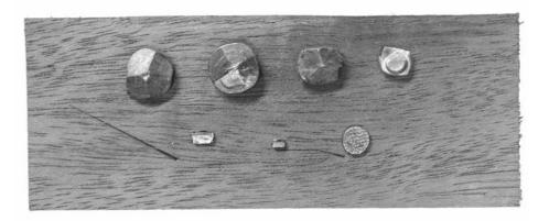
What you see is what you get. Different nail heads from left to right, top row: black-smith-made wrought-head nail; machine-forged nail; decorative "wrought head" cut nail; rosehead cut nail. Second row: fine finish brad; cut headless brad; wire sinker.
