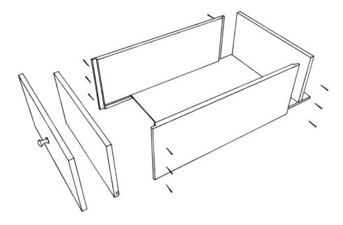
Realistic drawer. Skip the dovetails and assemble the drawer using rabbets and headed nails. The drawer bottom slides into grooves in the side and front pieces.
