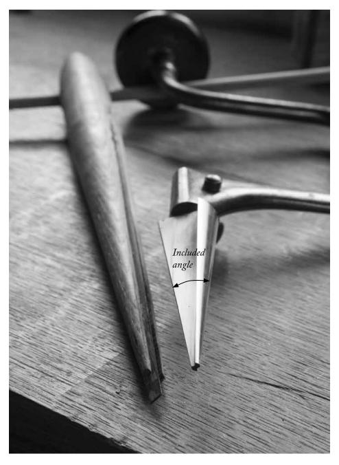
Both work. A metallic reamer and a wooden reamer (with a cutter made from saw steel) both do the job. Debate the fine points if you will. Or build stuff.
