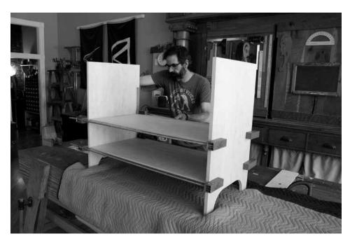
Correcting pressure. Here I am shifting a clamp to pull the rear of the case square. By applying the pressure above one dado and below the other, the case changes its shape. This is handy when clamping across the case diagonally isn't an option.
