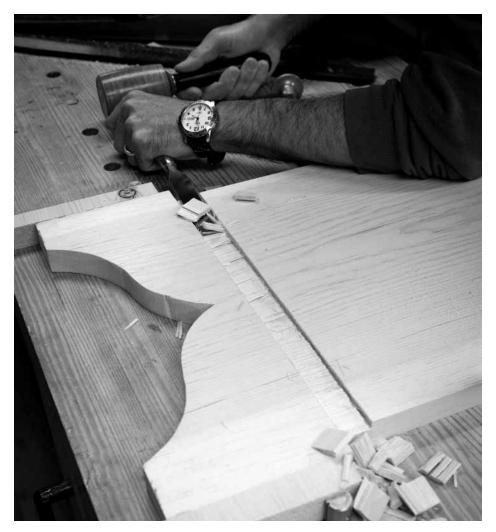
Work across. Chiseling out the waste in a dado is easy work. Begin with the chisel bevel-up as shown. Then switch to bevel-down when the handle gets in the way.
