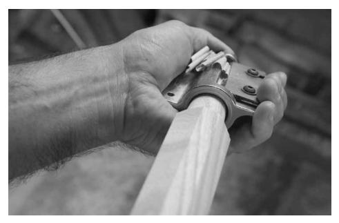
Maker's-eye view. This is what I see when I turn the tenons on my legs. My eyeball is glued to the gap between the leg and the tenon cutter.
