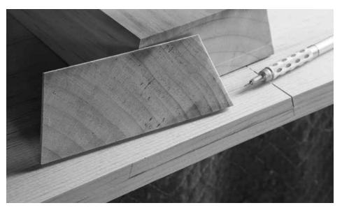
Measuring is the enemy. Rather than measure the width of the batten and its slope, use an offcut of the batten itself as a pattern for the dovetail socket.
