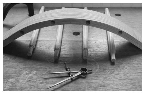
Ready to assemble. The holes are drilled. The spindles are shaped. Nothing is left to do but glue the thing together.
