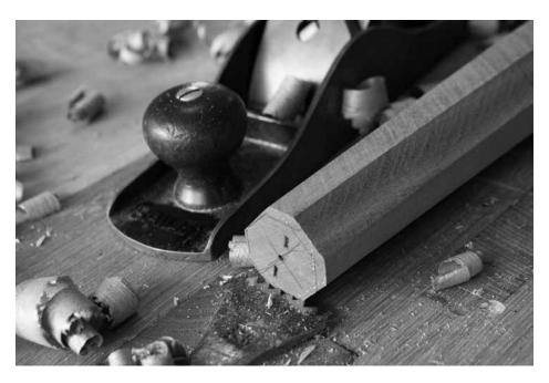
To the line. Tapering legs with a sharp jack plane is simple. Work to the lines marked on the feet and try to keep the facets consistent around the leg.
