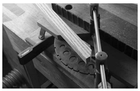
Quick cut. Many early chest lids had rounded corners on the battens. Or the battens would taper toward the front, ending in a rounded corner.
