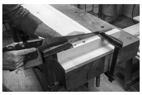
One side. You can see how I use a fence and saw to cut a perfect wall for the dado. After sawing this first wall, don't remove the fence.
