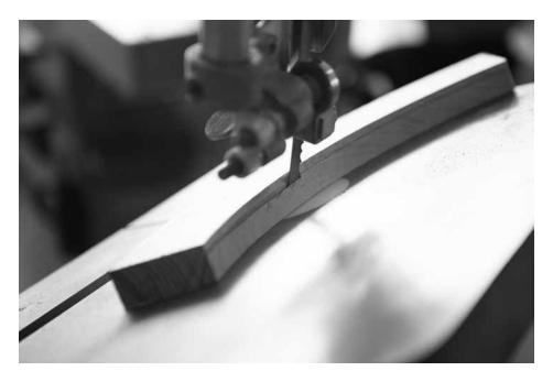
Bevel the doubler. The 30° bevel on the front of the doubler avoids some lower back pain for the sitter. Set the table of your band saw to 30° and make the cut. (Note: The pencil line on the stock shows what a 45° cut would look like.)
