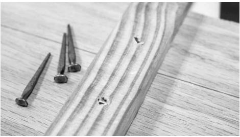
Not much to see. When done correctly, the tip of a clench nail hits the metal surface and turns back into the work. What you see on the exit side is a rectangle of metal.
