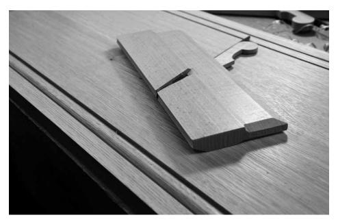
Simple moulding. After plowing two grooves in the stiles, shape the interior bit into a curve with a rabbet plane. Then finish up with a small hollow plane.
