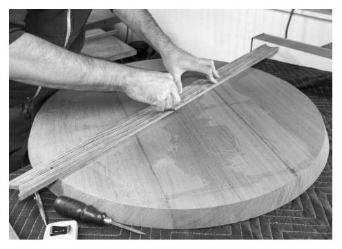
Create sightlines. Use a straightedge to join the center of the circle to the three mortise locations. These are your sightlines for boring the mortises.
