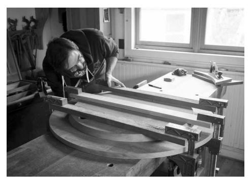
Three cauls. Rough scraps that are cantilevered off the subtop are all you need to get the pressure where you want it. Clamp the ends of the cauls and you'll press the two pieces together just fine.
