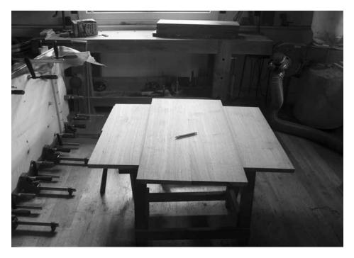
One-board top. Though there are four boards in this glue-up, they all were cut from the same long plank to ensure the top will be consistent in color and grain.
