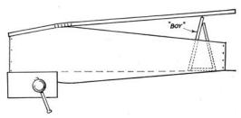
Fig. 6. Side being nailed down supported by "boy".
