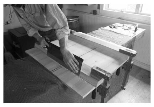
One wall. The best saw in my shop for this operation was a large tenon saw that was filed rip. It chewed up the underside of the tabletop a bit, but I got over it.
