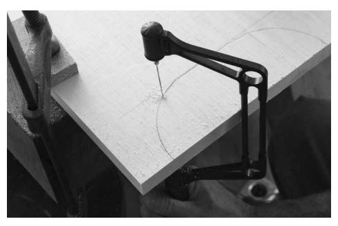
Better for me. I like to hold a coping saw vertically when making scrolling cuts such as these. My saw cuts end up more square through the thickness of the work.
