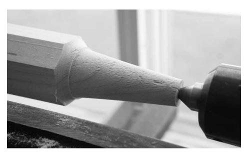
Tapered on the lathe. The conical tenon is 3-1/4" long with a cove at the shoulder. The base of the tenon is about 1-1/16" diameter.
