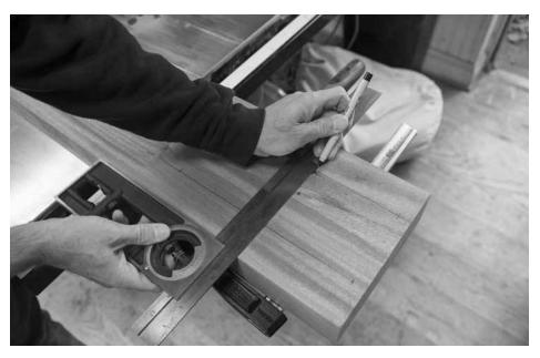
One to one. After marking the layout on one batten, clamp the batten to its mate. Transfer the location of the holes to the second batten.
