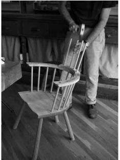
Bring on the mallets. Drive in the back spindles until they bottom out in their mortises. Then start knocking the armbow and the short spindles down.
