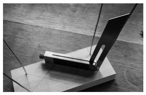
The result. Put the handle of your bevel gauge on the sightline. Set the blade to match the leg. That's the resultant angle – you just did a good thing.
