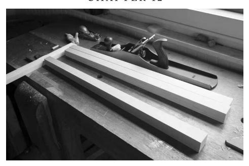
All downhill. If you use straight (or rived) stock for your legs, planing the tapers should be easy. Plane from the bottom of each leg to the top until the tops of the legs are 1-1/4" square.
