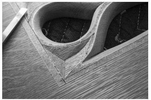
Quick chips. The triangular depressions at the corners of the piercings are easy to make with a chisel and mallet.
