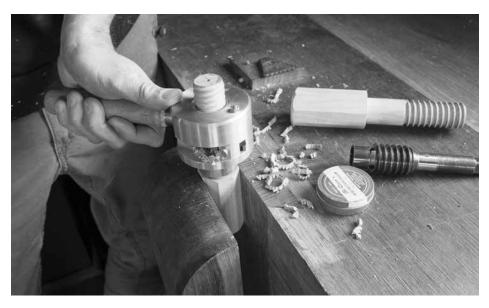
Totally screwed. The wood threader cuts nice threads if the tool is well-lubricated. You can use tallow or wax. Another way to get clean threads is to soak the shafts in boiled linseed oil for a couple days before threading. No, it won't gunk up the cutter.
