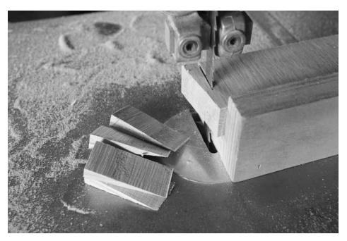
Band-saw wedges. This shop-made sled is angled at 2° to the blade. So by making a cut and flipping the stock to make a second cut, you make a wedge with a 4° included angle.
