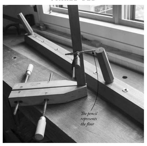
Flat-footed. Clamp a mechanical pencil so it marks the exact length of the legs. Shift the entire jig around to mark all the facets on the legs.
