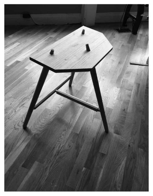
Better. Here the simple tapers have kicked in and the stretchers are proportional to the rest of the piece.
