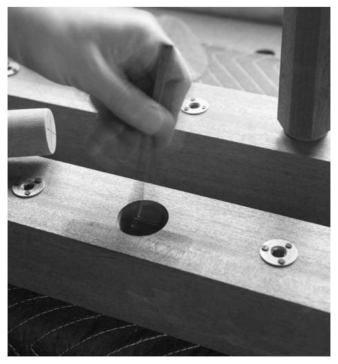
Twist again. Paint the mortise and tenon with liquid hide glue then twist the leg into its mortise. Whack it with a mallet to get it to seat fully.
