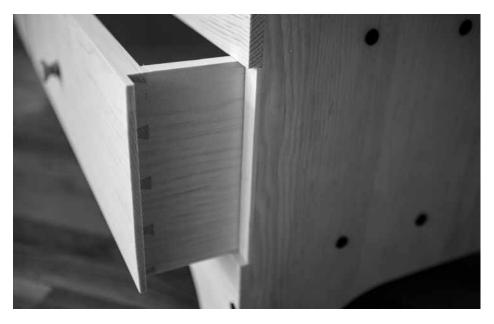
A scab. You can see the thin filler piece I added to the carcase to make the drawer sit flush and tight when closed. This error was caused by making the false drawer front too thin.
