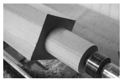
It's a dowel. A cylindrical tenon has all the hallmarks of dowel joinery. It is simple to make but weak in service. Chairs made using dowels are doomed from birth.
