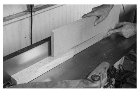
Pop the wheelie. A substantial push stick will push the leg into the correct position for the second pass. This time the top of the leg is first across the cutterhead.
