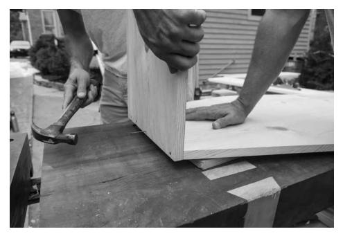
Prop it up. Hasluck suggests propping the bottom up on a scrap to make it easier to nail on the headboard and footboard. Good call.
