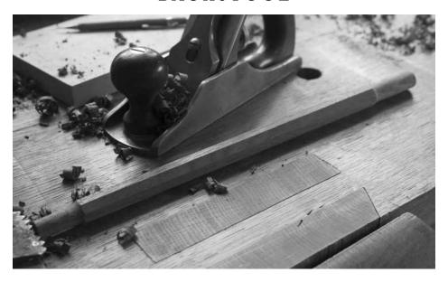
Tapered octagons. After creating the tenons on the ends of the octagonal spindles, I used a plane to taper the spindles to get smaller at the top.
