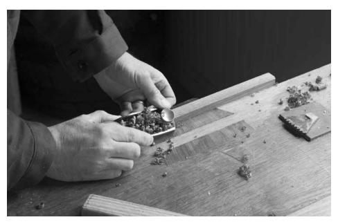
Automatic chamfers. Consistent chamfers are easy with a block plane. Clamp the work in your face vise so it is about 3/8" above the benchtop. Rest one corner of the plane on the benchtop and plane for 20 strokes. Flip the board over and repeat.
