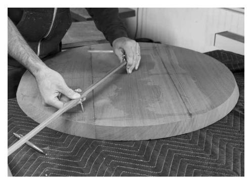
Scribe the circle for the joinery. With the trammels set to a 12-5/8" radius, scribe a line for the joinery all the way around the smaller circle on the subtop.
