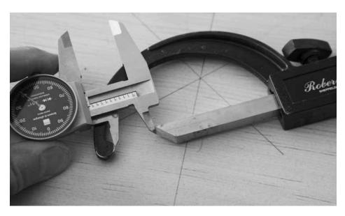
How this works. The bedan tool's sizing attachment is set to .940" – the diameter of the bit for the leg mortises. Slide the sizing tool toward the cutting edge until it matches this measurement. Then lock the position of the sizing attachment and make a test tenon. Really. Test tenon. Don't ignore me.
