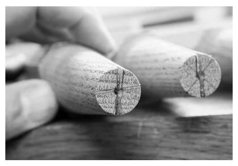
The right kerf. In the top of each leg, saw a kerf that is perpendicular to the annular rings of the end grain. This will help keep the leg in place over the long haul.
