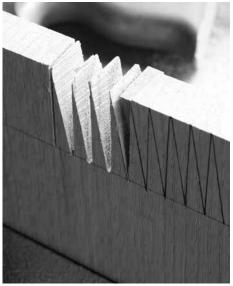
Sawing practice. Wedges are a good way to warm up for dovetails. Half the wedges will fall out as you make these rip cuts. The remainder can be released by crosscutting the end off the board.
