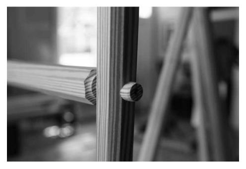
The joint. Here's the through-tenon after drilling. Not bad for freehand work.
