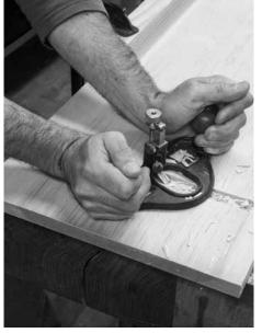
Clean-up. The router plane will make the bottom of the dado perfectly flat and the same depth – even if the stock is a bit cupped.
