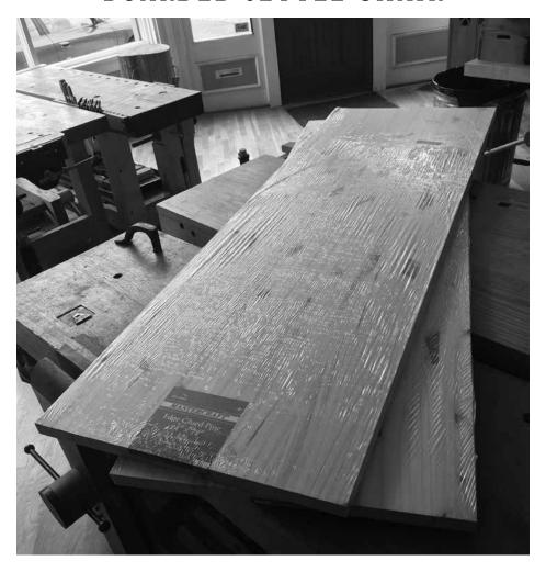
Sealed for your protection? Premade pine panels can speed you up, but they have some headaches built-in – moisture and knots, for example.
