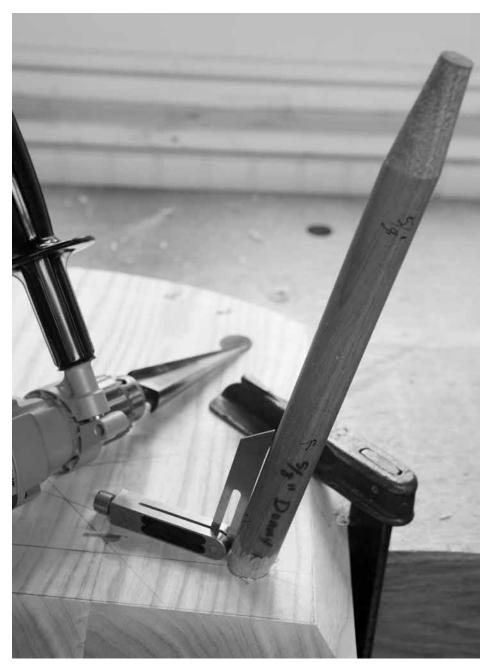
Your dummy. A "dummy leg" that is shaved with the correct tenon shape is a valuable aid when dialing in the correct angle of the mortise as you ream it.
