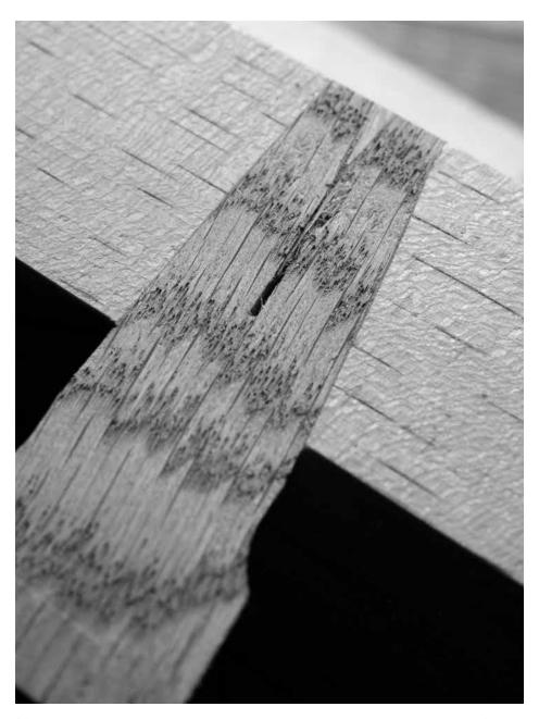
Tighten up. A staked joint can be as simple as a cylindrical mortise and tenon. Or it can be as complex as a tapered mortise and tenon that is back-wedged, as shown here. The advantage of this conical joint is that it gets tighter with use.
