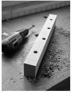
Drill, then saw. The crest is more stable on the bench and easier to drill while it is thick and square.
