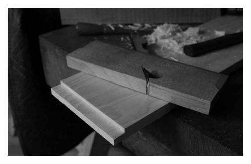
Clean rabbet. The batten helps ensure the shoulder of the joint is crisp and square. If it's a tapered mess, clean it up with the rabbet plane run on its side.
