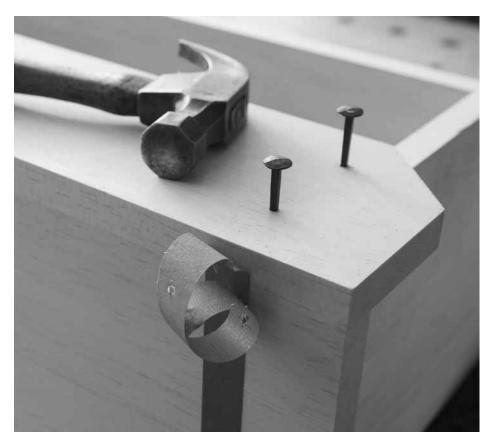
Driven. Headed nails hold the aprons in place much like a nut and washer hold machine-screw parts in place. So I recommend headed nails (such as roseheads) for a long-term joint.
