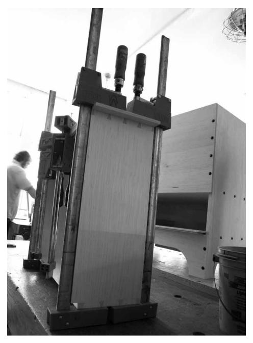
False front. Here you can see one dovetailed drawer with a false front glued and clamped in place. The false front creates a rabbet that fills in the empty area between the plinth and the chest's front (also seen in the background).
