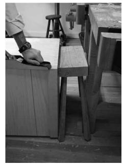
A good stand-off. Here my sawbench allows me to plane a carcase component without the plane ramming into the workbench.
