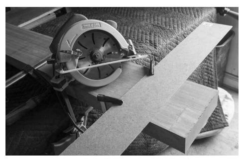
Accurate sawing. This can be done with a handsaw or a circular saw. If you cut the battens with a circular saw, clamp the two battens together then clamp a fence to the work to guide the saw.
