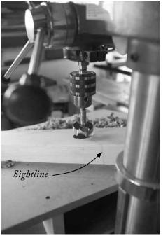
Boring mortises. Here my batten is clamped to the jig's platform, which is 16° off horizontal. The sightline is drawn on the batten – I've extended it off the edges of the batten to make it easier to line things up on the jig.
