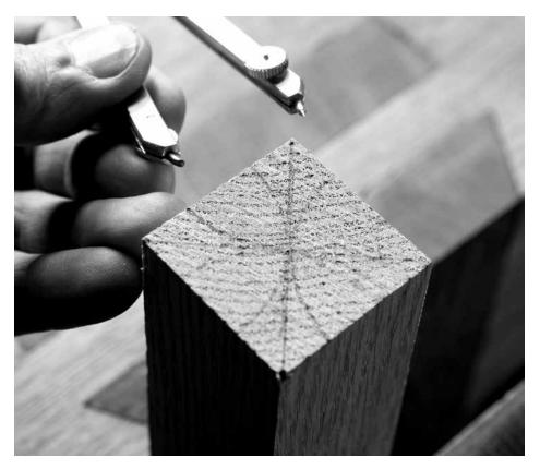
Easy octagons. To turn a square into an octagon, set your compass so it spans the space between one corner and the centerpoint of the square. Then, with the pin of the compass on the corner, scribe an arc. Repeat on the other three corners. Connect the endpoints of those arcs and you have an octagon.
