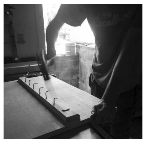
Finish the deed. Then drive the tip of the nail back into the work – making sure the tip goes across the grain.
