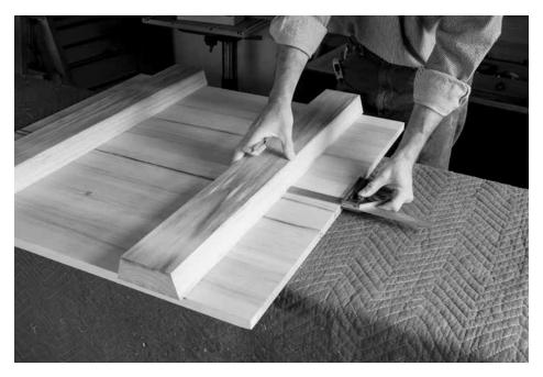
Square helps. Because the ends of the tabletop are square, you can use a combination square as shown to lay out one wall of the sliding dovetail socket.
