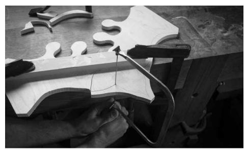
Cut vertical. I find that I can keep the coping saw's blade perfectly vertical if the work is horizontal and the blade is vertical. A traditional bird's mouth support platform can make this easier.
