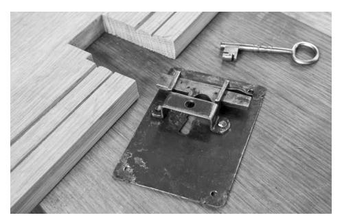
Install the lock. Sometimes a through-mortise is the best way to install a handmade lock. Begin the layout process by tracing the lock's shape on the door.
