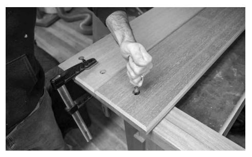
Mark, don't measure. Position the slats on one batten as they will go when everything is assembled. Then use the 31/64" drill bit to transfer the location of the holes from the slats to the batten below.
