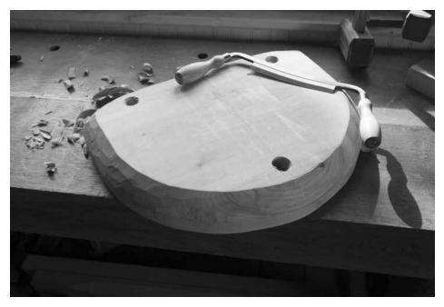
Easy peeler. You can remove a shocking amount of material with a sharp drawknife. Use a slicing motion; move the knife laterally as you pull it toward you. You will quickly get a feel for the seat's grain direction, even if it's your first time with the tool.
