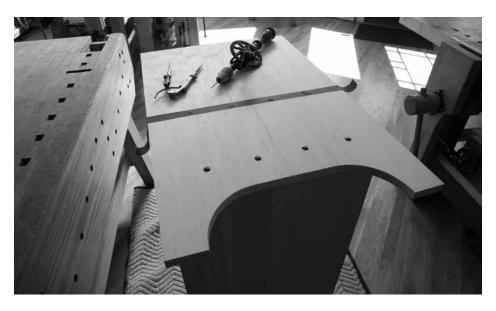
Template tape. Blue masking tape helps guide you as you drill your pilot holes. Once you finish one row of nails, pull up the tape and move it to the next location.
