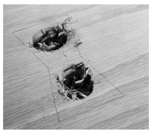
Room to chop. Bore out some waste to make the chopping easier. The holes also act as depth stops.
