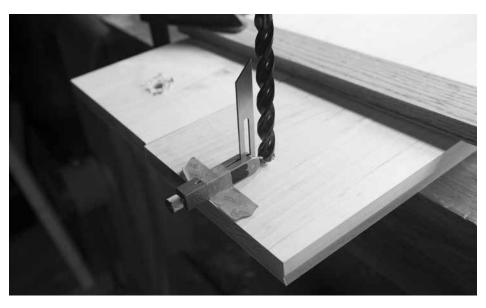
A clean exit. When boring the mortise with the auger bit, bore until you can feel its lead screw poke through the top of the plank. Then flip the plank over and bore the exit hole. Here I'm using the bevel gauge to guide me.
