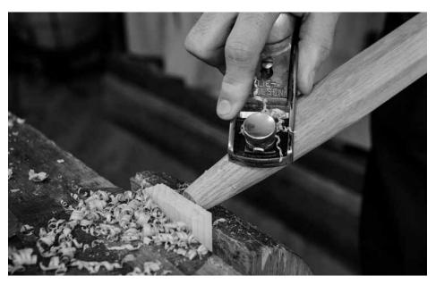
Remove the bulk. A rank-set block plane removes the high spots pointed out by the tenon cutter.
