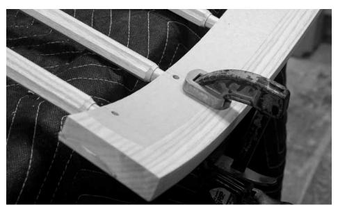
Protect your back. Where the bit exits the crest rail is vulnerable to splintering. So I clamp a bit of curved wood to the exit point. (You can't see it because it's under the crest rail.)
