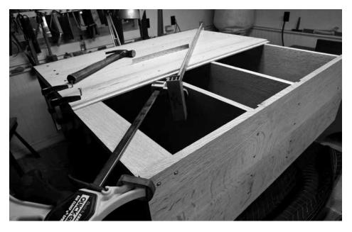
Rack the back. Here I'm pulling the case square with two clamps. Then I nail the backboards in place. When I release the clamps, the carcase will remain square.
