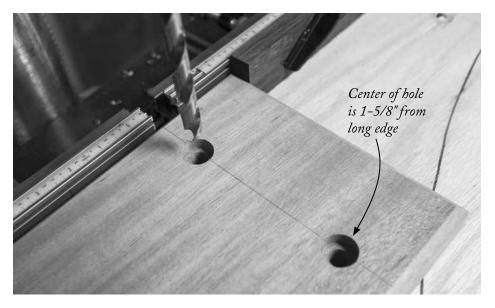
Counterbore first. The 7/8"-diameter counterbore holds the washer and head of the cap screw. Bore the counterbores first. Then follow up with the 31/64" through-holes.
