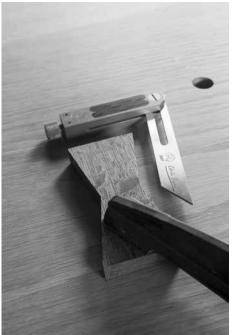
Check insurance. Clamp the key across the split and trace around it with a knife. Note the split is difficult to see here, but it crosses the key at its narrowest point.
