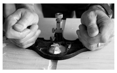
Press & push. After you clean the bottom of the dado, you can also clean up the joint's sidewalls by pressing the cutter of the tool against the wall and pushing. The bevel of the cutter will scrape the sides of the joint.
