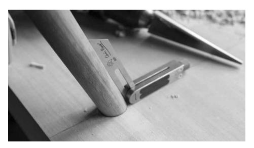
Ream & confirm. Ream each mortise and check your progress as you go. I have a 3/4"-diameter dummy leg with a tapered tenon cut on one end that I use to check the angle of the leg and the progress of the reamer.
