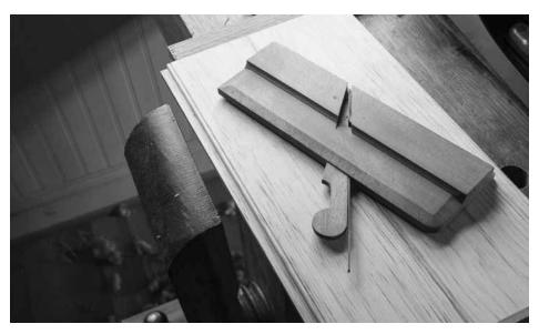
A strong bead. Bead the shoulder of the tongue section of the joint. If you bead the groove section you will weaken the joint.
