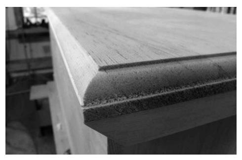
Across the grain. Cut the moulding across the ends of the lid first. Then cut the front edge with the same moulding plane.
