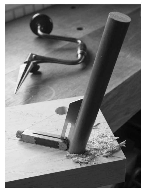
One angle. The bevel gauge is set to 15° and has been placed on the sightline on the underside of this sawbench. This "resultant" angle allows you to drill the holes for your legs with one line and one setting of your bevel gauge.
