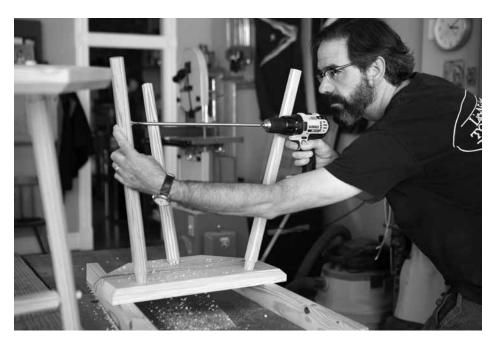
Hot dogging. Keeping the drill level and in line isn't as hard as you might suspect. Note that I have rotated the leg a bit so the inner flat face of the leg faces me.
