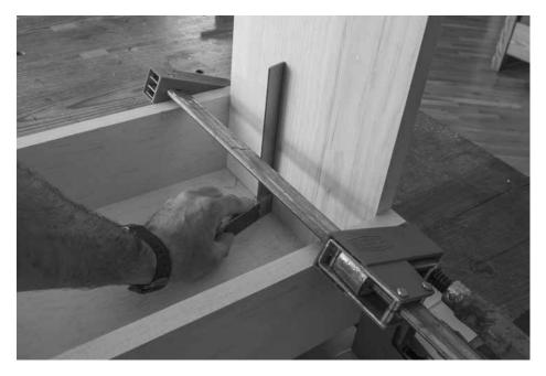
Square all around. Clamp the leg in place and use a mallet to tap it around until it is perfectly 90° to the seat and the aprons.
