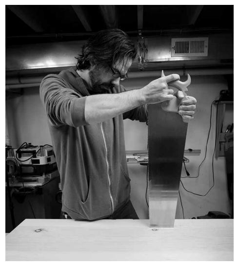
Rip, then crosscut. Rip the moulding from your boards before crosscutting the front and back pieces. It will make the moulding process easier and faster.
