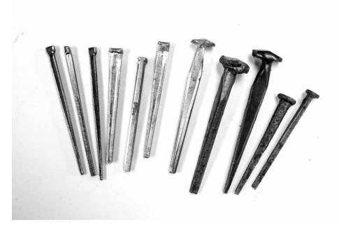
Cut one for me. Cut nails taper along two edges and don't taper on the other two. This taper is a result of the way they are sheared from a plate of steel or iron. Then the fasteners are headed by the machine.
