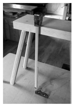
This high. The length of the tape indicates the final height of the sawbench. The combination square below records the amount of wood that needs to be removed from the legs.
