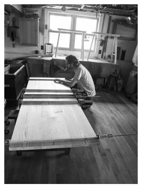
Feel the difference. I use a slow-setting liquid hide glue when making big table-tops. The extra assembly time allows me to shift the boards around as I apply clamp pressure.
