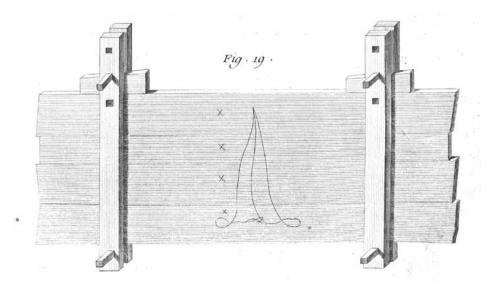
Forever together. The marriage mark – or cabinetmaker's triangle – keeps parts oriented before and after assembly. A better or simpler system has yet to be devised.
