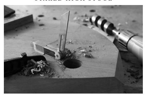
Quick joinery. Tapered mortises and tenons are not tricky to make as long as you have a reamer and tenon cutter that have matching included angles.
