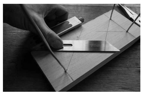
Mark the sightline. Use your bevel gauge to draw in your sightlines on the underside of the model. You are almost done. Unlock the bevel gauge.
