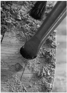
A handy notch. This V-shaped notch tells you when to stop drilling the mortises in the seat of the chair.
