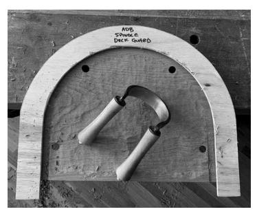
Safe scorping. If you have trouble nicking the spindle deck, apply a thin layer of plywood over it to protect it. I stuck mine on with carpet tape.
