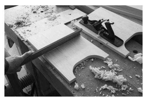
Get it flat. Here I'm working on the interior surface of a leg panel. It needs to be flat so it meets the shelf without a gap. But it doesn't have to be beautiful because it's not very visible. So a little tear-out or a few plane tracks aren't going to matter.
