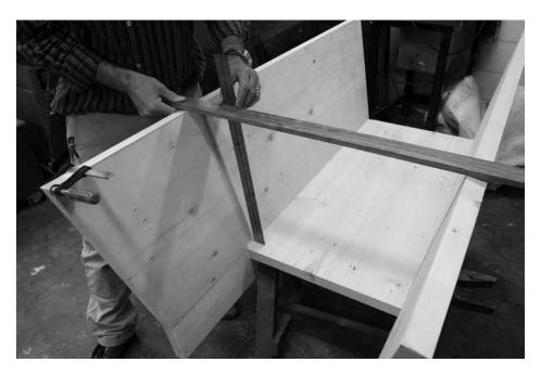
Two straight lines. The wooden straightedge represents the front edge of the seat. The perpendicular steel ruler determines the true depth of the seat.
