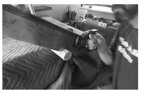
Compound crazy. This angle is something odd. Your best bet is to make a shallow kerf on four faces of the octagonal leg before sawing the waste off. The shallow kerfs will guide the saw during the cut.
