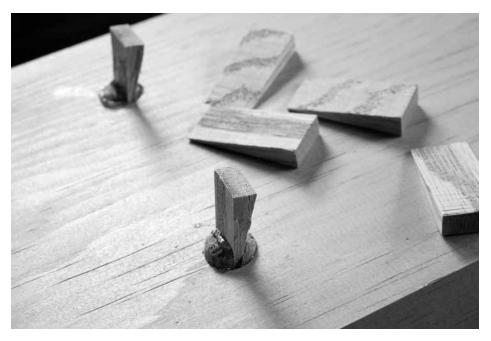
Grippy, not splitty. The wedge will be applied perpendicular to the grain of the top. If it were parallel, the top might split.
