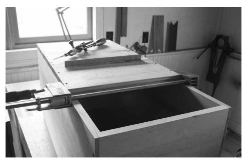
Nails all around. Don't glue the bottom boards, just use nails. I drive three nails into the ends of the carcase. Then I space the nails every 4" or 5" when nailing into the front and back of the carcase.
