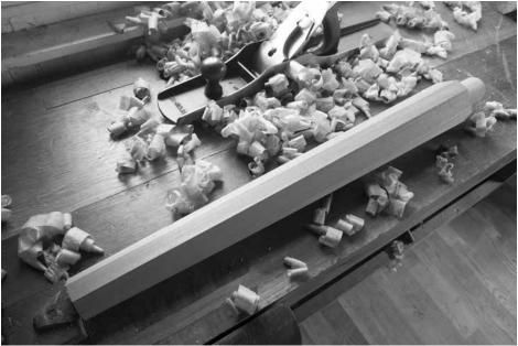
Work to lines. Here you can see the lines that demarcate the tapered octagons. Once you have layout lines such as this, it's easy to plane nice octagons.
