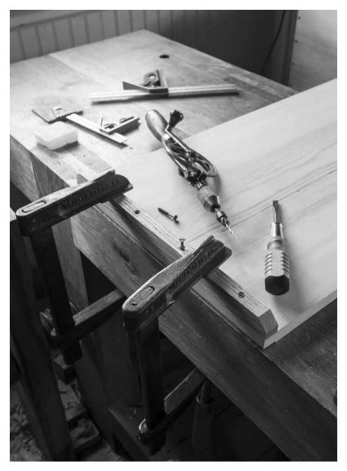
Screws that move. By elongating the clearance holes in the battens, the threads of the screw will stay tight in the lid (usually) without splitting.
