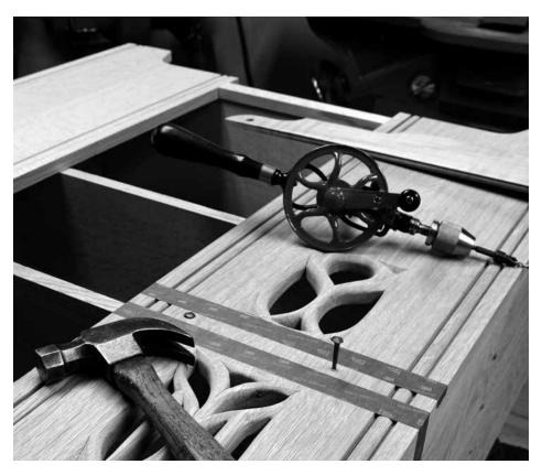
Nail job. The pilot holes for the nails should be about two-thirds the length of the nail. That will give the nail the holding power it needs to keep the face frame on.
