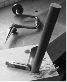
A smart dummy. Here I have shaved a dowel from another project to the shape of the tenon for this project. I can check and adjust my reaming using the dummy leg.
