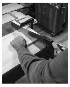
The pusher block. This is the same operation as above, but on the other side of the fence. Note the pusher block.
