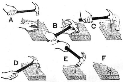
Figs. 177 to 182.—How not to drive a nail, or method employed by greenhorns and some amateurs. A, stroke I, hits nail (accident); B, stroke 2, hits thumb; C, stroke 3, oblique blow causes hammer to slide off nail and hit board (first dent); D, stroke 4, second oblique blow bends nail; E, stroke 5, side blow to straighten nail; F, appearance of nail and board after "driving."
