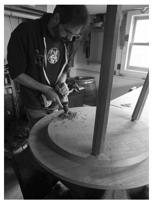
Deeper for strength. To deepen the mortises into the top, insert the Forstner into the existing hole and run your drill up to full speed before pushing the bit into the top. Take it slow and the results will be crisp.
