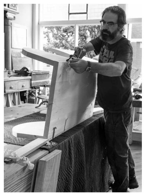
Hide the geometry. It's easier to plane the  $9^{\circ}$  angle on the back after assembly instead of before.
