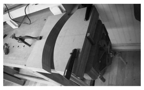
Horizontal press. A vise gives you tremendous mechanical advantage when bending wood. A child can provide enough force to bend a 3/4"-thick crest rail.
