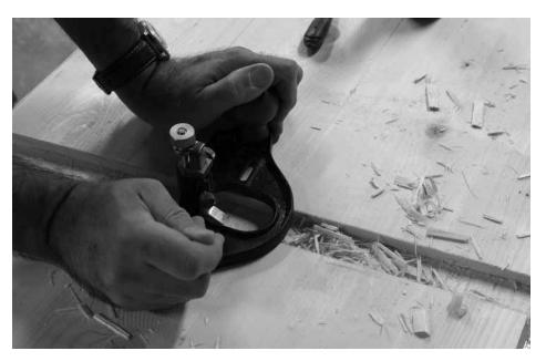
A clean bottom. Shave the fur from the dado's bottom with a router plane. Light cuts work best with this tool.
