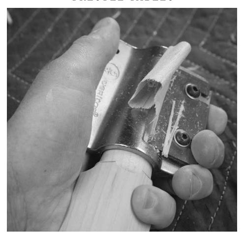
Instant, perfect tenon. The tapered tenon cutter makes a finicky operation easy. Hold the tenon cutter with one hand and the leg with the other. This particular grip allows you to eyeball the gap around the tenon to ensure it is centered on the leg.
