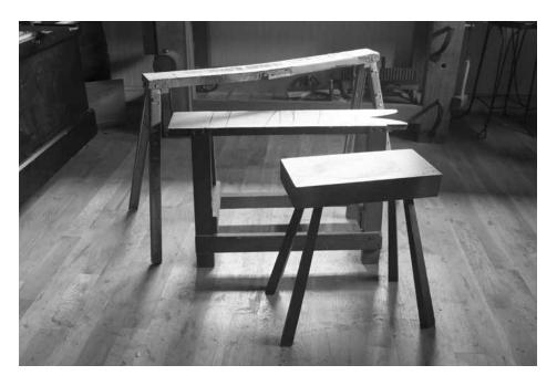
Saw-somethings. All these forms are made for sawing. The sawbenches are for hand-saws. The taller sawhorse is for electric saws.
