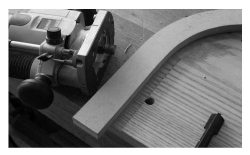
Dirty cheater. I stick the pattern to the seat with double-stick tape. Then I rout the trough by swinging the router counterclockwise around the pattern. Then remove the pattern and the tape.
