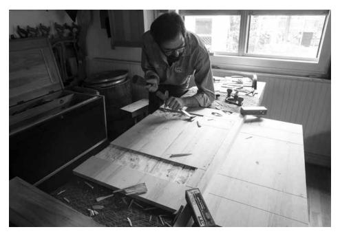
The chiseler. Most of the waste removal is done with the chisel held bevel-down. This orientation of the tool allows you to control how aggressively the tool cuts. If you use the chisel bevel-up, it will dive into the work too quickly.
