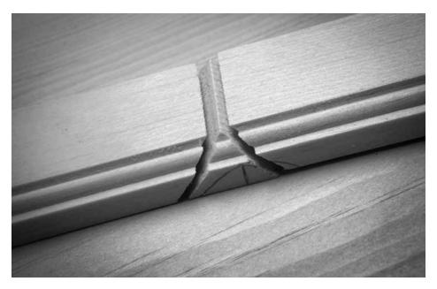
Remember that long rip? Ripping the moulding from a long bit of wood allows you to do this. When these two miters go together they will match perfectly.
