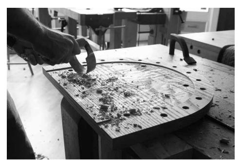
Across & angled. The grain in this seat runs from left to right. So, when I scorp the material, I work across the grain but have the cutting edge skewed slightly toward the right. This helps control tearing. As the saddle gets deeper you'll have to adjust the tool to always work downhill.
