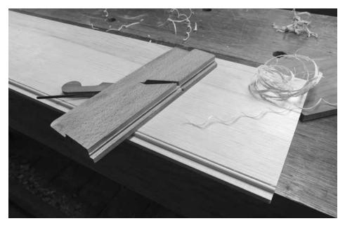
Shiplapped & beaded. The backboards have a 1/4"-thick x 5/16"-long tongue on their long edges. On the tongues that face the viewer, I cut a 3/16"-wide bead to help conceal the joint between the backboards.
