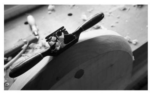
A close shave. A flat-bottom spokeshave set to a fine cut will remove the tool marks left by the drawknife. Stop refining the surfaces when you are satisfied.
