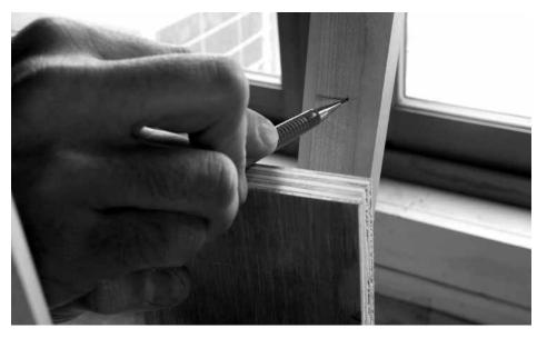
Marking mortises. The scrap is a platform for the pencil. Mark the mortise locations on both legs and mark at least three flat faces of each octagonal leg.
