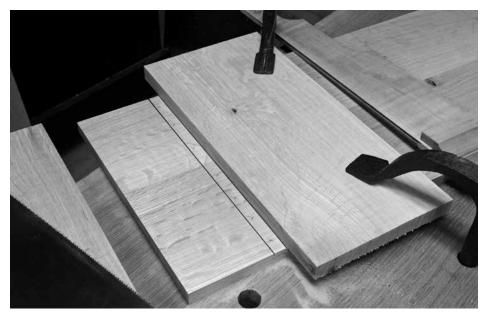
Second wall. Because of the set of the saw's teeth, clamp the batten so it covers your layout line for the second wall. This will ensure your dado isn't too loose.
