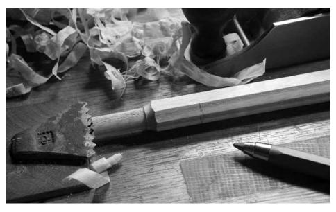
Taper the spindles. The spindles should be skinnier at the top. I tapered mine using a handplane. The guiding light was the shape and size of the shoulders at each end of the spindle.
