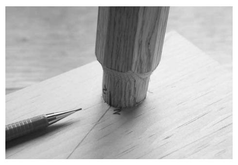
Important marks. Number each tenon and mortise. Rotate the tenon so the annular rings of the leg's end grain are parallel to the top's grain. Then mark the tenon and top.
