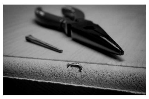
Clenched batten. The nail passes through the lid batten and the lid, then is bent back into the wood like a staple.
