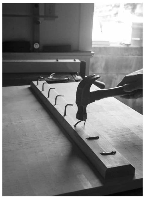
Clenched. The tip of this nail has been diverted back into the wood to hook two pieces of wood together. The only way the joint will fail is if the wood or nail is destroyed.
