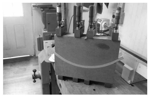
Clamp & set aside. With the form closed on the stick, clamp the form tight. Remove it from the bench and set it aside for a few days.
