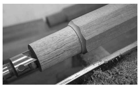
Turn the tenon. The cylindrical tenons for this bed are 1-1/2" in diameter and 2-1/4" long. The little cove I turned at each tenon shoulder is 100-percent decorative.
