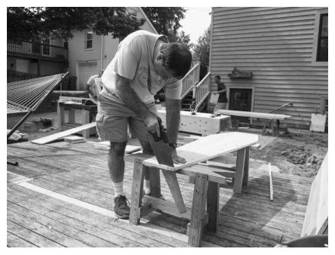
Bigger at the top. The top and bottom of the coffin toe out about 6°. Cut this bevel on the ends by eye with a handsaw. Plane the ends smooth.
