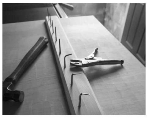
A good start. A pair of pliers allows you to bend the tip of the nail in the desired direction. Note that large works requires longer clench nails, as in this example.
