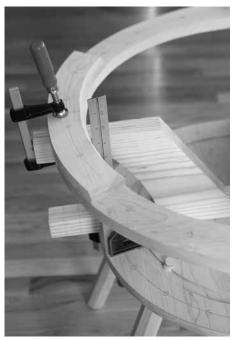
Here. This is where I like the back of the armbow to go. Its inside edge lines up with the outside edge of the seat. The square shows this relationship clearly.
