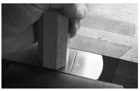
Fine-tune the feet. Clamp a block plane in a bench vise so its sole is coplanar to the benchtop. Pull one of the long legs across the cutter.
