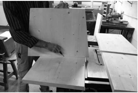
Start a dado. Lay out the dado using a knife. A knife will sever the grain, making for a clean arris. Once you lay out one wall of the dado, use the seat to lay out the second wall.
