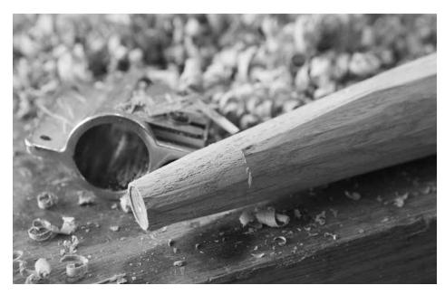
Where to cut. The tenon cutter tells you where you need to remove material.
