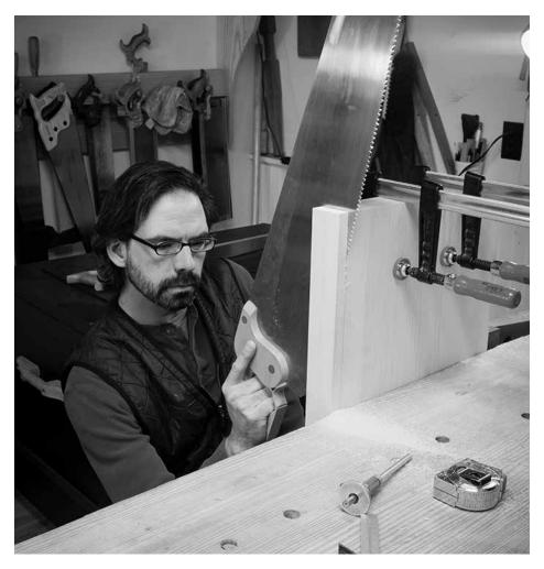
An easy rip. Cut the notches simultaneously and you will get better results. The thickness of the two pieces will make it easier to stay 90° to the face.
