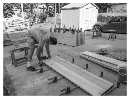
Glue up. If using dimensional wood, you'll need to glue up at least two boards to create the bottom, sides and lid. My coffin was less than 23" wide – just enough to squeeze by with two 1x12s.
