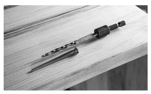
Tape marks the stop. The pilot hole should stop short so the nail has to burrow its way into the material. Here I'm using a tapered drill bit for the pilot holes. It isn't strictly necessary, but it helps.
