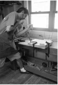
Awkward angles. It's easy to see if the brace is in line with your body along the sight-line. But it's a trick to see if you are doing right by the resultant. The best solution is a spotter to act as an extra set of eyes. Barring that, you can tilt your head around the brace to peek at your progress.
