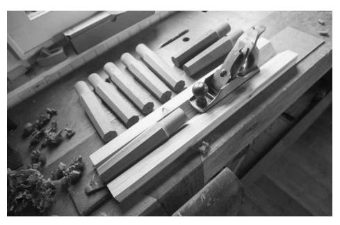
Taper the legs. This simple bench fixture allows you to transform each leg into an octagon, then taper it with a handplane.
