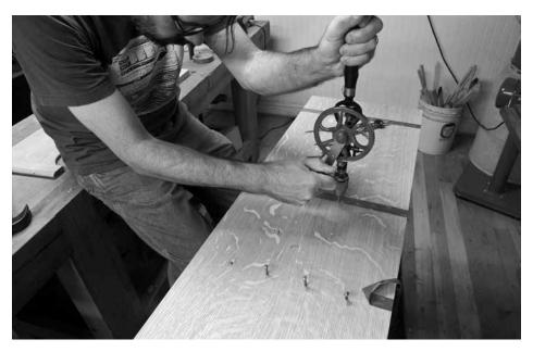
Square nails. Use wrought nails or rosehead cut nails to fasten the sides to the shelves. Use tape to remind yourself where the nails go – the tape is easier to remove than a pencil line.
