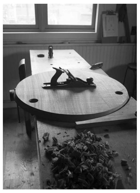
Scraps for stops. Clamp the scraps from cutting your top to your bench and use those as stops to restrain the subtop while planing it.
