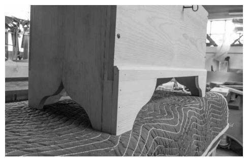
Base bits. Here you can see how the additional foot pieces are added to the carcase to enclose the base on the front of the chest. It's all glue and nails.
