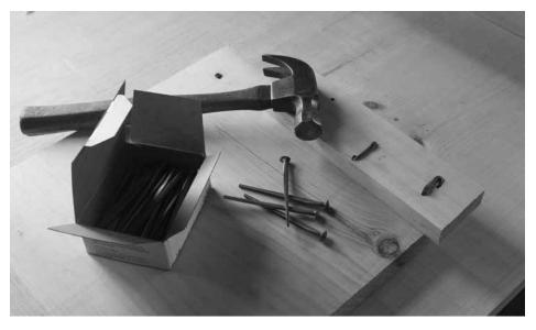
Samples. If you don't know this particular nail like a brother, make test joints and clench the nails to make sure things will work. Repeat the test. Then you can drill the pilots for real. I used eight nails in each batten.
