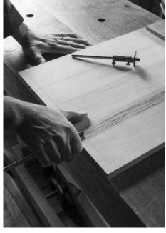
Two triangles. Mark the triangles on the top edges of your panels. Each triangle should point toward the front of the chest and he marked when the panel and its opposite part are placed together.
