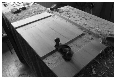
Router it flat. A full-size router plane is just big enough for this operation. If your dovetail socket is too wide, attach a thin and wide temporary sole to the router plane with double-sided tape.
