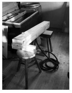
The high-class setup. A steam box with a steam generator makes it easy to get your parts limber enough for bending.
