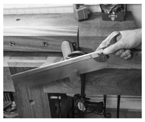
Trim the legs. A carcase saw makes short work of trimming the legs to their final length. Simply follow the pencil lines you marked on the legs.
