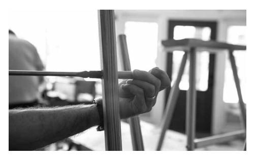
The backup plug. The 5/8" dowel prevents the spade bit from wrecking the mortise as it drills from the outside of the leg.
