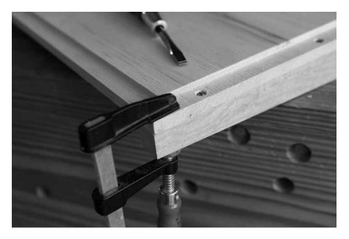
Hold it. A couple F-style clamps hold the batten and lid in place while you drill the pilot and clearance holes for the screws. Here I used four  $\#8 \times 1-1/4$ " screws in each batten.
