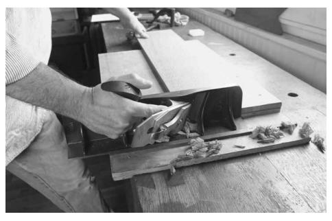
Shoot the bottom. After cutting the till bottom to a close size, shoot its ends until the bottom slides smoothly on its runners.
