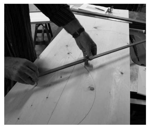
Not for CAD. I recommend you finalize your layout on the workpiece itself. After drawing this up a dozen times in CAD, I realized that direct experience was superior.
