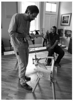
The magic wand. I can see if the drill needs to be adjusted left or right. Brendan, holding the stick, can see if I need to tilt the drill forward or back.
