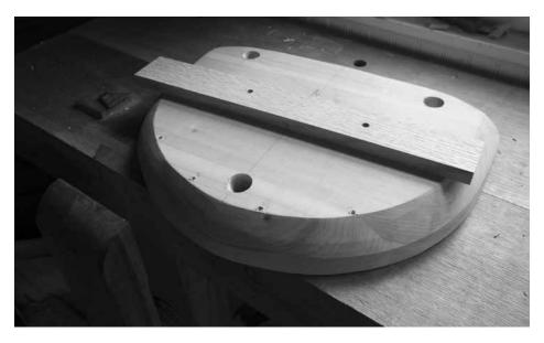
Not fancy. I forget who showed me this trick – perhaps bodger Don Weber. Instead of rigging an odd dog system on your workbench, you can hold the seat in place by screwing a board to its underside. Then clamp that board in your face vise.
