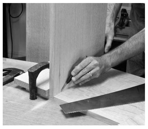
Don't measure. Use the mating shelf to strike the second wall of the dado. Use a pencil or knife to mark this wall.
