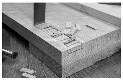
Chop  $\mathcal{E}$  stop. The stopped grooves for the interior rails are made the same way you made the dados for the shelves.
