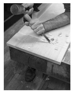
Quick work. Knock the chisel with a mallet to remove the waste. Use the chisel bevel-down so you have more control over how aggressive the cut is.
