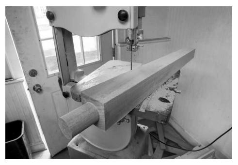
Long tapers. The band saw is ideal for long rips such as this. Lay out the tapers on one face. Make that rip. Then lay out the tapers on the adjacent faces and rip those.
