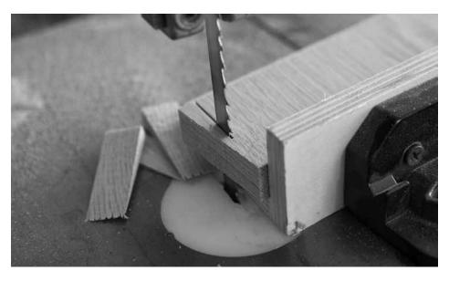
Cut & flip. The advantage to using the miter gauge is it's faster. The downside is that your fingers get closer to the blade at the end of the process.
