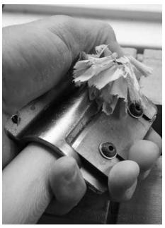
Make a sample tenon. Use your 5/8" tapered tenon cutter to shave the end of a dowel to shape. You will use this to test the angle of your mortise.
