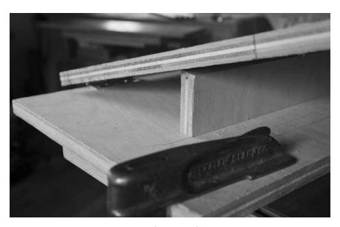
A scrap sets it. A scrap that is screwed (or clamped) between the two bits of plywood sets the angle, as shown here.
