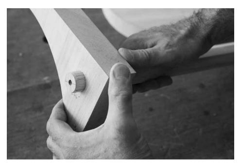
Test each tenon. After I cut each tenon, I check it in the test mortise (made with scraps from the seat). This is a backstop because I don't trust my bedan sizing tool, though it has yet to let me down.
