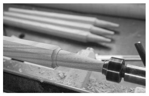
Overly fancy. Once the leg is on the lathe, it's easy to taper the tenon and elaborate. Here I've added a cove at the point where things transition from octagon to round.
