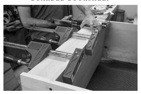
Long-grain kick. The kick is glued in place to the underside of the lower shelf. Then it is nailed in place through the sides of the bookcase.
