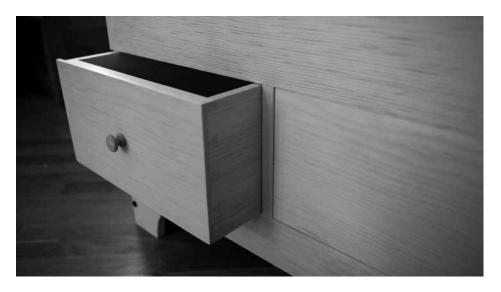
Another scab. I added the vertical divider between the drawers with some glue and headless brads. My original plan was to have the drawers' false fronts fill in this area, but I changed my mind and decided I wanted a vertical element to break up the façade.
