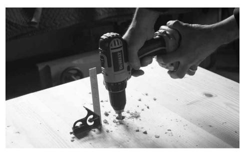
Round & square. Take your time when boring this hole. Check your drill from both axes to ensure it is boring perfectly perpendicular to the tabletop.
