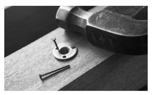
Beat down. Small headed nails hold the weld nuts in place. If you don't like nails, consider using small screws to do the job.
