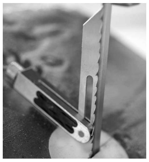
Set to bevel. Tilt the table to 14° and confirm the setting with a bevel square. The exact angle is unimportant, but a consistent bevel is.
