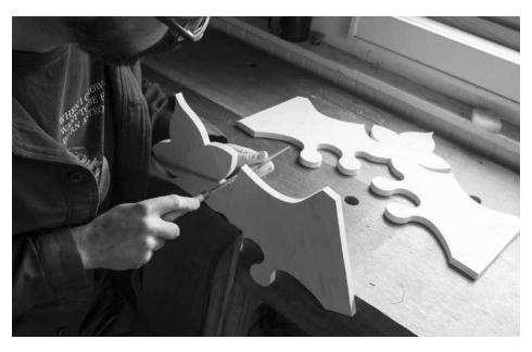
Rasp horizontal. When I clean up the sawblade marks with a rasp, it's easier for me if the work is clamped in a vise. Here I'm using a fine rasp.
