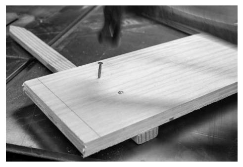
Bounce then clench. Put the work on a metal plate and drive the nail into the work. When the tip encounters the metal surface below the batten, as shown above, it will bend over back into the work, clenching things together.
