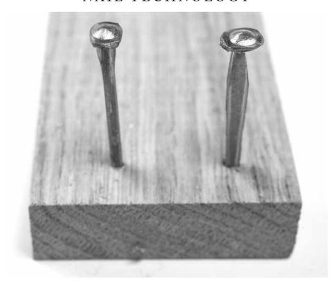
Right & wrong. The cut nail on the left is oriented properly. The one on the right is oriented wrong – its wedge shape is likely to split the wood.
