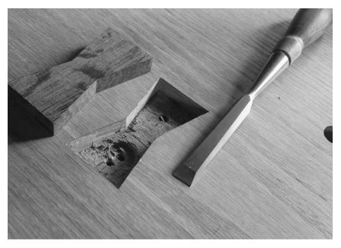
Clean the floor. The bottom of the mortise is where the patch gets its strength. So get it mostly flat. I always leave a couple low spots for excess glue, however.
