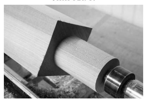
Turn or chisel. The 3"-long x 2"-diameter tenons can be turned on the lathe or pared out with a chisel.
