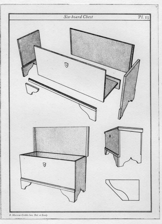
These chests disobey almost all of the rules of wood movement. The grain on the front and back of the chest runs horizontal. The grain on the ends runs vertical. The front and back should have split and fallen off. And take a gander at the lid. The grain of the battens that help keep the lid flat and the dust out is 90° to the grain on the lid.
