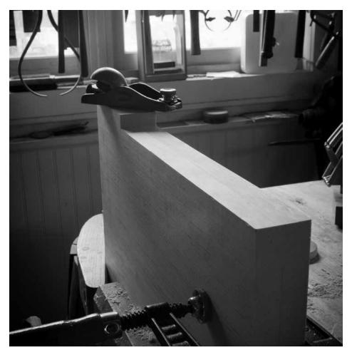
Always together. Plane the notches flat and true with them pinched together. I always seek to do one operation on multiple boards whenever possible.
