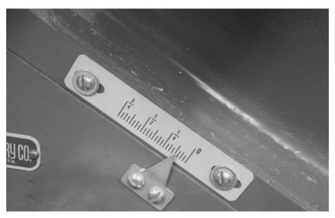
Set the infeed table. If you are going to taper a face of a leg by 1/4", set the infeed table to remove 1/8".
