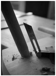
Test it. Place your sample tenon into the mortise and check your work. Correct the angle of reaming if you are off.
