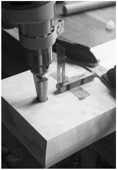
Ream & verify. After every four rotations of the reamer, remove the tool from the mortise and insert the dummy leg. Make small adjustments to how you tilt the reamer to correct the angle.
