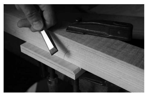
Batten down the rabbet. Here I've clamped a batten to the end of a plinth. The rabbet is marked in with a cutting gauge. And I've relieved the end of the cut with a bevel to prevent the "spelch."
