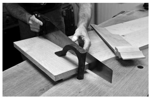
First wall. Clamp a batten on your layout line and saw the first wall of the dado. Press the sawplate against the batten to create a vertical cut.
