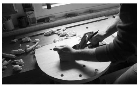
Meet jack. With a properly curved iron, a jack plane can easily create a deep valley in the seat. Set the iron rank. Plane until the tool stops cutting, then shift to the side. Repeat. Check your work.
