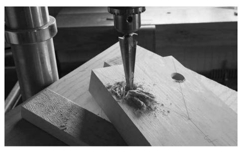
Drill press tricks. One of the problems with using reamers in a drill press is the "throw" of the machine – how much vertical plunge you have. If your drill press doesn't have enough throw you can finish the job by propping your work up on battens, as shown here.
