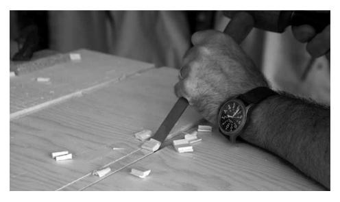
Guided by wrist. Raising or lowering your wrist controls how deep the chisel will cut. Find the right bite, then lock your wrist against the work and drive the tool forward with a mallet.
