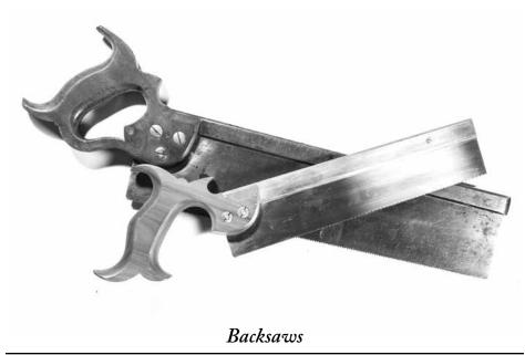
For cutting pieces to final size or cutting joints, you need a backsaw or two. Most woodworkers end up with three backsaws: a 10-point tenon saw filed with rip teeth, a 14-point carcase saw filed with crosscut teeth and a 15-point dovetail saw filed with rip teeth.
