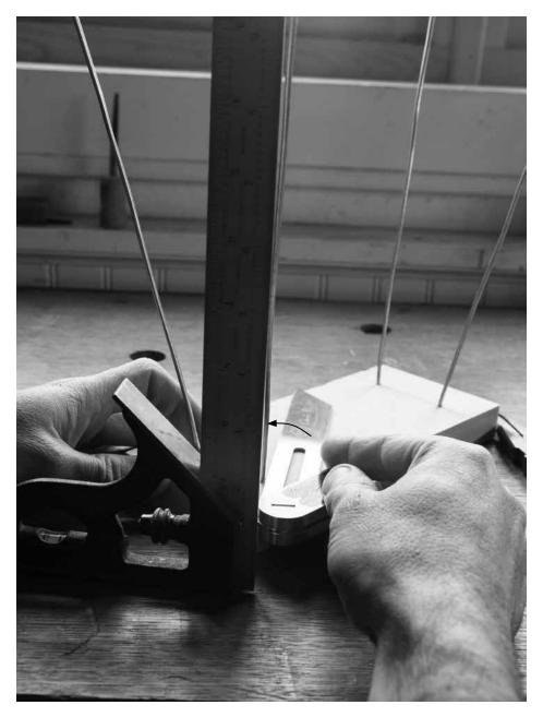
When the tools align. Rotate the sawbench until the leg looks vertical compared to your square. Adjust the bevel gauge until its blade aligns with the leg and square. In the photo I am pushing the blade toward the vertical line made by the leg.
