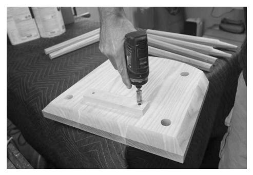
Easy seat. A temporary block on the underside – cheated toward the front edge of the seat – allows you to clamp the seat to plane it flat.
