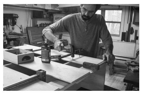
Secure the back. Nailing the back to the shelves helps prevent the shelves from sagging and the backboards from pulling away from the carcase.
