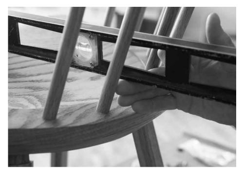
Three fingers. On my hand, three fingers is about 2". Prop up the bubble level with your fingers. When the bubble level reads level, the slope is correct.
