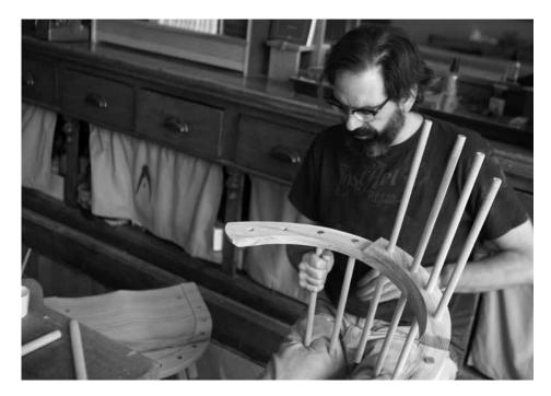
Wiggle up. Here I'm rotating the short stick as I push it upward. This spreads the glue around the joint and allows me to position the kerf in the stick correctly.
