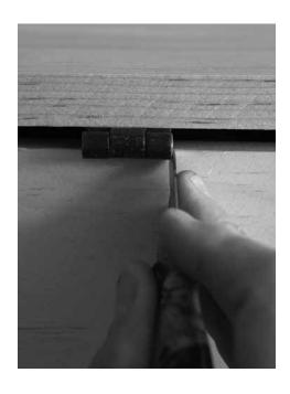
A little nick. I use a marking knife to nick the carcase on either side of the hinges. Then I remove the lid to mortise the carcase. Remove the lid and lay out the mortises to receive the hinges in the carcase. Cut this out with a saw, chisel and router plane. Then screw the hinges to the carcase.
