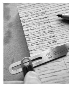
Saw your own. Set your bevel gauge to 2° and mark down to a baseline. Flip the gauge over and mark down to the same point from the first mark. Keep flipping and marking.
