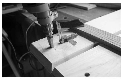
Ream in pairs. Here I'm reaming two legs to make sure they lean at the same angle. By reaming each hole bit by bit, you end up with trestles that look identical.
