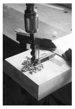
In line. Here I'm boring the rear leg. The centerline is the sightline. The bevel square is set for 4°.
