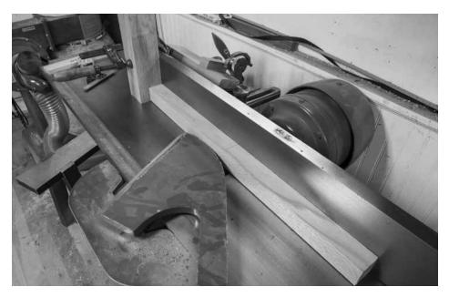
Set the stop. The leg should stop halfway along the taper.
