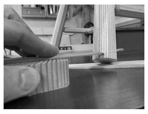
The half-pencil and a block of wood helps you mark out the correct length of the legs.
