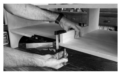
Guides the drawers. Clamp the low divider in place, then affix it with screws from below. Done.
