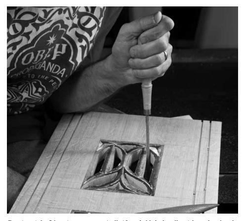
Rasping right. It's easier to rasp vertically if you hold the handle with one hand and the tip of the rasp with the other. Check your work with a square until you get a feel for the operation.
