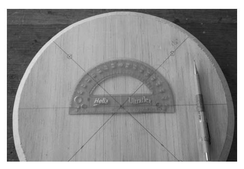
Good layout. There are 100 ways to do this. Place the protractor on your line and mark the seat at 45° on both sides of the protractor. Connect these marks to the centerpoint. And done. Perfect.
