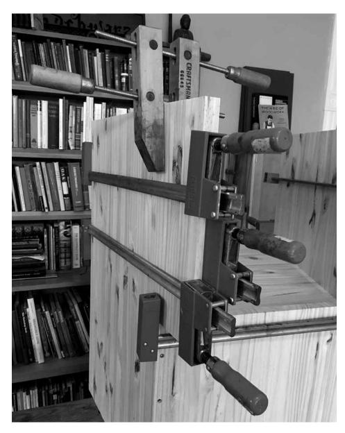
Tricky clamping. This is a second (and ultimately unsuccessful) chair I made, which is why things look odd. Here's how to clamp the back feet to the sides. Apply glue to the edges. Use a handscrew to pinch the two parts to keep them aligned. Then apply bar clamps. Start clamping next to the handscrew and work down. Place bar clamps on both faces of the joint.
