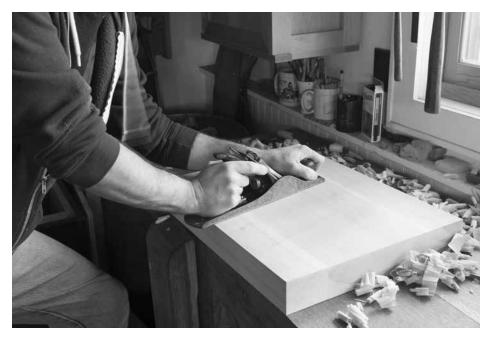
Thickness by hand. By traversing the seat blank with a jack plane, you can quickly flatten it and get it to its finished thickness. Don't bother removing the furrows – called "dawks" – left by the jack.
