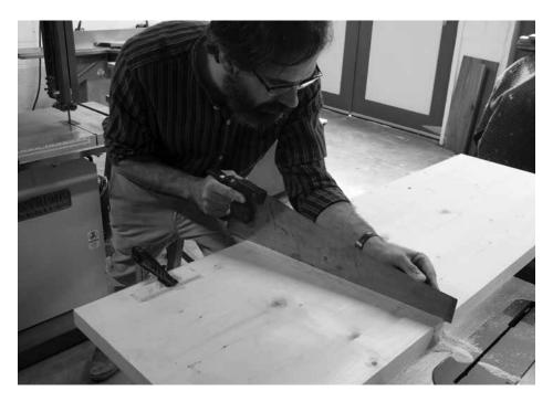
Two-handed saw. Nibble next to the knife line along the entire wall of the dado before trying to make significant progress in the depth of the cut. Once you have laid in a kerf all along your knife line, use your off hand to keep the toe of the saw engaged and square to the work.
