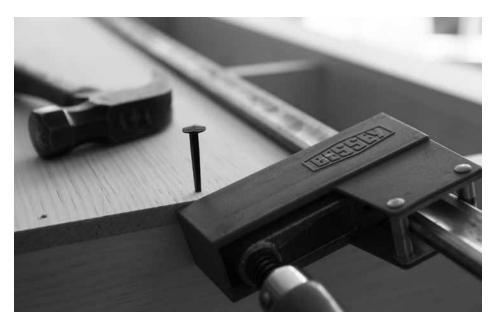
One clamp. Clamping the end grain - hard - helps prevent splits.
