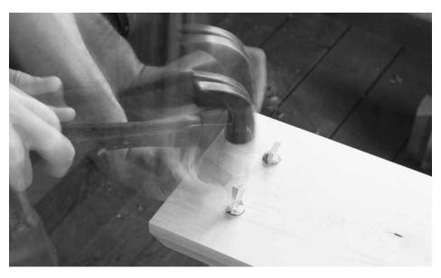
Back-wedging. I use oak wedges with a 4° included angle to back-wedge the tenons in their mortises. Paint glue on the wedges and drive them in with a hammer. When the wedges stop moving into the joint, stop hammering them.
