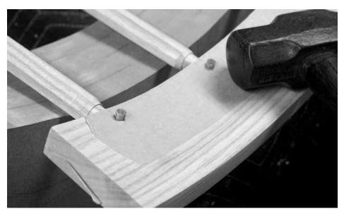
Tight fit. I protect the crest rail with masking tape on both faces before drilling holes for the pins. The tape prevents glue from sticking to the crest rail.
