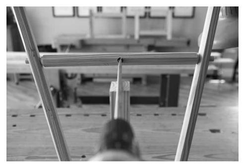
A crutch. If you aren't confident in your drilling you can cut a block of wood to the exact height required to keep your drill level. This works as long as you can clamp the block firmly in place.
