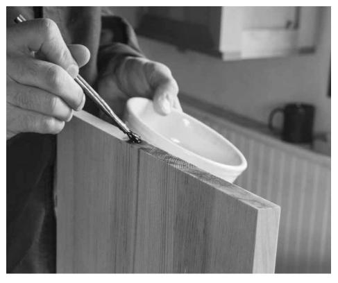
A minute for strength. The thin coat of glue size on the end grain is an important component of a strong rabbeted butt joint.
