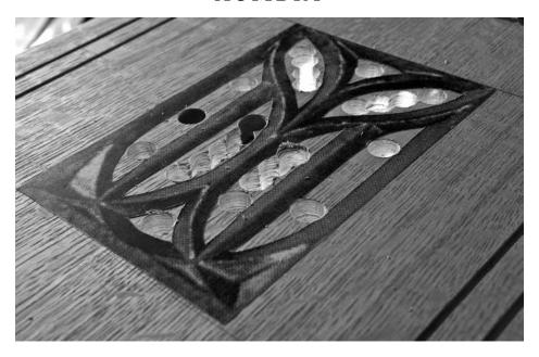
Pattern & piercings. Apply the pattern with spray adhesive and drill out the waste with a 1/2" Forstner bit.
