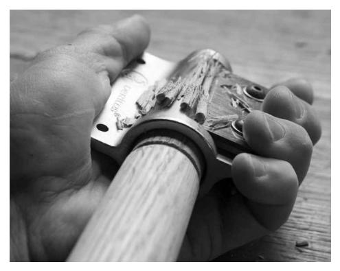
Eyeball that gap. Hold the tenon cutter and leg like this to ensure the tenon will be centered on the leg. If you cannot see the gap between the tool and the leg then you cannot control it.
