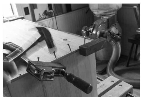
A clamp for safety. Clamping across the joint significantly reduces the chance you will split the top part of the joint or the board below. Note the alternating slopes of the nails – sometimes called "dovetailing" a nail.
