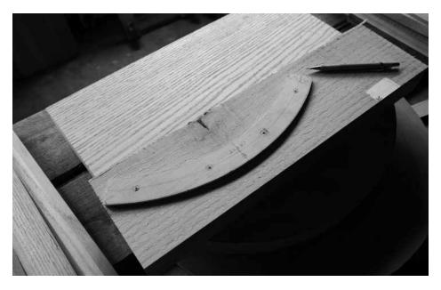
Around the knot. Your curved components will be stronger if the grain is curved. Look for curved grain around knots and from boards that came from the base of the tree in particular.
