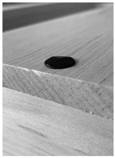
No clamp & with clamp. Without a clamp, the nail dislodged the end grain and split the work. With the clamp pressed hard against the end grain, there was no problem. There are limits to this trick, I'm sure.
