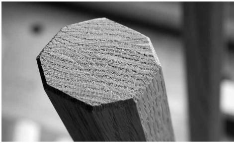
Foot protection. Chamfer the feet with a rasp or plane. This will protect the legs from splintering when they are dragged across the floor.
