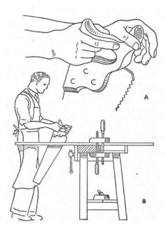
Overhand rip. I prefer to rip at the bench with the work secured like this or with it parallel to the benchtop – with the waste hanging off the front edge.
