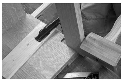
Knock & nail. Drive the interior rail in place. Then fasten it from the outside of the case with two 6d rosehead nails at each end.
