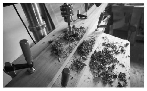
The easy mortise. The mortises for the middle legs have a 90° sightline and an 18° resultant angle. The mortises should be about 2-1/4" deep.
