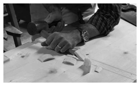
A ripper. Bash out most of the waste between the walls of the dado with a chisel. Begin working bevel-up. Then work bevel-down. Get as close to the bottom of the dado as possible. Chisels are fast. Router planes are slow.
