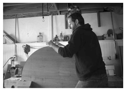
Shaved round. A sharp spokeshave makes short work of the sawblade marks. The standard shave with a flat bottom will work fine.
