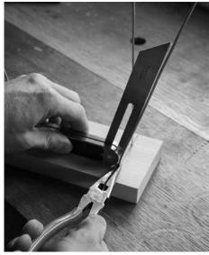
Make the rake. Use the pliers at the base of the legs to bend them to 14° to match your bevel gauge.
