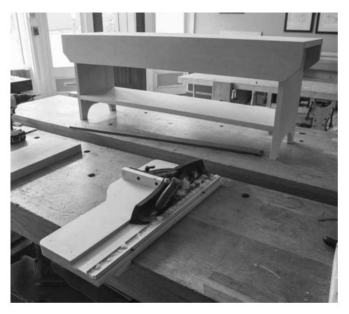
An easy shot. If the legs are square, then the shelf should slide right in. If the legs aren't square, you'll have to taper the ends of the shelf to fit the odd-sized hole.
