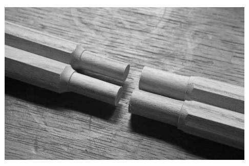
Tenons sized. The spindle tenons should be carefully shaped to final size so they have to be driven with a hammer into their mortises. I turned these on a lathe and added a cove as a transition between the octagon and round shapes.
