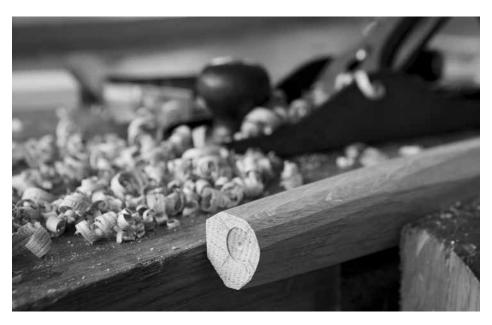
Jack the waste. A coarse-set jack plane makes short work of this oak leg. Here I'm removing half the waste around the tenon. Then I'll finish the job on my next go-around.
