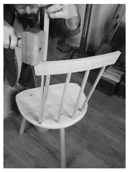
Knocked flat. Tap the crest up and down until it is parallel with the seat board. It might look cockeyed, but that's because you haven't leveled the feet of the backstool. Obey the tape measure.
