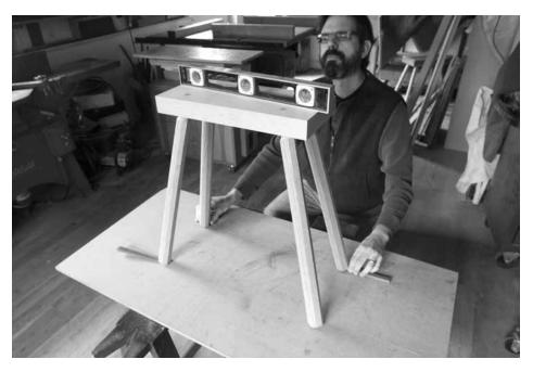
Level the playing field. Level the top of the sawbench by sneaking wedges under the feet until the sawbench is level from the front and the side.
