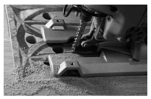
Saw out the windows. Use a jigsaw set with minimal orbit to remove waste as close to the line as possible. I used a standard jigsaw blade for this. I tried using a narrow blade intended for scrollwork, but it deflected too much.
