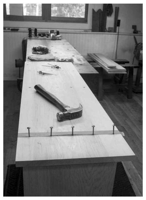
Tape guides me. I use a strip of painter's tape to lay out the location of the nails on the sides of my carcase. Once I lay out the pilot holes on the first joint, I mark the location of the pilot holes on the tape with a marker. Then I re-stick the tape to a new place.
