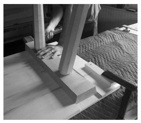
Ready for glue. Only the front 1" of the joint should get glue. This drives all the wood movement in the tabletop to the back edge.
