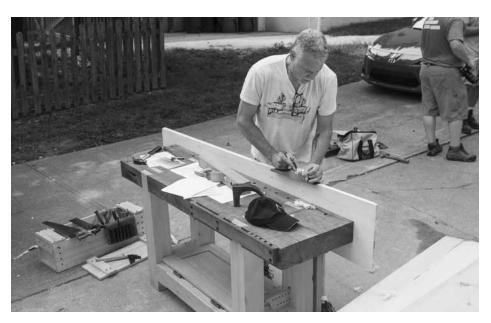
Easy jack work. Mark the 2" taper on one of the long edges of the sides. Remove this material using a jack plane. Plane the second side to match the first.
