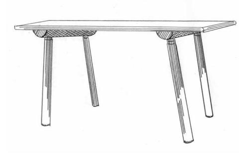
Pre-Lincoln logs. This Scandinavian table uses split logs as a way to beef up the joinery area between the legs and the tabletop.
