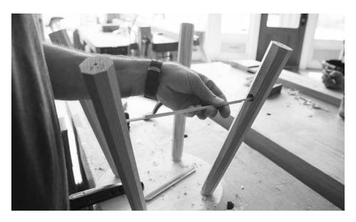
Tiny test tenons. These thin offcuts determine the final length of the stretcher. Pinch them together and mark across the offcuts. Remove the pieces and reassemble them to determine the final stretcher length.
