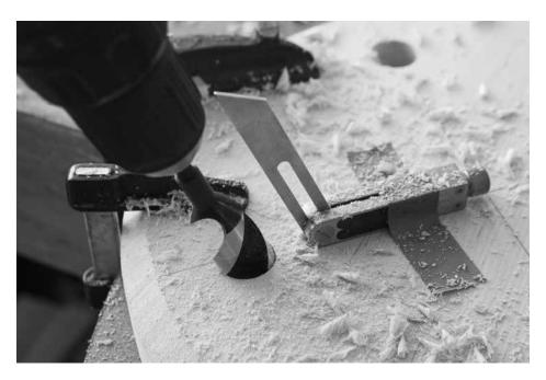
The tape helps. The vibrations from boring can make your sliding bevel move. And even a little bit of movement makes a big difference in the leg angles. So spring for the tape.
