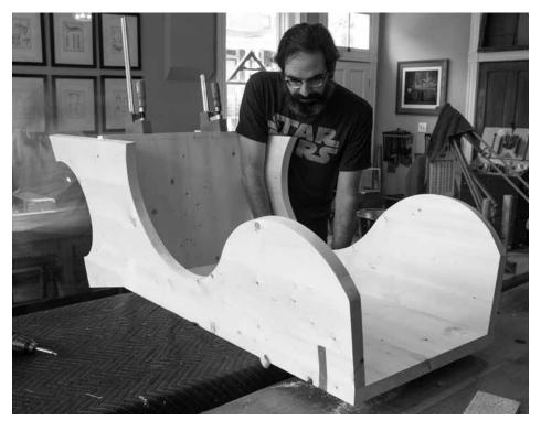
Scrub it now. Even if you use hide glue, which is easily cleaned with water, it's easier to remove any squeeze-out while the glue is wet. Use a toothbrush and warm water to get in the corners.
