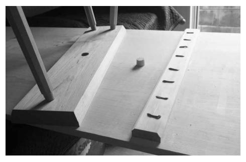
A peg & its hole. You can see there's a slight taper on the peg, which allows the top to slip on easily and slide into place.
