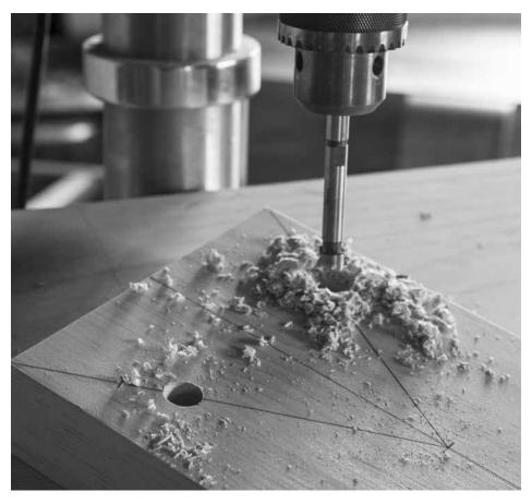
The good eyeball. When I drill holes in tops or seats, I line up the sightline, drill bit and center post of the drill press by eye. No fussing. I am usually off by a half-degree or less. In chairmaking, that's gold. Trust your eye.
