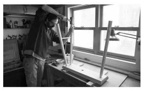
Drive it. Knock the legs into the plank until you hear a dull thud and the legs stop moving. If you hit the leg again after that point you risk splitting the top plank.
