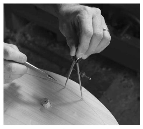
Walk this way. With dividers set to 2", you can easily lay out the four spindles with 4" between each mortise.
