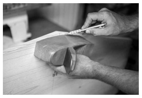
Two coffins. The boat shape of a coffin smoother is ideal for fairing the curves on the long edges of the bottom board.
