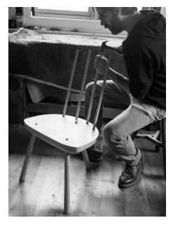
Driving spindles. Check the diameter of the spindles with care before driving them in. The tenoned section should be a cylinder, not a cone. Fat spindles can split the seat.
