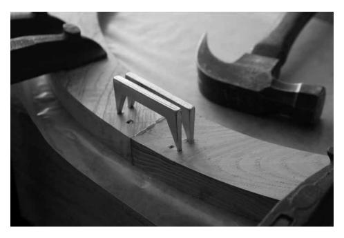
Pinch it good. Put glue on the ends of the hands and drive in the pinch dogs with a hammer to draw the bits together. Note the wax paper below the hands.
