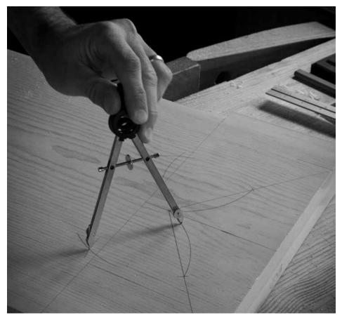
One setting. Here you can see the arc struck by the compass both above and below the baseline. That's all it takes to make a symmetrical S-curve.
