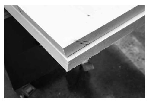
Angled edges. The angle doesn't look like much, but it dramatically changes the chair. No matter how you cut this angle, clean it up with a smoothing plane and confirm the angle is correct along its entire length.
