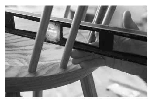
Three fingers. Here I've elevated the front legs of the chair until the seat is three fingers out of level. This tilt slides the body back toward the tall sticks and armbow.
