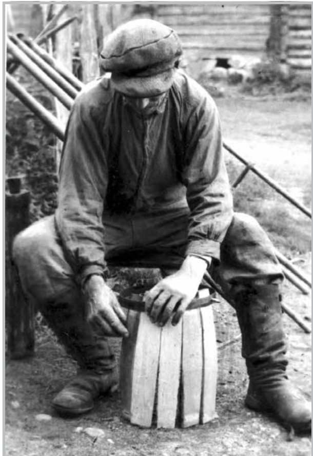
FIG. 113. Assembly of barrel, Avinurme, Vadi village, Photograph by author, 1947. Photo library 1089:74.
