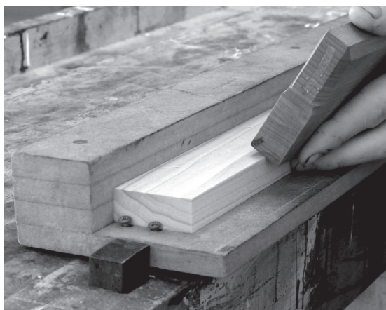
Fig. 4-9. Chamfering. Again, my fore and middle fingers are guiding the plane. When possible, I allow my trailing fingers to fall upon the workpiece. This will help gauge uniformity.
