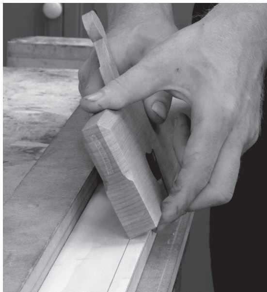
Fig. 4-3. Tilting a rabbet plane. My fore and middle finger, located in front of the cutting edge, help lead the plane down the length of the stock. Pressure is applied from the top of the plane toward your body, the sole and cutting edge. Do not apply this force away from your body against the side of the plane. This second method may result in the iron's side scraping the far side of the gauge line and slightly widening the rabbet prior to starting.
