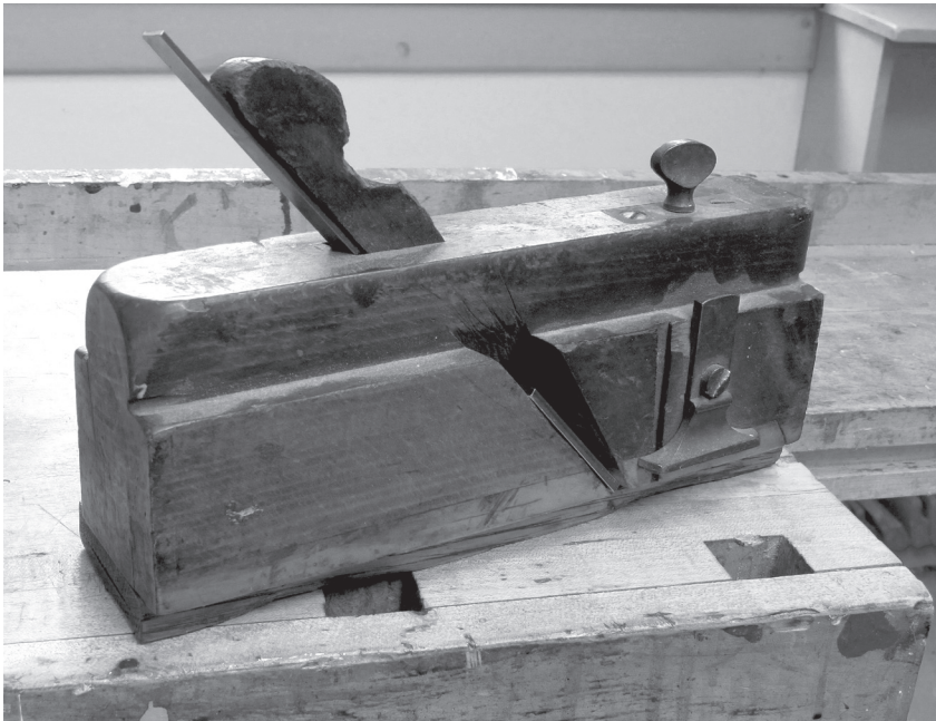
Fig. 4-1. Moving fillister. This moving fillister has a brass depth stop that is adjusted with the knob on top, along with an adjustable fence upon which this plane is standing. The iron is skewed across the sole and has a nicker ahead of the cutting edge for shearing wood fibers while working across the grain.
