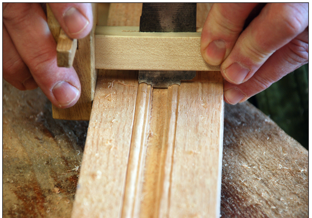
Fig. 4.35 This scratch stock uses a marking-gauge type format; it's cutting both sides of the plowed groove at the same time. Sometimes you need to lean this way or that, depending on how the cutter fits into the staff.
