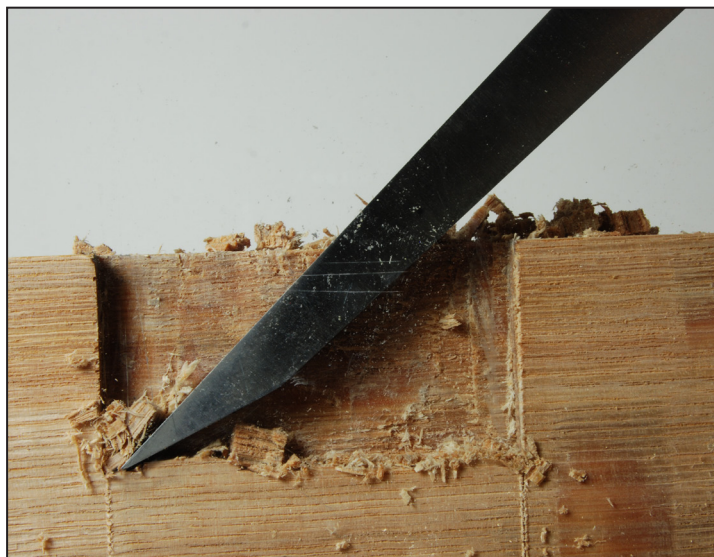
Fig. 4.15 This photo and previous one were shot between a piece of oak and a pane of plate glass. This allows a cross-section view of a chisel cutting a mortise. This experimentation was quite helpful in understanding what goes on during the mortising process. Thanks to Roy Underhill for teaching us this technique.
