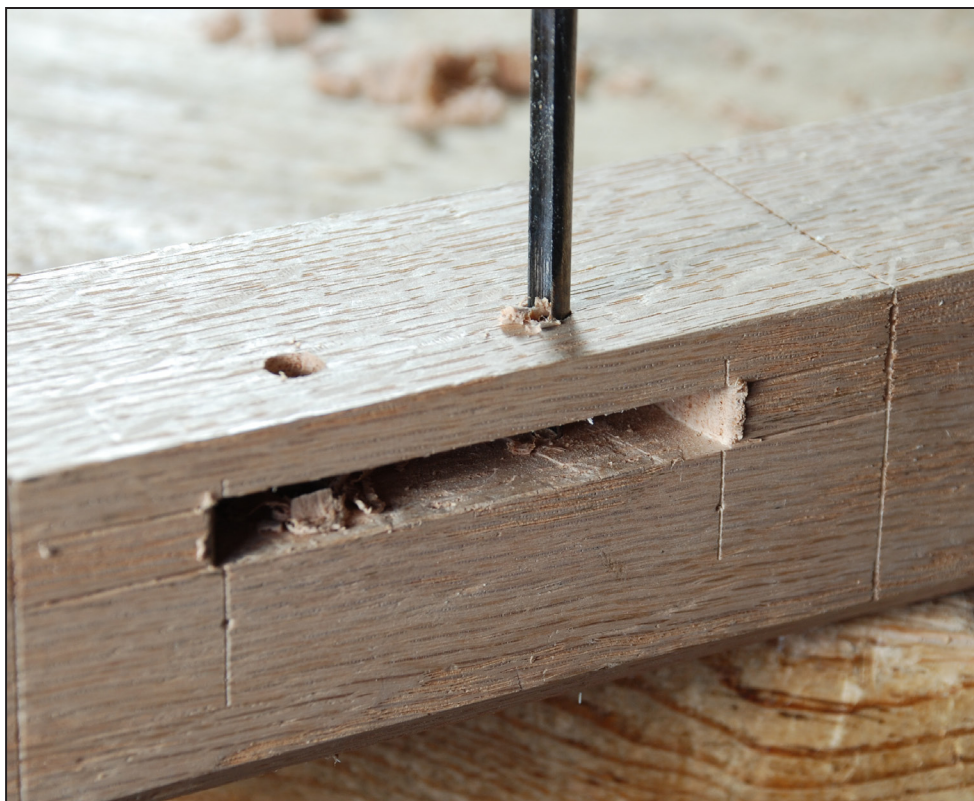
Fig. 4.20 If the holes are too close to the ends of the mortise, you might blow out the tenon's edge later when pinning the joint. Once you're finished boring the holes, you might go in the mortise with a paring chisel to clean up the interior surfaces.
