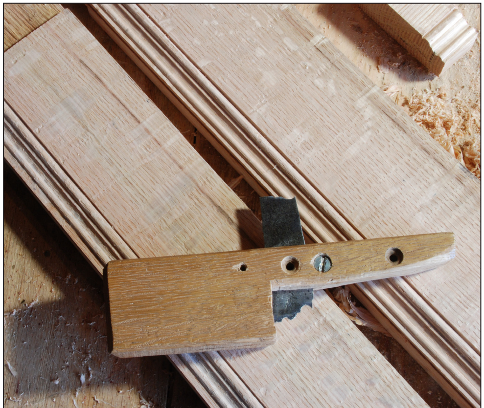
Fig. 4.28 The most common form of scratch stock, this time it's made from an off-cut of riven oak. You can cut a shape on each end of the blade and then switch it around for a different moulding. Make these as you need them. The price is right, as is its effectiveness and ease of use.
