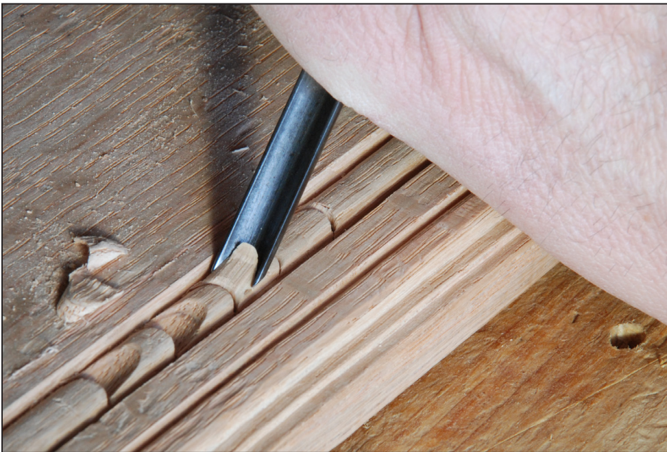
Fig. 4.31 Here is the chip coming up as the gouge meets the first incised vertical cut. Learn this, and any blank piece of oak becomes something more....
