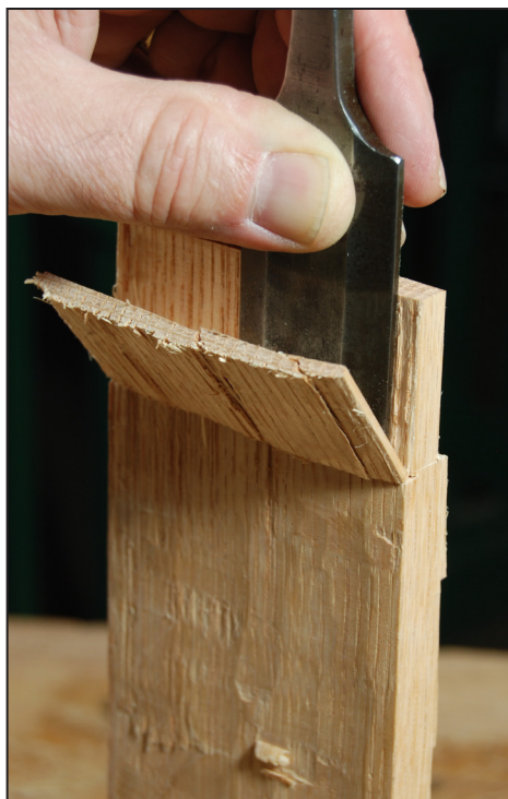
Fig. 4.42 Your fingers hit the rail's end grain to stop the motion of the chisel. That way, you don't drive the chisel into the shoulder.
