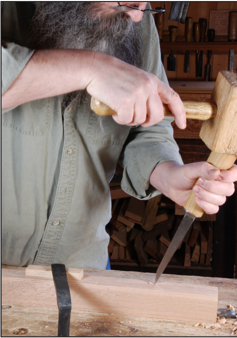
Fig. 4.11 Coming at the mortise first this way, then that requires some shift in posture. Experiment with different methods to see what feels best. The idea is to get the mortise chopped quickly and easily.
