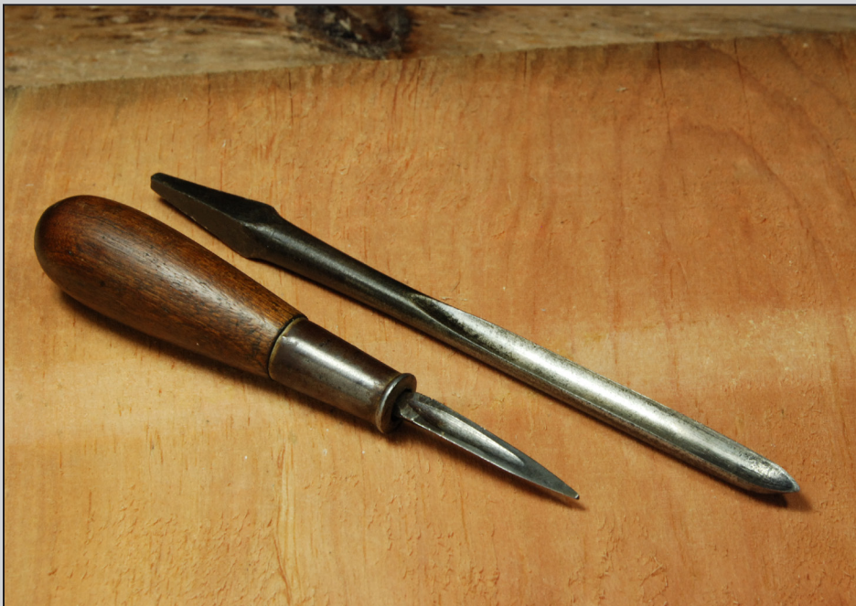
Fig. 4.17 All you need to sharpen the piercer bit is a triangular burnisher, like the one shown here mounted in a turned handle. It is hard enough to turn a hook on the piercer's steel.
