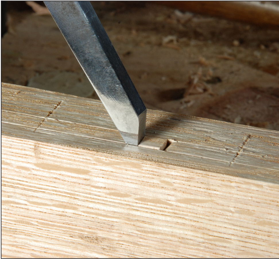
Fig. 4.9 This is the first pair of blows with the mortise chisel. Note the chisel's bevel is just about plumb.
