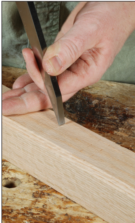
Fig. 4.5 Now move the chisel over one chisel-width. And lean on it. Now your setting is marked on the timber, and you just need to set the mortise gauge according to the chisel marks.
