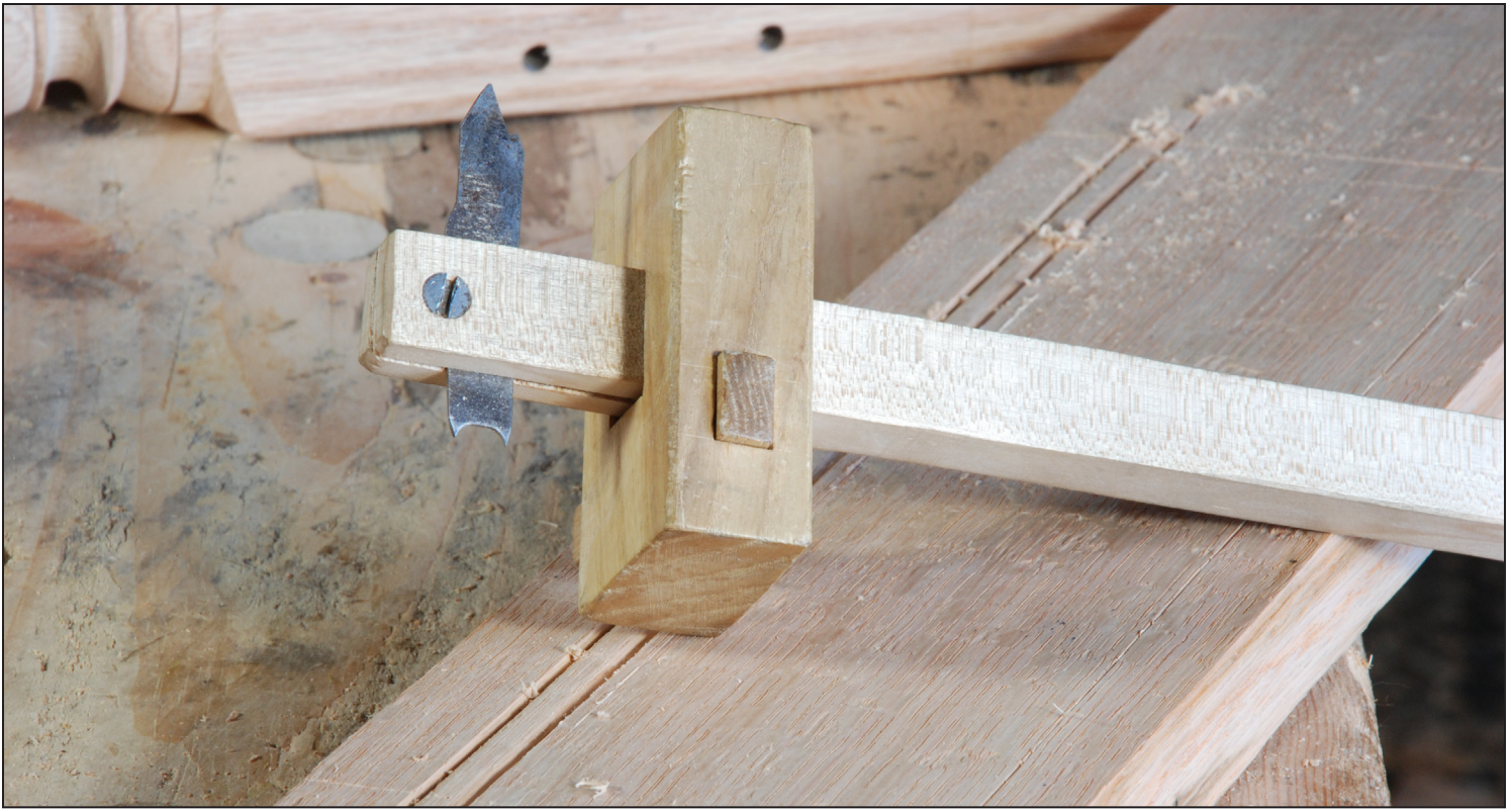
Fig. 4.27 Make your scratch stocks from hard woods. This one is has a maple staff, an ash fence/head and a hickory wedge. A mixed bag to be sure, but it's worth keeping a selection of dry, straight-grained hardwoods around for just this sort of project.
