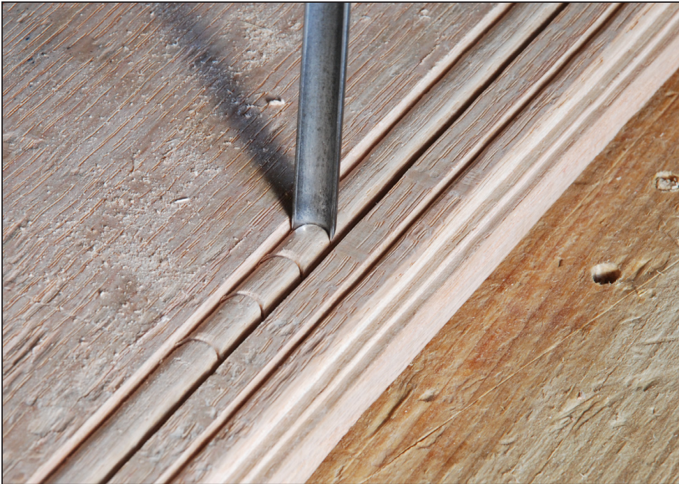
Fig. 4.30 Carving is a study by itself, but this is the simplest shape to get the hang of – one tool, two moves. This form of carved work is utilized in most 17th-century carved oak.
