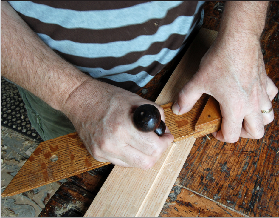
Fig. 4.36 The shop-made miter square is taken right from Moxon's plate of joiners' tools. Sometimes we've seen this zig-zag motif done freehand, but it only takes a moment to lay it out.
