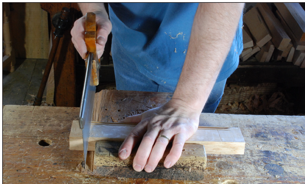
Fig. 4.39 The undercut shoulder is one of the critical elements in this joinery. It saves time when fitting the joints because only the scribed shoulder hits the mortised piece. It is just a slight tilt of the saw.
