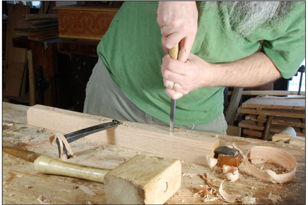
Fig. 4.12 The amount of work that is split between hand pressure and mallet-driven will vary. Moisture content plays a role in this, drier stock is less forgiving with hand pressure. But either way, oak will convince you to use your whole body.
