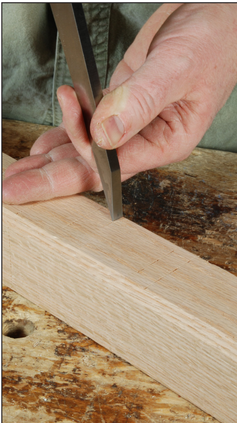
Fig. 4.4 This is a technique that if we heard it somewhere, we have forgotten where. It works very well. No ruler, no fiddling with the gauge up against the chisel's sharp edge. Mark the timber with the chisel, then put the chisel down. Very safe, and simple.
