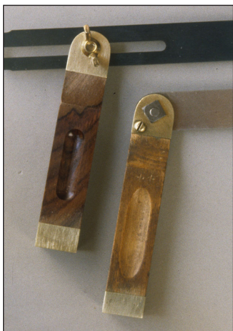
Fig. 4.7 Here is an adjustable bevel, and the modified one Alexander turned into a fixed bevel. If you are using one flare angle regularly, this is the way to go. It's easy enough to come up with an extra adjustable bevel.
