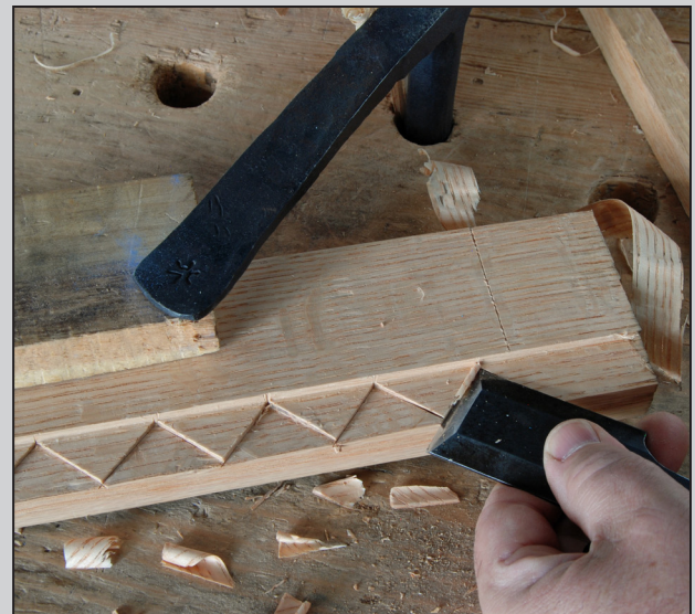
Fig. 4.38 Use a nice sharp chisel and some raking light for these cuts. In a sense, this is like the gouge-cut carvings done on the scratched mouldings earlier. Make a vertical incised cut, then remove a chip down to that cut. Then light and shadow.
