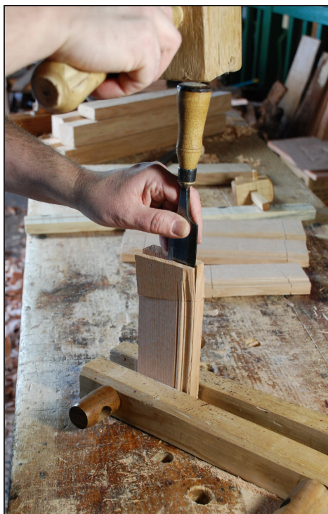
Fig. 4.41 This step is more akin to timber framing than modern furniture making. Its success comes from the intimacy with which you know the wood when you've worked it all the way from the log. Straight-grained oak is the key.
