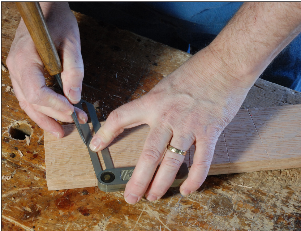
Fig. 4.26 Adjustable bevels are often small enough that you can grip the handle and blade in one hand, pinching the whole tool against the rail's top edge. However you hold the tool, be sure it has not lost its setting, and keep it steady while scribing the shoulders.
