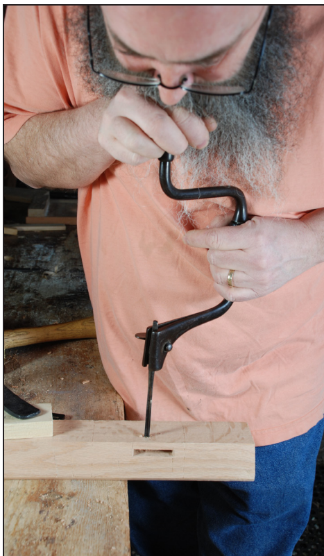
Fig. 4.19 Boring with this type of bit requires some downward pressure because the piercer bit doesn't draw itself in. You can lean with your shoulder, forehead or chin. Try different approaches and use one that works.
