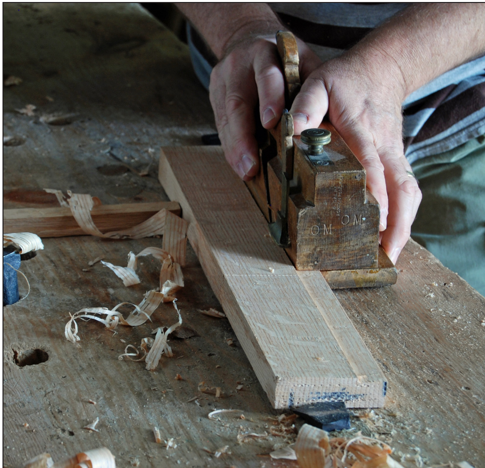
Fig. 4.33 This is a moving fillister plane, which is basically a rabbet plane with a movable fence attached to its sole. The best ones have skewed irons. This one has a depth stop that you needn't be concerned with for this sort of work.
