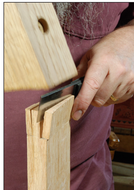
Fig. 4.43 The hacking knife/cleaver spans the full width of the tenon, so it's one position and one whack.
