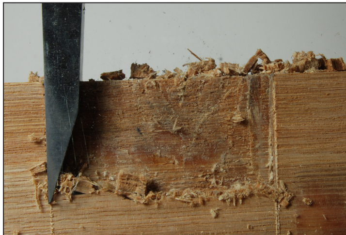
Fig. 4.14 Here, the mortise's bottom is ragged, but it doesn't need to be much cleaner than this. The tenon will never reach that far.
