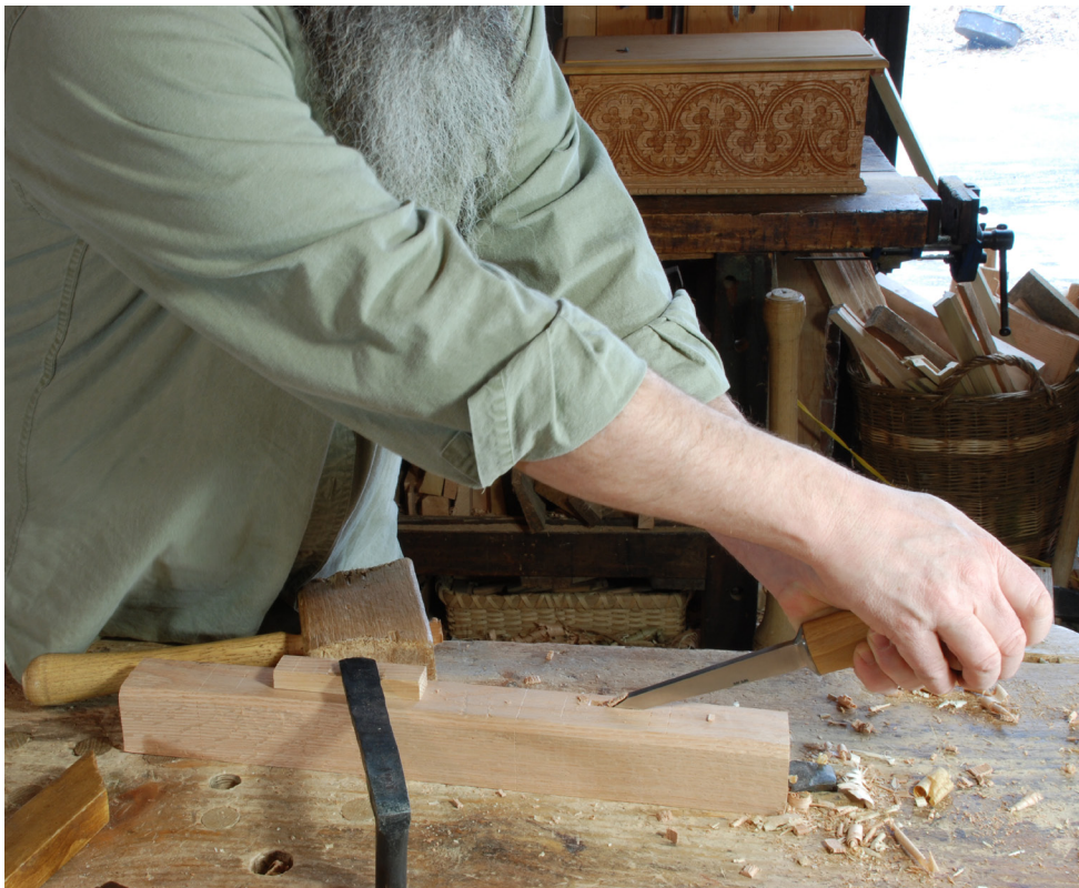
Fig. 4.13 A nice stout mortise chisel is essential when prying the material out of the mortise.
