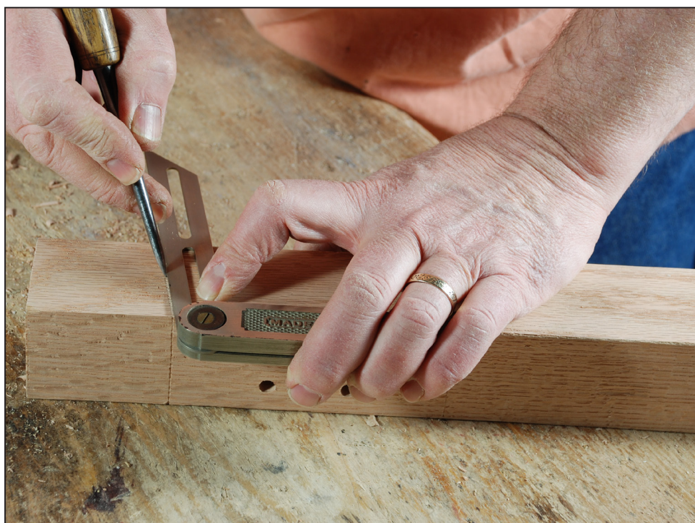
Fig. 4.8 Marking this angle is the same as any layout, a couple of light passes will carefully scribe a line on the stile. We have often joked that this step requires two consecutive thoughts. It might be three.
