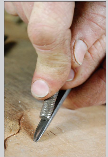
Fig. 4.18 This version of sharpening a piercer is not all that different from the previous idea. Blacksmith Mark Atchison pushes the file/burnisher down along the inside of the piercer's flute. This creates a hook, much like on a cabinet scraper.
