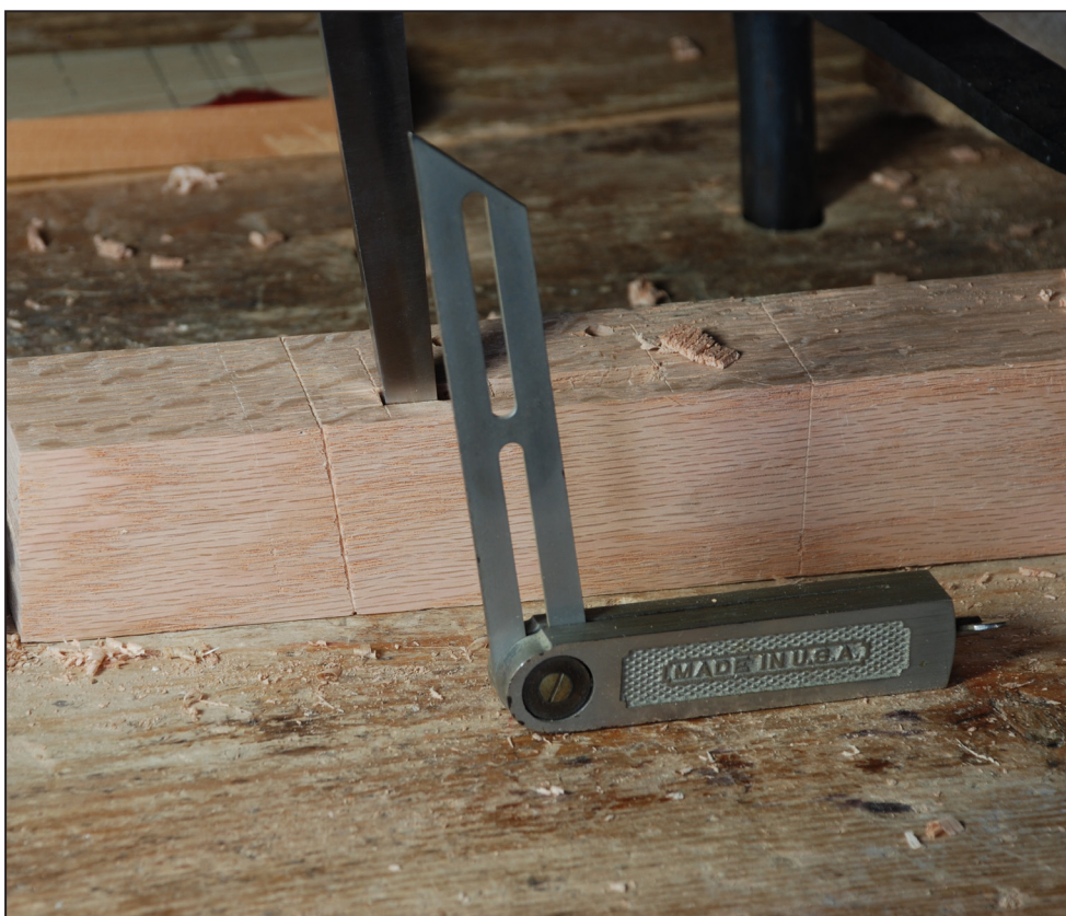
Fig. 4.21 On your first few stools, it's helpful to align the adjustable bevel to sight against. Over time, you will get the feel for the angle and be able to chop these mortises without it.
