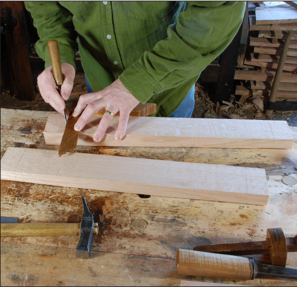
Fig. 4.23 17th-century joinery tolerates a great deal of variety in its textures and workmanship. But the tenon shoulders' layout is one of the places where you need to be absolutely accurate. Carefully scribe these lines. If you use a wooden square, check its blade from time to time to be certain that it's not deformed from use.
