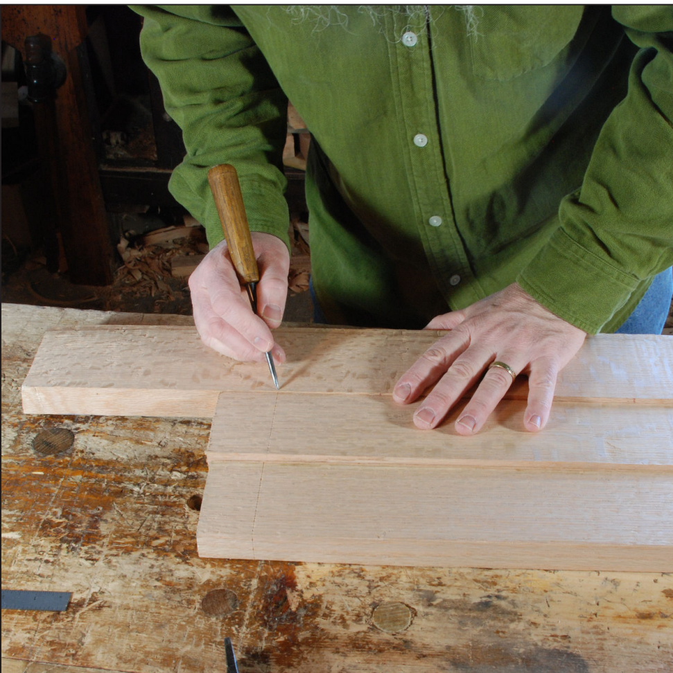
Fig. 4.24 Scribing this layout from one rail to another is the same concept as laying out the stiles' joinery. This method is favored over using a ruler to mark each rail. You need a ruler in your toolkit, but you don't want to use it too much.
