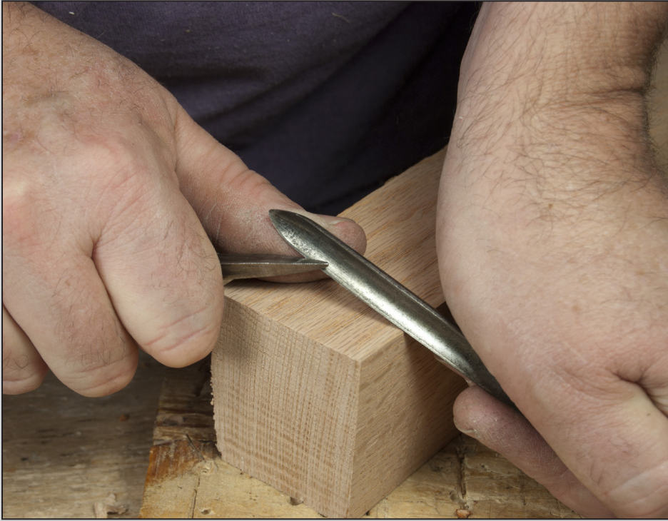
Fig. 4.16 Lay the burnisher flat on the cutting face. You only need to work near the bit's end. It's not necessary to sharpen all the way up the flute. We usually only sharpen one side, but piercers are made to bore holes both clockwise and counterclockwise. Sharpen the side or sides according to how you will use the tool. Do not touch the outside of the piercer.
