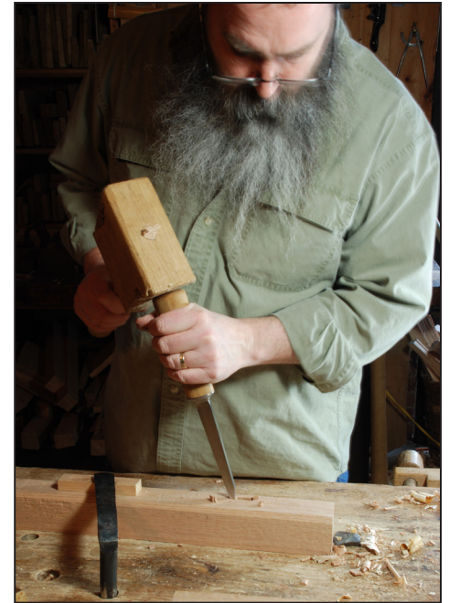
Fig. 4.10 Here, the stile is held in place by a holdfast, with a scrap of pine between the holdfast's "pad" and the stile. This prevents bruising the stock.
