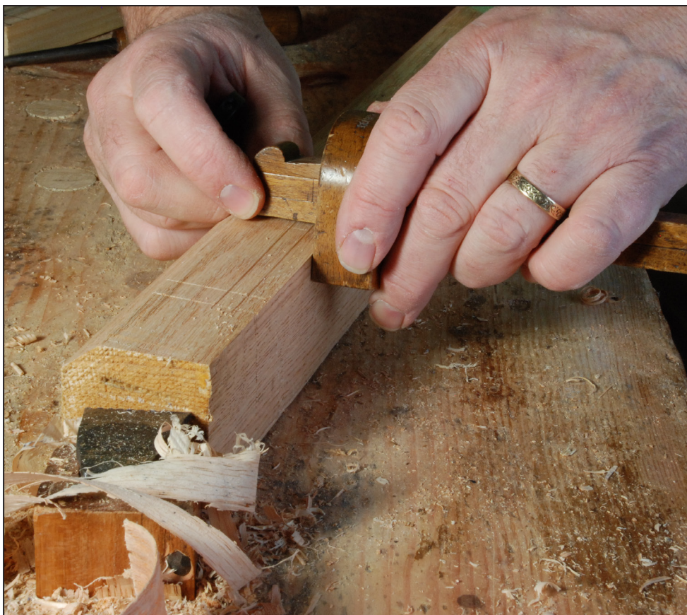
Fig. 4.6 Using both hands on a marking or mortise gauge might seem like overkill, but the oak is very fibrous, and when it's green it can catch the gauge's pins. The result can be irregular and it's hard to re-mark a line once it goes astray. Extend the marking lines beyond the top and bottom of the mortise, this way you can check the spacing of the joint if you find you need to reset your gauge – if, for instance, it falls on the floor.
