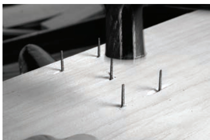
I have a steel plate behind the head of this nail as I clinch it. Here is the nail tip right before the first strike.
