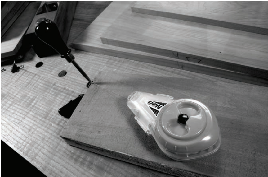
Thomas used a brad awl to secure one end of the chalk line. A nail or a helper monkey are other good options (speaking as a former helper monkey).
