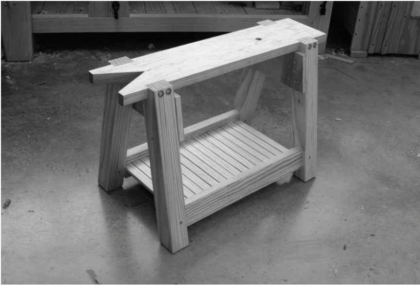
Shown is one common pattern for a sawbench. Note the flat top that is about 7" wide and the height of the bench, which is just below the worker's knee.
