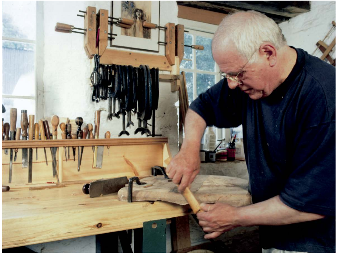
At work on the underside of a chair seat with a wooden-bodied spokeshave.
