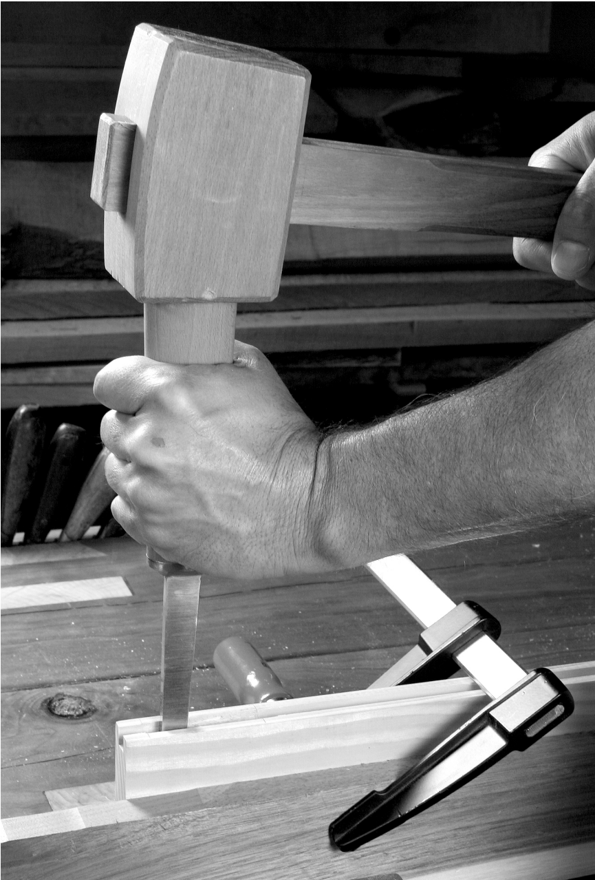
Photo 13 Chopping the mortice. The true mortice chisel is shown and the workpiece is cramped to a mortising block which is held in a bench vice
