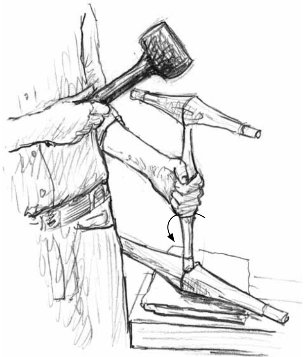
FIG. 21.3 How to twist the center stretcher as you seat the tenon.
