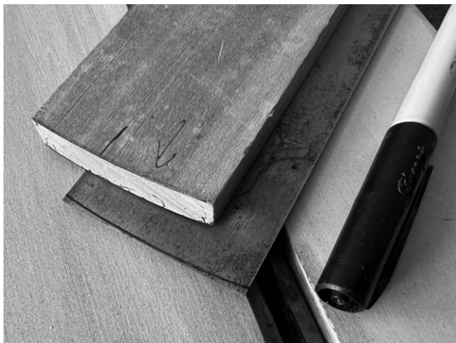
Fig. 33. A wooden template helps you reestablish the curved edge after dozens of honings and polishings.
