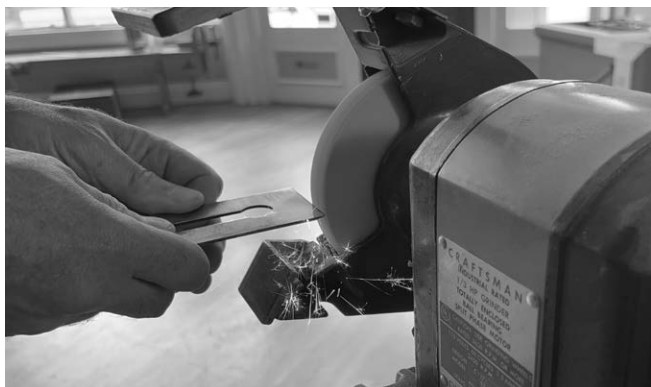
Fig. 31. Removing the tip of the blade prevents it from heating up. And it gives you a target to shoot for.
