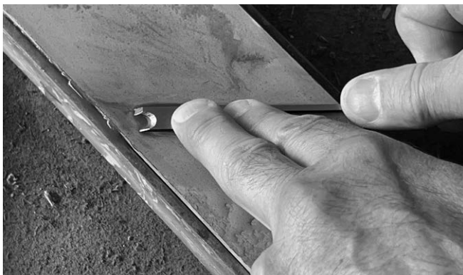
Fig. 58. Stoning the flat face of the iron will keep the edge fresh for a long while.
