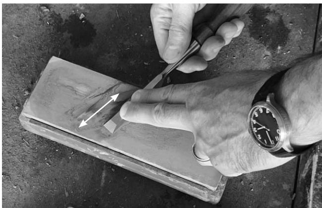
Fig. 52. Though polishing the flat face can be done in 5 seconds or so, I usually spend some extra time in polishing the flat face to keep it clean and polished.
