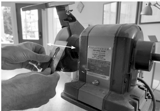
Fig. 27. Once the blade contacts the wheel, slide the blade left and right on the wheel, grinding its entire edge.
