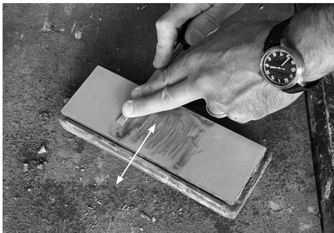
Fig. 16. This motion prevents the flat face of the narrow tool from becoming rounded.
