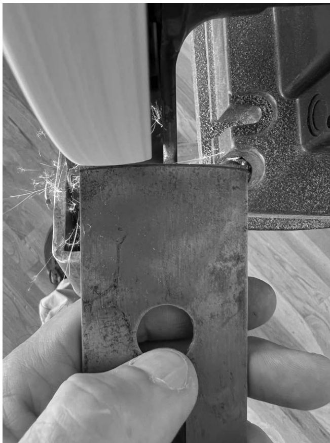
Fig. 34. Create the blade's new shape by blunting the tip of the tool. Then grind the bevel to match that new shape.
