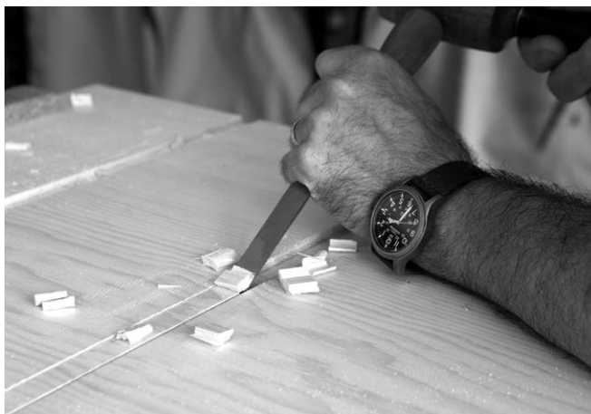
Fig. 5. A bevel-down chisel work finishes the waste removal.
