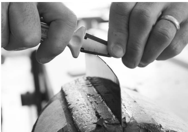
Fig. 63. Tilt the burnisher the other way to turn a hook on the adjacent edge.
