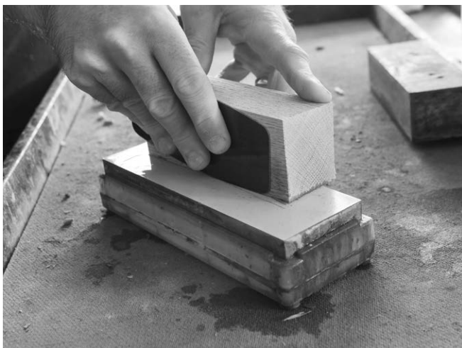
Fig. 61. Stone the long edges of the scraper using a block of wood as a guide.
