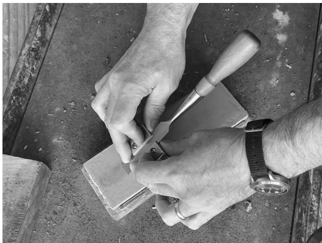
Fig. 40. In general, my hands only gently touch the guide. Most of my hand pressure is on the blade.
