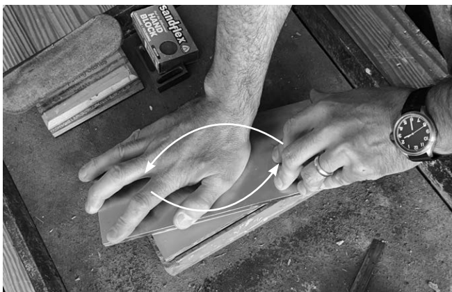
Fig. 56. This motion is vaguely elliptical to spread the diamond plate's cutting action out on the sharpening stone.
