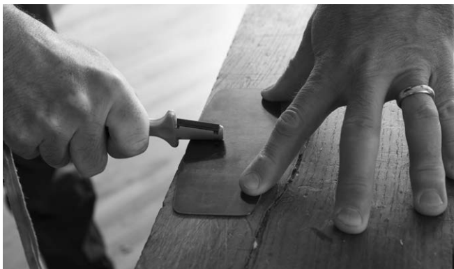
Fig. 60. Remove any burr or old hook using the burnish as shown.
