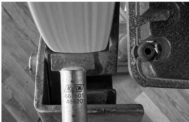
Fig. 23. The diamond dressing wheel requires a light touch to leave a smooth surface behind.
