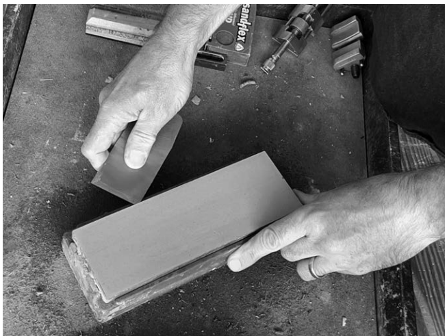
Fig. 43. The unused edges of a sharpening stone are a great place to do the dirty work of rounding the corners of the iron.
