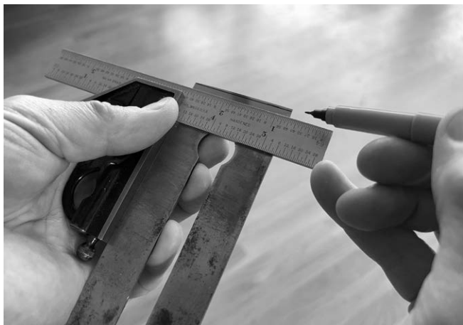
Fig. 30. A marker line tells you when to stop grinding and keeps the edge 90° to the blade's sides.
