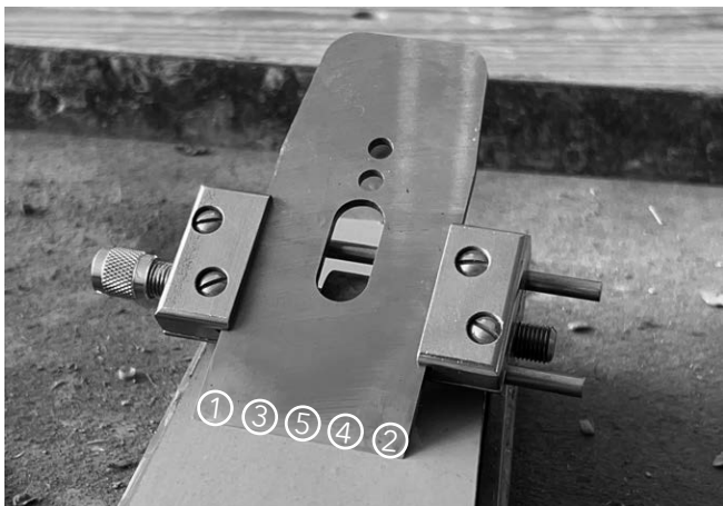
Fig. 44. For most plane irons, I divide them into five stations. Narrow blades (such as block plane blades) have three stations.
