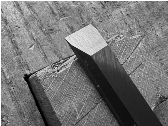
Fig. 15. The least you should ask from a tool manufacturer is a ground bevel that is the correct angle and straight across.
