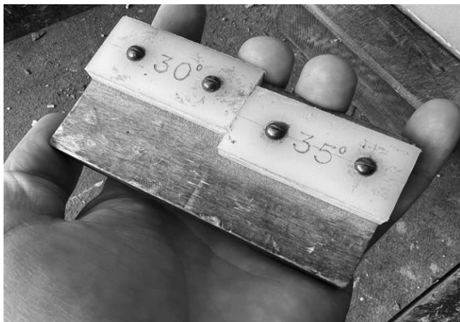
Fig. 38. The plastic block sets the blade's location in the jig.
