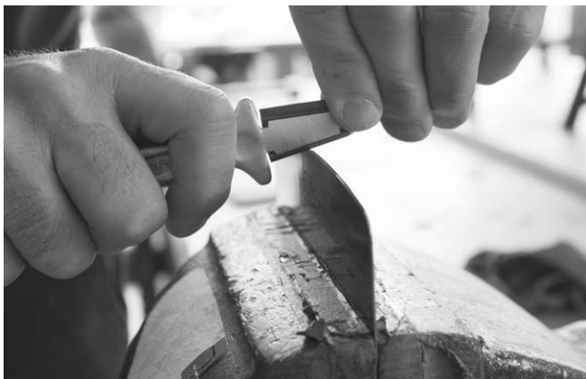
Fig. 62. Tilt the burnisher and turn a hook on one edge.
