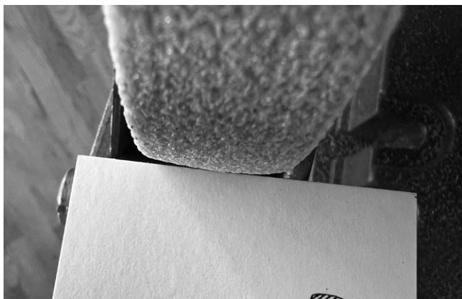
Fig. 24. A slightly convex wheel gives you enormous control over the shape of the tool's edge.
