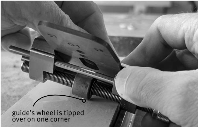
Fig. 47. Putting pressure on the corner should tip the guide on its wheel. Unfortunately, some guides have really wide wheels. Avoid these.
