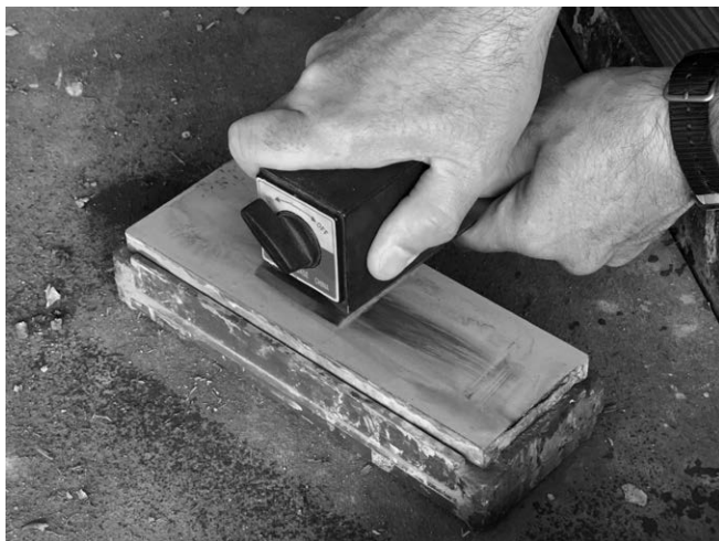
Fig. 19. A magnetic base helps you apply downward pressure right where it is needed.
