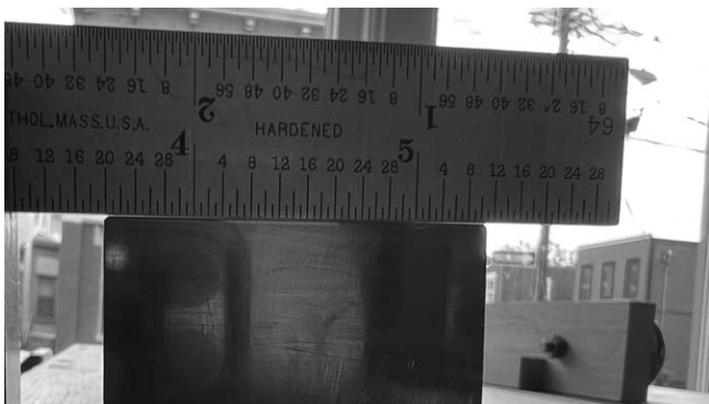
Fig. 45. The curve on a No. 3 smoothing plane. In short order you will get a feel for how much curve each tool requires.
