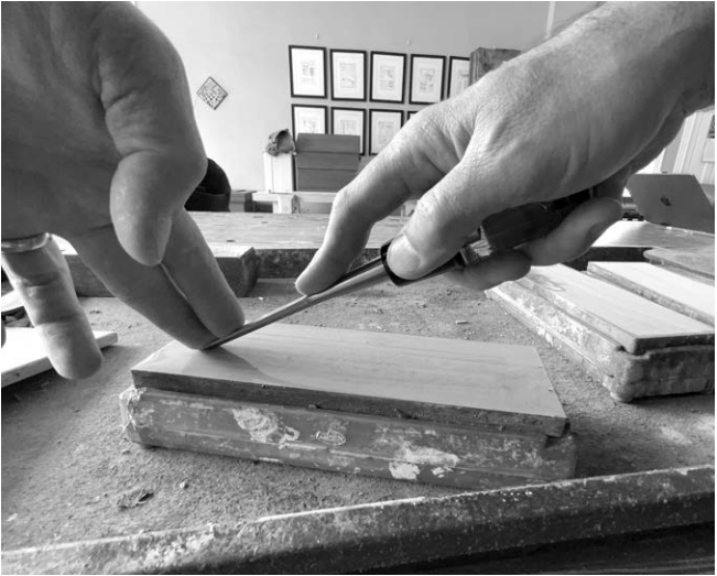
Fig. 42. Press the bevel flat to the stone. Raise the handle of the tool 1/8" (no more). Pull the tool backward.
