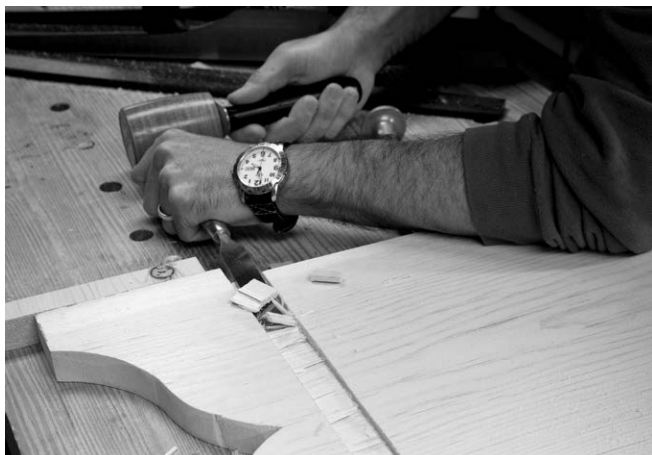
Fig. 4. A bevel-up chisel starts the waste removal in a dado joint.
