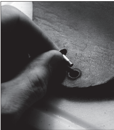
Fig. 6.11 Insert the rivet. Put the rivet through the holes. The flat face of the rivet should be on the top surface of the seat.
