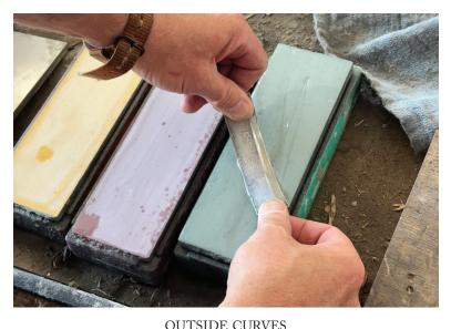
Polish the outside curve of the travisher on a flat polishing stone (shown is an #8,000-grit stone).
