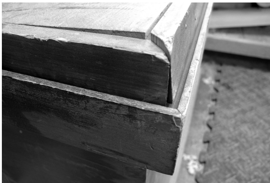
Miters & mayhem. The flat-panel lid warped and shrank. The miters lost their hold. This lid is a mess.
