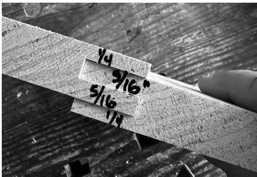
Groove-in-groove. The lid (left part) nests into the rails and stiles like this. The construction makes the lid strong across its entire surface.
