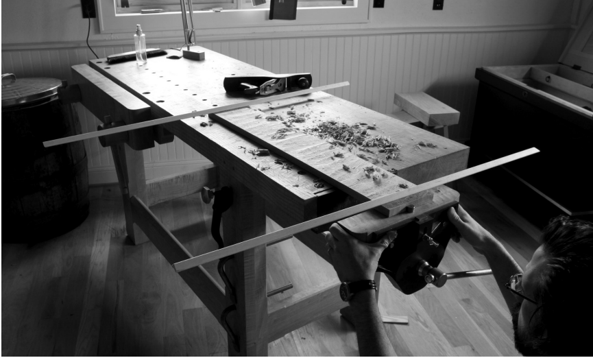
Jack's buddy. Winding sticks help you gauge your progress. You should make your own, which is discussed in the section on marking and measuring tools.
