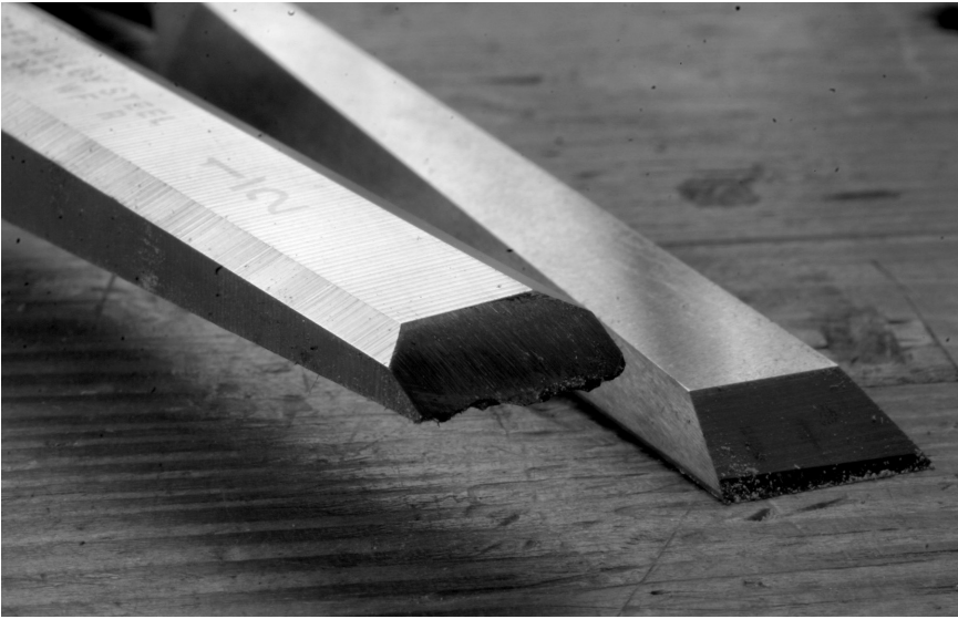
Bad bevels. Here you can see the difference between a poor modern tool with its buck-tooth side bevels – called “lands” – and a proper tool for woodworking.
