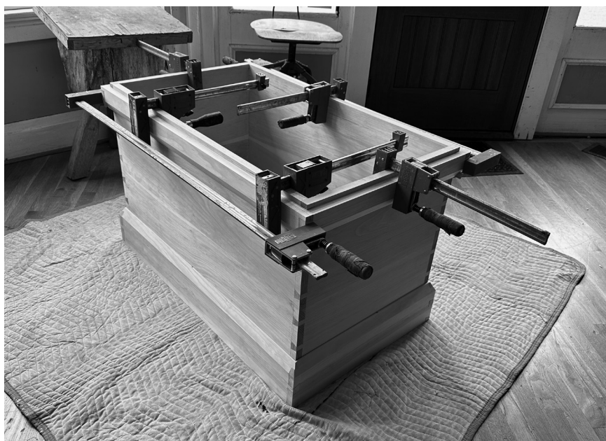
Layers of clamps. The long clamps press the dovetails together. The short clamps press the skirts to the shell. Both are important.
