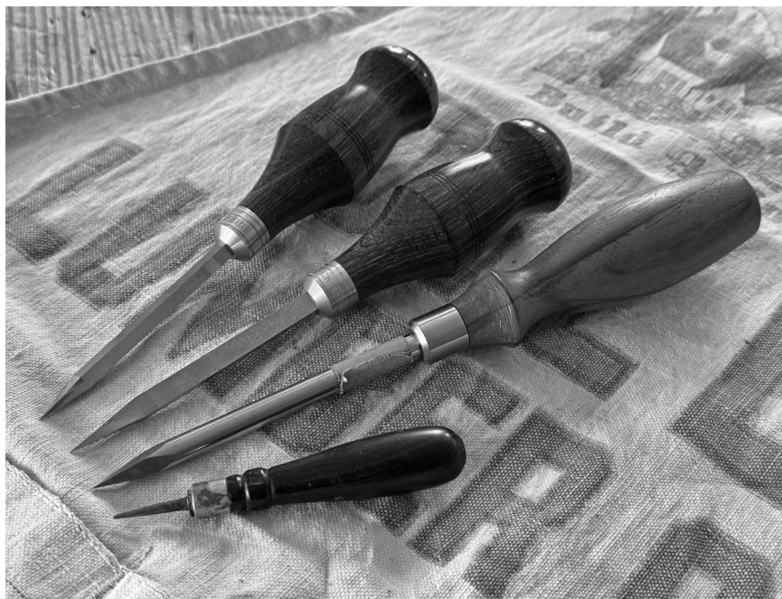
All about awls. A birdcage awl (the top three tools) is the most useful awl for making holes.
