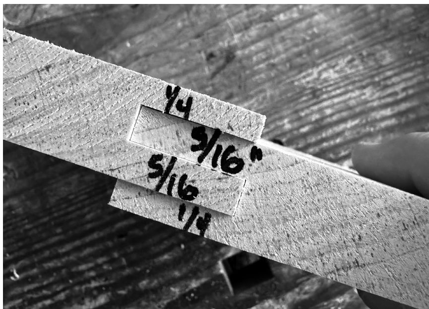
Inside the lid. When the panel, rails and stiles are fit, this is how they nest together to create the lid's raised center panel.
