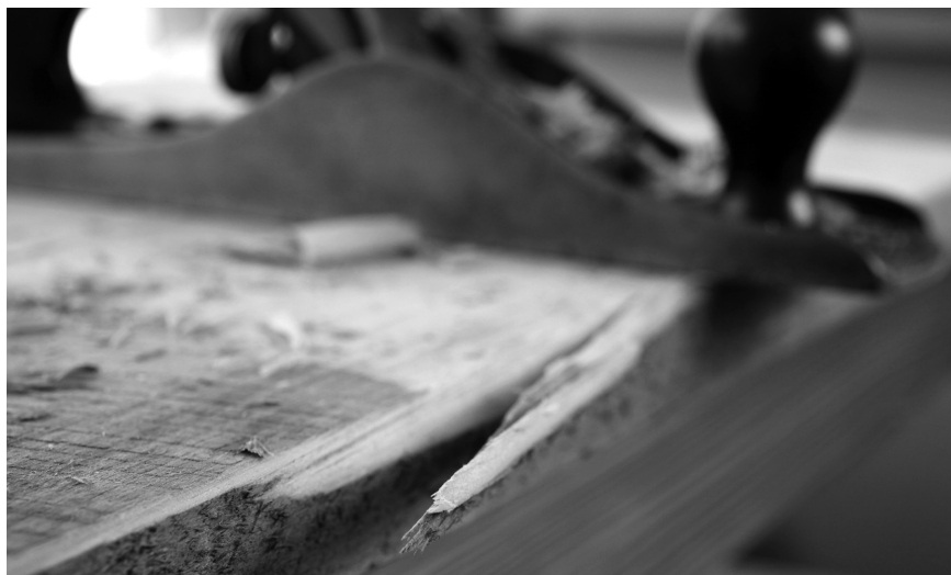
The spelch stopper. A bigger chamfer on the edge of this board would have helped prevent the edge from splitting off when I traversed it.
