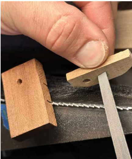
Reorient your file parallel with the bevel guide. The rake and slope orientation are the same.
