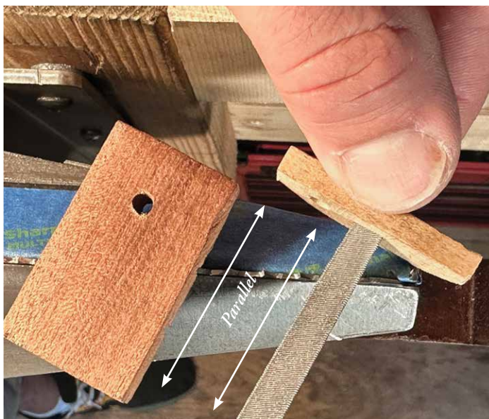
Bevel: 25°. Keep your file parallel with the long edge of the guide. Sharpening beveled teeth is a two-step process. First, file one set of bevels in one direction, then rotate your guide and file the other set of bevels in the opposite direction. I like to start filing toward the heel, but it doesn't make a difference which you do first.
