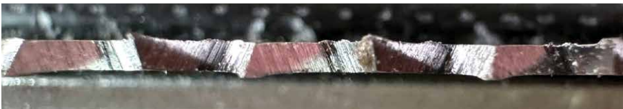
These teeth have the right amount of set for a crosscut saw. It can be hard to see, so rely on your test cut at the end to confirm your results.
