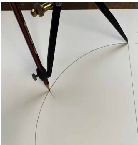
Without adjusting the dividers, step off marks around the circumference by walking the points from mark to mark.
