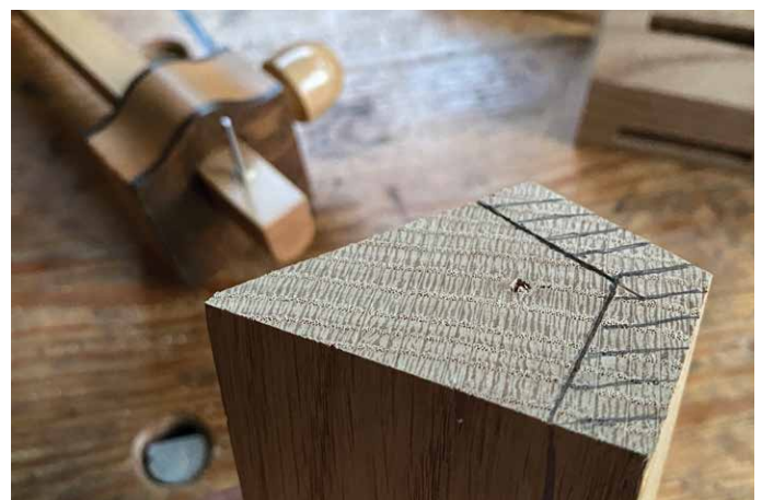
Gauge a line from the internal faces on the bottom of the leg for tapering.
