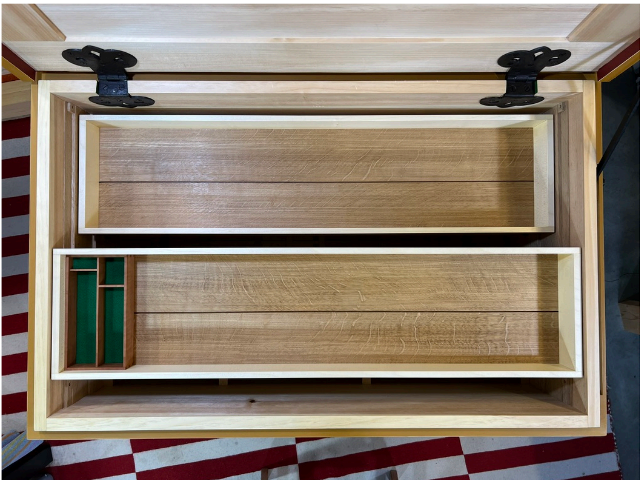
Plenty of margin for no overlap between the sliding tills.
