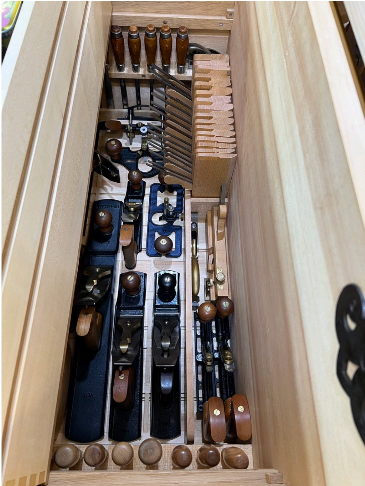
The rear of the central well and the molding plane corral. Why do I have two #5 planes? The Stanley is set up as a true jack and the Lie-Nielsen as a short jointer. They may look alike but do different jobs.
