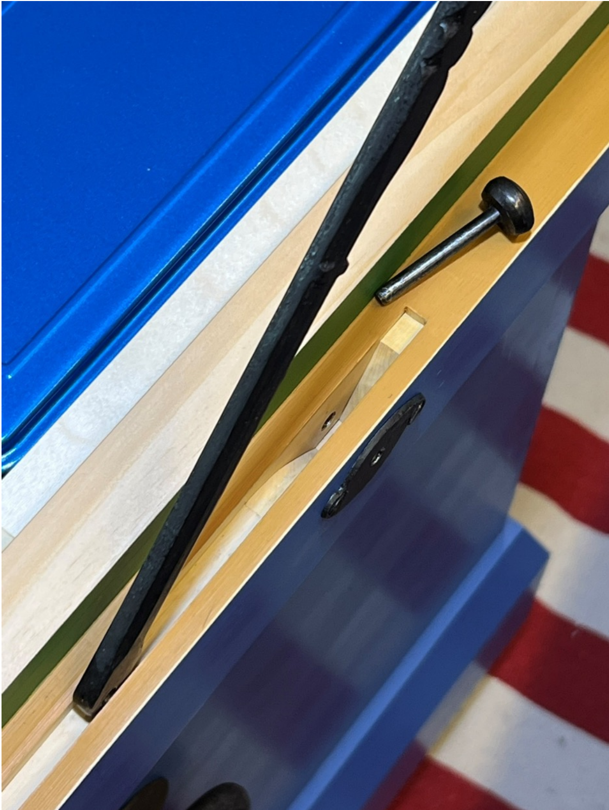
The locking end of the lid stay with stay arm, mortise, strike plate and loose pin.
