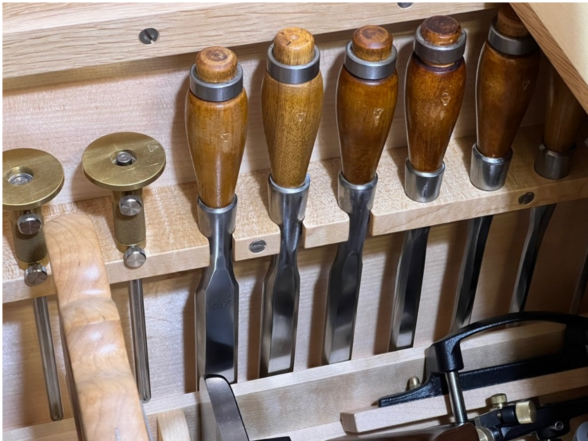
Part of the left-hand side tool rack: the handles clear the runner and till bottom, and the edges are protected behind the guard rail.
