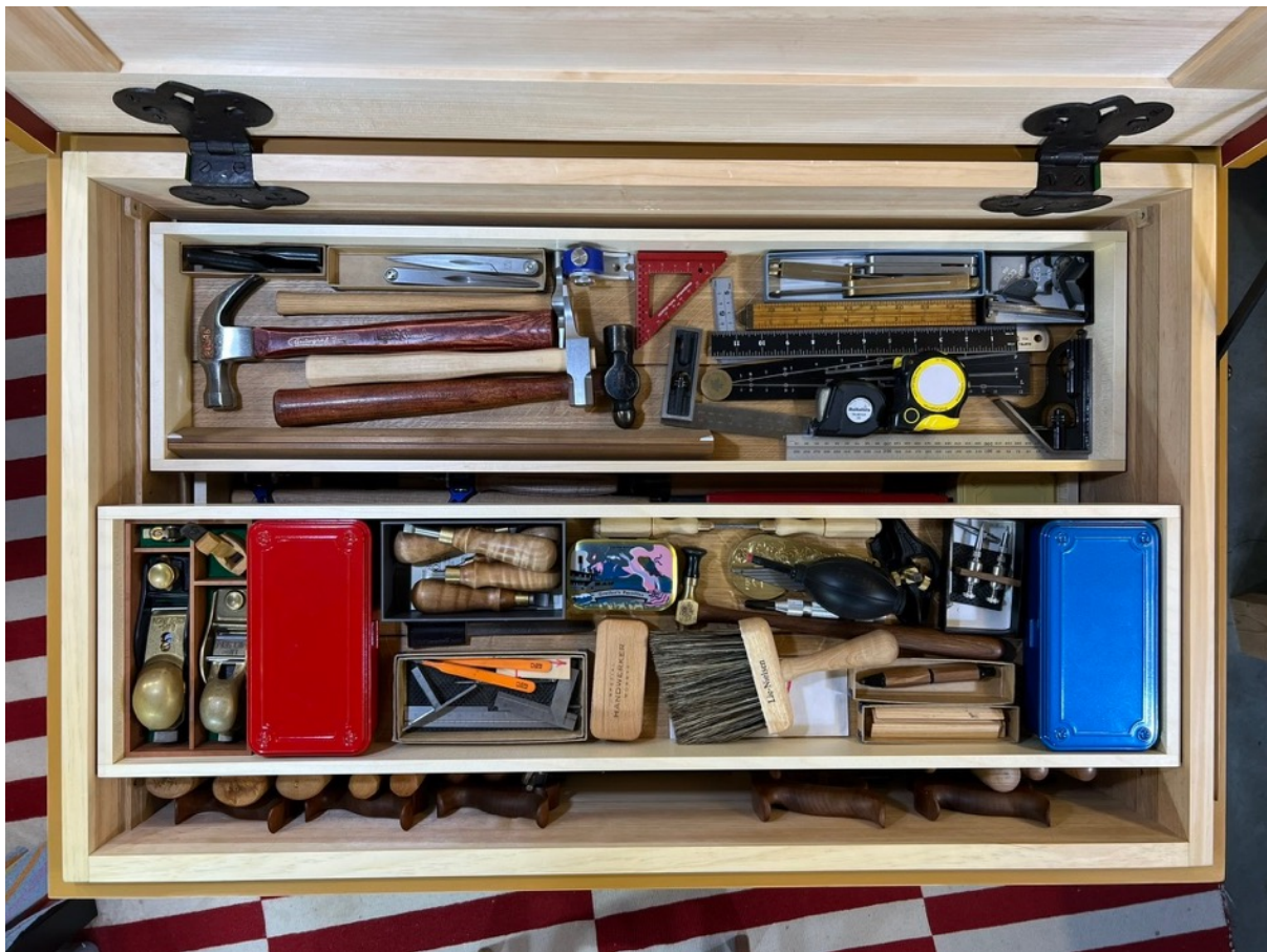
Middle till with hammers and measuring tools.
