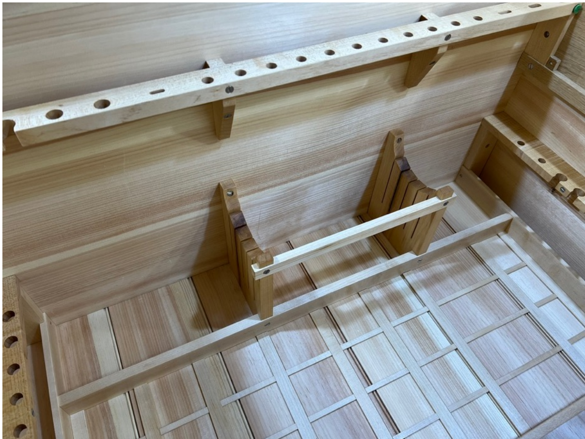
The finished saw till, with the uprights in line with two middle spacer blocks behind the front rack above. The top cross brace is much shorter than what's suggested in the literature, for a reason. Having it go all the way out to the side walls would not make the construction meaningfully stronger, but it would interfere with tool storage in the side racks.
