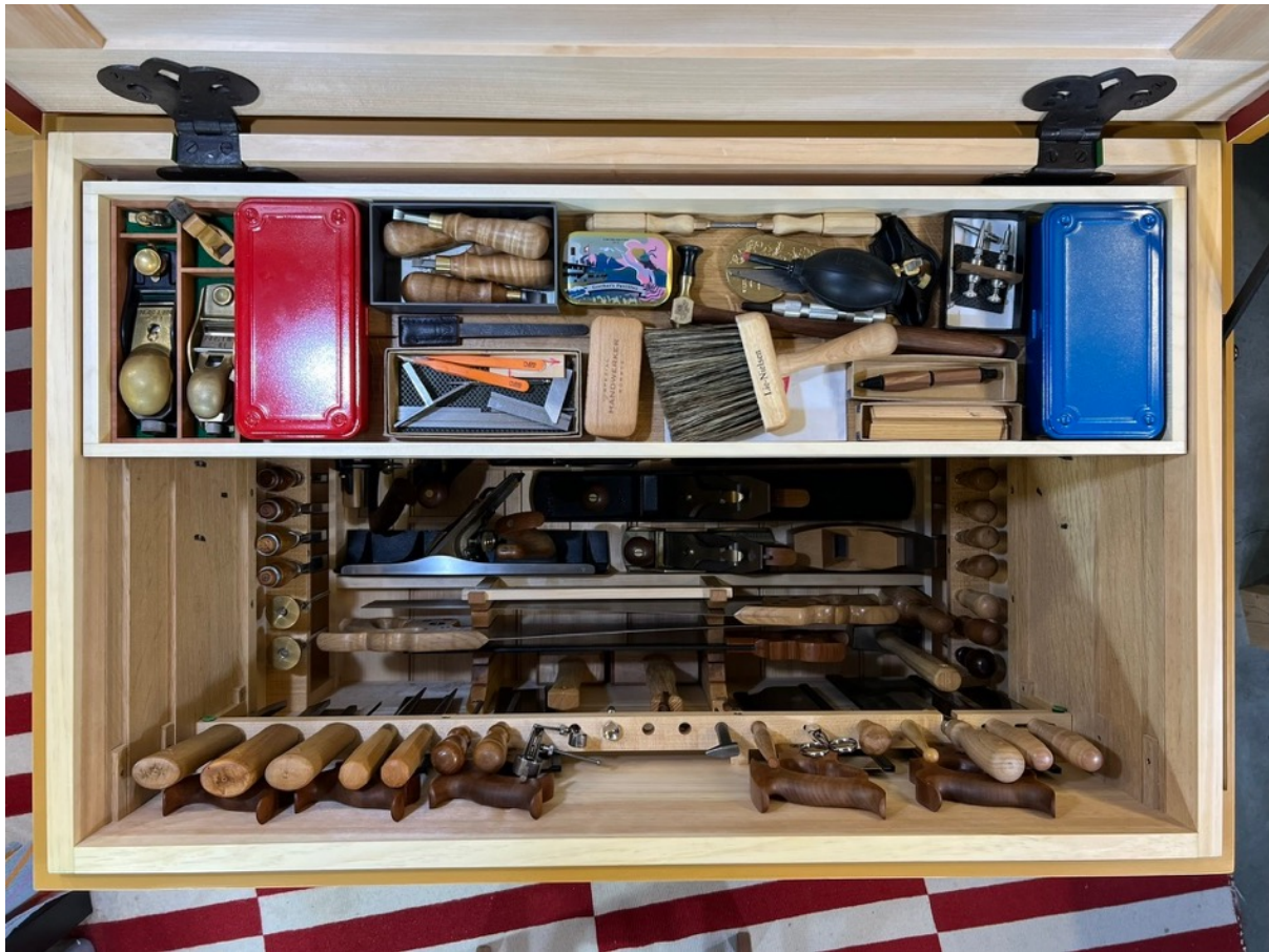
Top till with block planes, woobie box (red), favorite (my Vesper square and Blue Spruce forged marking knife!) or often used smaller tools and pencil box (blue)
