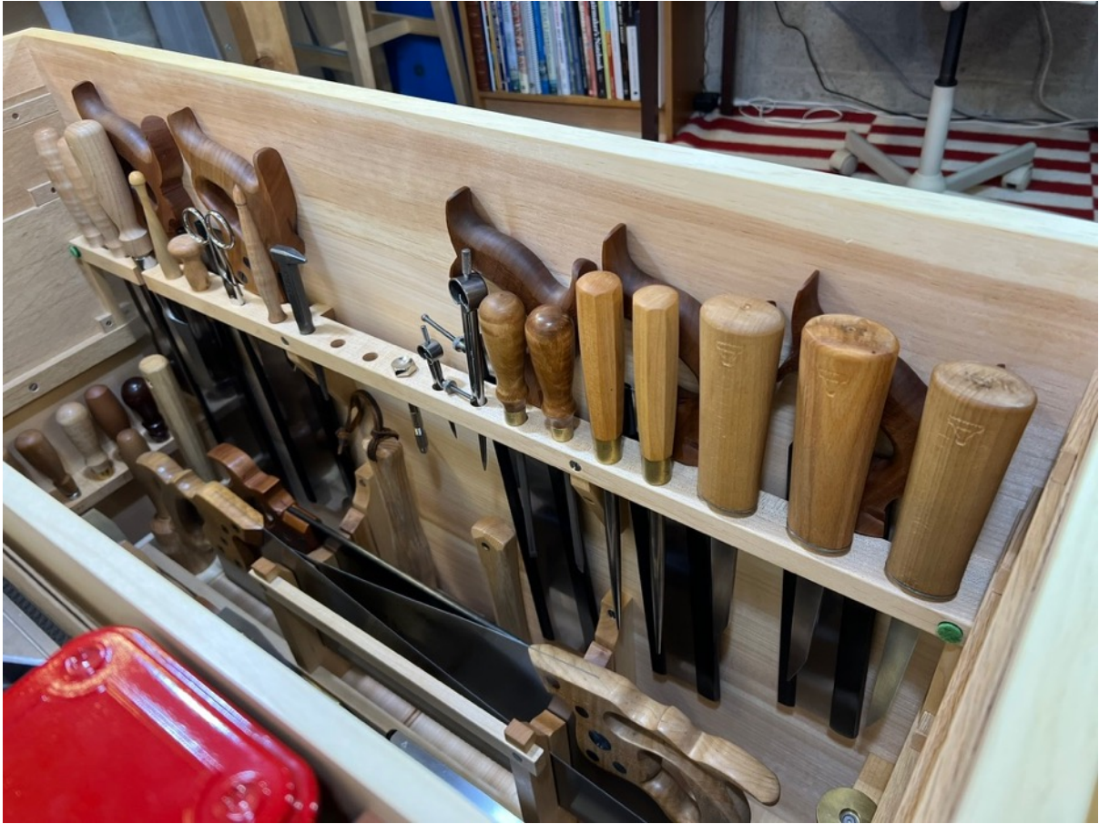
The front tool rack with backsaws hanging behind it.
