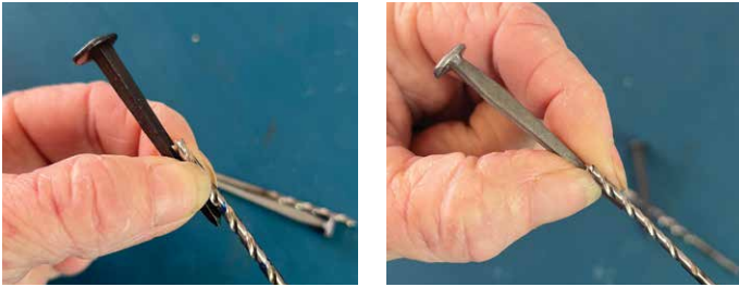
The 50mm Rivierre nails get a 1/8" pilot (and a 9/64" or 5/32" hole through the lip at both ends). The pilots for the 6d cut nails are 3/32".
