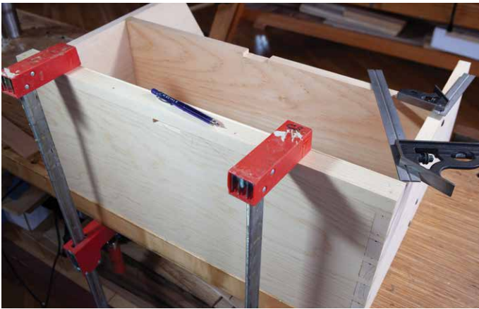
Clamp the lip securely to the carcass while also clamping the entire assembly securely to the bench – you want no movement.
