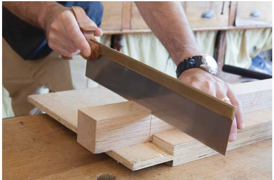
Figure 7.6. Broad shoulders. If you are going to rive the cheeks of your tenons, first saw the 1/8"-deep shoulders all around. Mark the depth of the shoulder to guide your sawing.
