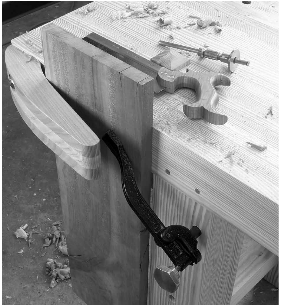
Figure 5.45. Good enough for dovetailing. A crochet and holdfast (or bar clamp) do a fine job of keeping the work in place for dovetailing.
