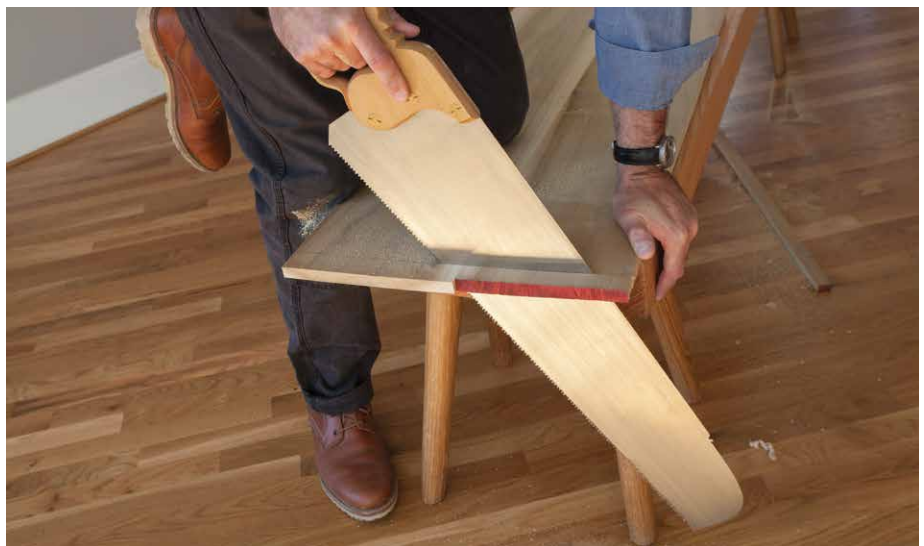
Figure 5.33. You won’t shave your legs. All eight legs are tucked under the shadow of the benchtop, so it’s difficult to nick them with your saw.
