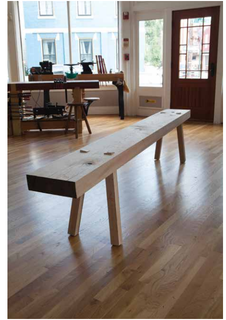
Figure 7.10. On your feet. Drive in all four legs, turn the bench over and check your work. If your bench doesn't immediately capsize, you're in good shape.
