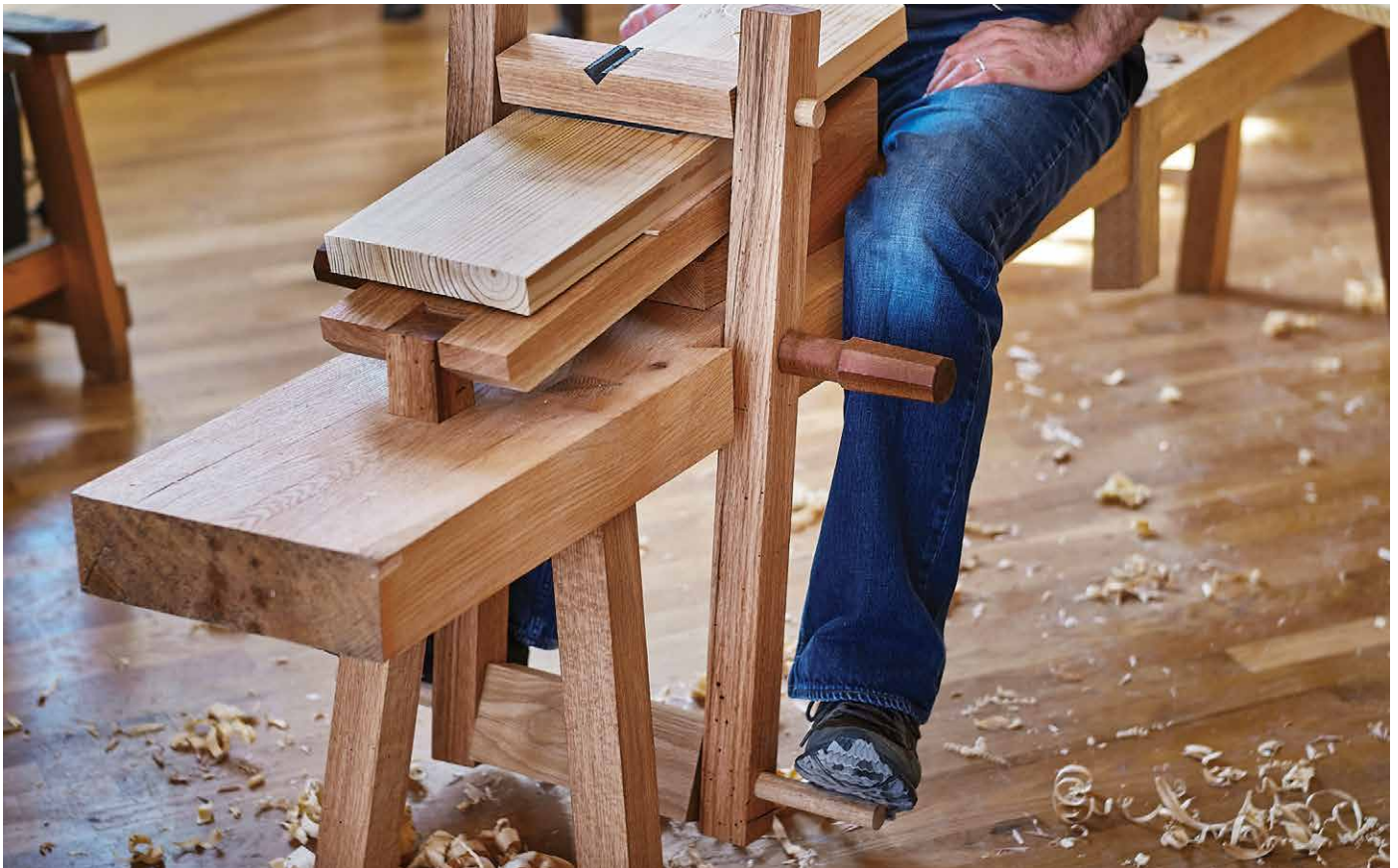
Figure 5.60. An easy accessory. Adding a shaving horse to a low workbench takes about a day. This one was made using oak scraps (hence the different species) that I pulled from my burn pile.
