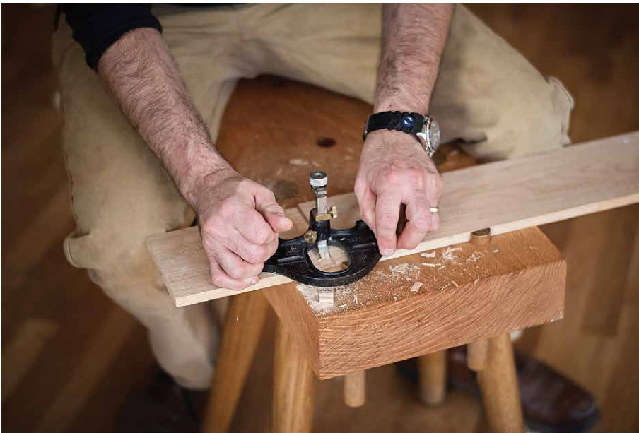
Figures 5.34 & 5.35. Knees and force. Cutting a dado with the assistance of the pegs is a totally natural operation. The only caveat is sometimes you need a sawbench to the side to support long stock.
