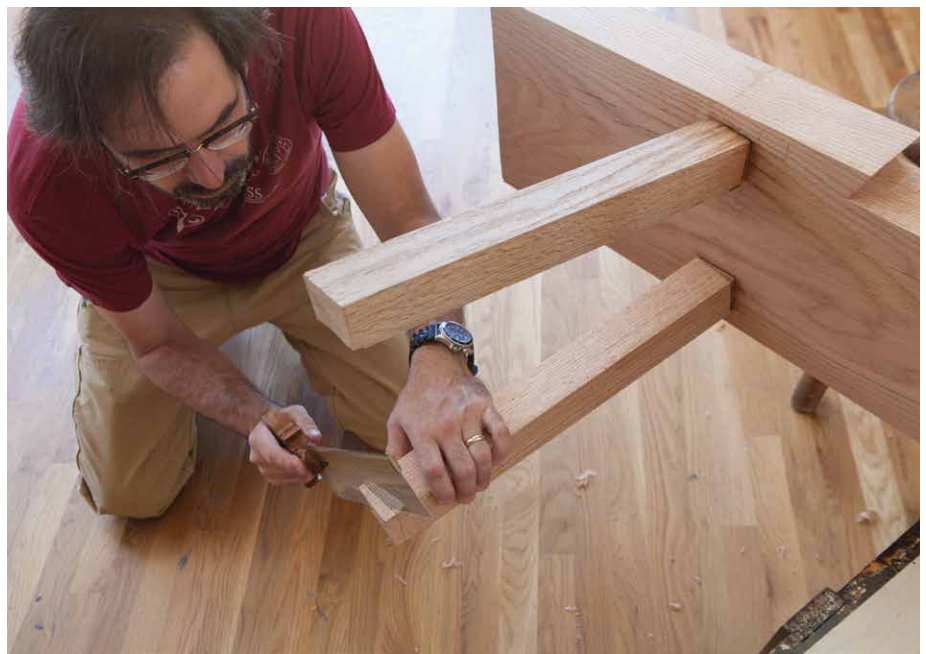
Figure 7.21. Follow three lines. Kerf the one line on the foot. Then tilt the saw to kerf the two adjoining lines that you can see. Then saw through.
