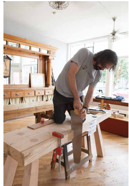
Figure 9.9. Finish it. Clamp the chop as shown to prevent it from splintering when you have sawn it free. Clean up the chop and the notch with chisels and planes.
