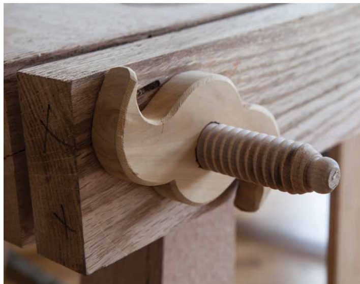
Figure 9.15. Third nut. This shape I drew freehand. No compasses or French curve. This nut I liked.
