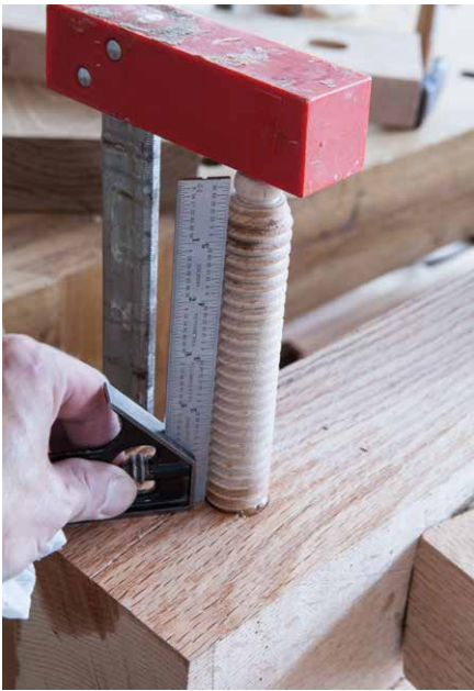
Figure 9.12. Keep it up. There will be slop between the fit of the screws and holes. Epoxy will fill the gap. A try square can confirm the post is truly vertical to the front edge of the benchtop.
