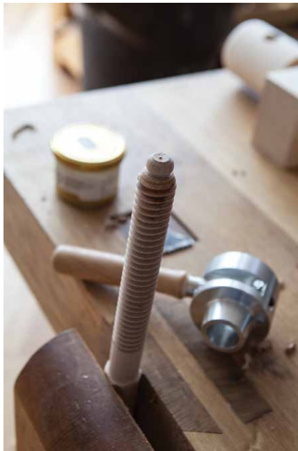
Figure 9.10. Around and around. Threading wood is about steady pressure, steady rotation and avoiding cross-threading the post (with either too much or too little pressure). Practice on a couple sticks before you go for broke.
