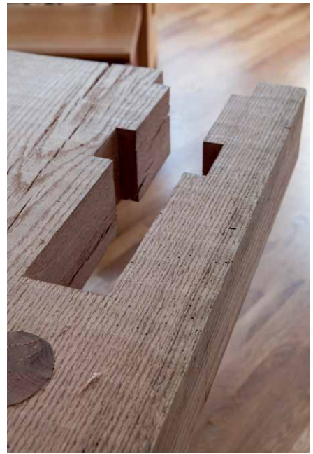
Figure 1.13. The first? Löffelholz's tail vise is surprisingly effective in use. But, like all tail vises, it is an involved process to install.
