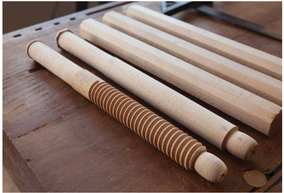
Figure 5.53. The finished screw. The last 4" of the stick is 1" in diameter. The remainder is 1.10" in diameter and threaded.
