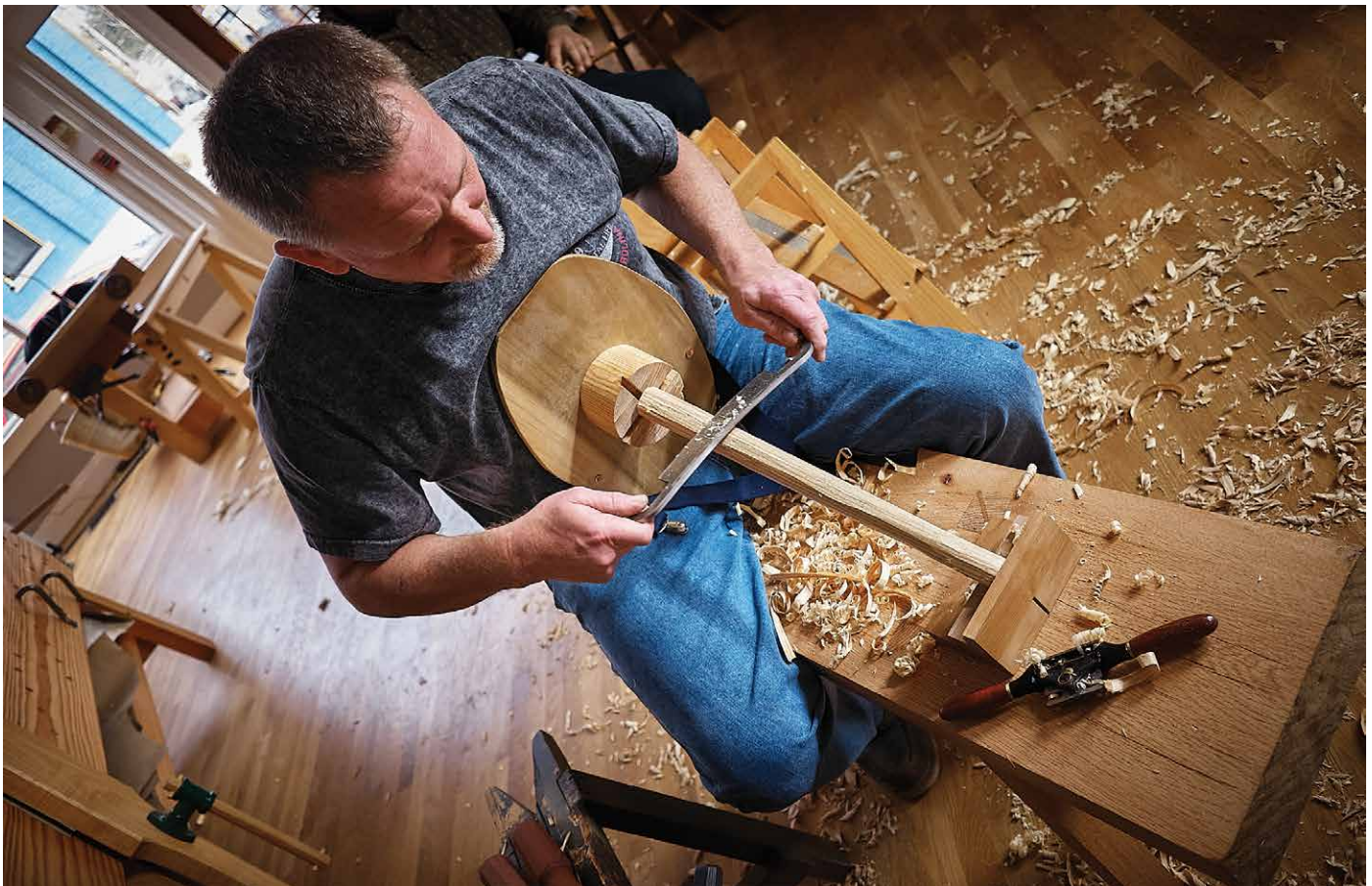
Figure 5.71. Good design. The block in the middle is thick for good reason. Its thickness allows you to get your drawknife right up to the end of the work with remarkable control.
