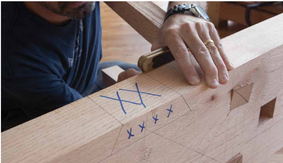
Figure 7.14. Both sides now. Lay out the notches for the side stops on the top and bottom of the benchtop to assist accuracy.
