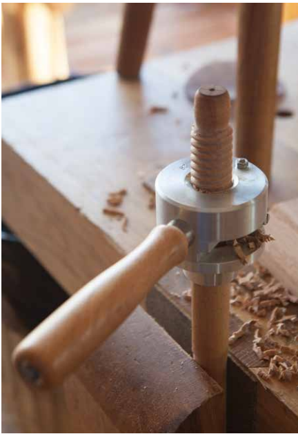
Figure 5.52. One slick tool. Lubricate the cutter with a little tallow or wax with each use. Some people soak the screws overnight in linseed oil. This is supposed to result in crisper threads. It's not entirely necessary with a sharp cutter and a little lubricant.
