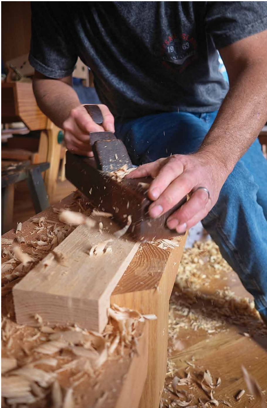
Figure 5.28. Or sit on the work. You can traverse a board diagonally with the assistance of the side stops by sitting on the work. This set-up is remarkably effective for right-handers (left-handers should sit facing the other way).
