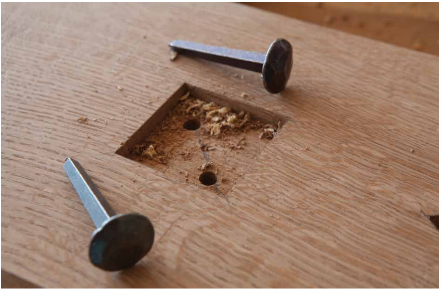
Figure 5.19. Clearance holes. The holes in the palm should be slightly smaller than the shaft of the nail as measured right under the head.
