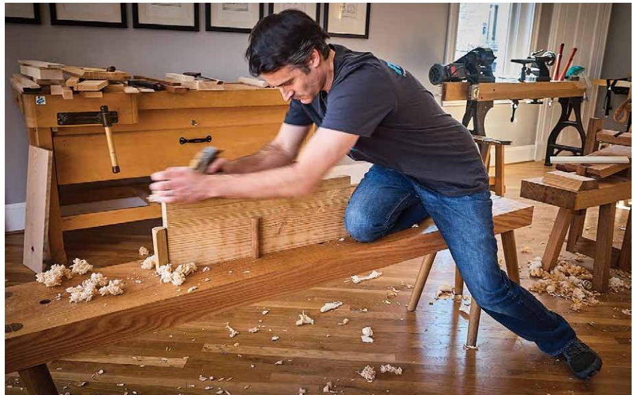
Figure 5.30. Another leg vise. Here Andy Brownell uses his right leg to help immobilize a board for edge planing. This is a trick Megan Fitzpatrick showed us.
