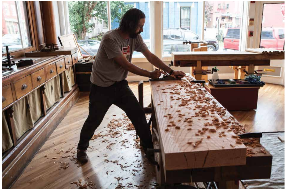
Figures 6.5 & 6.6. True all around. With big slabs you can use fore planes or scrub planes to traverse all the surfaces (even the edges, as shown at left) and bring them into truth.
