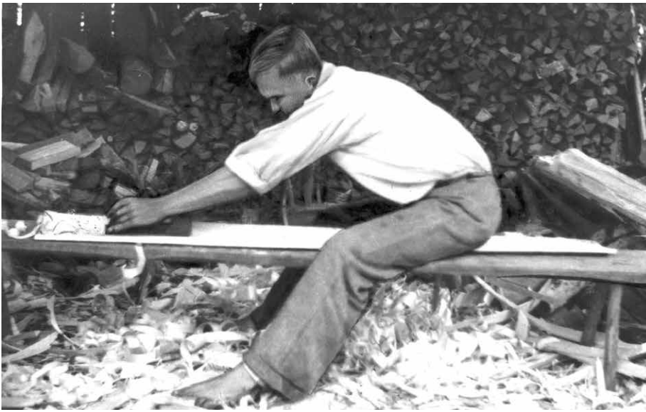
Figure 5.37. Scooting and planing. Planing long boards on a low bench is best done in sections. Each section is as long as your arms can reach.
