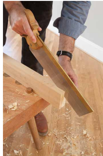
Figure 5.43. Saw, then flip. I'm kneeling on the tenon to saw the face cheek of this tenon. At the end of the cut my saw is nearly vertical. Then I saw the face shoulders while sitting on the bench.
