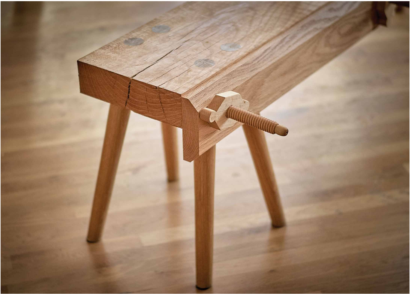
Figure 5.51. Roll your own. Simple screw vises such as this one are quick and easy to make with a threadbox and scraps. You can make as many as you like and as large as you like – even the entire length of the workbench.
