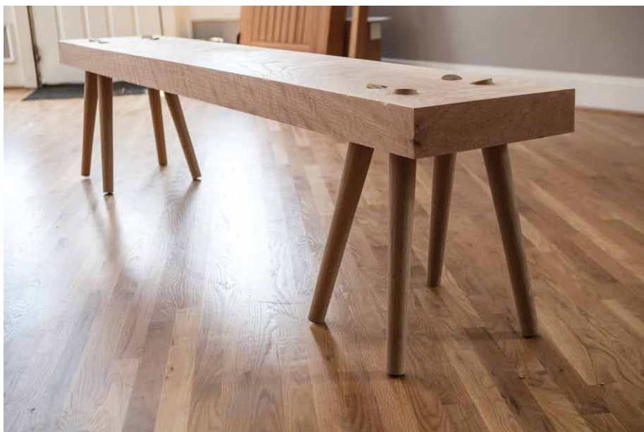
Figure 6.13. Driven. Drive the tenons into their mortises. Flip the bench over and prepare to wedge the tenons.
