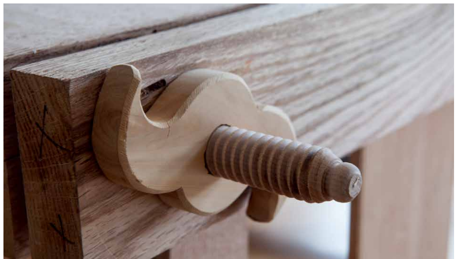
Figure 1.11. German ingenuity. Martin Löffelholz drew two workbenches in a codex dated 1505. Equipped with both a face vise and a tail vise, this appears to be the first modern workbench. The unusual tail vise was the biggest question mark. How well would it work?
