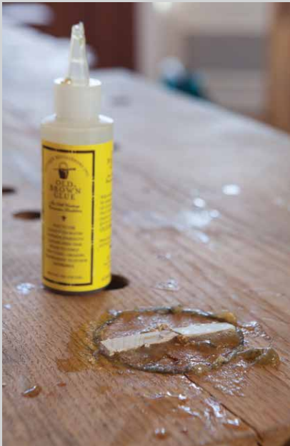
Figure 9.7. Below grade. If you cut your tenons a tad short, it will be easier to flatten the benchtop after assembly.
