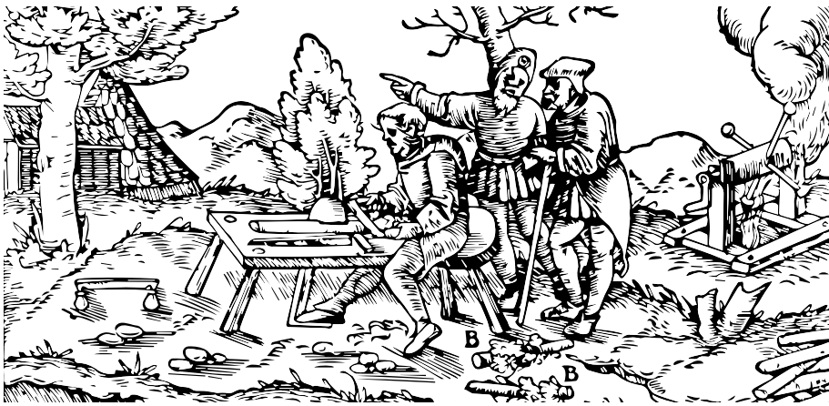
Figure 3.31. Early shavehorse. What is interesting about this image, compared to the Estonian shavehorse, is that some provision has been made to round or shape the seat of the horse, implying that it was purpose-built as a shavehorse.
