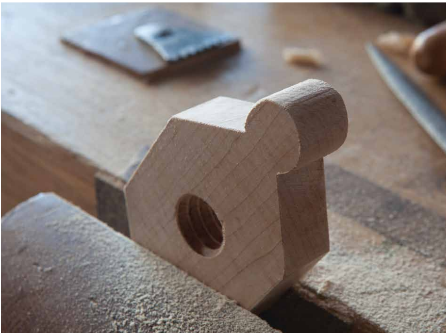
Figure 5.56. Rasp for comfort. After you drill and tap the holes in the nuts, cut them to shape and ease the corners with a rasp. Shown is an alternative shape to the nut above.
