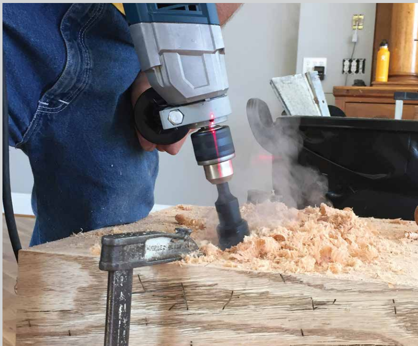
Figure 2.6. That's steam. You can get away with using wet stock if you know the risks.
