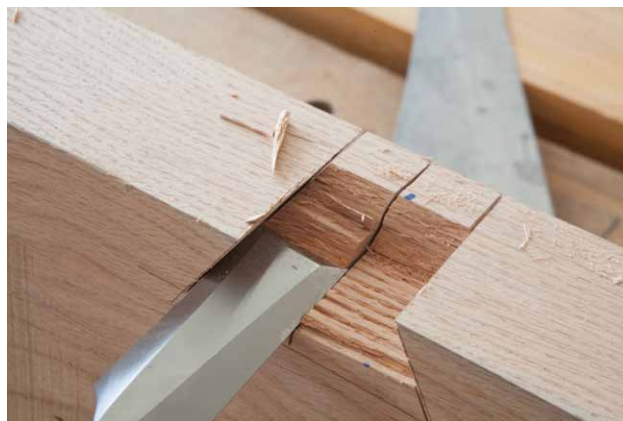
Figure 7.14. Both sides now. Lay out the notches for the side stops on the top and bottom of the benchtop to assist accuracy.
