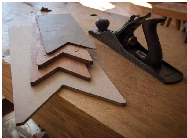
Figure 5.9. No tail vise needed. A notched stick placed at the rear of your work can help immobilize it so you can work across or with the grain of a board.
