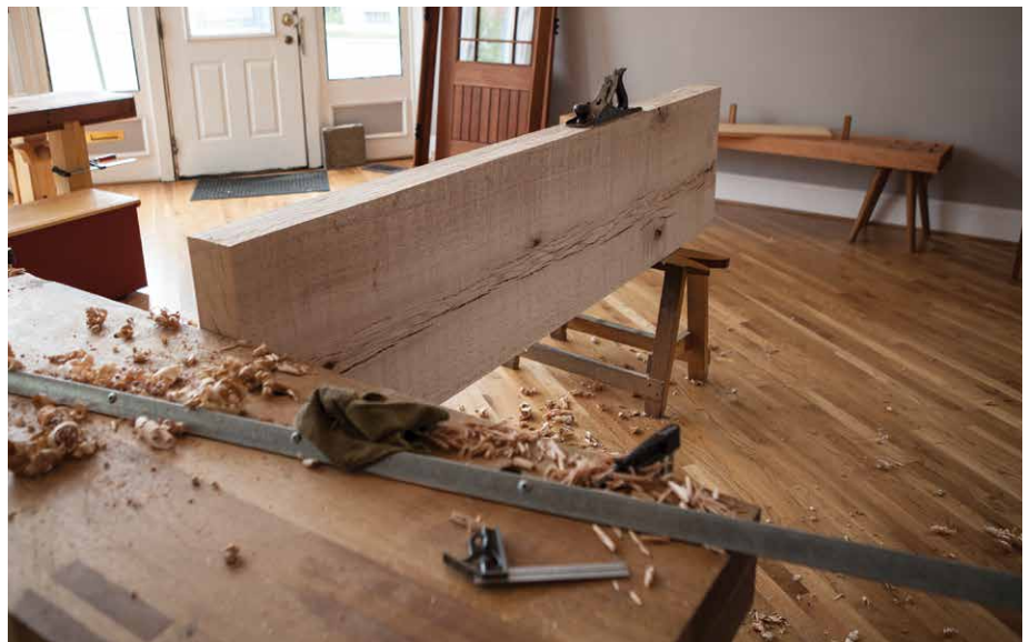
Figure 9.3. Two true. Plane one face flat. True one edge of the slab. Then make the opposite edge parallel to the first. Finally, make the second face parallel to the second. All this fussing will make installing the vise hardware much easier.
