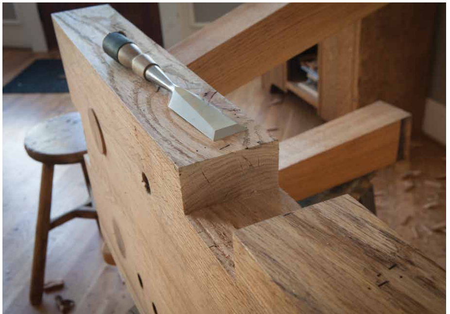
Figure 5.50. Ready to go. With only about 10 minutes of work, you can create a face vise for any work surface. Just make some softwood wedges and get to work.
