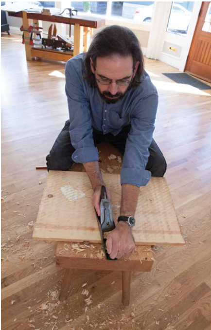
Figure 5.38. Bench stops. Traversing short boards is simple; with longer stock I use a stool or sawbench to support the end that is hanging off the benchtop.
