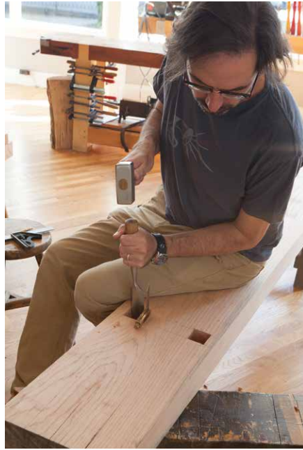
Figure 7.9. Accurate eyes. If you take your time, you'll be surprised by how accurate your compound-angle mortises can be. Just make sure you eyeball the blade of your bevel gauge with the back face of your chisel before every strike. This might seem a slow way to work, but it's faster than fixing overcuts or undercuts.
