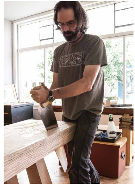
Figure 9.17. Two long rips. Lay out the long rips for the notch and saw them with a coarse rip saw. When the saw is vertical it will cut quickly. Varying the angle – forward and back – will help the saw track vertically.
