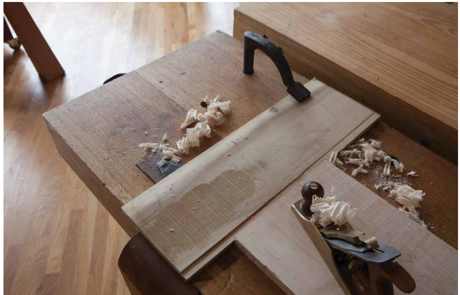
Figure 5.5. Wide planing stop. Add a thin batten in front of your planing stop and you've made an effective planing stop for wide panels.
