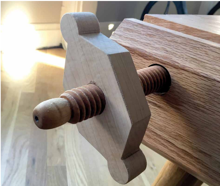
Figure 2.11. I'll stick around. These vises are simpler to make than modern vises, but they are not as convenient (until you get used to them).
