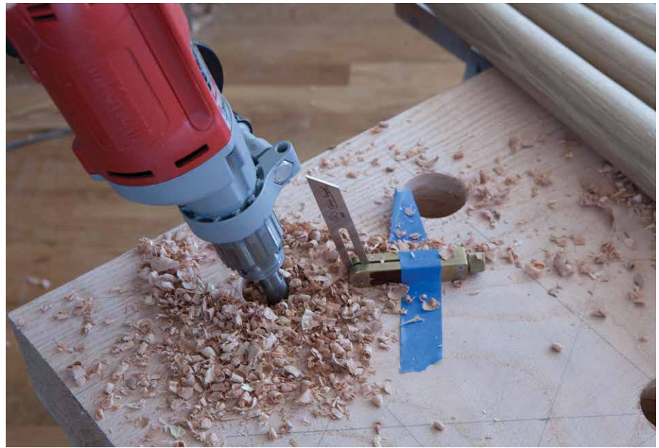
Figure 6.12. Follow the bevel. Here I'm lining up the chuck of the drill with the blade of the sliding bevel. If you are using a long auger bit you can line up the shank of the bit so it's parallel to the blade of the sliding bevel.
