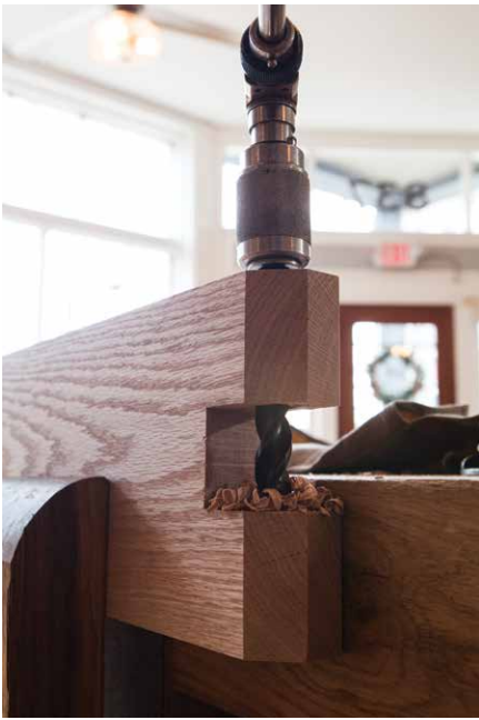
Figure 5.61. Bore the barrel. Bore a 5/8"-diameter hole for the barrel of the hinge. It doesn't need to pass all the way through the width of the stage.
