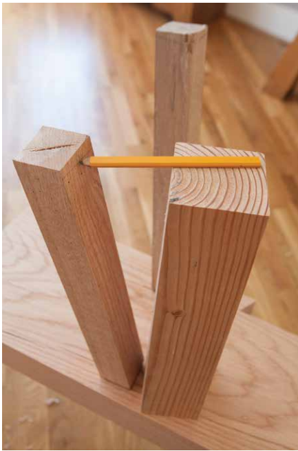
Figure 7.20. Marking a compound cut. The top of the 4x4 represents the floor of your shop. Move the “floor” around and use a half-pencil to scribe the “floor” onto each leg.
