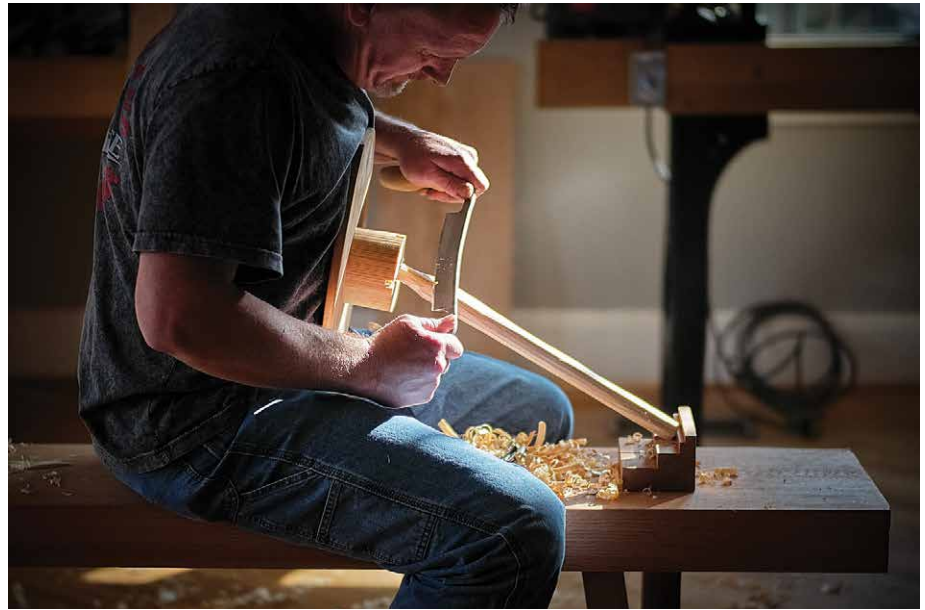
Figure 5.70. Minute made. The "belly" is a remarkable appliance for shaving chair components. While it's not as adept at shaving long, thin spindles, it excels when shaping legs or short spindles.
