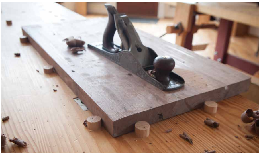
Figure 5.27. With the board. Planing boards 6"-10" wide can be a little tricky because the work is restrained by only one end stop and can rotate. You can fix this by putting a batten in front of the two end stops, making a wide planing stop.
