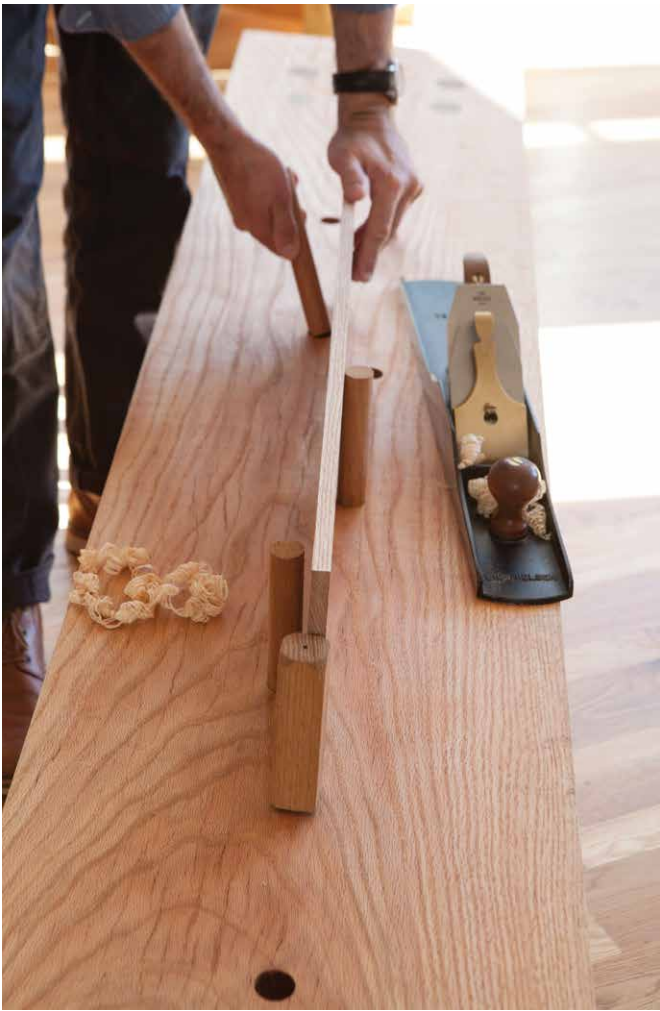
Figure 5.41. I've got this pegged. By having a selection of pegs that vary in length and girth you'll find it easy to secure most boards on the benchtop.
