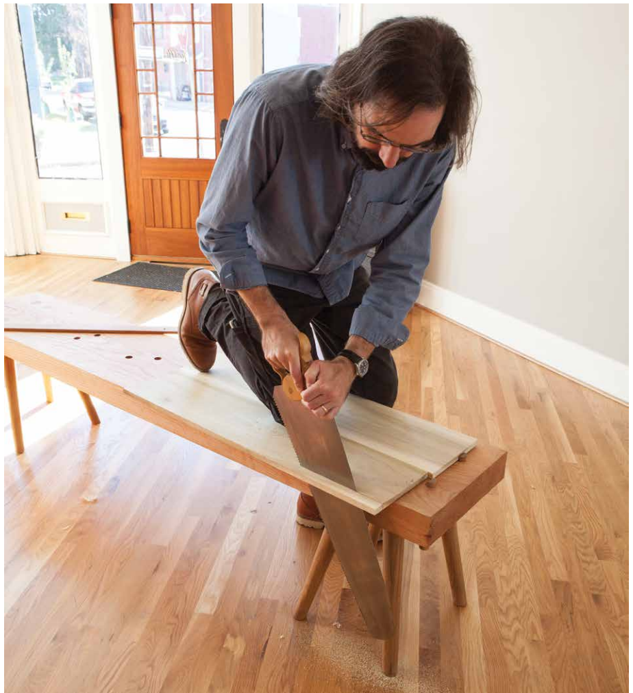
Figure 5.32. An easy rip. Here I’m ripping with one knee on the stock. Occasionally it is more comfortable to rip with both knees on the stock.
