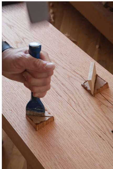
Figure 7.18. That's cold. Open the kerf with a cold chisel before driving in the wedge. This reduces the chance that the wedge's tip will crumple as you drive it.
