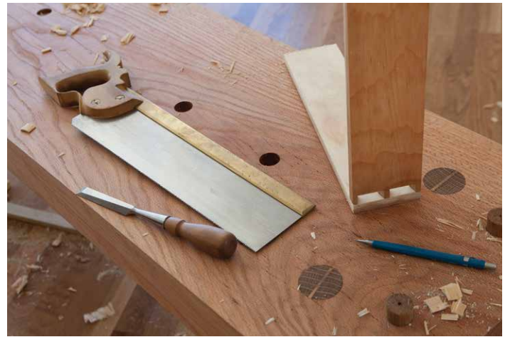
Figure 5.42. Pins first. Transferring the shape of the pins onto the tails is the way to go with this workbench.
