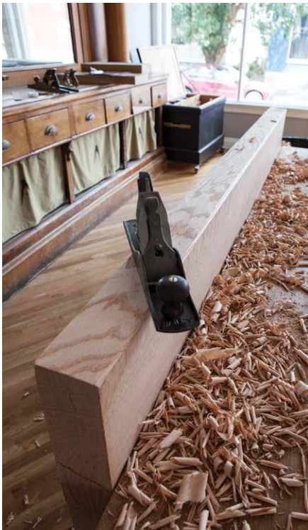
Figures 6.5 & 6.6. True all around. With big slabs you can use fore planes or scrub planes to traverse all the surfaces (even the edges, as shown at left) and bring them into truth.
