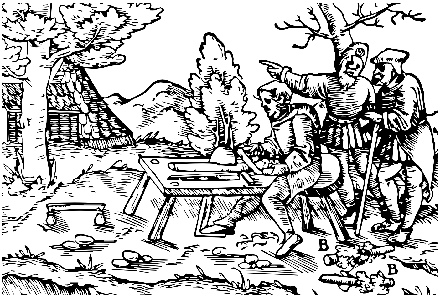
Figure 5.59. Early shaving horse. This horse is featured in the 1561 book “De Re Metallica” (“On the Nature of Metals”) by Georgius Agricola.
