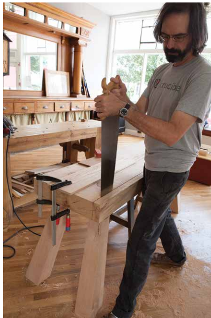
Figure 9.8. Overhand ripping. Ripping the chop is a fantastic lesson in overhand ripping. This technique can be used with the teeth facing the operator or away.
