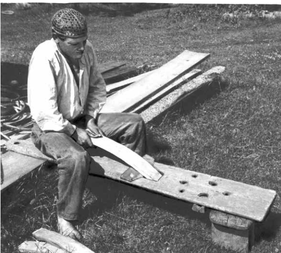
Figure 3.32. A bending bench. Avinurme, Enniksaare village. PHOTOGRAPH BY ANTS VIRES, 1947, FROM "WOODWORKING IN ESTONIA" (LOST ART PRESS). PHOTO LIBRARY 1089:82
