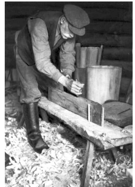
Figure 5.40. More Estonian insight. The peg in the foreground was a clue as to how to edge-joint on a low workbench. The woodworker here is shown straddling the bench; I find it more natural to stand to one side.
