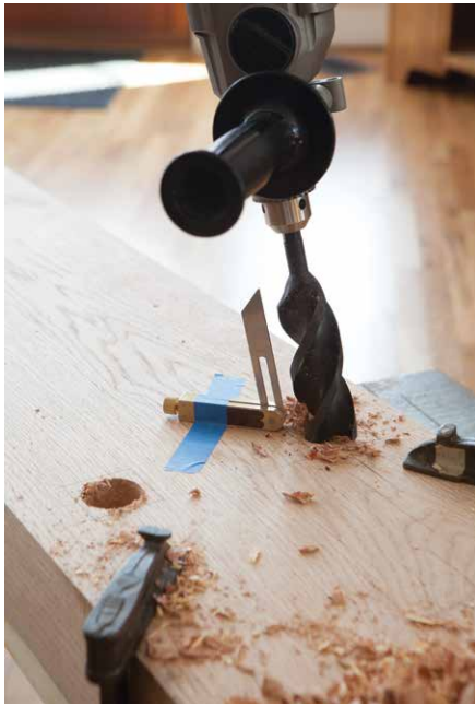
Figure 7.8. Not a masochist. I don't own a 1-1/2" hand-powered auger, so I gladly grabbed my electric drill for this operation. Note the right-angle grip on my drill. If you have one, use it. Your unbroken wrists will thank you.
