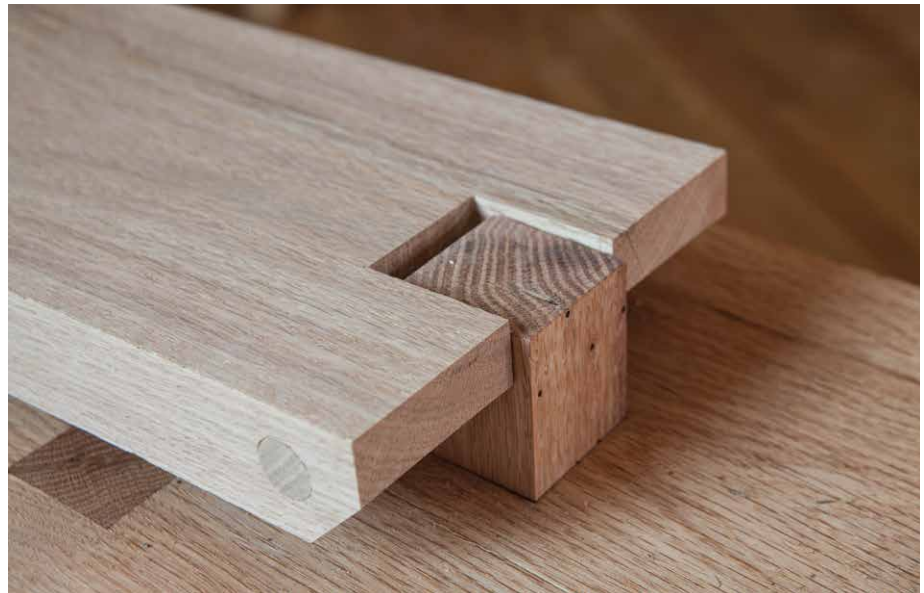
Figure 5.62. Off center. Here you can see how the post protrudes from the rear of the notch. This is because the hole in the post is off center. This allows the stage to move freely.
