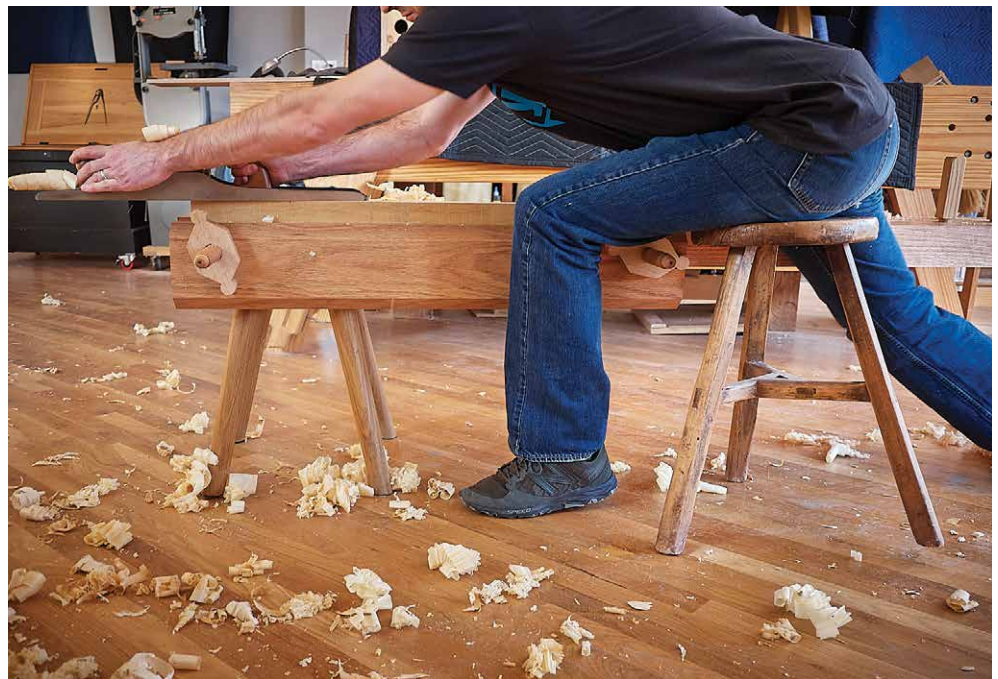
Figure 5.58. Your friend the stool. A sawbench or a stool that is the same height as your bench is a remarkable helper during some operations.
