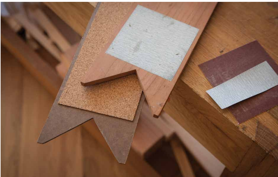
Figure 5.12. A coarse grip. Sticky-back sandpaper or cork can greatly increase the grip of a doe's foot on your benchtop.
