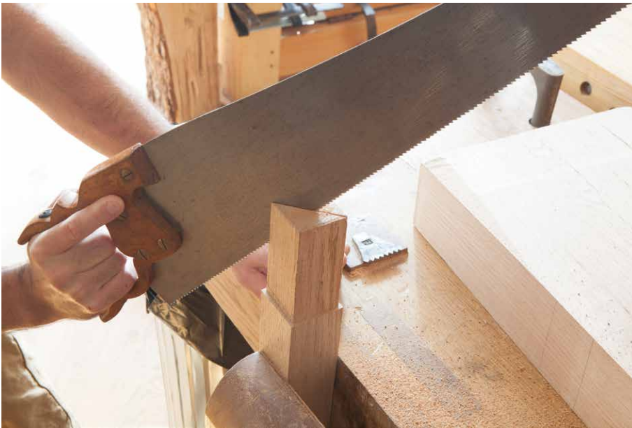
Figure 7.16. Corner to corner. Choose your saw based on how tight the joint is. If your joint is loose, use a fine tenon saw. If it's tight, use a rip panel saw or full-size rip saw. Mark your diagonals with care so they line up in some sort of pattern or it will look disconcerting.
