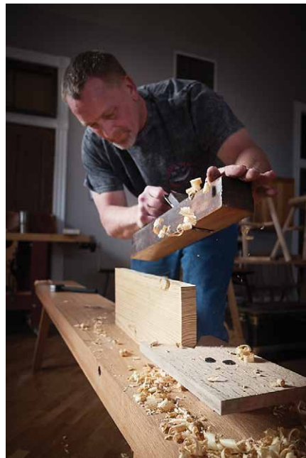
Figures 5.21 & 5.22. Get over it. The palm effectively restrains your work when planing edges and faces. Most of all, the low bench allows you to get your mass right over the cut.
