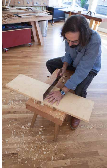
Figure 5.39. Rotate and saw. Sawing while sitting is surprisingly easy once you can shift your body away from your sawing arm.
