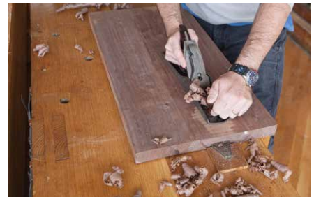
Figure 5.5. Wide planing stop. Add a thin batten in front of your planing stop and you've made an effective planing stop for wide panels.
