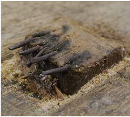
Figure 5.4. The lockjaw stop. This French bench uses nails, now rusty, to secure the work. I have yet to cut myself on a metal planing stop during the last 12 years. So, this looks worse than it really is.
