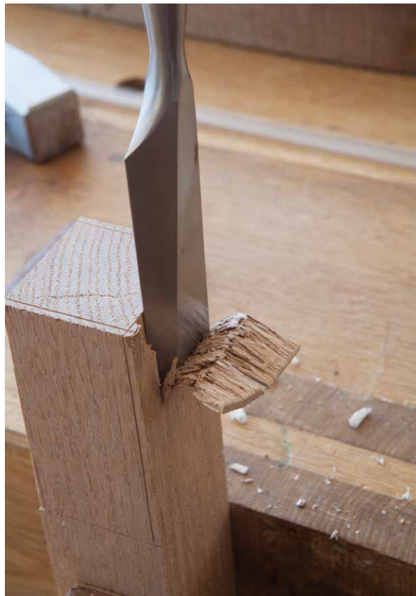
Figure 7.7. Scribe and rive. Before riving the tenon cheeks, use a cutting gauge to mark out the tenon's cheek shape on both the end grain and the long grain. These knife lines will guide your chisel. Place the chisel directly in the gauge line and knock the chisel in. The cheek will peel off as if by witchcraft.
