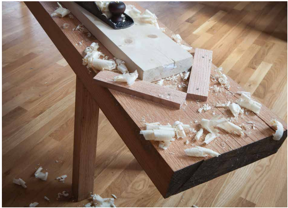
Figure 5.15. A palm. Here I've attached a palm to one of my low workbenches. This arrangement imitates a palm shown on a wheelwright's bench in the "Qingming shanhe tu" scroll made by Zhang Zeduan during the Song Dynasty in the first quarter of the 12th century.
