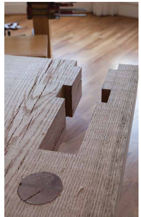
Figures 9.19 & 9.20. Kerf and chop. Waste away as much as possible of the material for the bushing with saw cuts. Then chop the remaining waste away. Confirm the walls are perpendicular and square throughout the process.
