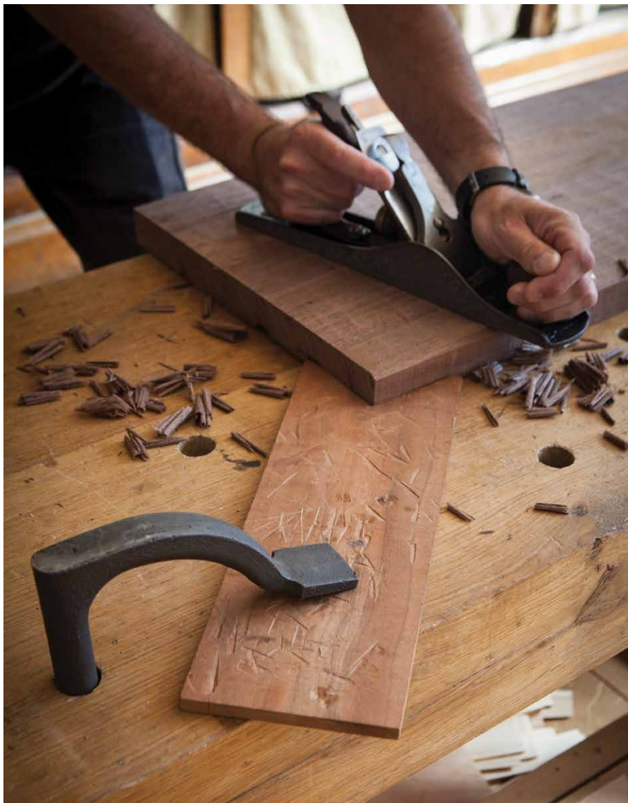
Figure 5.9. No tail vise needed. A notched stick placed at the rear of your work can help immobilize it so you can work across or with the grain of a board.
