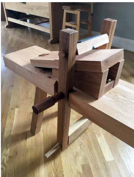
Figure 1.5. Teach a Roman to shave. It is a short intellectual leap from the low workbench to other “sit and work” appliances, such as the shavehorse.
