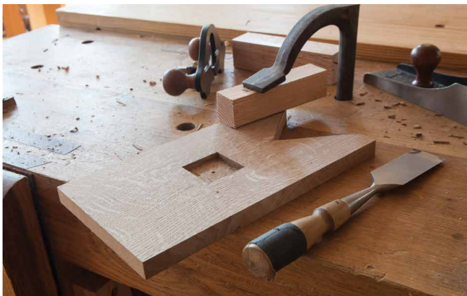
Figure 5.18. Every little bit helps. This shallow mortise in the underside of the palm helps prevent the palm from coming loose from the post.
