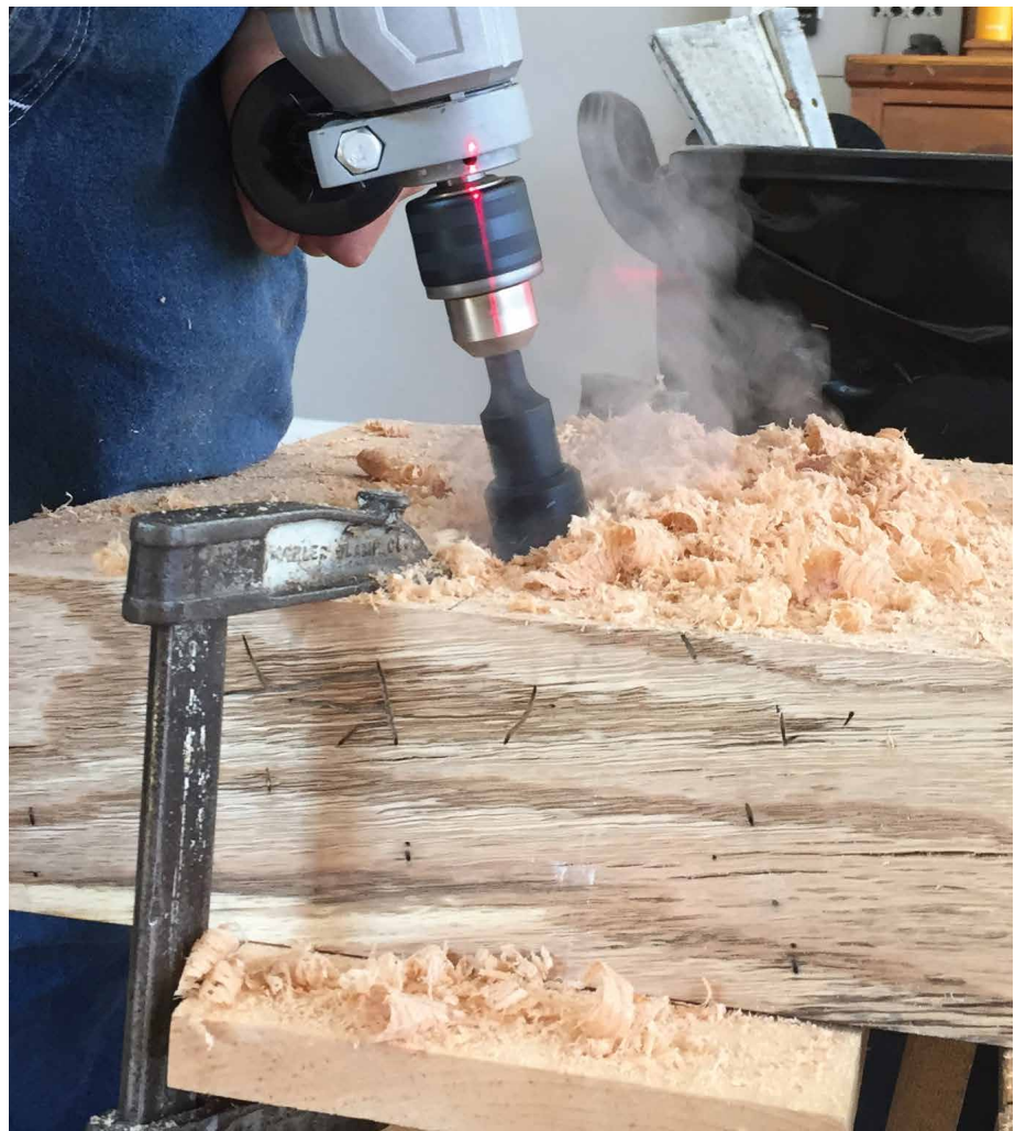
Figure 9.4. Where there’s smoke. The heat of the bit combined with the sopping wet wood resulted in a plume of steam. It was alarming at first, amusing at second and annoying at third.
