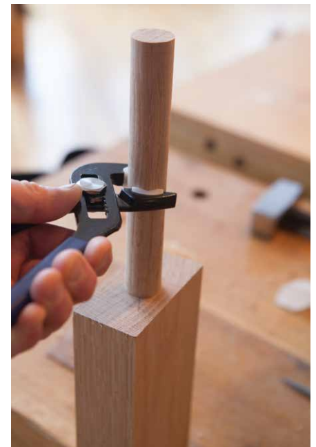
Figure 5.67. Compress the dowels. How do you fit 1" dowels in a 1" hole and allow them to spin freely? Compress the dowels a bit with nylon-jawed pliers.
