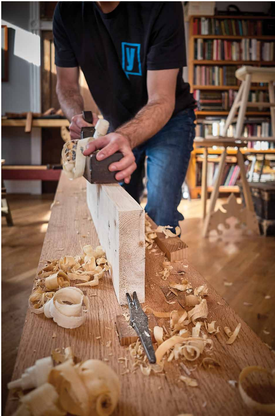
Figure 5.3. It bites. A toothed planing stop is an indispensable appliance for a low workbench. Yes, it marks your work, but many times this isn't a problem if you consider carefully the order of operations on a board (i.e. crosscut the marks away at the end).
