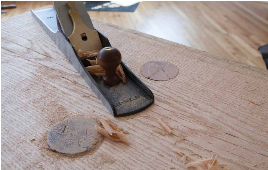
Figure 9.6. Not the last time. As everything dries out, you will need to plane the tops of the tenons flush to the benchtop several times. A heavy plane helps get things close to flush. A small plane finishes the job.
