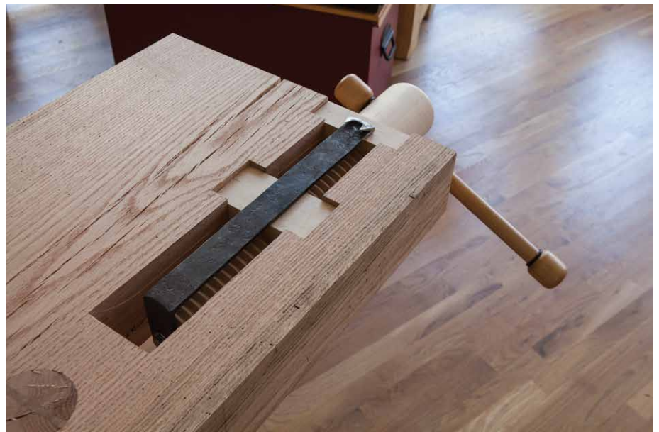
Figure 9.21. Fit and functional. Once you get the vise block bolted in place, the next step is to knock the bushing block up and down until things move smoothly. I thought I would have to secure the bushing block with screws at some point, but everything has shrunk around the bushing block nicely.
