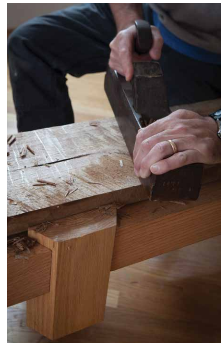
Figure 5.29. Be seated. When traversing boards on a low bench, sit on a sawbench (or any low seat) to get the job done. Yes, it's OK to sit when you work.
