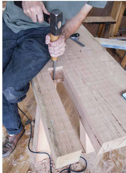
Figure 9.16. In place. Most of your questions about the layout for the tail vise can be answered by laying out the components on the benchtop. Use the components – not measurements – to draw in your lines.
