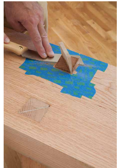
Figure 7.19. Saw around. Kerf the tenon on all four cheeks before committing to sawing all the way through. The kerf will help guide the saw and prevent it from scarring the benchtop.
