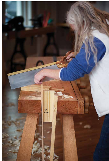
Figures 5.46 & 5.47. Don't dismiss it. We were all shocked at how much holding power a wedge and a notch could provide. Tenoning and even planing the end of this 12"-wide oak board (shown above) was easy.
