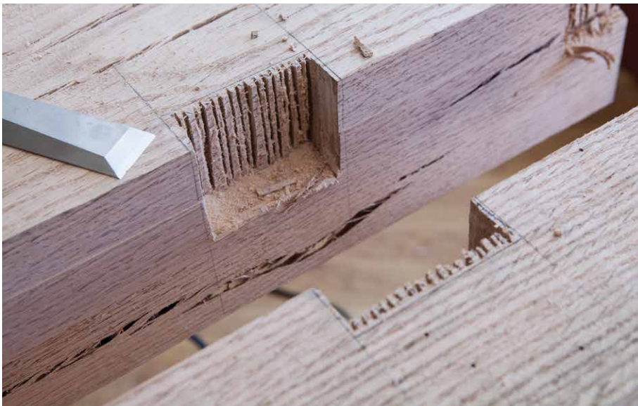
Figures 9.19 & 9.20. Kerf and chop. Waste away as much as possible of the material for the bushing with saw cuts. Then chop the remaining waste away. Confirm the walls are perpendicular and square throughout the process.
