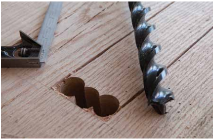
Figure 9.18. Drill and chop. Remove the waste between your two long rips. I bored a few holes at the end of the notch and levered out the waste with a heavy chisel.
