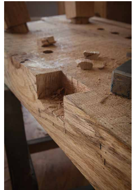
Figure 5.49. Quick work. With the notch on the edge, you saw the walls and pry the waste out easily with a chisel. Then clean the long grain of the notch with paring cuts.
