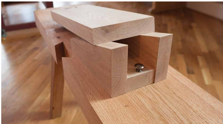
Figures 5.64, 5.65 & 5.66. It's a chock. The chock of the shavehorse is three bits of wood planed up and glued together. Nothing fancy.
