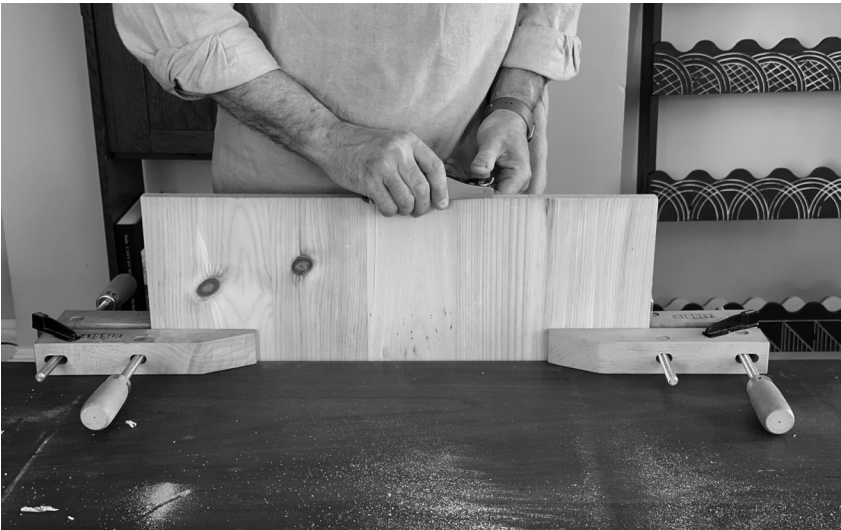
Two handscrews clamped to your table make an effective vise for planing end grain or even sawing dovetails.
