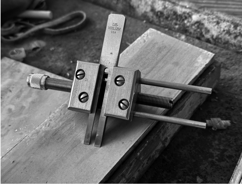
The ingenious Lie-Nielsen forked cutter clamped (with care) in a honing guide.
