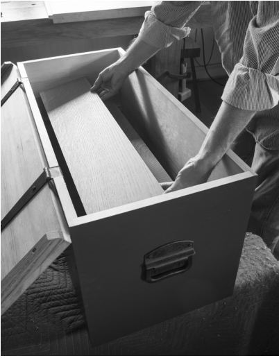
Shoot the bottom. After cutting the till bottom to a close size, shoot its ends until the bottom slides smoothly on its runners.
