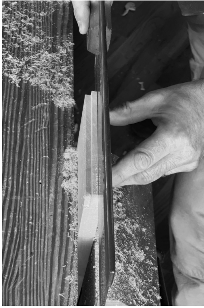
This is like using a flush-cutting saw. Press the sawplate against the little stub of a tenon.
