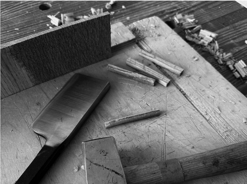
A hacking knife quickly splits out raw trenails from a board.
