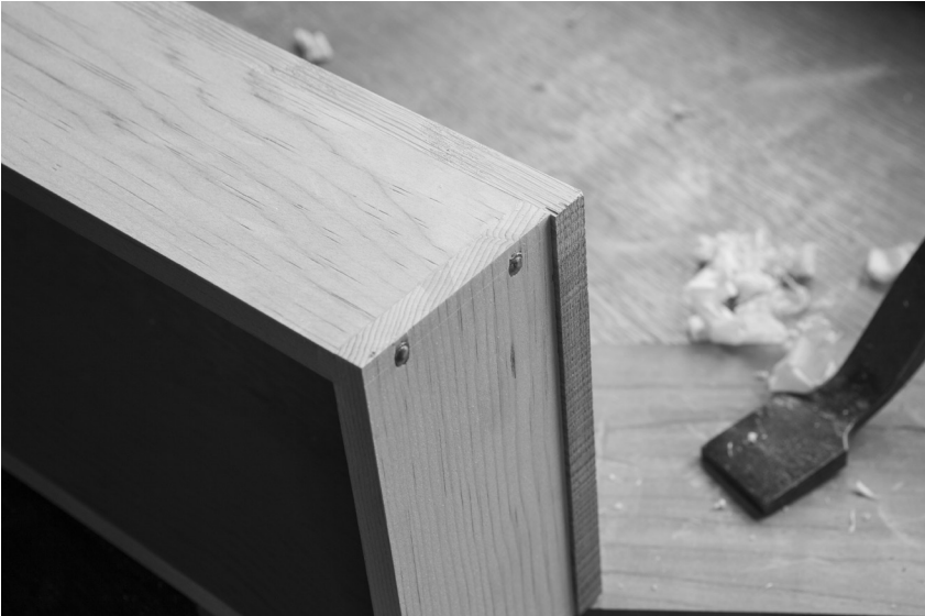
Slightly proud. Leaving the bottom end slightly proud of the tray solves a variety of potential problems.
