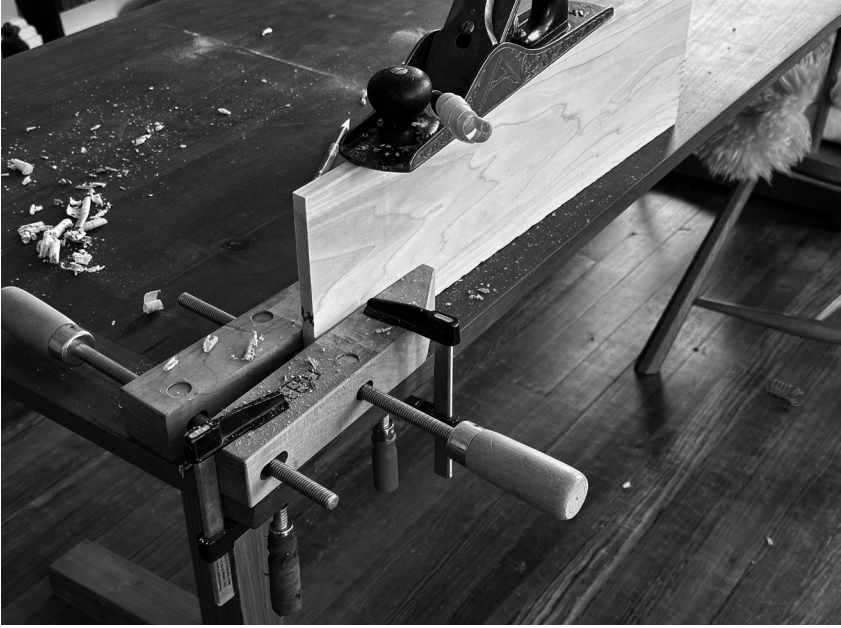
A handscrew clamped to the corner of your dining table is an effective vise for holding boards on edge while planing them.
