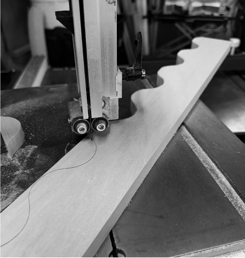
An inexpensive band saw makes easy work of the dozens of curved bumps.
