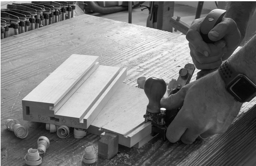
Now groove the interior face of each post as shown. These grooves receive the coffer's side panels. If you don't have a tail vise, put the post in your face vise and plane the groove with the tool turned 90° (it's easy).
