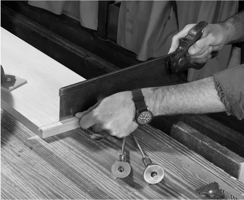
The knife line from the cutting gauge guides the backsaw as you cut the shoulder of the rabbet.
