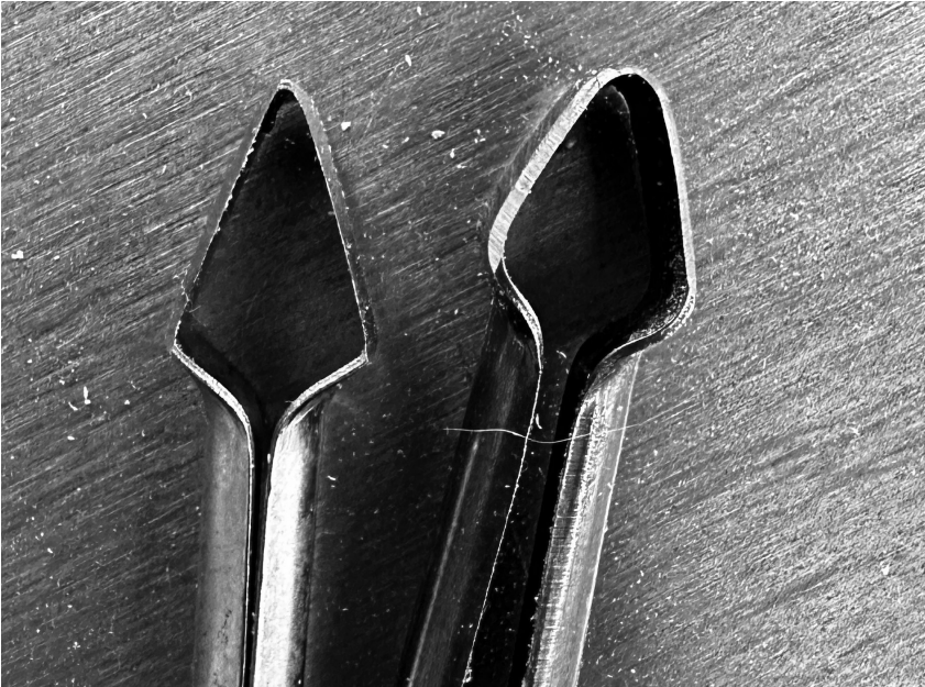
The pear-shaped vinyl cutter on the right is ideal. The one on the left is difficult to sharpen. Both are available world wide (with some effort).
