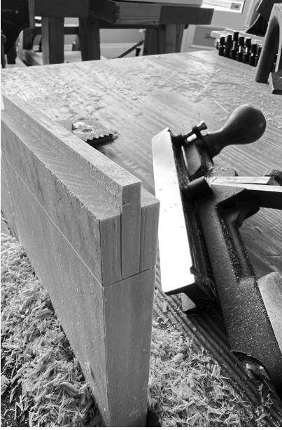
The end of the tenon after you use the No. 48 on it.
