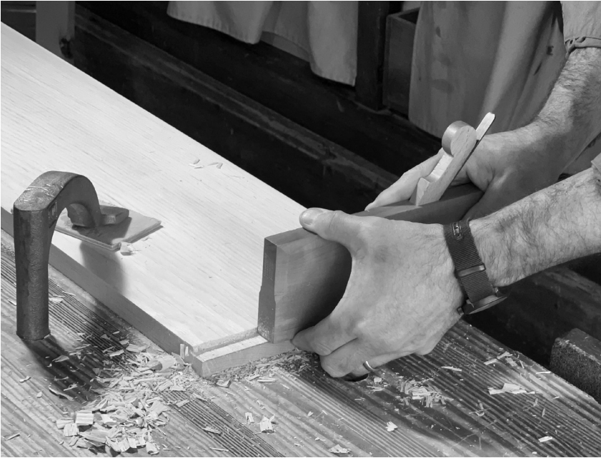
Straight rabet planes are a joy to use – and are simple to sharpen.
