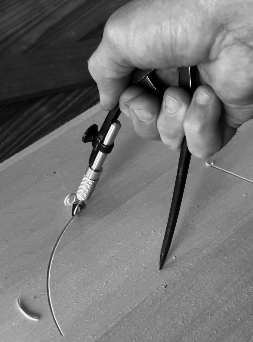
This is a small compass, but note how I am grasping the tool to stabilize it during the cut.
