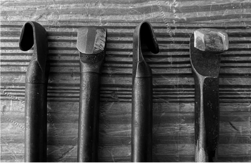
Some of the early engraving cutters that blacksmith Peter Ross made for me.
