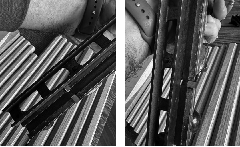
A Stanley No. 48 set up for tonguing (left) and grooving (right).
