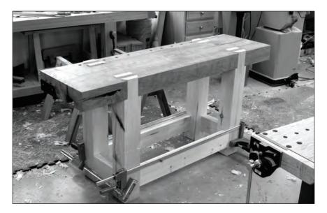
**Permanent.** The sliding dovetail and through-tenon on this French bench makes a bench where the base and top act as one.
