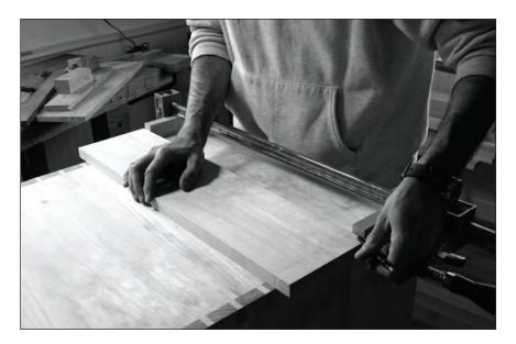
**Skirt in the air.** With the partially finished skirt clamped to the carcase, show the fourth skirt piece to the assembly. Mark where they intersect so you can trim the long skirt boards to their finished length.
