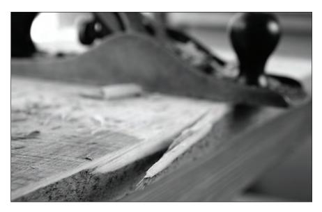
**The speich stopper.** A bigger chamfer on the edge of this board would have helped prevent the edge from splitting off when I traversed it.
