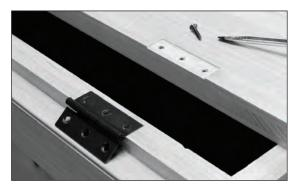
**Install, remove, repeat.** After installing one hinge leaf, remove the hinge and cut the mortise for the other leaf. Having the hinge unattached makes a good fit easier to accomplish.
