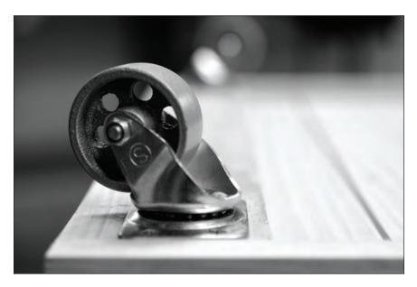
**Cheap and durable.** These cast metal wheels are inexpensive and work well on my flat wooden shop floor. They squeak (even when greased), but oh well.
