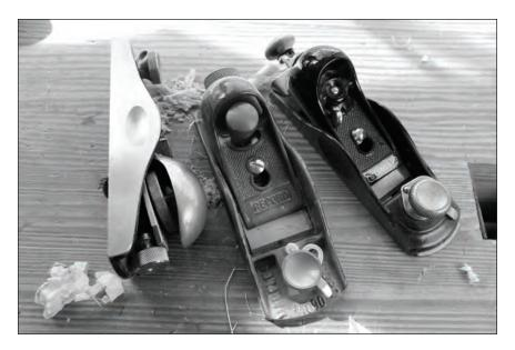
**The run-around.** The lever cap can be locked down using a screw-feed mechanism, a lever or even other mechanisms, such as a wedge. I like the screw-feed mechanism, but the other ways work fine, too
