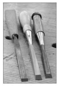
Three styles. Tang chisels are the easiest to make and repair. Socket chisels are durable. And Japanese chisels combine characteristics of both and are nigh on bulletproof (but harder to make).
