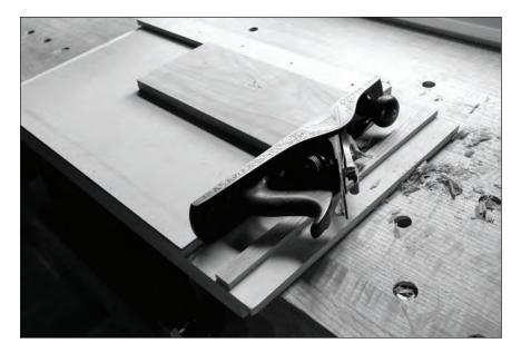
**The saw's friend.** A shooting board removes the sawblade marks from the end of a board and trues it up. Plus, you can adjust the length of the board in .001" increments.
