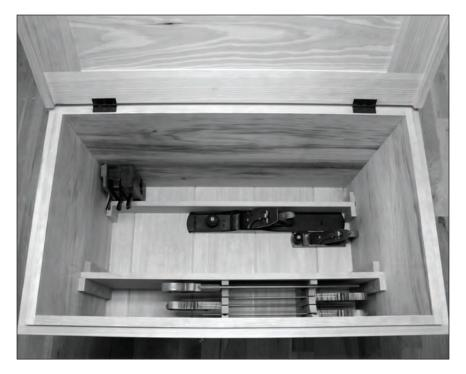
**The long of it.** My 24"-long jointer/try plane is the biggest plane I own. So I made sure that it would fit in the bottom of my chest and could be easily removed.
