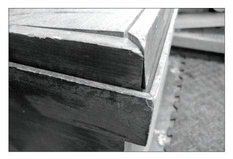
Miters and mayhem. The flat panel lid warped and shrank. The miters lost their hold. This lid is a mess.
