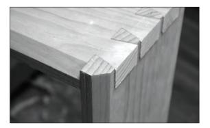
Almost right. By chamfering the skirt before assembly, I made it easy to lay out and cut the profile – it was all with-the-grain work. But when the corners are assembled you can see how the half pin needs to be cut back.
