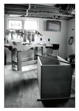
**Assemble slowly.** You can assemble this case one panel at at time if you like. Begin by making one corner by assembling the back and one end. Add the other end piece. Then add the front piece.
