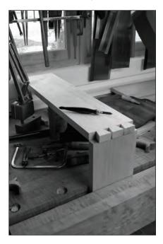
Tails on the ends. The tail board of the skirt should have about three tails. You can keep this simple and just use through-dovetails. Save your mitered dovetails for an instance where they will show.
