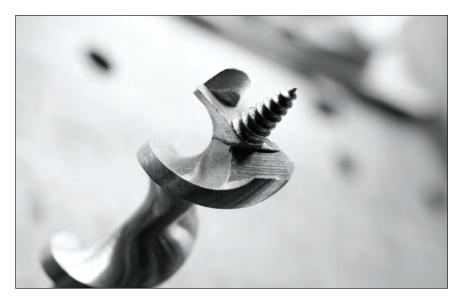
**The important bits.** Here you can see the lead screw, the spurs and the cutting lip. Keep these sharp. Keep the spirals polished. Do these two things and you will be a human drill press.
