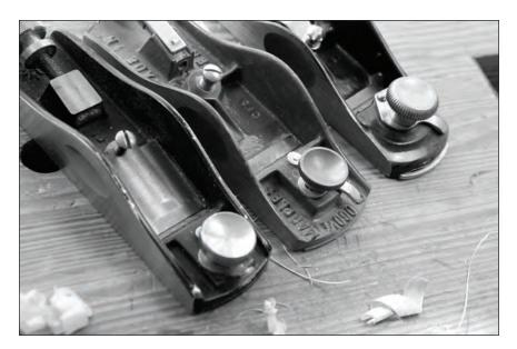
**What you pay for.** At front is what the bed will look like if it has been machined by a milling machine. This is the most accurate way of milling the bed for the iron. A small error in the bed of a block plane is disastrous.
