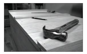
**Three disposable strips.** These battens will rot first if your chest is exposed to water, and they are easy to replace because they aren't nailed to the base moulding.
