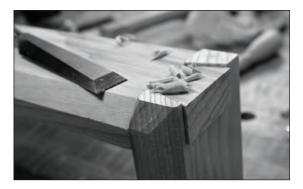
**Coping with a chisel.** Cut the chamfer with your block plane before assembling the dust seal. Dry-fit the seal then chamfer the corners with a chisel to make the profile follow all around the carcase.
