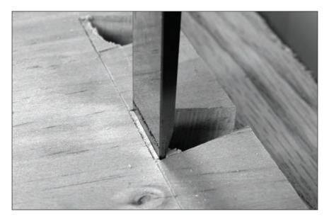
**Halfway home.** Here I have about 1/8" of waste left, so I place the chisel 1/16" away from the baseline and drive the tool halfway through the thickness.
