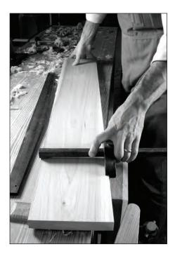
accurate than one mighty stroke. After a few strokes you can really bear down on the gauge's pin or knife to deepen the line. But don't do that on the first stroke.
