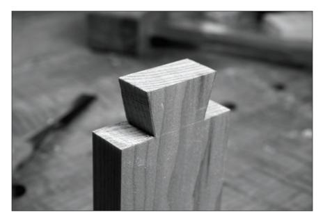
**One tail.** Because the mini-skirt is so narrow you really can't put more than a single dovetail at each corner unless you decrease the slope of the joint. One tail will do the trick – especially when compared to a plain old miter on some chests.
