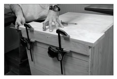
**A fitting end.** Place one of the skirt's end board on the end of the chest. Clamp it to the chest and then lay out your baselines for your dovetail joints by marking the seam between the carcase and the inside of the skirt board.
