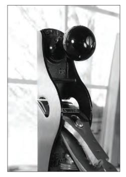
work well with taller workbenches unlike the wooden-bodied planes. The metallic mass of the plane helps keep the tool in the cut, and the orientation of the tote and knob allow you to use the tool without getting your entire upper body over it, which is a necessary body position when using wooden planes.
