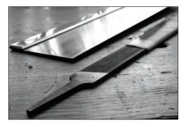
der of business when sharpening a scraper. The file removes the fatigued steel and exposes a fresh edge to hone and polish. You can file a saw or scraper freehand if you have the hand skills, but I prefer to do both operations guided by a block of wood to keep the file at 90° to the tool I'm sharpening.
