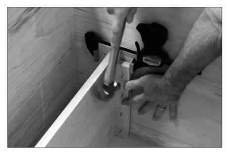
**Cleats for now.** There are more permanent ways to install the wall between the sawtill and well for the bench planes. But the problem is that those methods are more permanent. Four nailed cleats will do the job admirably and allow changes down the road.
