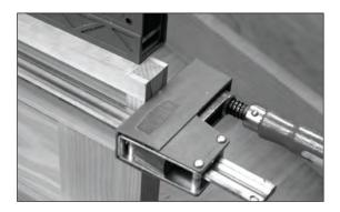
**Slightly off.** Don't clamp right on the dovetail joints. Clamp on the baseline instead. This will close up the joint and press the skirt to the lid.
