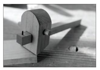
**Here, diagonally.** This shop-made marking gauge, modeled after early tools, uses a wedge that crowds the step of the gauge into a corner of the head, which makes the tool more accurate.
