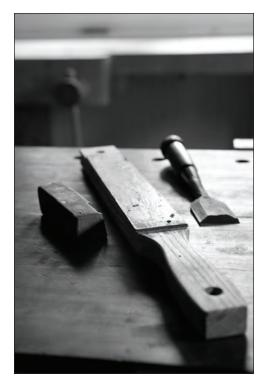
**It's just polish.** Many woodworkers find stropping mysterious. Like the strop compound is some magic paste. Stropping is simply polishing at the very fine spectrum. The strop compound is just an abrasive.
