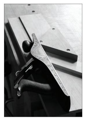
**For 45°s.** A miter shooting board is an ideal appliance if you don't have a good miter box. It can correct wayward hand-cut miters.
