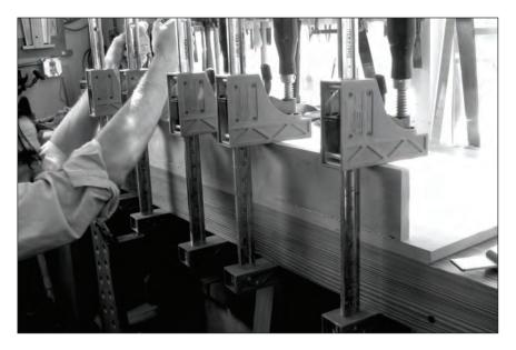
**No skirts**. A thin and wide skirt on a workbench will impede your clamping efforts at every turn. A flat underside is a nice feature, no matter what sort of woodworker you are.
