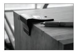
minum one for a trifling. I like the aluminum one because I can use it without worrying about my knife slicing it up. And it has handy little grips. The downside to these little tools is that they lock you into one particular angle. Me? I don't mind this. I like the look of 14°, and that angle works for every dovetail application I've come across.
