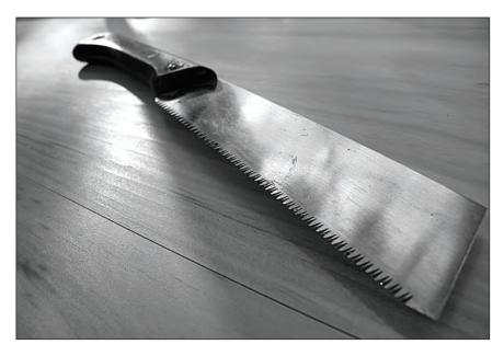
**Useful when understood.** Flush-cut saws are supposed to have no set, so they won't scratch the work. Truth is, they have a little set on one side and no set on the other. You need to get this straight in your head before making critical finish cuts.
