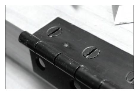
It's all about timing. Lining up the slots on the screw heads is called "timing" the screws so they all stop in the same place. Yes, it is totally anal retentive.
