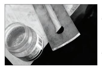
**The grind.** The jack plane blade should have a cutting edge that is shaped like a thumbnail. The gentle curve allows you to remove lots of stock without the corners digging in.
