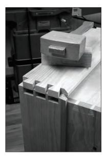
**Not mitered.** Dovetail your skirt and dust seal to the shell to ensure they stick around. Literally.
