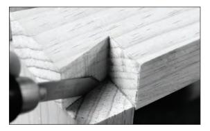
**Pointy bit by bit.** Use light downward pressure on your first two strokes. Then you can increase the downward pressure during subsequent strokes to create a nice crisp line.
