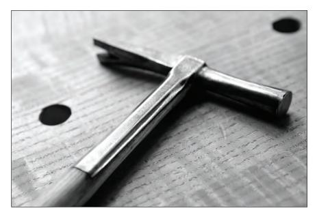
**Hold my head.** The straps, sometimes called "ears," were designed to keep the head and the handle together. Flying heads were once a common scourge.
