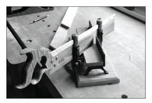
Once I sharpened the saw and lubricated the parts, I cut some miters with it.
