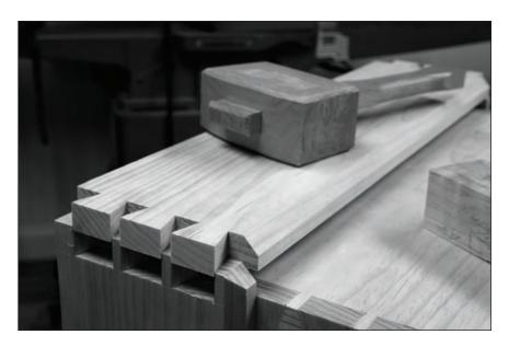
**Before the great slide.** This is the dry-assembly, right before I broke out the glue and all mayhem broke loose. Just keep lots of clamps handy for this process. This is the trickiest glue-up of the project.
