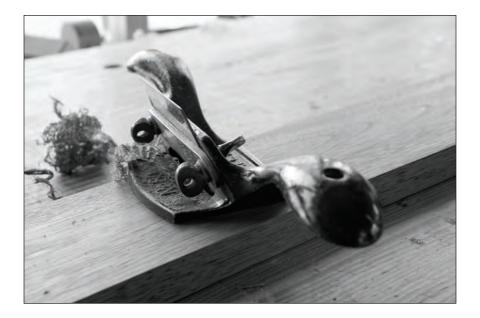
hook faces forward. Secure the iron. Turn the tool's thumbscrew slightly to bow the blade. If you take a light cut you will have tremendous results. Tooheavy a cut will result in chatter.
