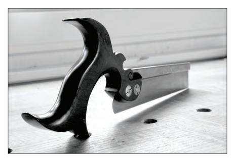
**The small saw.** Dovetail saws are used for dovetailing and for any other small joinery chore. Don't abuse it, however, because these tools are easy to mangle.
