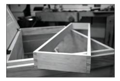
Two for the top. I used two through-dovetails at each corner of the small trays. There is no groove for the bottom, so these are as simple as it gets.
