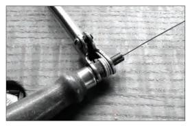
The string is the thing. The Jones patent coping saw has a string through the frame that links the toe and the heel of the blade. They rotate together as a result. It works, but there is a bit of a delay.
