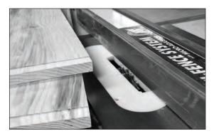
**Run rabbet run.** This shallow rabbet on the inside of my tail boards makes transferring the tail shape to the pin board a quick and fuss-less process.
