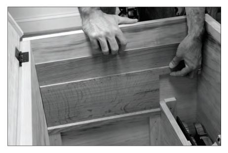
**Stacked.** Here you can see how the runners work. The lower runner rests on the cleats below. Above that are the 1/2"-thick runners (note the extension near the front of the chest). The top 1/4"-thick runner runs the full inside depth of the chest.
