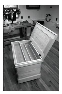
**Three trays.** Here you can see my three sliding trays arrayed out so I can see everything in them. I'm only one hand motion away from accessing any of the three bins in the bottom of the chest. chest so that each tray can be pulled up and out of the chest if you need to repair it or mess around with some serious business below. Trust me on this – you don't want your trays to be a permanent installation.
