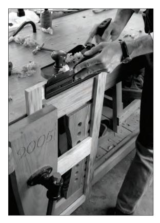
**Plane into the screws.** Many woodworkers want to reverse the positions of the vises on their bench because they think it will make crosscutting easier. But if you don't plane into the screws of your face vise, you'll tend to pull the board out of the vise's grip.
