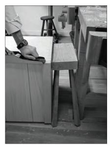
And the hard bits. You might be wondering how to true up the end grain of the bottom boards. The answer: mass and sharpness. A sharp metal try plane can plow through the end grain and bring the proud bottom bits flush with the carcase.
