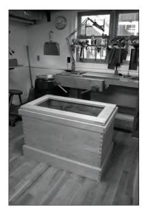
A trial fit. You want to discover if your lid frame needs fixing before you get out the glue. A little twist or some undersized rails are a rude surprise that you can avoid. I'd rather re-make one component than glue up an entire lid that needs to go on the bonfire.
