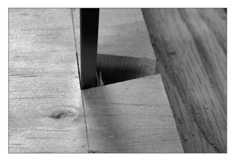
**On the line.** When I have 1/16" of waste left (or less), I drop the tip of the chisel in the baseline and drive down.
