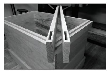
**Mortises that don't mess around.** Yeah, using a through-mortise here at the corners of the lid's framework is definitely excessive. But after dealing with a wimpy lid for more than a decade....
