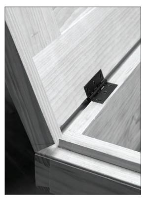
A temporary stop. By beveling the excess of the lid's skirt, you can create a temporary stop for the lid. You can use this as a permanent stop if you are careful, but using a chain is gentler on the hinges and the screws.
