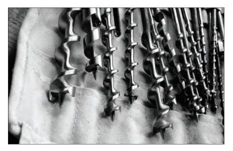
**Wood chewers.** Auger bits are mechanical marvels. When sharp, they allow you to chew through wood at an astonishing rate.
