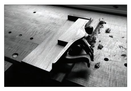
**For edges.** If you are unsteady with your jointer plane, a long grain shooting board is an ideal way to shoot long edges and maintain a square edge. They are built like the end grain shooting board, but with a much longer and narrower bed.
