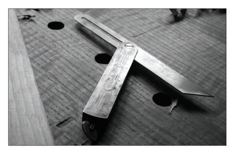
**Better in metal.** Sliding bevels are tricky tools. Even expensive ones are poor. You need one that locks securely and doesn't interfere with layout. In general, the ones that lock at the base of the handle are the best.
