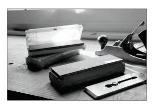
How fast? The honing process on a waterstone can be as brief as three or four strokes. On an oilstone, I would expect to make 20 or 30 strokes to cut a fresh edge. For a hobbyist woodworker this difference isn't all that big a deal. But for a person who sharpens as much as I do, the cutting speed is noticeable.
