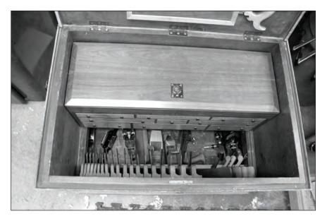
**Sliding till.** The fancy-pants solution to divvying up the top of the chest is to make a large sliding till with integrated drawers. This has upsides and downsides.
