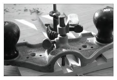
**Yup, a depth stop.** The plate and post that close up the mouth of the Stanley No. 71 can be turned upside down to serve as a depth stop. When the collar of the plate touches the base casting, you are done.
