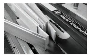
**Long and strong.** These tenons have an enormous gluing area thanks to the length and width of the tenons. Take care when assembling things; the mortises are a bit weak until the rails and stiles are glued up.
