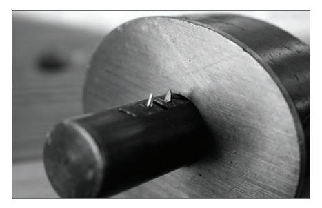
**Twice the chore.** A mortise gauge seems like a good idea, until you have to set it over and over for different widths of mortises. I started using a single cutting gauge for marking mortises, and found it easy to do. The pins of this gauge are filed to mark tenons.
