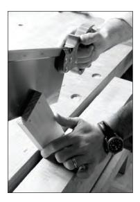
**Angles are essential.** The trick to sawing accurately and not choking the gullets is to saw the tenon at 45°. Three cuts at 45° ensure the teeth will rarely engage the full width of the work.
