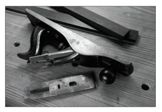
**Bend me, shape me.** A jack plane can be easily pushed to do the jobs of longer and shorter planes. A couple extra irons for the plane make this a simple switch.
