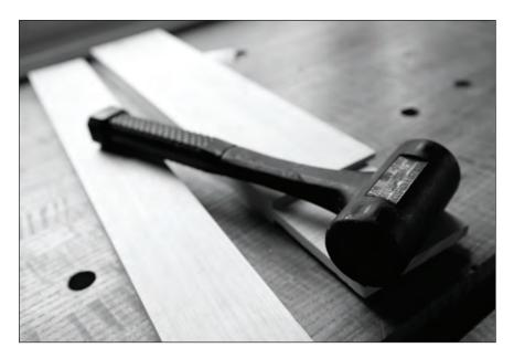
**Dead to me.** The dead-blow mallet is an inexpensive tool that helps you disassemble joinery. It could be moved to the "not necessary list" if you are down to your last \$10.
