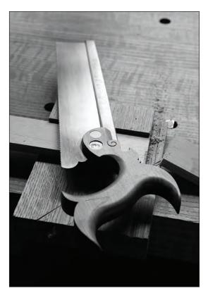
**For accurate crosscuts.** The carcase saw is a tremendous saw for no-compromise cuts when making furniture. It cuts smoothly and cleanly thanks to the fleam on its teeth.
