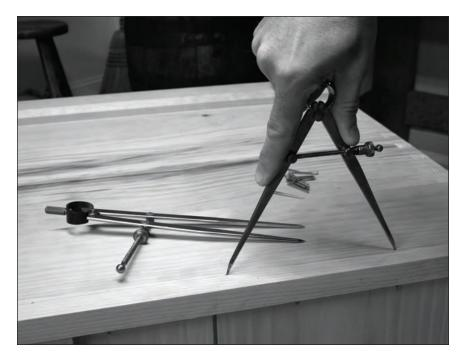
**More nails in your bottom.** After everything is together, I recommend a few extra steps to make the chest nicer. Nail the bottom boards of the shell through the skirt. I spaced the pilot holes with dividers.
