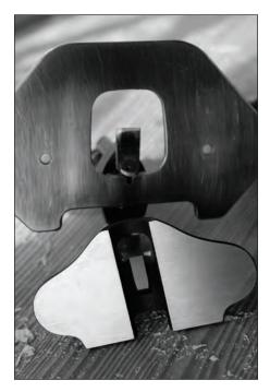
**Open and closed.** An open-mouth router gives you more visibility during the cut. A closed-mouth router allows you to work on narrow edges. If I had to have only one, it would probably be the closed-mouth router.
