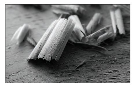
**Thick is better.** When you work across the grain, you can take a monstrous bite. In soft woods, I can rip 1/16" off in a single pass.
