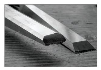
**Bad bevels.** Here you can see the difference between a poor modern tool with its buck-tooth side bevels – called "lands" – and a proper tool for woodworking.
