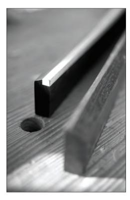
Truth-tellers. Winding sticks are one of the most powerful measuring tools you own. They are second only to your eyes, which are pretty good at spotting some twist. Winding sticks can find almost any twist. black to help the camera see how my winding sticks work. These winding sticks are super-accurate and butt-ugly.
