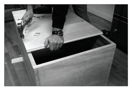
**Fixable.** By securing the bottom with nails instead of a fancier joint, you are making the chest easier to repair in the future. Bottom boards can rot.
