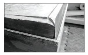
**Fragile seal.** The thin rabbet below the lid makes for a fragile dust seal, which has split off in several places.
