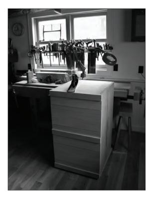
**Tried and true.** With the carcase assembled, you can true up all the proud bits, such as the bottom boards, the battens and the ends of the tail boards. A try plane has the mass and momentum to do this job with ease.
