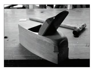
wood is cantankerous. diagnosing problems with wooden-stock planes can vex beginners. Is the problem with the sole? The wedge? The abutt-Experienced ments? woodworkers can hone in on the problem in short order, however, And once revealed, the
