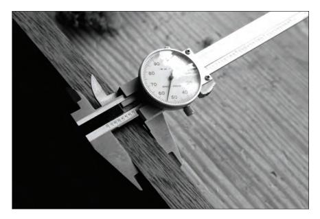
**Pinch in.** As much as I have tried to wean myself off this tool, I'm afraid it's hopeless. I use it all the time when dimensioning stock because I find the dial easier to deal with than fractions.
