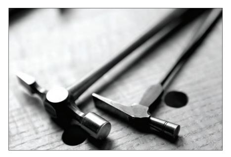
**A woodworking hammer.** While claw hammers are mostly for carpenters, the cross-peen hammer is for us. The peen helps start nails and is ideal for adjusting plane irons, too.
