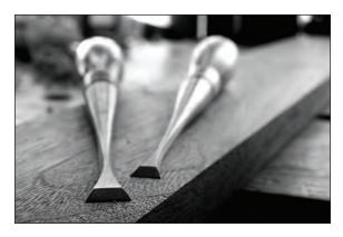
angled at 14°, so my chisel needs to have its long edges ground back at 15° or slightly more. This allows me to get the corner of tool into the corner of my joint.
