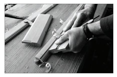
nutty world of Ohio Tool), let's talk about how to answer the question about your set of planes. Take a hollow plane, a No. 4 plane. Take a ruler and measure the iron's width from tip to tip. That is the radius of the circle it will cut. If it's 1/2" from tip to tip, then the plane will create segments of a 1/2"-radius circle. This allows you to lay out your work on your end grain of both ends of your stock – handy and necessary.
