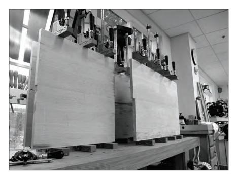
**A good kind of paneling.** I made the front, back and sides of the chest from panels made up of two boards each. Arrange the grain so it all runs the same direction on a single panel.
