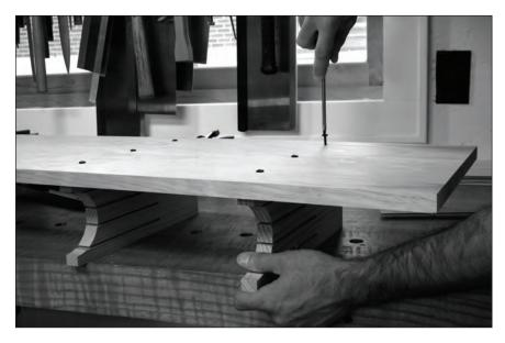
**Screw then slide.** Attach the sawtill parts to the wall using #8 wood screws. Drill your pilot and clearance holes before wedging the wall inside the chest. Note: I countersunk these screws after thinking about the screw heads scraping the sidewalls of my planes.
