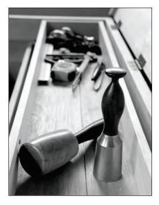
A beater for biter. A good chisel mallet is heavy, compact and packs a lot of punch. Even individual mallets that appear identical can be remarkably different because of differences in the wood.
