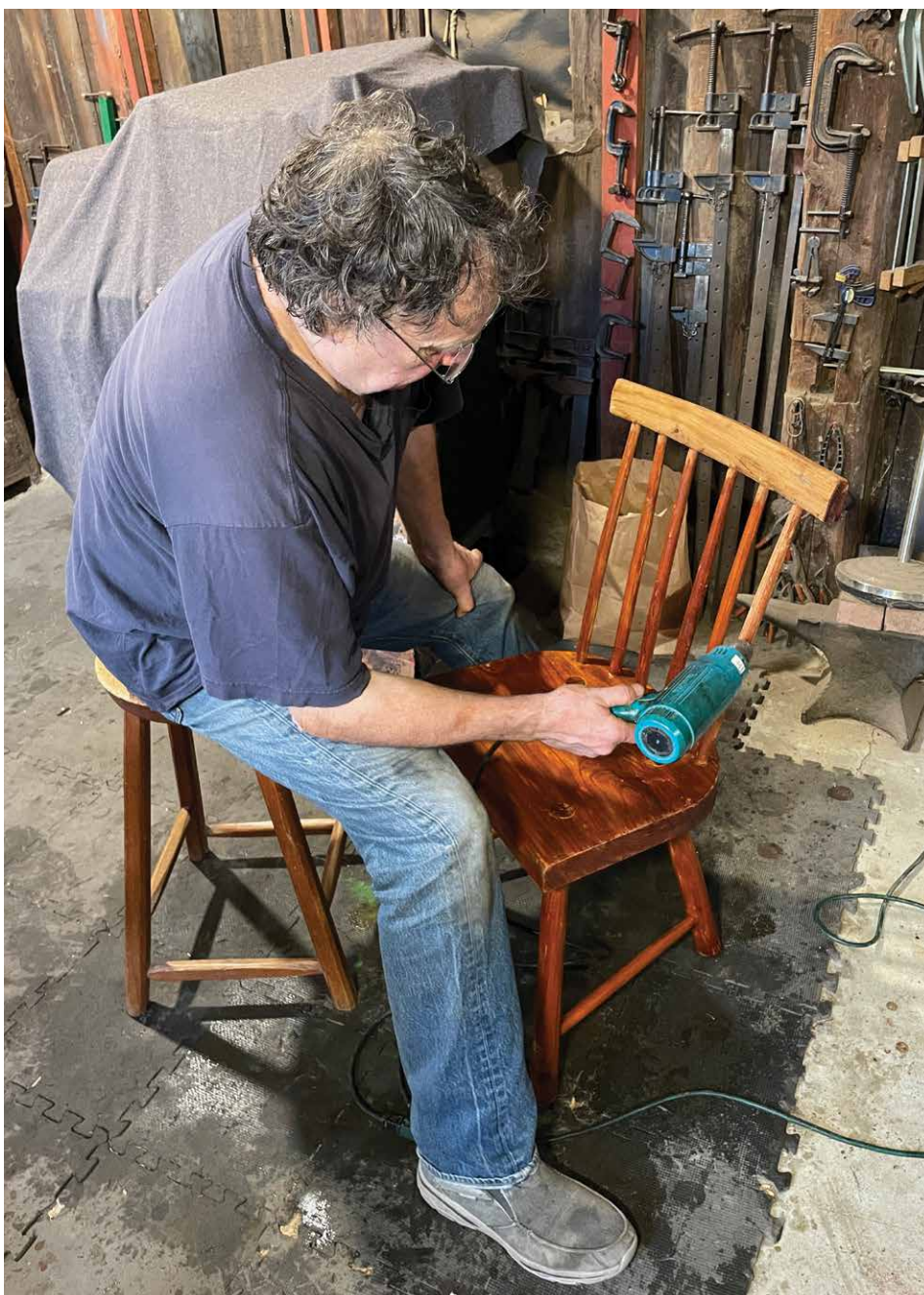
After the coat of hydrogen peroxide, dry it with the heat gun.
