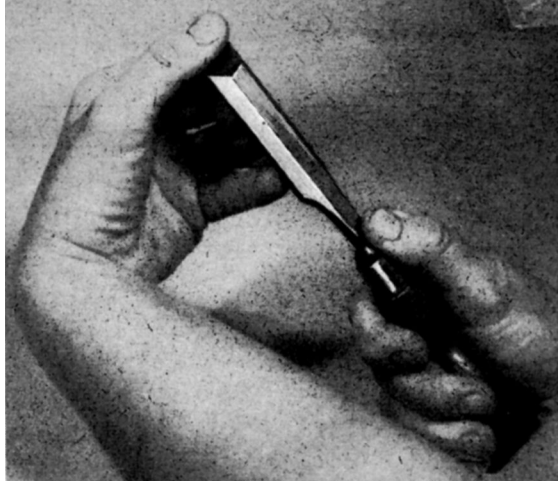
FIG. 1. TESTING AN EDGE FOR SHARPNESS
