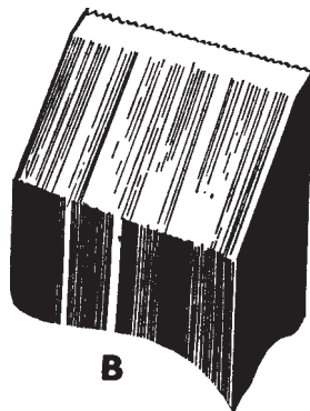
FIG. 5. DIFFERENCE IN QUALITY OF AN EDGE A shows the coarse "teeth" of a ground edge, and B the fine "teeth" of a honed edge
