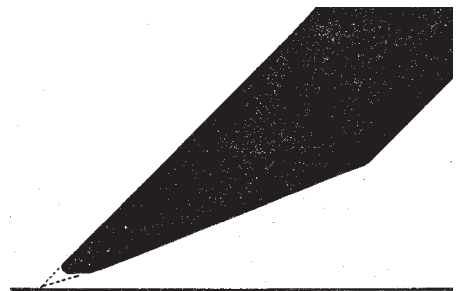
FIG. 4. HOW PLANE IRON LOSES ITS EDGE
