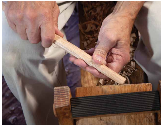
Microchamfer on the shavehorse.
