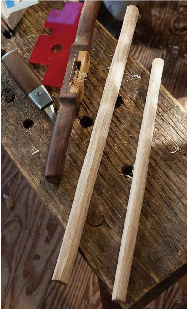
A rough rung (left) and a finished rung (right).
