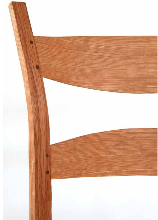
Detail of slats/post. The flat, or relief, shaved on the rear post makes it easier to bend and more comfortable for the sitter than a fully-round post.
