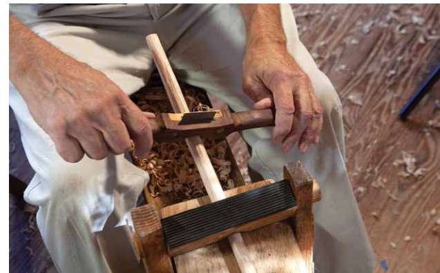
Larry Barrett's round rung scraper. The blade is from an old saw blade with a 3/4"-diameter half-circle at the cutting edge. Shifting it just a little bit one way or the other gets at half the circumference of the rung without repositioning the rung.
