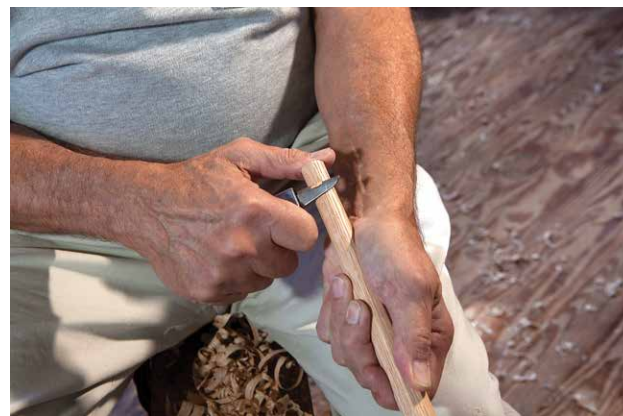
Slicing off the radial side of the tenon. Keep your thumb back out of the way as you pull the knife upward.
