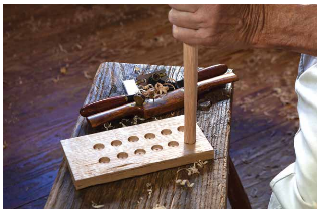
Testing the end of the tenon in the test hole. The resulting bur-nished end gives you a target to shave down to.
