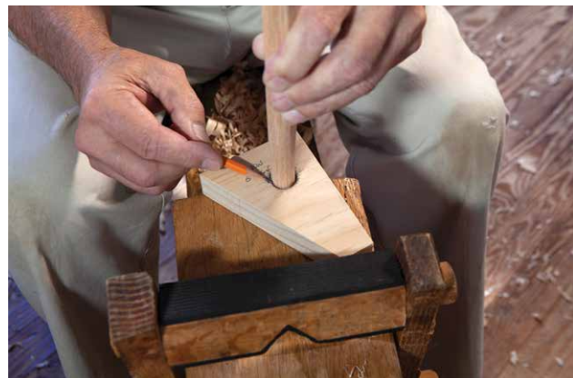
Marking tenon length in a test hole.
