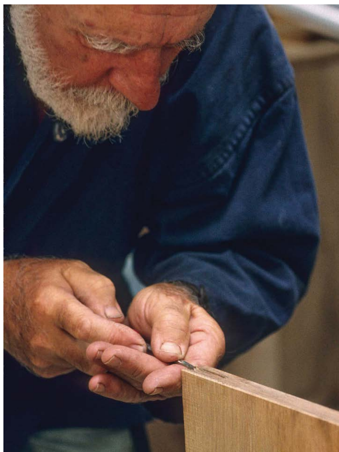
Figure 6: A shot from a series of photographs illustrating the installation of knife hinges, taken in 1995. Photo by David Welter.
