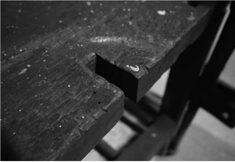
NOTCH IN A SHAKER WORKBENCH, OHIO COLONY NOTCHES SHOW UP IN BENCHTOPS ACROSS CENTURIES AND CULTURES. A WORKPIECE (OR APPLIANCE) CAN BE WEDGED IN PLACE IN THE NOTCH.
