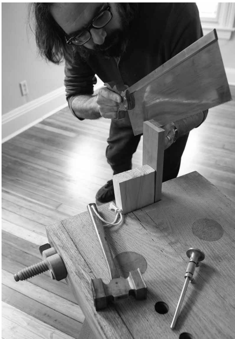
SAWING A TENON USING A NOTCH SOFTWOOD WEDGES PROVIDE EXCELLENT HOLDING POWER.
