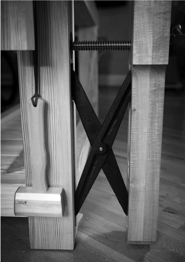
CRISSCROSS REPLACES A PARALLEL GUIDE BASED ON EXAMPLES FROM THE 19TH CENTURY, THE BENCHCRAFTED CRISSCROSS PROVIDES THE OPPOSING FORCE AUTOMATICALLY.
