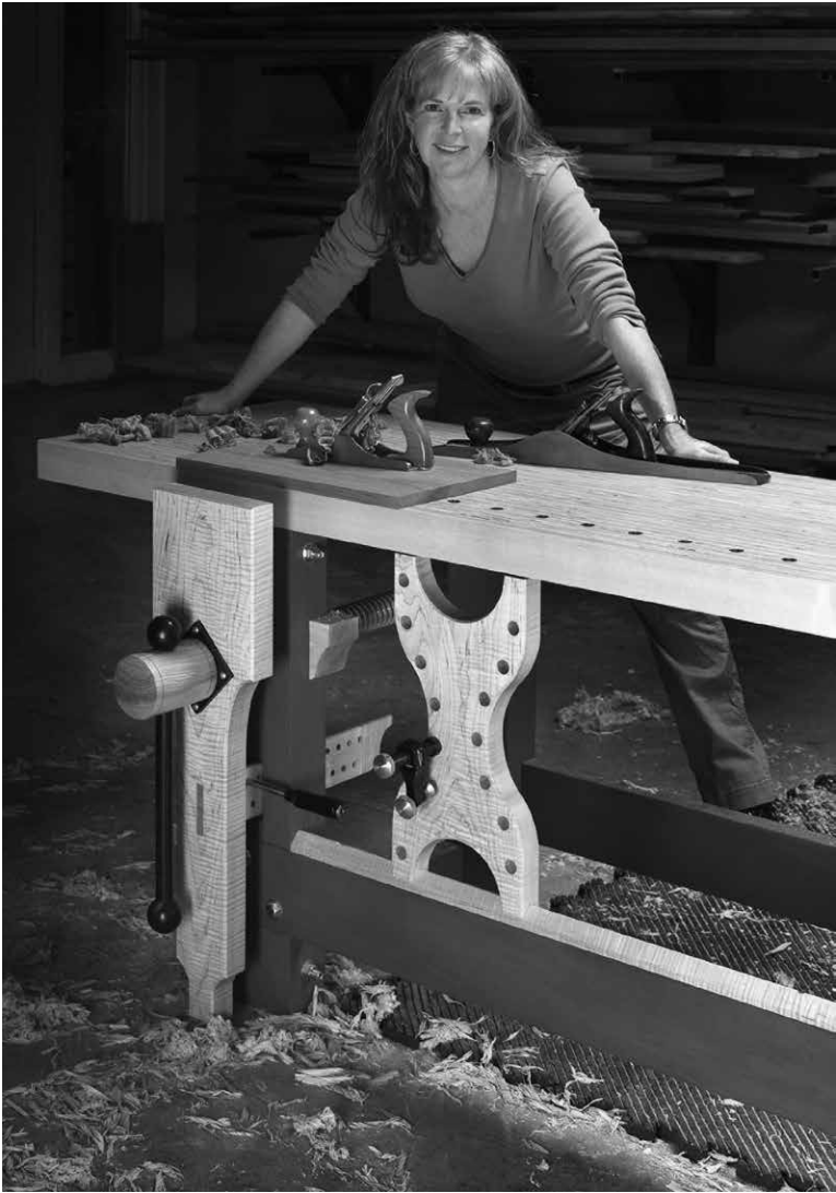
LAMINATED VENEER LUMBER BENCH, 2009 ONE OF MY MORE EXTREME EXPERIMENTS WITH MATERIALS, THIS WORKBENCH USED LVL THROUGHOUT.
