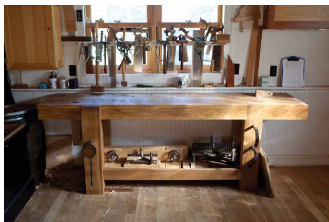
From the past. A simple and solid bench, built to the plan in André-Jacob Roubo's 18th-century "l'Art du menuisier."
