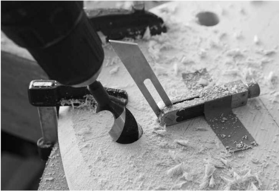
*The tape helps. The vibrations from boring can make your sliding bevel move. And even a little bit of movement makes a big difference in the leg angles. So spring for the tape.*
