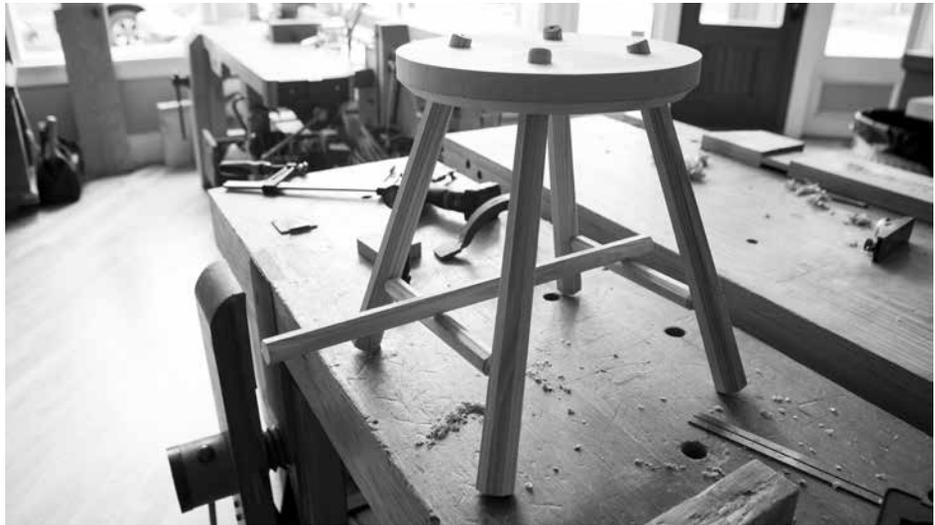
*Stretchers. The side stretchers are installed. And the medial stretcher is laid on top. Now we're ready to drill the mortises for the medial stretcher.*
