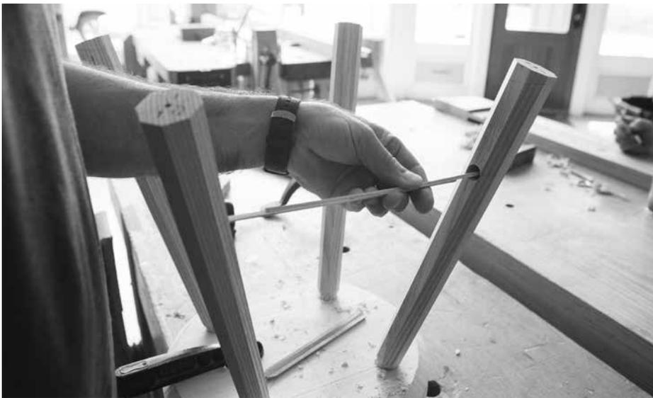
*Tiny test tenons. These thin offcuts determine the final length of the stretcher. Pinch them together and mark across the offcuts. Remove the pieces and reassemble them to determine the final stretcher length.*
