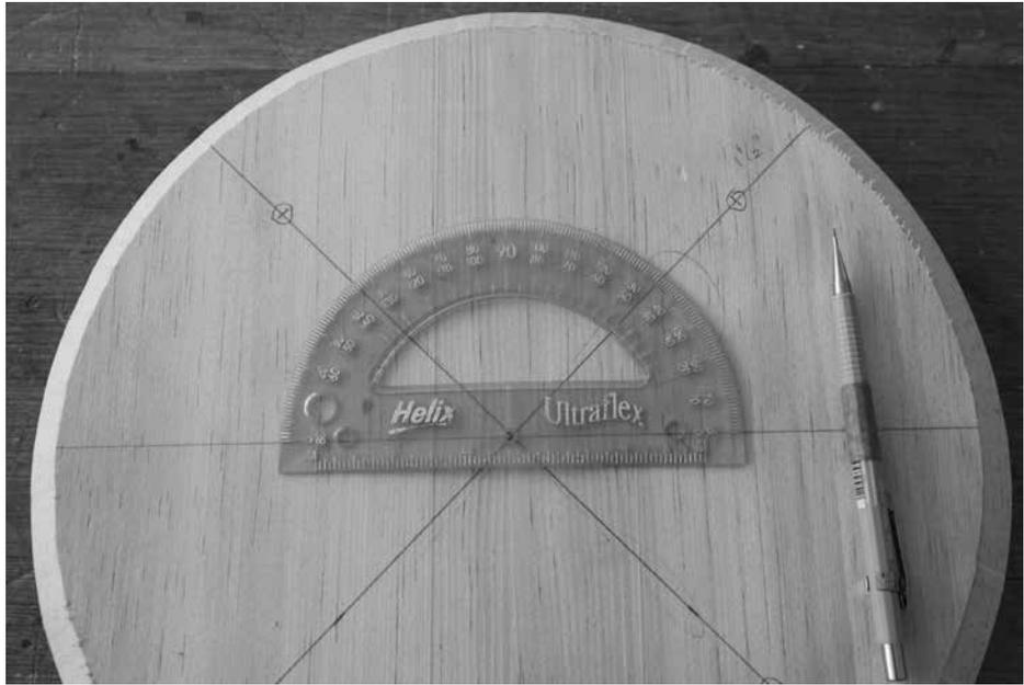
*Good layout. There are 100 ways to do this. Place the protractor on your line and mark the seat at 45° on both sides of the protractor. Connect these marks to the center-point. And done. Perfect.*
