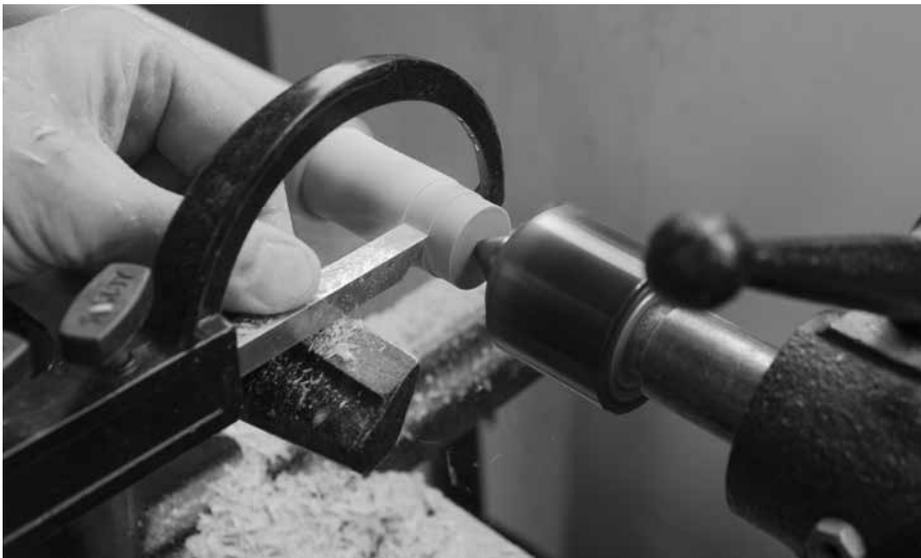
*Perfect tenons. The sizing tool lets you cut tenons within .001". The tooling works just like any standard parting tool.*
