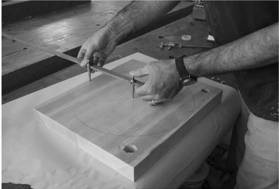
*Around & around. Here I'm marking out the diameter of the seat. Note the two holes in the corners of the blank. These are test mortises that will allow me to test the fit of the tenons on the legs. Waste not, blah blah, blah.*
