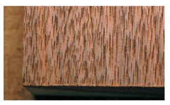
5–35. The scribe line marked on the edge is revealed on the face by planing. Note the fuzzy-looking inner edge.
