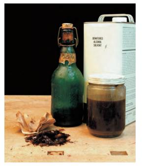
5–42. The products and materials needed for a shellac finish include shellac flakes, a jar of shellac stock solution, an applicator bottle with diluted shellac, grain or denatured alcohol, and an applicator cloth.
