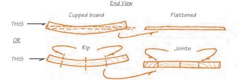
5–13. Above is a cupped board that has been left intact and then flattened. Below is a board that has been ripped into staves that are individually flattened and then rejoined. Note the difference in final thickness.
