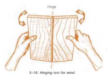
remains firm, or if there is any rocking within the joint betraying the presence of a wind. If it feels firm, the board is in good shape. If a small amount
