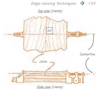
5–23. Proper alignment of clamp and boards.
