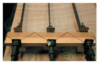
5–21. Forty-five-degree lines have been drawn across the face of the board to approximate how many clamps to use when edge-joining boards.
