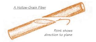
5–7. If a board has run-out, the hollow fibers of an openpored wood are cut obliquely at the surface. The point of the resultant teardrop shape indicates the planing direction.
