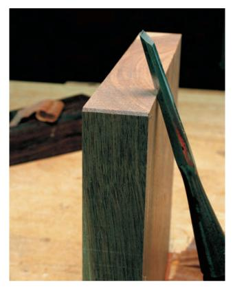
5-38. Chamfering the corner of the board.
