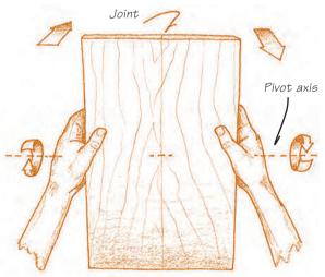
5–15. Pivoting test for tight board ends.
