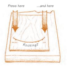
5–30. Checking a surface for a widthwise hump.
