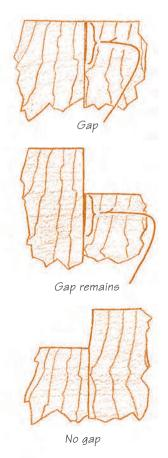
5–17. Offsetting ends to identify a board with a defective end.
