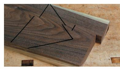
5–18. Aligning grain and indexing with a line. Notice the offset of the pieces at the end of the joint.
