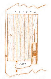
5–31. Correcting a widthwise hump.
