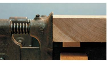
5–22. Aligning the centers of the thickness of the board and the clamp screw minimizes skewing of the joint during glue-up.
