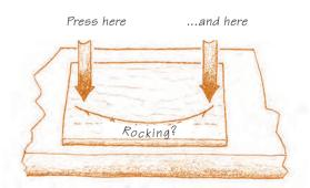
5–28. Checking a surface for a lengthwise hump.
