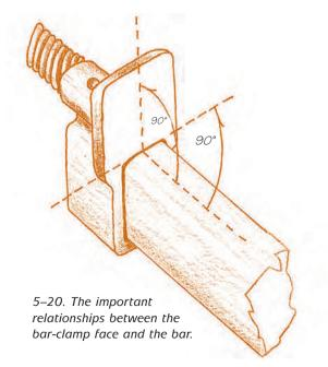
The faces of the clamp heads should be flat, smooth, and square to the bar in both directions that is, in line with and across the length of the bar (5–20). Lumpy or misaligned clamp heads exert pressure at an angle to the bar, skewing the boards as pressure is applied. The effect is greatly magnified when glue lubricates the joint. If the clamps need attention and you cannot do the work, have it done by a machinist.
