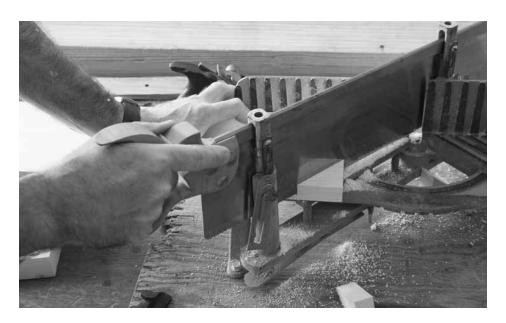
Clip the corners. This old miter box is handy for angled cuts that have to be repeated several times. These tools are common in the used tool market as they were popular among garage woodworkers and carpenters before the age of electric miter saws.
