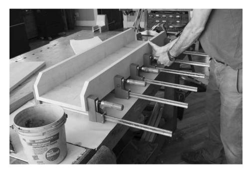
Glue the 'U.' Tight joints between the seat and aprons ensure the bench will look good and last a long time. Clamp the parts together, adjust them as needed to ensure they are flush and clean off the glue. Then wait for an hour before removing the clamps.
