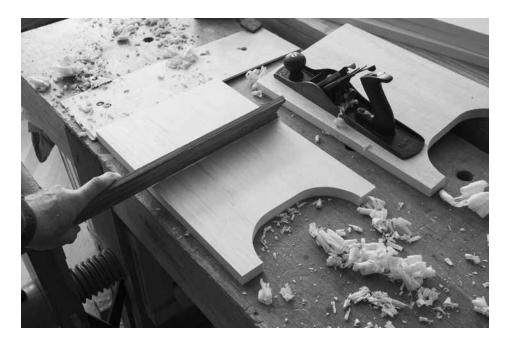
Get it flat. Here I'm working on the interior surface of a leg panel. It needs to be flat so it meets the shelf without a gap. But it doesn't have to be beautiful because it's not very visible. So a little tear-out or a few plane tracks aren't going to matter.
