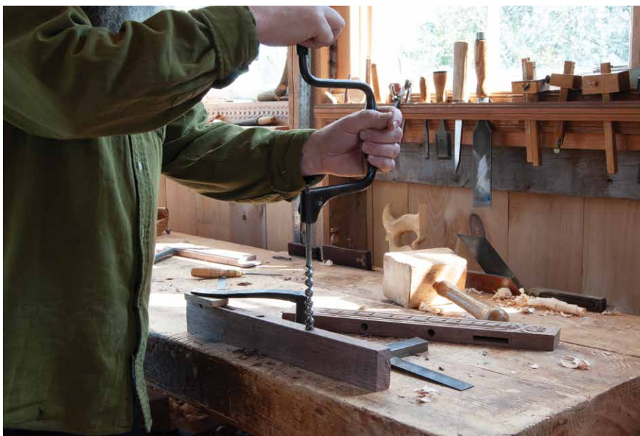
Fig. 9.3 I used a small square to line up the auger bit, then set it out of the way for boring.
