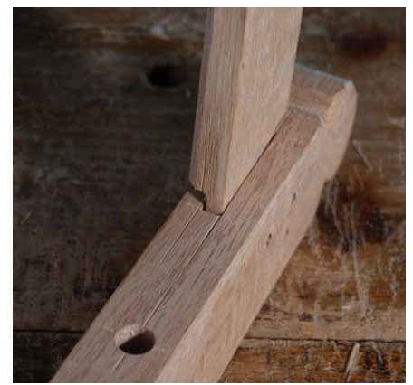
Fig. 9.5 A barefaced tenon, shown from the back. This is a common joint in joined chairs. I used it here to help lighten the bookstand. Or to add variety to my narrow joinery repertoire.
