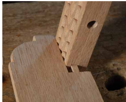
Fig. 9.7 The shelf entered into the stile. See how the "lipped" section fits in front of the stile.
