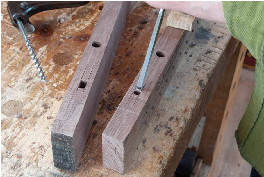
Fig. 9.2 Careful paring with bench chisels will get this mortise trimmed to the proper size, without crushing the surrounding wood.
