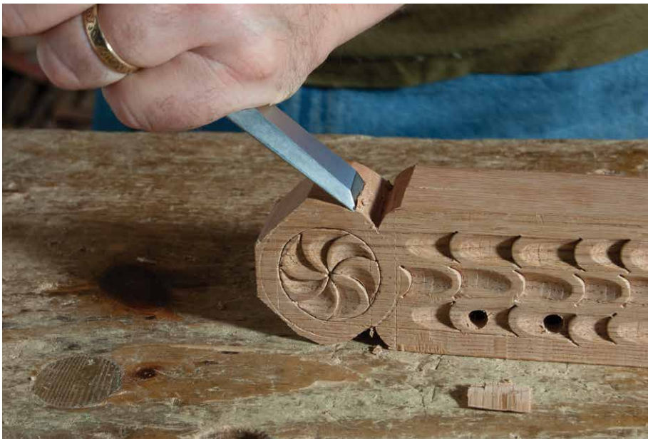
Fig. 9.4 A simple way out: Saw facets around a scribed circle, then pare it round with a chisel.
