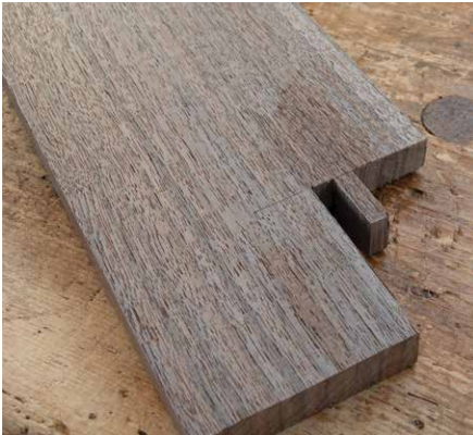
Fig. 9.11 The finished joint before trimming the ends of the shelf.
