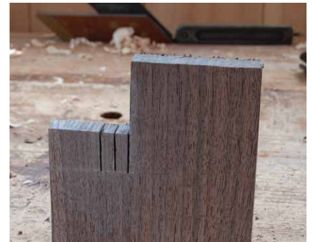
Fig. 9.8 Three rip cuts define the lipped tenon. I made a cut across to bring the tenon to its finished length.
