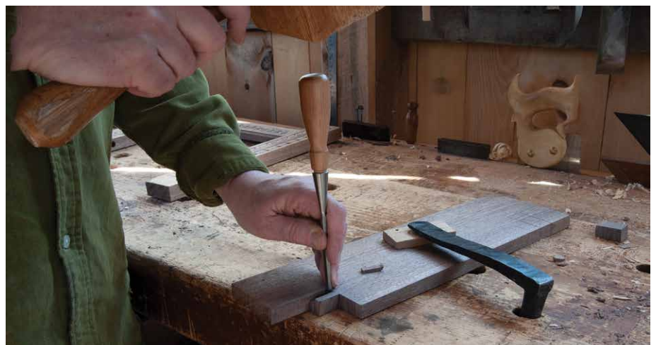
Fig. 9.9 I've cut the rear shoulder out of the way. Now chop out the waste between the tenon and the shelf.
