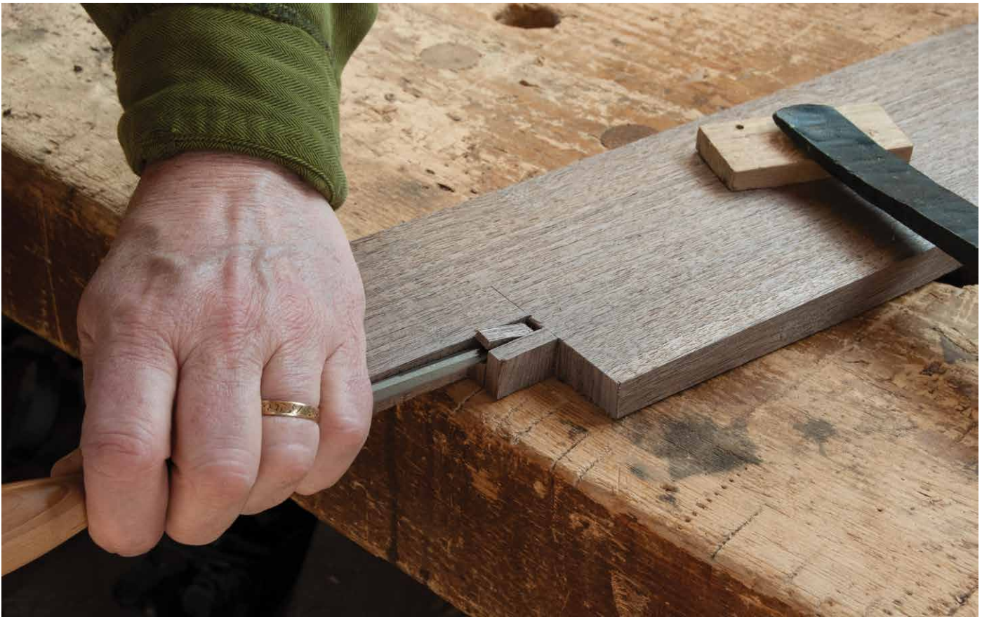
Fig. 9.10 Alternate between the vertical chopping and breaking out the waste.
