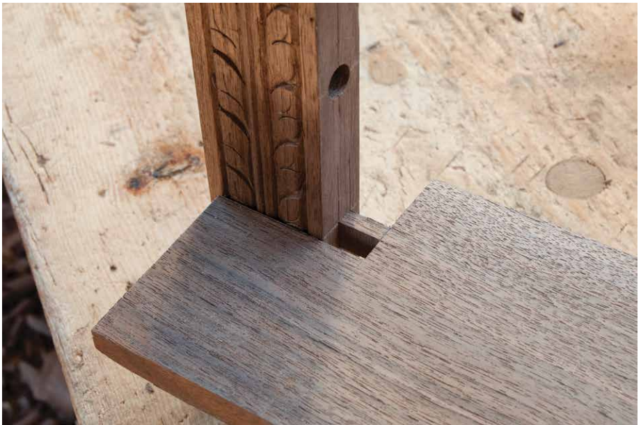
Fig. 9.12 Test fit in the stile.
