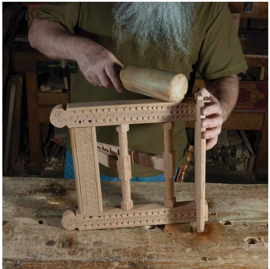
Fig. 9.13 A very simple assembly, just the top rail and the shelf are critical. The middle rails need to be loose.
