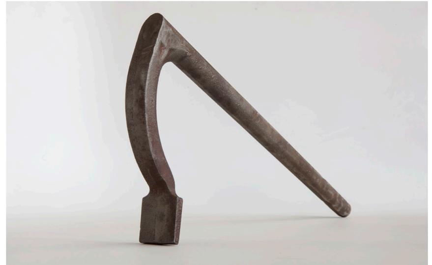
Crucible holdfasts are unlike many mass-manufactured holdfasts made today and require careful fitting to your benchtop for the best performance. This short tutorial guides you through the fitting process so the holdfast will grip tightly in even the thickest workbenches, and it will work even when its pad is 6" (or more) above the benchtop.
