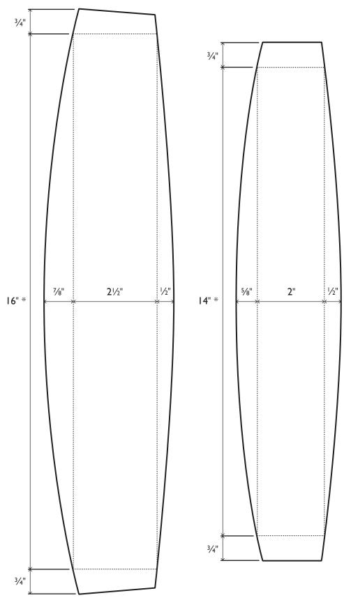
All units in inches One-half scale \* Note: lengths shown are typical, but will depend on the actual flare angle of the back posts
