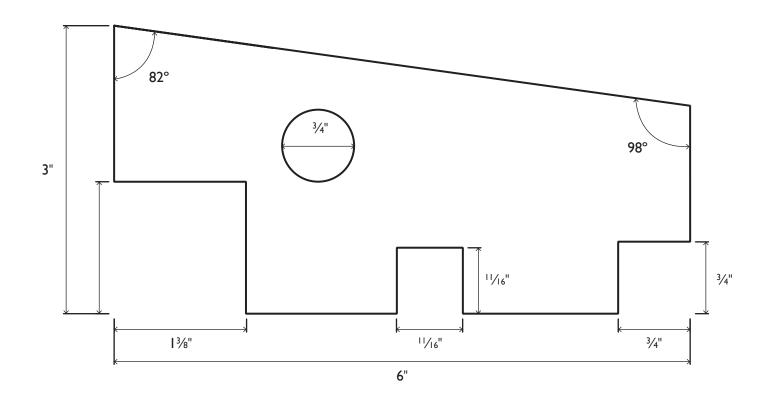
Rung and post gauge Make a Chair from a Tree Suggested dimensions and devices
