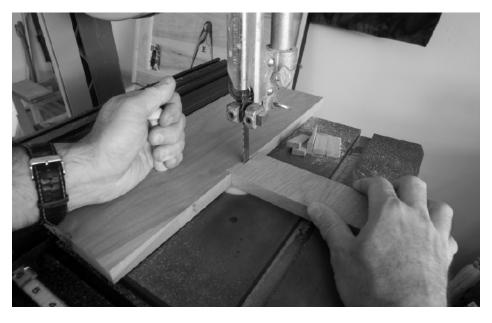
With a fence. For this jig, you need a fence on your band saw (or clamp a piece of stock to your table). The jig is a block of wood with a wedge-shaped notch cut into its side. The jig passes between the fence and the blade. Press your wedge wood into the notch, push the jig forward and cut a wedge free.
