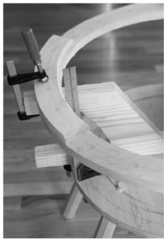
Here. This is where I like the back of the armbow to go. Its inside edge lines up with the outside edge of the seat. The square shows this relationship clearly.
