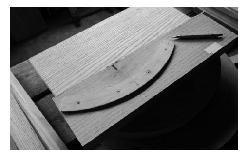
Around the knot. Your curved components will be stronger if the grain is curved. Look for curved grain around knots and from boards that came from the base of the tree in particular.
