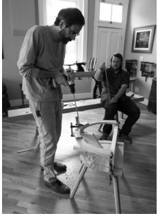
The jig is down. Here's the armbow jig in action. The front piece supports the hands. The back piece supports the remainder of the armbow. This jig – rough as a cob in an outhouse – provides unparalleled drilling stability.
