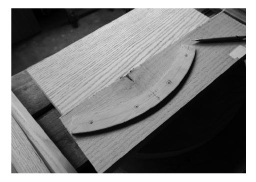
Sawing for strength. The grain bends a little around this knot. I wish it bent more, but this what I had on hand.
