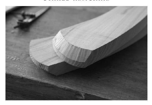
Soft hands. The bevel on the underside of the hands is a quick addition to the armbow but makes a huge different to how it looks.
