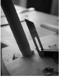
Ream it. Chuck a reamer into your brace or electric drill and ream the mortise.
