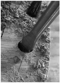
A handy notch. This V-shaped notch tells you when to stop drilling the mortises in the seat of the chair.
