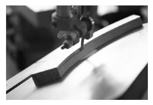
Bevel the doubler. The 30° bevel on the front of the doubler avoids some lower back pain for the sitter. Set the table of your band saw to 30° and make the cut. (Note: The pencil line on the stock shows what a 45° cut would look like.)
