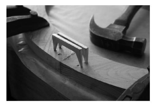
Pinch it good. Put glue on the ends of the hands and drive in the pinch dogs with a hammer to draw the bits together. Note the wax paper below the hands.
