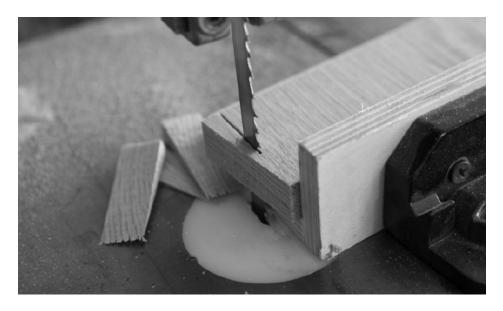
Cut and flip. The advantage to using the miter gauge is it's faster. The downside is that your fingers get closer to the blade at the end of the process.
