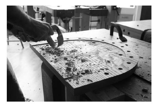
Across and angled. The grain in this seat runs from left to right. So, when I scorp the material, I work across the grain but have the cutting edge skewed slightly toward the right. This helps control tearing. As the saddle gets deeper you'll have to adjust the tool to always work downhill.
