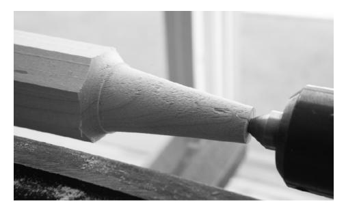
Tapered on the lathe. The conical tenon is 3-1/4" long with a cove at the shoulder. The base of the tenon is about 1-1/16" diameter.
