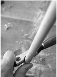
A little compression. The pliers press and burnish the wood a bit. When the tenon encounters the warm hide glue (which is nearly 50 percent water) it will swell up to its full size and lock the joint.
