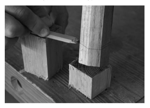
An artificial floor. Think of the scrap as an artificial floor. Here I've planed a carpenter's pencil in half and have it held tightly to the scrap. Mark all around all four legs.
