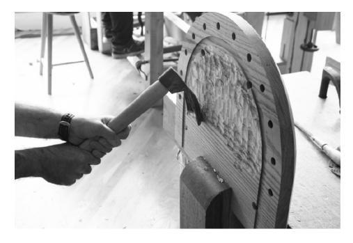
A is for Adze. Adzes are an important part of the pre-industrial method for processing lumber. You can also use it to scoop out a seat, as shown here.
