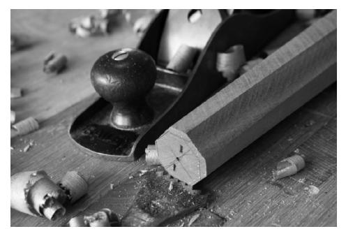
To the line. Tapering legs with a sharp jack plane is simple. Work to the lines marked on the feet and try to keep the facets consistent around the leg.
