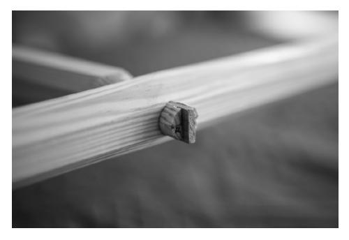
Wedged. Here you can see how the wedge is 90° to the grain of the stretcher. Had I oriented it parallel to the grain, the stretcher would have been a goner.
