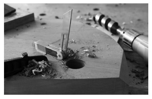
Quick joinery. Tapered mortises and tenons are not tricky to make as long as you have tools, a tenon cutter and a reamer, with matching angles.
