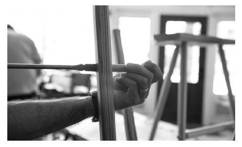
The backup plug. The 5/8" dowel prevents the spade bit from wrecking the mortise as it drills from the outside of the leg.
