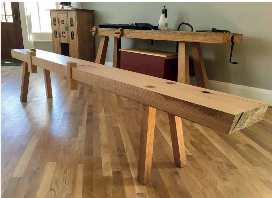
Figures 1.8 & 1.9. Well made. This Roman bench is a copy of the oldest surviving bench I know of – a circa 187 C.E. bench that was pulled from a Roman well in Saalburg, Germany (at top). The dovetail-shaped notches on the long edge were the biggest mystery.
