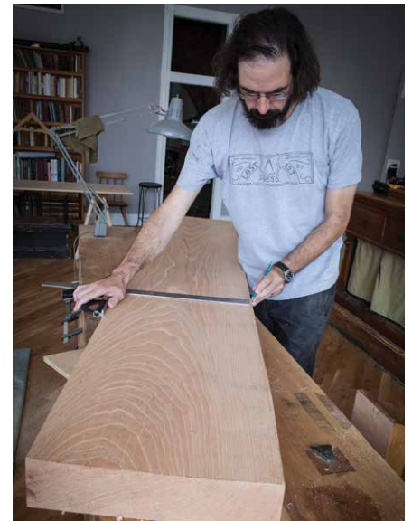
Figure 6.4. Gauge the width. Use a panel gauge or a large combination square to gauge the final width of your slab. The head of the square should run against the true edge.
