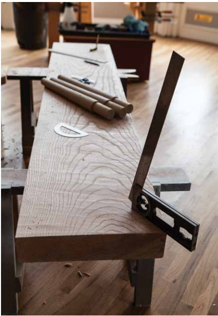
Figure 6.11. Before boring. After I made the model, I confirmed the compound angle looked correct with a large sliding bevel square. You can skip this step if you trust me.
