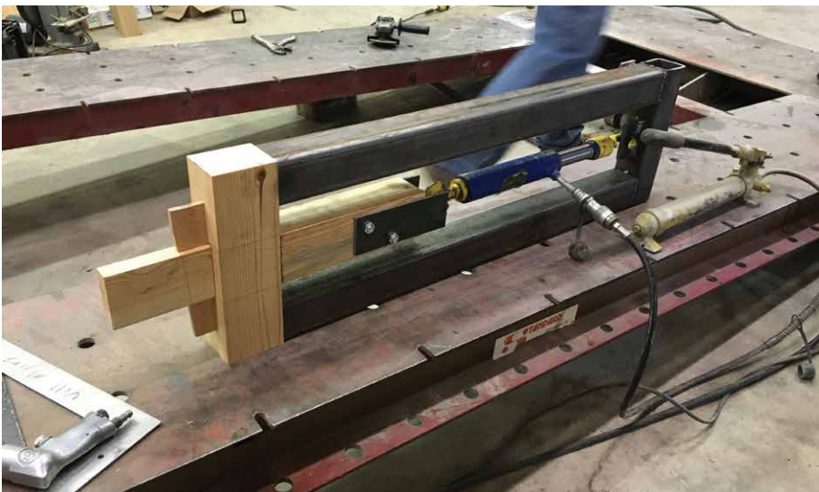
Figure 2.7. Redneck engineering. This ingenious contraption tests how many pounds of force a tusk tenon can withstand. (Tusk tenons are a common workbench joint.) The answer: This joint is well-suited for workbench joinery.
