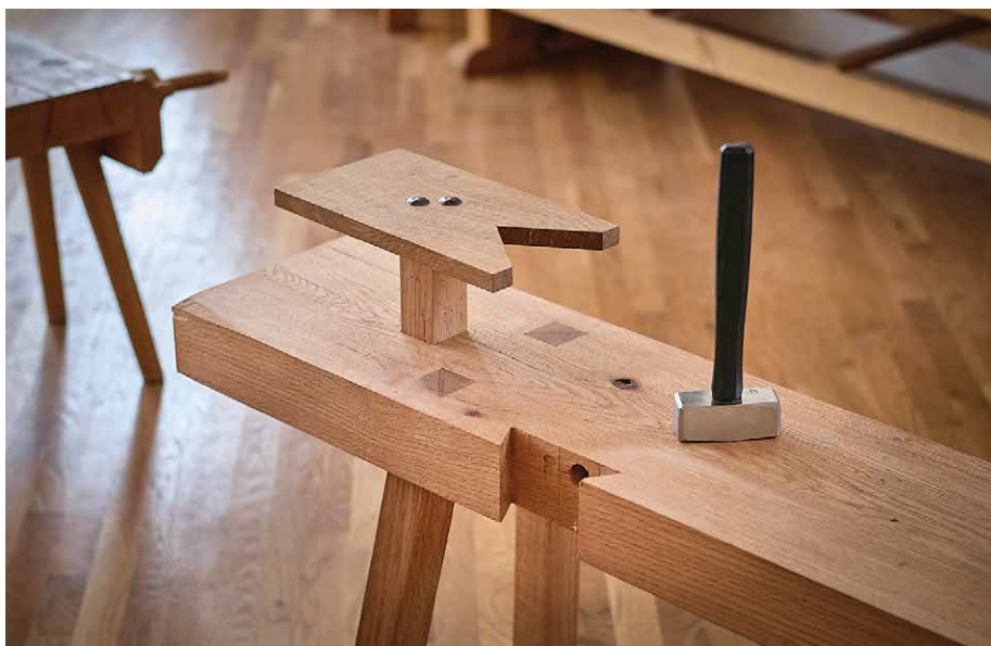
Figure 5.17. The moving palm. The palm is attached to the top of the planing stop with heavy Roman-style nails. It is adjusted up and down with hammer blows.
