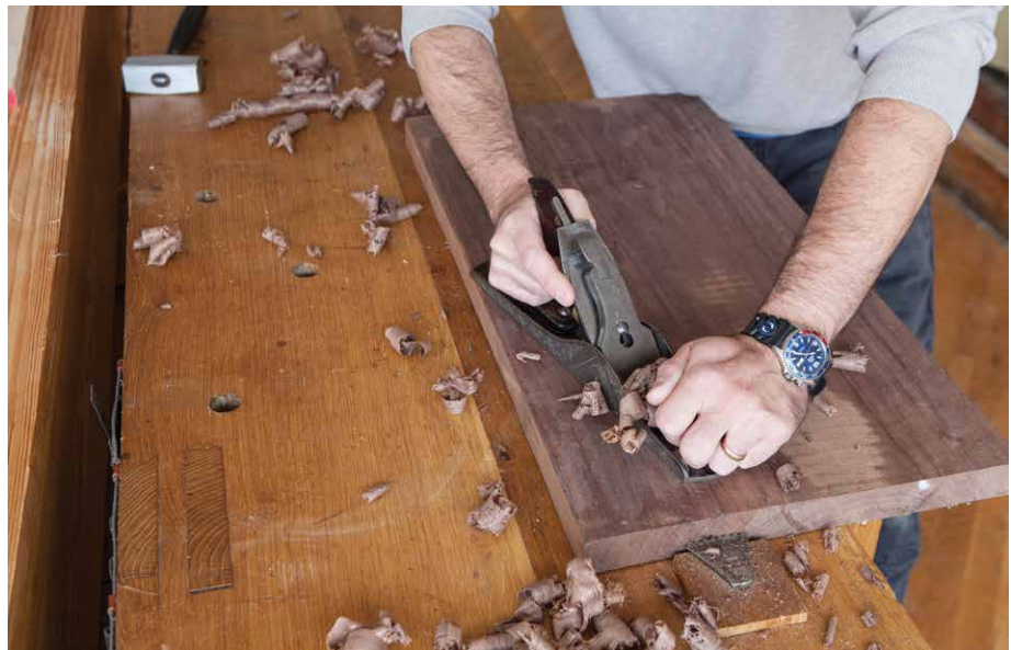
Figures 5.6, 5.7 & 5.8. Immobile but movable. Keep the handplane in line with the planing stop and move the workpiece. As the piece starts to hang off the front edge of the bench, press the rear corner with your hip or extend the jaw of your face vise (if you have one) to help stabilize it.
