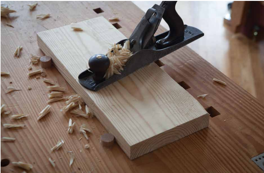
Figure 5.26. Across the board. For short boards, you'll need to shift the work left or right occasionally to keep the board under control. This is not a big deal.
