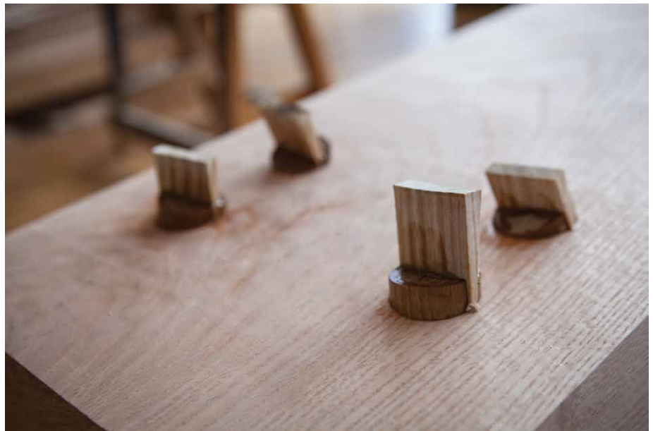
Figure 6.14. Wedge the tenons. Note how the wedges are perpendicular to the grain of the benchtop. This is the typical arrangement when building furniture. In the next chapter, you'll learn another way to do it.
