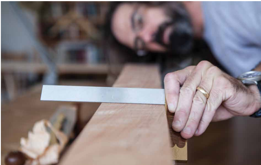
Figure 6.3. All 90°. There are times when square-ness is overrated. This is not one of them. If you make your faces and edges square to one another, it will make the leg joinery easier.
