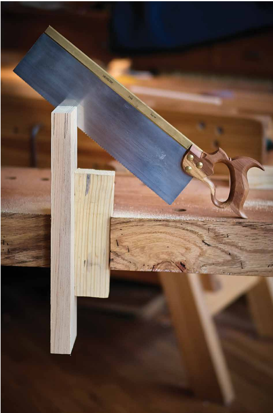
Figure 1.12. Novel notches. Many early workbenches feature simple notches in the benchtop, including one of the benches drawn by Löffelholz. Add a softwood wedge and you have an effective face vise.
