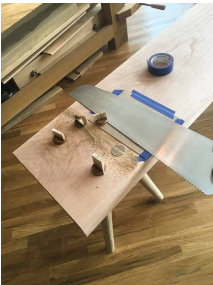
Figure 6.15. One way to do it. My oak legs were incredibly dense. So, I had to break out the full-size crosscut saw. To protect the benchtop from the set of the saw teeth, I taped a thin bit of cardboard to the bench.
