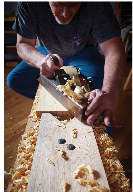
Figures 5.21 & 5.22. Get over it. The palm effectively restrains your work when planing edges and faces. Most of all, the low bench allows you to get your mass right over the cut.
