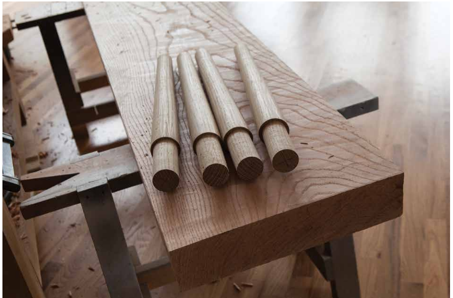
Figure 6.10. The first four finished legs. These are just the right size for a pirate's peg leg. However, I wouldn't want to make that mortise.
