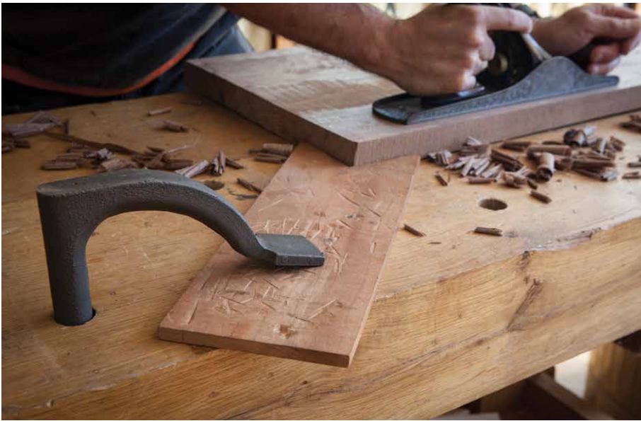
Figure 5.11. A kick to your backside. With the doe's foot behind the work you can plane wide panels parallel to the grain or across it.
