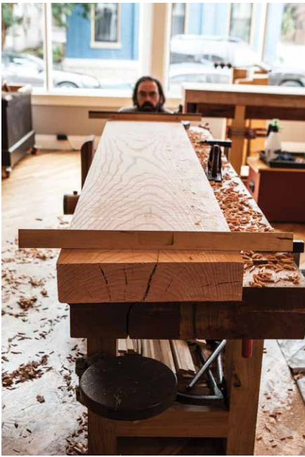
Figure 6.7. Wind out. With large slabs, your eyes can see obvious twisting. But the true test is to use winding sticks.
