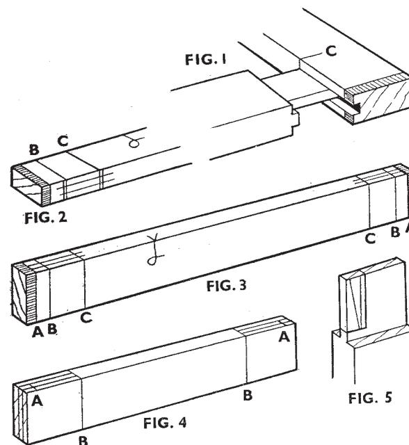
**FIG. 1.** MORTISE AND TENON JOINT WITH SQUARE HAUNCH
