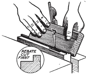
4. CUT REBATE FIRST, USING REBATE PLANE, THEN WORK MOULDING. IF A PLANE IS NOT AVAILABLE, THE SCRATCH CAN BE USED.
