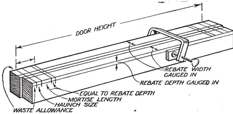
FIG. 3. STILES CRAMPED TOGETHER DURING MARKING OUT
