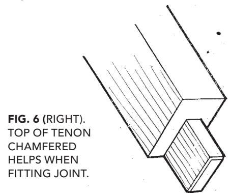
FIG. 6 (RIGHT). TOP OF TENON CHAMFERED HELPS WHEN FITTING JOINT.
