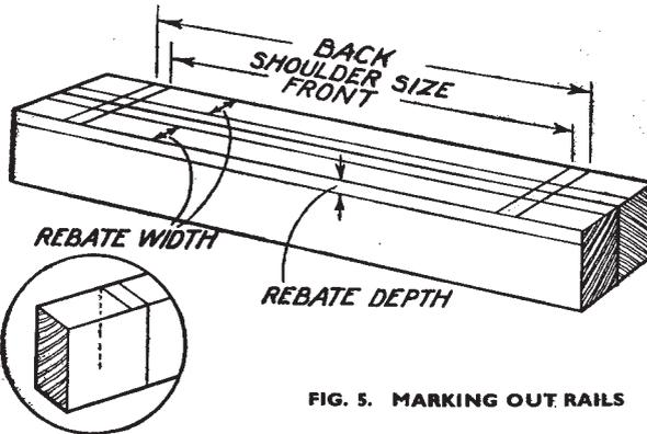
FIG. 5. MARKING OUT RAILS
