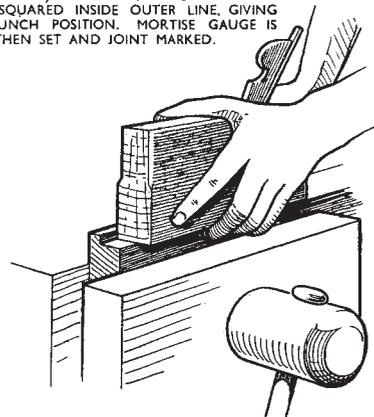
4 WORK REBATE AFTER JOINT IS CUT. FINGERS HELD BENEATH SOLE ACT AS FENCE IF A FILLISTER PLANE IS NOT AVAILABLE.
