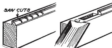
5. TO REMOVE MOULDING AT MORTISE MAKE SERIES OF FINE SAW CUTS
