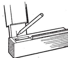
10. MARK PART OF TENON TO BE CUT AWAY, ALSO HAUNCH. MITRE MOULDING (AS IN 7) AND FIT UP JOINT.
