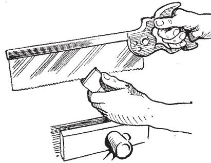
FIG. 2. FIRST OPERATION WHEN SAWING THE TENON
