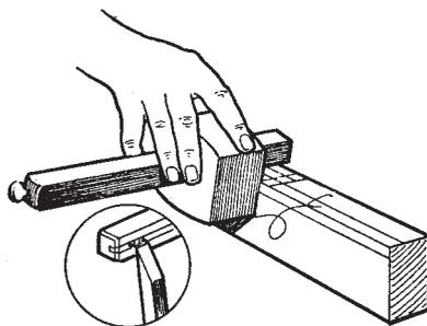
2. SQUARE ACROSS MORTISE POSITION (SEE INSET NO. 3). SET MORTISE GAUGE TO CHISEL WIDTH ( $\frac{1}{2}$  IN.), SET TO CENTRE OF WOOD AND MARK FROM FACE SIDE.
