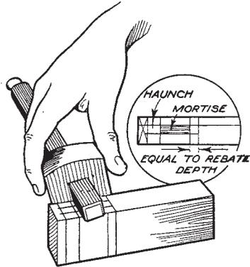
2 MARK OUT MORTISE. FIRST SQUARE OVER-ALL RAIL WIDTH, AND ADD THIRD LINE  $\frac{1}{2}$  IN. (REBATE DEPTH) INSIDE INNER LINE. A FOURTH LINE IS SQUARED INSIDE OUTER LINE, GIVING THE HAUNCH POSITION. MORTISE GAUGE IS THEN SET AND JOINT MARKED.
