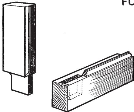
USEFUL JOINT FOR MAKING DOORS AND FRAMES OF ALL KINDS. THE MOULDING IS WORKED IN THE SOLID AND IS MITRED. NOTE THAT THE BOTTOM MEMBER OF THE MORTISE IS LEVEL WITH THE REBATE SO THAT THE SHOULDERS OF THE TENON CAN BE LEVEL. THE MORTISED PIECE SHOULD BE EXTRA LONG, AS THIS MINIMISES RISK OF SPLITTING AND ALLOWS FOR TRIMMING.
