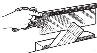
8. SQUARE ROUND SHOULDER MARKS OF RAIL WITH CHISEL, AND GAUGE IN POSITION OF REBATE AND MOULDING. SAW TENON, HOLDING SAW AT WASTE SIDE OF GAUGE LINES. FIRST CUT AT ANGLE IN VICE, THEN REVERSE WOOD, THIS TIME UPRIGHT.
