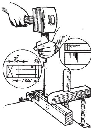
3. FIX WORK TO BENCH, AND PUT THUMBSCREW AT END TO PREVENT SPLITTING. BORE AWAY PART OF WASTE WITH  $\frac{1}{4}$  IN. TWIST BIT, AND CHOP MORTISE. PAPER STUCK TO CHISEL ACTS AS DEPTH GAUGE.
