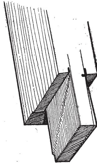
**FIG. 1. BAD FAULTS IN A TENON.** Note how the saw has been taken beyond the shoulder and the tenon lines, the crooked sawing of the sides, the gap at the back, and the unnecessary gauge lines.
