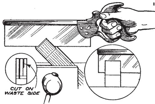
6 WHEN SAWING TENON FIX WOOD IN VICE AT AN ANGLE. AFTER MAKING CUT AS FAR AS DIAGONAL, REVERSE IN VICE, THIS TIME UPRIGHT, AND COMPLETE CUT. NOTE THAT CUTS ARE MADE AT WASTE SIDE OF GAUGE LINES.
