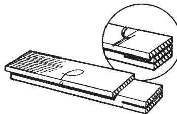
7 AFTER WORKING REBATE CUT THE SHOULDERS WITH FINE SAW. IF SLOPING GROOVE IS CHISELLED AT WASTE SIDE OF LINE, A CHANNEL WILL BE FORMED IN WHICH SAW CAN RUN.
