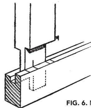
**FIG. 6.** MARKING SET-IN OF TENON FROM MORTISE
