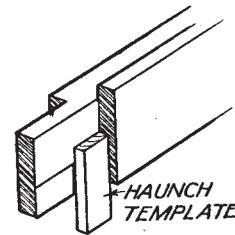
FIG. 7. HAUNCH LENGTH MARKED WITH TEMPLATE
