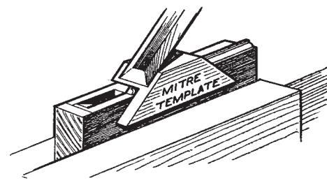
7. TO CUT MITRE ON MOULDING USE THE WOOD MITRE TEMPLATE, HOLDING CHISEL FLAT ON BEVEL AND CAREFULLY PARING. WOOD CAN ALSO BE CUT AWAY AT MORTISE END TO FORM SLOPING RECESS FOR HAUNCH.
