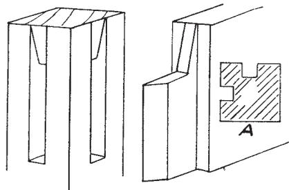
**FIG. 4. BEVELLED HAUNCHES ARE STRONGER IN LIGHT TABLE LEGS**
