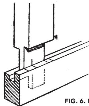
**FIG. 6.** MARKING SET-IN OF TENON FROM MORTISE
