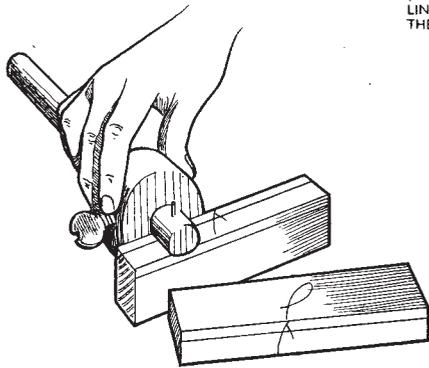
1 HAVING SQUARED UP THE WOOD GAUGE IN THE DEPTH AND WIDTH OF THE REBATE, USING THE GAUGE ALWAYS FROM EITHER FACE SIDE OR FACE EDGE OF WOOD.
