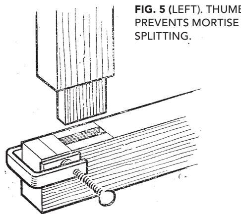
FIG. 5 (LEFT). THUMBSCREW PREVENTS MORTISE FROM SPLITTING.
