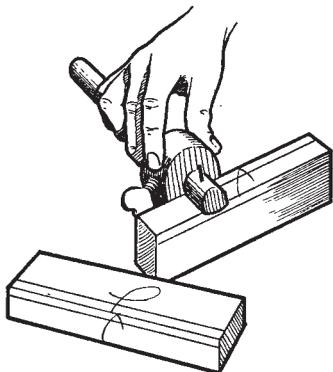
1. SET GAUGE TO  $\frac{3}{8}$  IN. (MOULDING AND REBATE DEPTH) AND MARK BOTH SIDES FROM FACE EDGE. RE-SET GAUGE TO DISTANCE 1 IN. OF REBATE AND MARK FROM FACE SIDE AS ABOVE.
