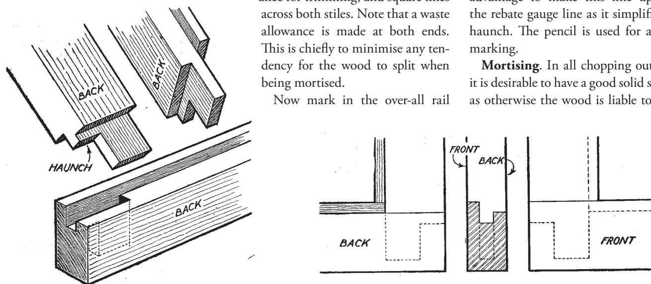
**FIG. 1.** PERSPECTIVE VIEW OF JOINT, AND ELEVATIONS SHOWING ITS PROPORTIONS
