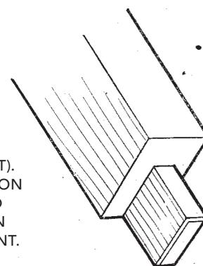
FIG. 6 (RIGHT). TOP OF TENON CHAMFERED HELPS WHEN FITTING JOINT.
