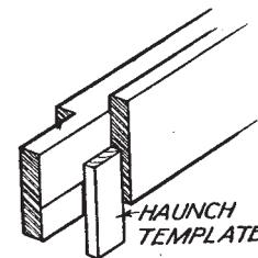
**FIG. 7.** HAUNCH LENGTH MARKED WITH TEMPLATE
