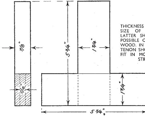
THICKNESS OF TENON IS FIXED BY SIZE OF MORTISE CHISEL. THE LATTER SHOULD BE AS NEAR AS POSSIBLE ONE THIRD THICKNESS OF WOOD. IN THIS CASE  $\frac{3}{8}$  in. IS NEAREST TENON SHOULD MAKE HAND-TIGHT FIT IN MORTISE, AND SHOULD FIT STRAIGHT FROM SAW
