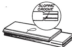
9. WORK REBATE AND MOULDING (SEE 4), AND SAW SHOULDERS, FIRST CUTTING SLOPING GROOVE TO FORM CHANNEL FOR SAW.
