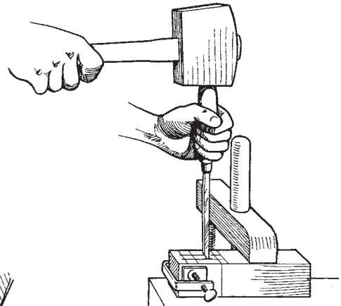
3 MUCH OF THE WASTE CAN BE BORED AWAY WITH BIT SLIGHTLY SMALLER THAN MORTISE WIDTH. THUMBSCREW ON END HELPS TO PREVENT WOOD FROM SPLITTING WHEN MORTISE IS CHOPPED WITH CHISEL. CHOP MORTISE HALF THROUGH FROM EACH SIDE.
