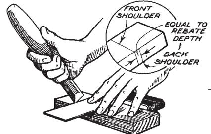
5 MARK BOTH SHOULDERS ON EDGE WITH PENCIL. AFTERWARDS SQUARE EACH ACROSS ITS SIDE WITH THE CHISEL.
