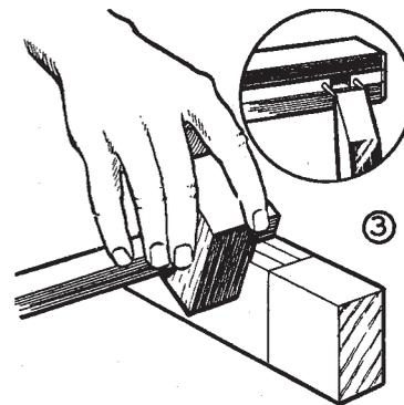
6. Mark tenon with gauge from face side. Fix wood at an angle to start cuts and hold saw to waste side of gauge line. Reverse and fix upright to finish (inset).
