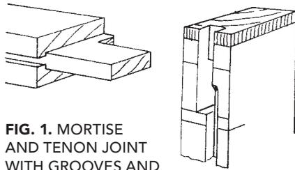
**FIG. 1. MORTISE AND TENON JOINT WITH GROOVES AND SQUARE HAUNCH**
