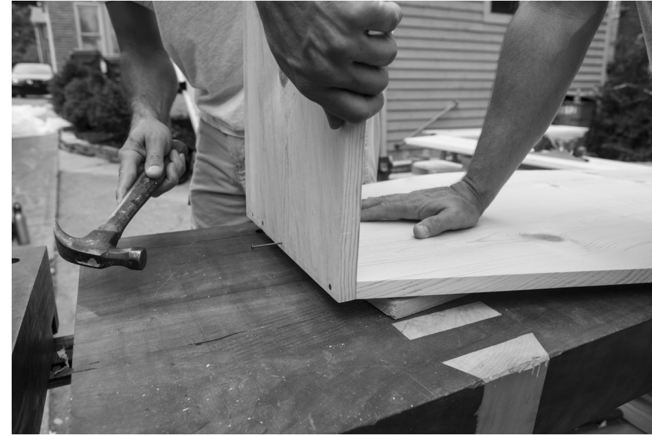
Prop it up. Hasluck suggests propping the bottom up on a scrap to make it easier to nail on the headboard and footboard. Good call.
