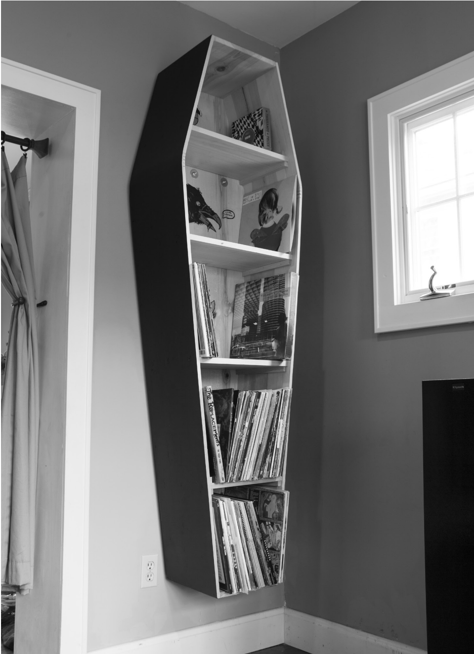
What's important. With a few removable shelves, you have a spacious bookcase that can hang on a French cleat attached to the wall. The shelves rest on nailed-on cleats. The French cleats are bolted to the case so the unit will hold a lot of weight.
