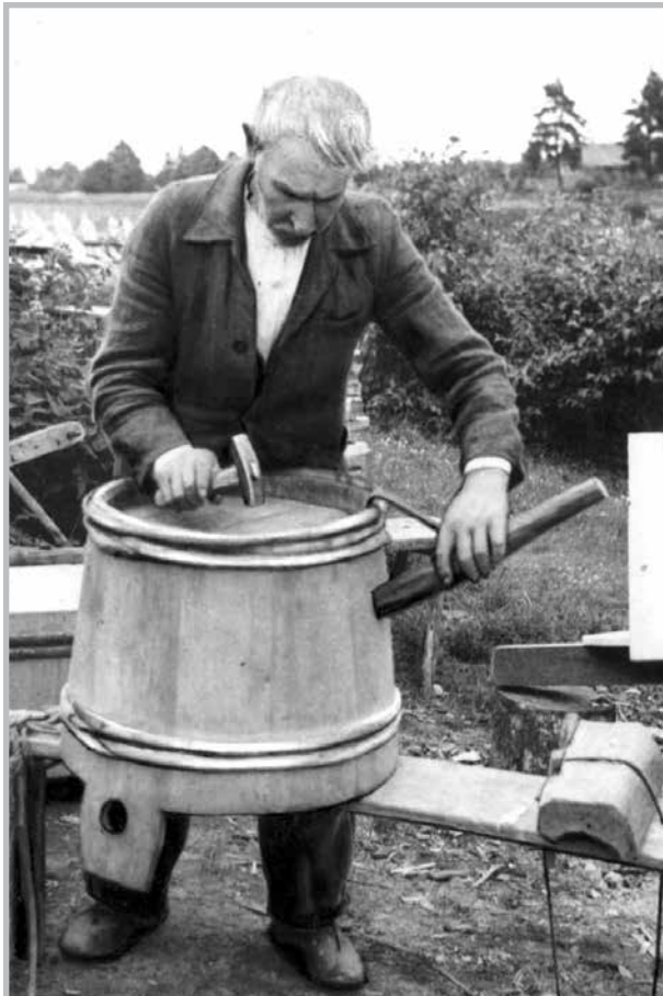
FIG. 103. Hooping a tub. Avinurme, Vadi village, Photograph by the author, 1947. Photo library 1089:71.
