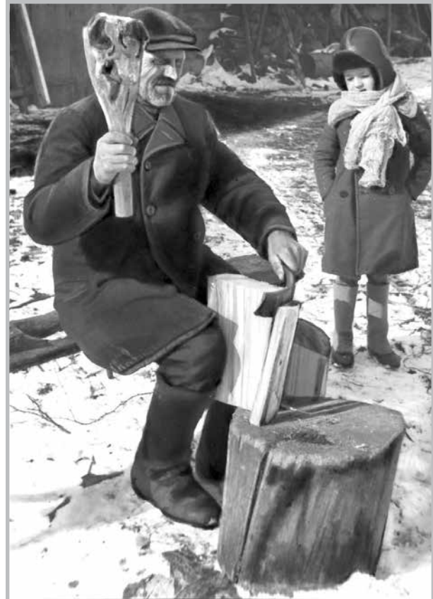
FIG. 92. The trunk being split with a curved froe, Avinurme Enniksaare village, photograph by G. Ränk, 1939. Photo library 836:14.
