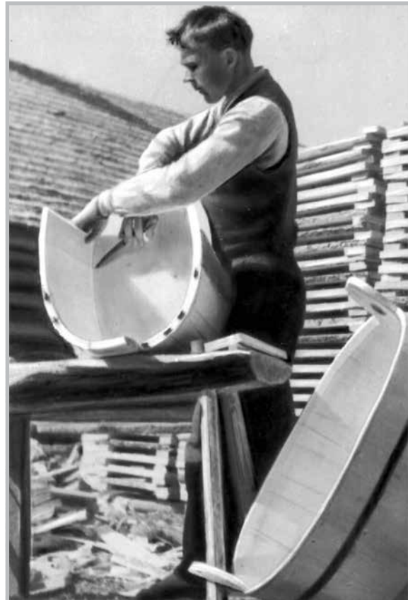
FIG. 95. Marking groove lines on boards. Avinurme. Photograph by J. Triefeldt. Photo library 1116:82.
