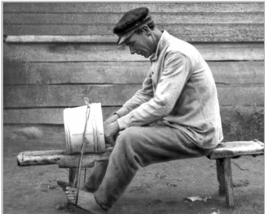
FIG. 106. Cleaning out piggin with drawknife. Avinurme, Karusoo village. Photograph by author, 1947. Photo library 1089:42.
