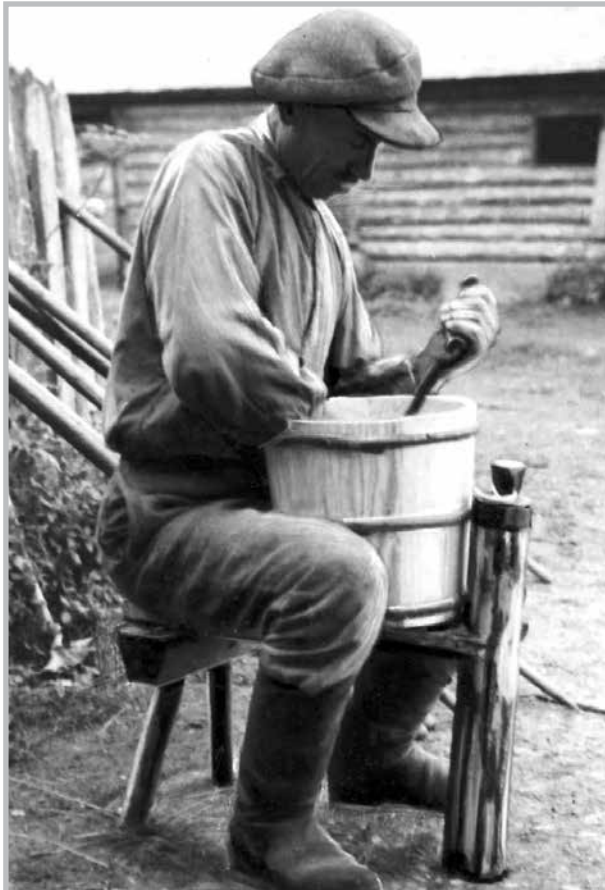
FIG. 114. Cleaning inside of barrel with specially shaped planing knife ( vintrik ), Avinurme, Vadi Village. Photograph by author, 1947. Photo library 1089:76.
