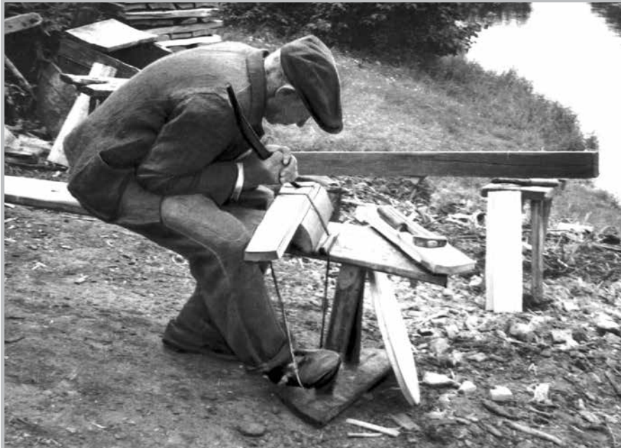
FIG. 96. Grooving on a grooving stool. Avinurme, Vadi village. Photo by author, 1947. Photo library 1089:68.
