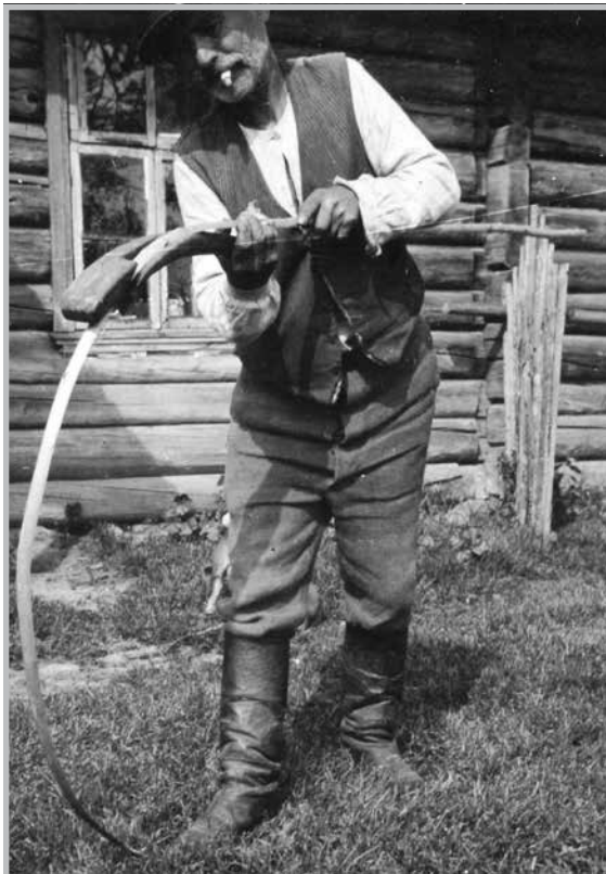
FIG. 101. Bending hoop with windlass, Avinurme, Kõrve village. Photograph by author, 1947. Photo library 1089:91.
