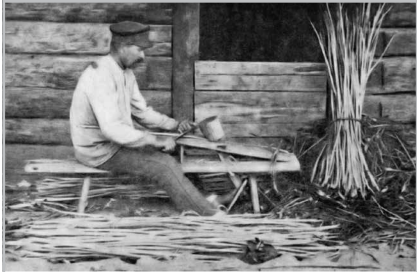
FIG. 100. Cutting hoops on cooper's bench, Avinurme, Piilsii village. Photograph by E. Vittoff, 1921. Photo library 439:313.
