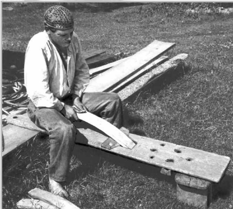
FIG. 111. Bending boards for barrel staves, Avinurme, Enniksaare village. Photograph by author, 1947. Photo library 1089:82.
