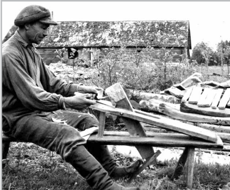
FIG. 110. Thinning down the board on cooper's bench. Avinurme, Vadi village. Photograph by author. Photo library 1089:72.
