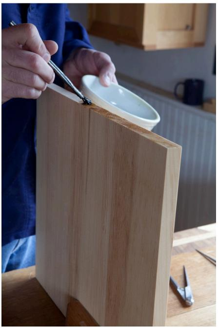
A minute for strength. The thin coat of glue size on the end grain is an important component of a strong rabbeted butt joint.
