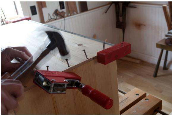
A clamp for safety. Clamping across the joint significantly reduces the chance you will split the top part of the joint or the board below. Note the alternating slopes of the nails.
