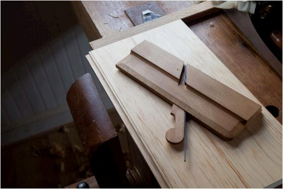
A strong bead. Bead the shoulder of the tongue section of the joint. If you bead the groove section you will weaken the joint.
