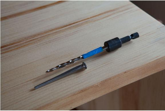
Tape marks the stop. The pilot hole should stop short so the nail has to burrow its way into the material. Here I'm using a tapered drill bit for the pilot holes. It isn't strictly necessary, but it helps.
