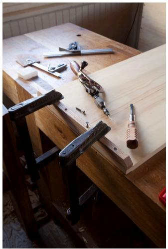
Screws that move. By elongating the clearance holes in the battens the threads of the screw will stay tight in the lid without (usually) splitting.
