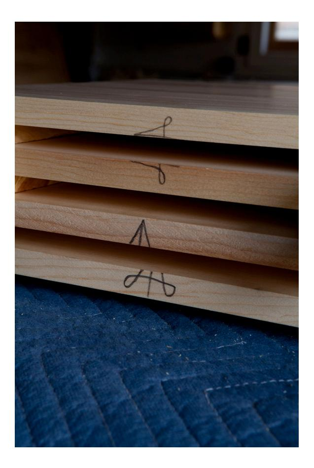
Two triangles. Mark the triangles on the top edge of your panels. Each triangle should point toward the front of the chest and be marked when the panel and its opposite part are placed together.
