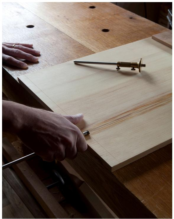
*Extra step.* Scribe in the width and depth of your rabbet with a cutting gauge. Then use these lines to guide you as you fine-tune the setting of your moving fillister plane.
