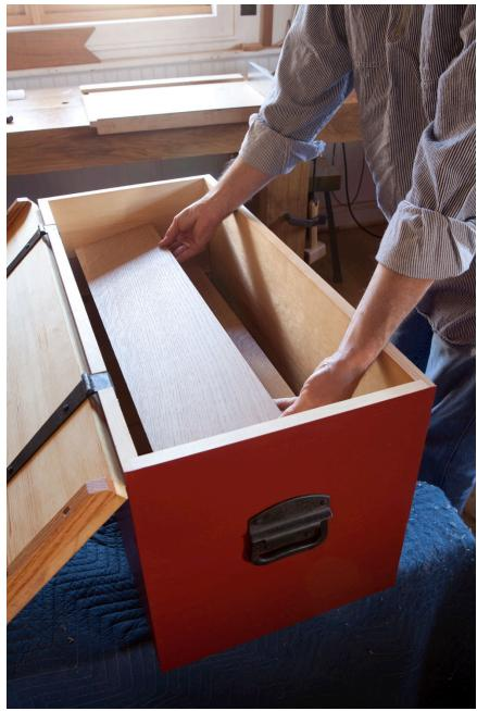
Shoot the bottom. After cutting the bottoms to a close size, shoot the ends until the bottom slides smoothly on its runners.
