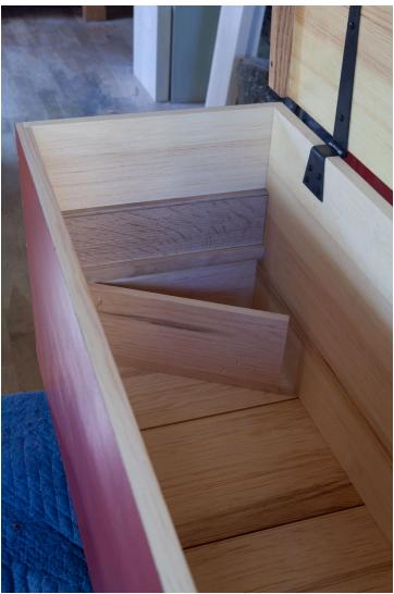
Permanent Jenga. The pine board shown at the bottom puts the lower runner in its correct position. After the first runner is in place, install the second runner on top of it. Then remove the spacer and repeat the process on the other end of the chest.
