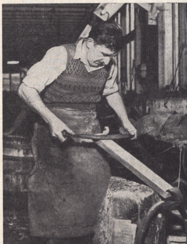
FIG. 2. SHAPING THE STAVES WITH A DRAW KNIFE
