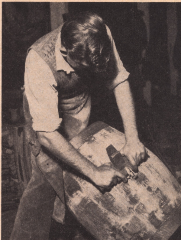
FIG. 3. FINISHING OFF THE OUTSIDE OF A BARREL The tool used here is the downright shave
