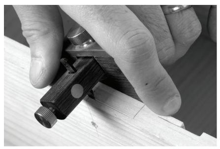
Here I'm using a cutting gauge to mark the front edge of the lockset on the top edge of the box. Then measure the thickness of this top plate and mark that on the inside of the box. Start wasting away this shallow mortise.
