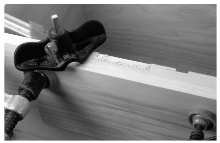
Router planes excel at this type of detail work. When you need mortises that are exactly the same depth (such as matching hinge mortises), a small router plane is the tool for the job.
