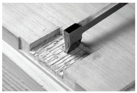
A drawer-lock chisel is great for this sort of close-quarters work. Score the waste with the drawer-lock chisel then remove the scored waste with a bench chisel by working from the top.
