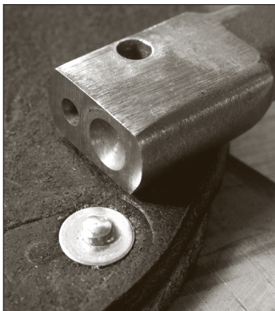
Fig. 6.14 Peened. Some people peen the rivet freehand with a hammer. I use a rivet setter, which makes a tidy dome. It's personal preference.
