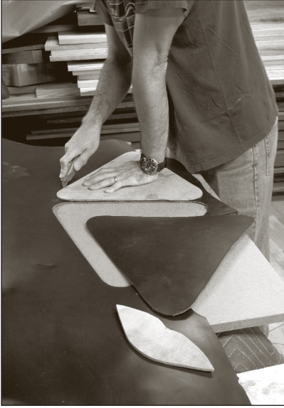
Fig. 6.9 Knife work. You will probably make more than one stool, so make plywood patterns of the seat parts and cut them out using a sharp utility knife.
