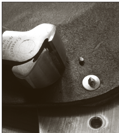
Fig. 6.13 Snip it. The post of the rivet should extend about 1/16 " or so from the burr. I use nail pincers to snip the post to length.
