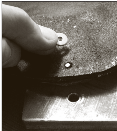
Fig. 6.12 Like a washer. The "burr" part of a traditional rivet is what pinches the leather. Place it over the post. Then drive it on the post with a rivet setter.
