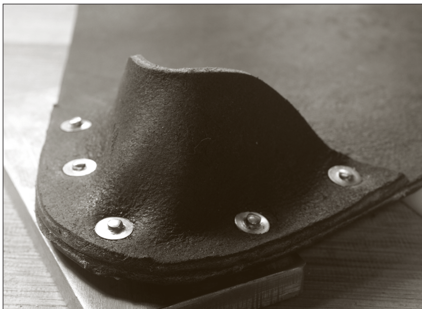
Fig. 6.15 Five rivets. Each pocket is secured with five rivets. One at the peak of the curve. Rivet the ends of the lips, then fill in with the rivets between.
