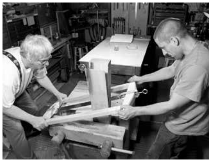
Fig. 4 The resawing bench is a fairly crude tool, but elegance is not really called for. My experience is that there is no way the bench portrayed in Figure 10 could have sufficed unless it was bolted to the floor. The only way I could get the bench to stop dancing across my concrete floor during sawing was to load it down with several hundred pounds of ballast.
