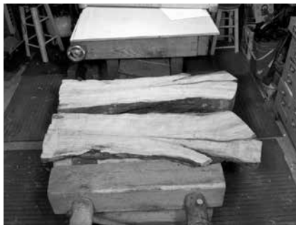
Fig. 5 Sawing this air-dried plum log was by no means effortless. With the tools and skills that I possess, it took us nearly three-quarters of an hour to saw this in half. Turning it into a complete flitch of veneers would have taken several days, and it raised my respect for the old craftsmen immensely.
