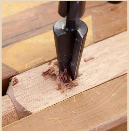
Loose, conical tenons. No glue.
