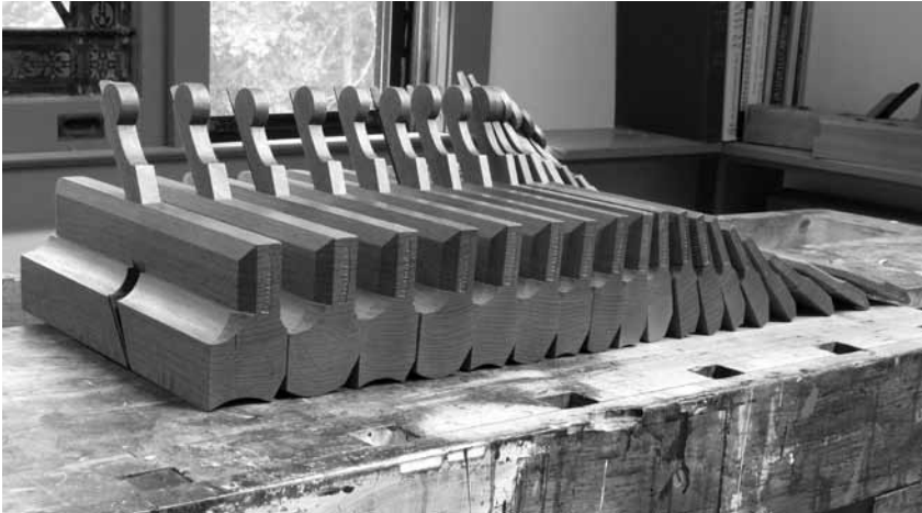
Fig. 3-1. A half set . This pictured half set is nearly all that you will need to reproduce the various moulded edges of all period pieces, regardless of period. It's also much more than many hobbyists will ever need.
