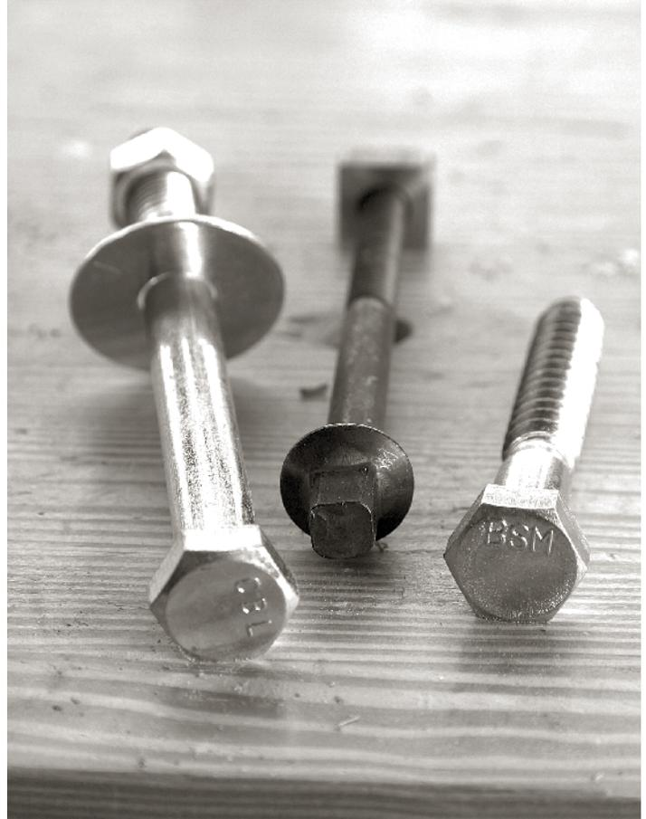
**QUICK OR COMPLEX.** You can use a simple lag bolt (right) to attach the top. Or you can use a through-bolting system that is typically used to attach the ends to the stretchers in the base.
