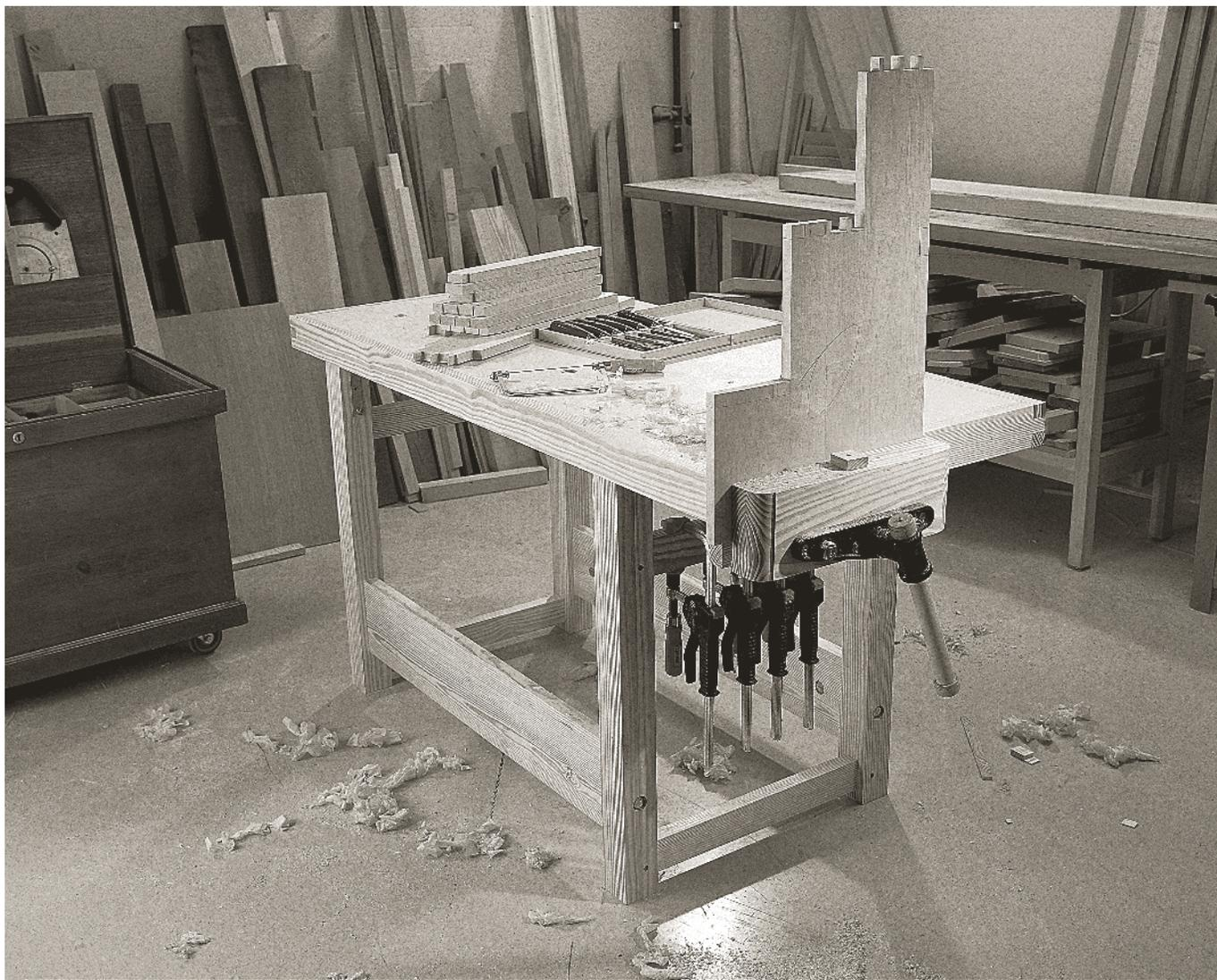
**BUILT TO TRAVEL.** This bench can be knocked flat in about 10 minutes with a  $\frac{3}{4}$ " ratchet set and a No. 3 Phillips screwdriver. I traveled all over the country with this workbench and became quite familiar with its assembly and disassembly. Finally, we gave the bench away to a reader of our magazine who won it in a contest. That guy made the moves on my managing editor, and so did the next reader who won one of my workbenches. So we stopped giving them away.
