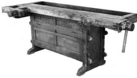
**TUSKS, IF YOU MUST.** Using tusk tenons creates a bench that can be knocked down without metal hardware, but the joinery does complicate the construction of the base.
