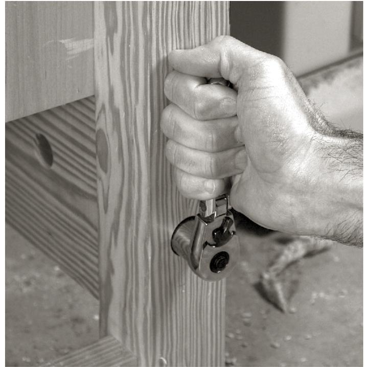
**THE VERITAS BENCH BOLT SYSTEM.** A few well-placed holes is all it takes to hold your bench together with the Veritas system. And tightening the bolts in the system is simple with a ratchet set – though mine have needed it only once in five years.
