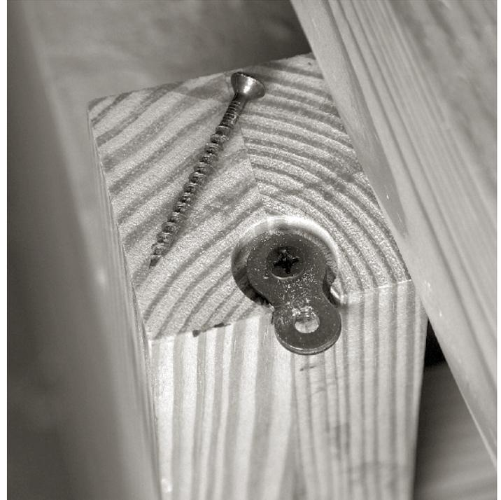
**TOUGH ENOUGH.** Here I attached the top to the base with a figure-8 fastener. The bench's rigidity is maintained by the stretchers below. So the method of attaching the base to the top is more about shear forces than racking forces. So the steel screws do the job quite well.
