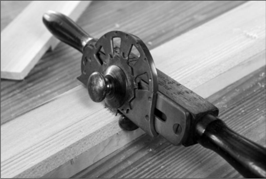
**Compared to a scratch stock.** My tool obsession knew few limits. This Windsor beader is a bit of a crazy multi-tool compared to a shop-made scratch stock. But I really wanted to try one out.
